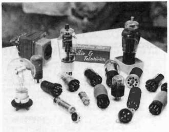
This selection of thermionic valves spans nearly sixty years of valve technology. A "semi-shrouded" mains transformer is shown in the background which was used to supply power to these valves. This (typical) one can supply 300-0-300V at 100mA, 6.3-0-6.3V at 6A, and 4V at 3A.
