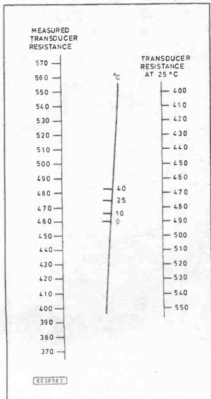
Fig. 8. Pressure transducer MPX100A resistance/temperature nomogram.
