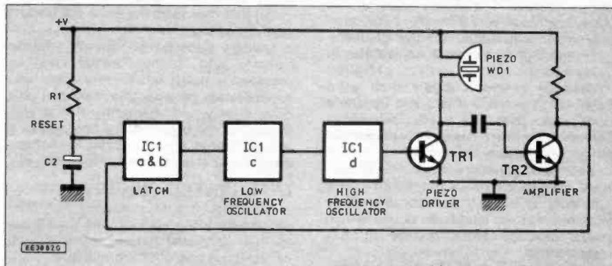
Fig. 1. Block diagram for the Vibration Sensitive Alarm.
