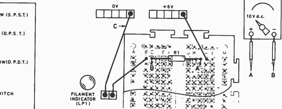
Fig. 1.7(b). Interwiring diagram. The locations "A" and "B" are connected to the positive and negative terminals respectively of your multimeter, set to a suitable voltage range. Repeat for BC and AC
