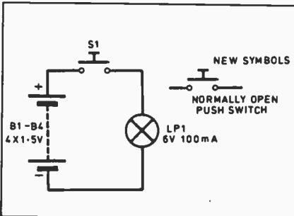
Fig. 1.2(a). Circuit with push switch.
