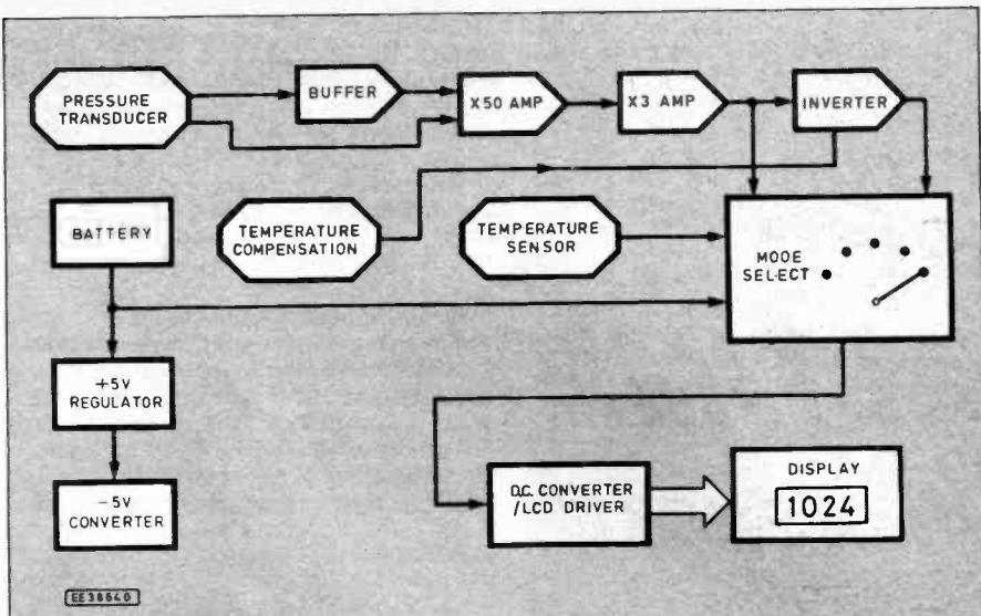
Fig. 4. Full block diagram for the EPE Altimet.
