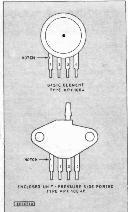
Fig. 12. Pressure transducer pintout details.
