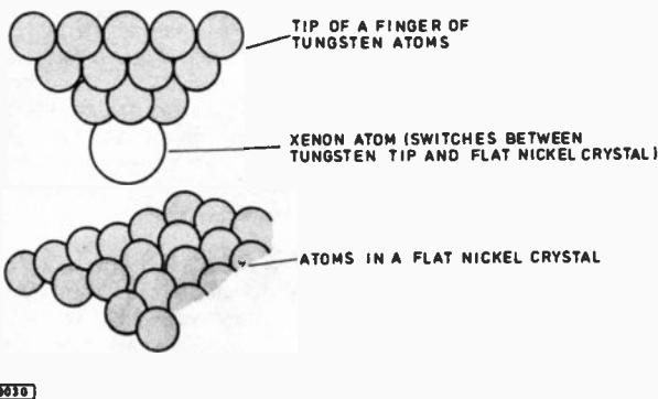
*Fig. 1. Structure of the atom sized switch.*
