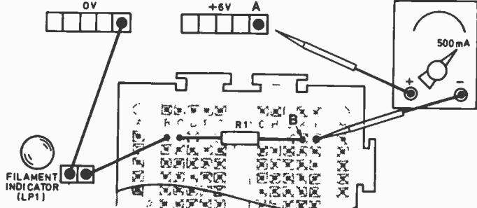
Fig. 1.7(d). Measuring current through the resistor and bulb.
