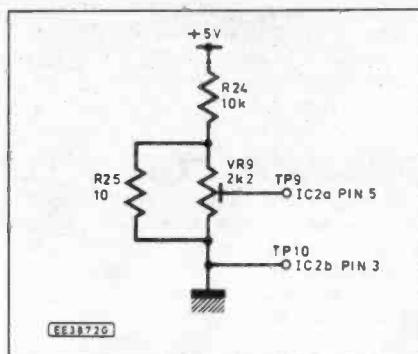
Fig. 13. Alignment and setting-up test circuit diagram.
