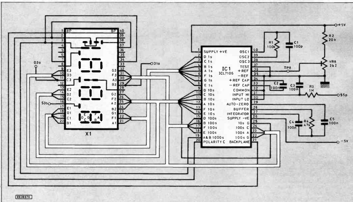
when VR5 and VR6 have been set to the relative span ranges for their mode scales, a common increase or decrease to the altitude and barometer mode gains can be effected by adjusting VR8.
