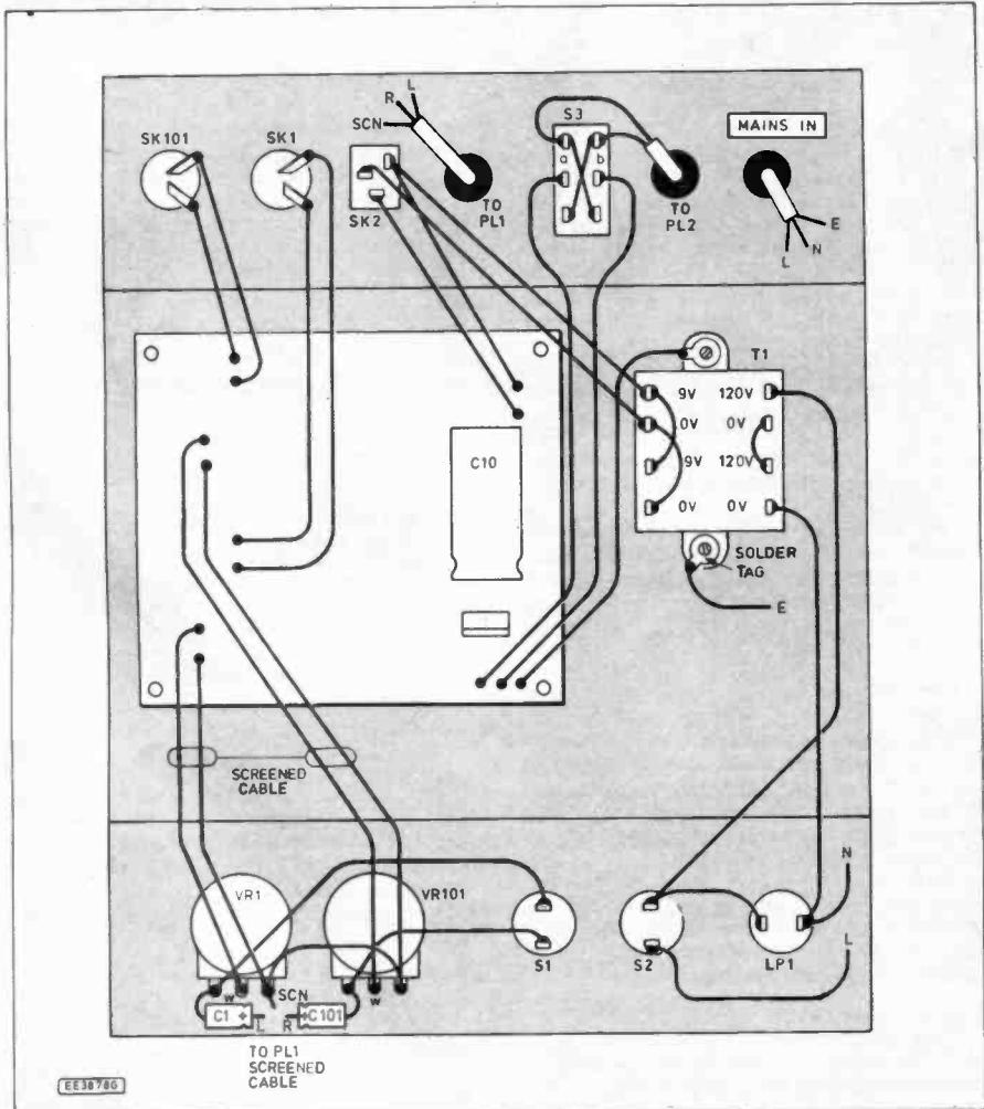
First though, examine your personal stereo and ascertain the diameter of the d.c. input socket and the headphone output socket. They will either be 2.1mm or 2.5mm, choose the correct type and fit them where shown.
