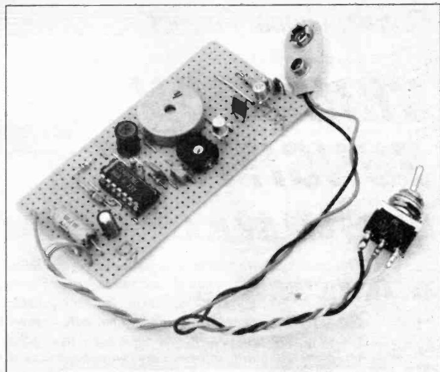
black, battery lead. This is to ensure that in the off position the electrolytic capacitor C2 is discharged.
