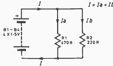
Fig. 1.9(a). Two resistors R1 and R2 in parallel across the 6V battery pack.
