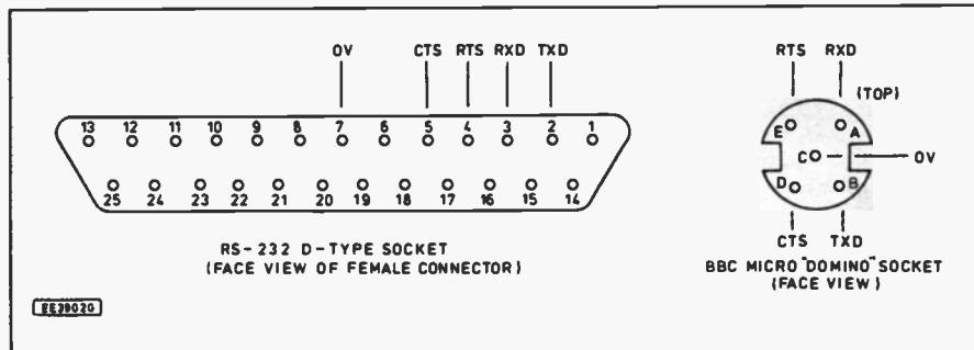
Fig. 3. Pin connections for the 25-way D-Connector.
