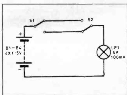
Fig. 1.5(a). Electrician's staircase lighting circuit.
