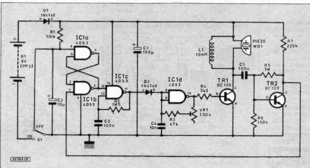
If an inductor is not readily available, it can be substituted with a resistor, typically 10 kilohms, and the unit will function as normal except for the reduced volume, which might still be sufficient in many cases.
