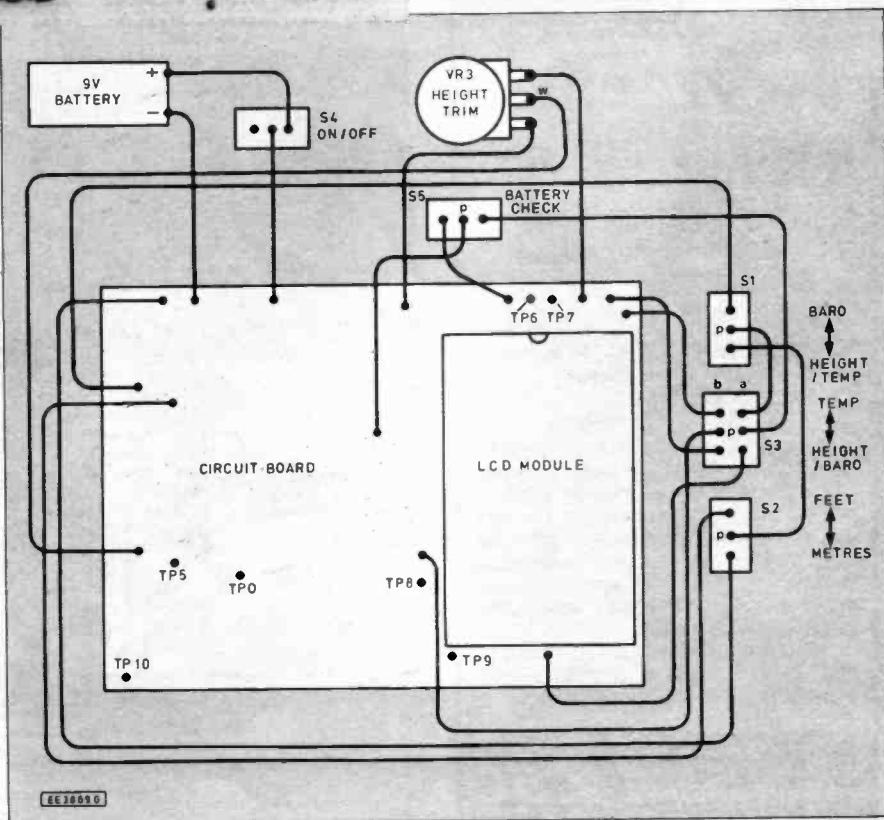
Setting-up falls into two parts, "workshop alignment" and fine tuning under "field conditions". Since the response of the transducer can vary in manufacture between 45mV and 90mV per 100kPa, the final alignment can only take place after subjecting the unit to known changes in barometric pressure, such as those experienced when using it at the top and bottom of a hill of known height.
