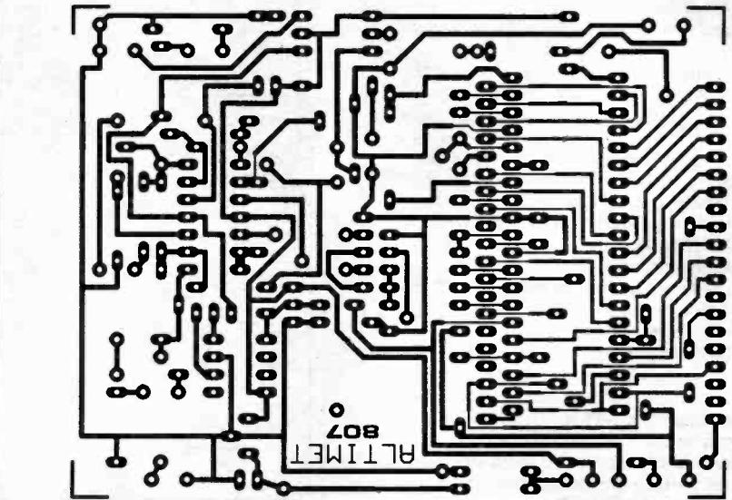
Fig. 9. Printed circuit board component layout and full size foil pattern.
