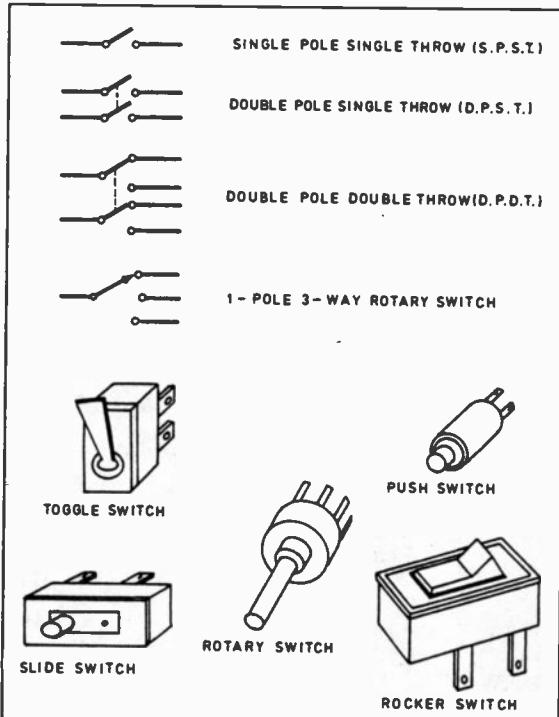
Fig. 1.6. A selection of switch types and styles.
