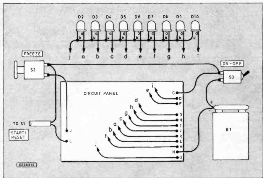
Fig. 3. Interwiring from the circuit board to the display I.e.d.s and other off-board components. Switch S1 is mounted inside the remote "tester" box.
