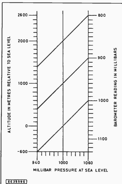
Fig. 2. Altitude to variable atmospheric pressure conversion graph.
