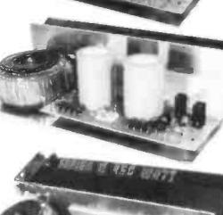
**OMP/MF 200** Mos-Fet Output power 200 watts R.M.S. into 4 ohms, frequency response 1Hz - 100kHz -3dB, Damping Factor > 300, Slew Rate 50V/uS, T.H.D. typical 0.001%, Input Sensitivity 500mV, S.N.R. -110 dB, Size 300 x 155 x 100mm.
