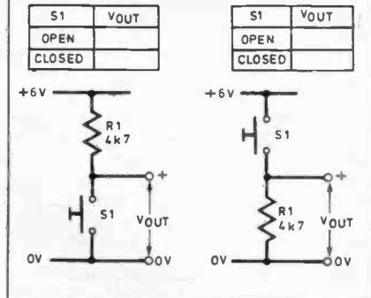
Fig. 1.12 (left). Switching System with Pull Up Resistor. Build this on the Mini Lab and record your voltage measurements in the table.
