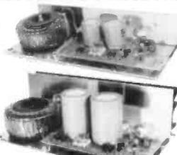
**OMP/MF 100** Mos-Fet Output power 110 watts R.M.S. into 4 ohms, frequency response 1Hz - 100kHz -3dB, Damping Factor > 300, Slew Rate 45V/uS, T.H.D. typical 0.002%, Input Sensitivity 500mV, S.N.R. -110 dB, Size 300 x 123 x 60mm.
