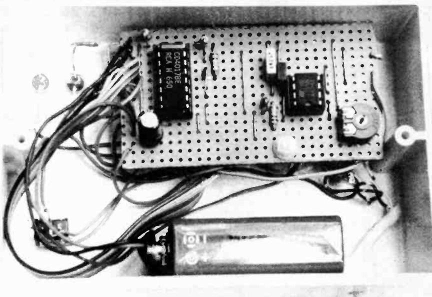
side to be held clear of the I.e.d. connections. A long 6BA nylon bolt with three nuts was used for the purpose in the prototype – one nut to secure the bolt and two to sandwich the circuit panel.
