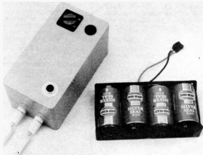
The mains supply unit (detailed in a later issue) and battery pack used with the Mini Lab.
