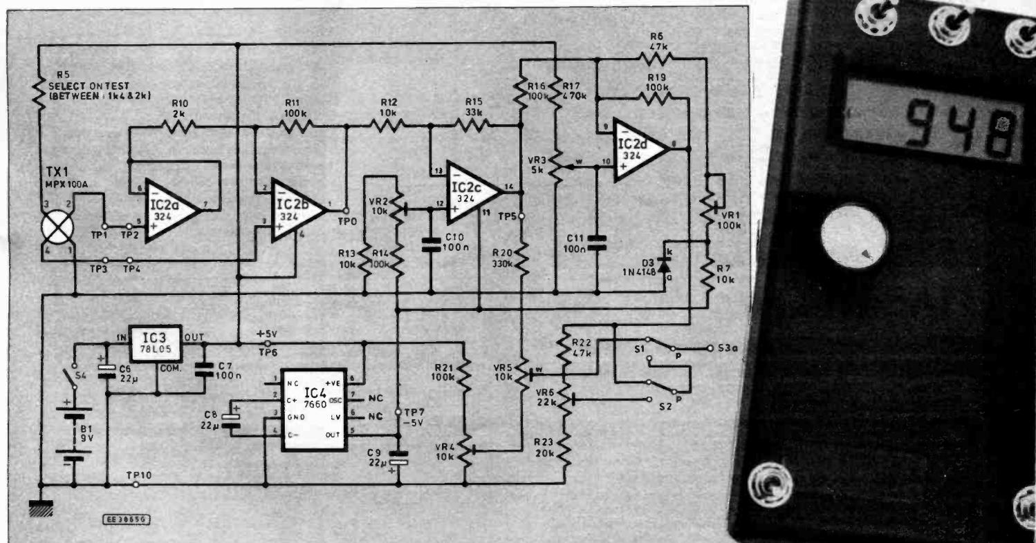
the Feet and Metres modes and feeds to switch S1 which selects between Height and Barometric modes.
