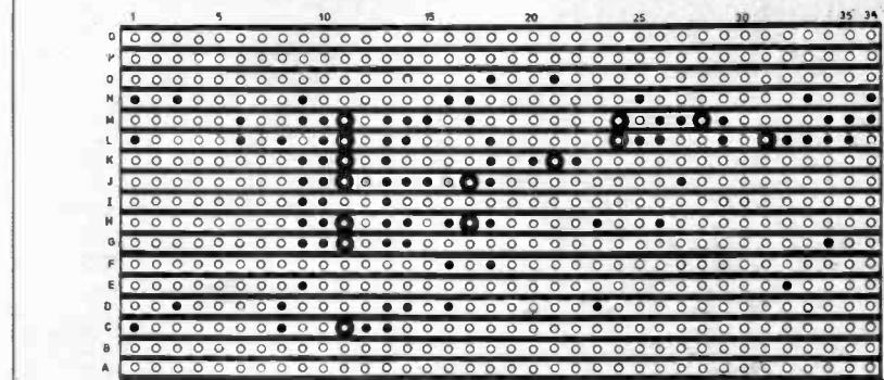
Fig. 3. Stripboard component layout and underside details of breaks required in the copper tracks.
