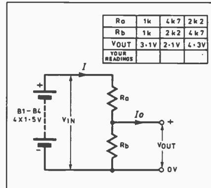
Fig. 1.10. The Potential Divider. Build this on the Veroblock yourself, and measure  $\text{V}_{\text{out}}$  (the voltage across  $\text{R}_b$ ) – fill in your results in the table.
