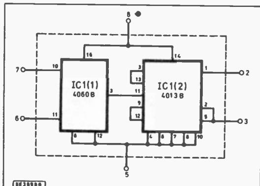
Fig. 1. Circuit diagram of the Daughter Board. Numbers outside the dotted line correspond to the original pin numbers.
