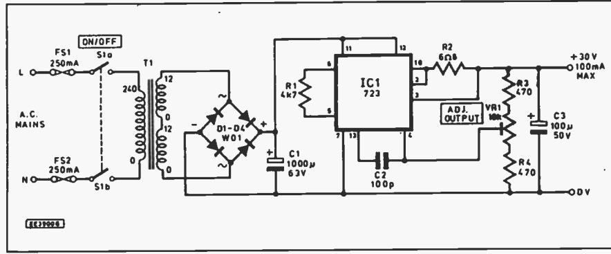
Fig. 2. Circuit of the 30V power supply.
