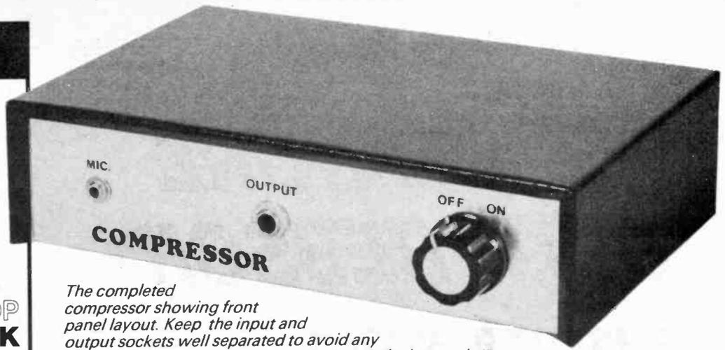
The completed compressor showing front panel layout. Keep the input and output sockets well separated to avoid any feedback pick-up from the output wires to the input wires.
