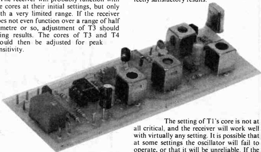
The setting of T1's core is not at all critical, and the receiver will work well with virtually any setting. It is possible that at some settings the oscillator will fail to operate, or that it will be unreliable. If the set will not work at all, or it only operates intermittently, try unscrewing the core of T1 slightly.
