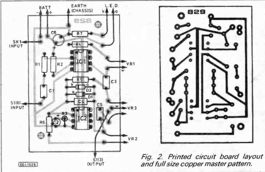
Fig. 2. Printed circuit board layout and full size copper master pattern.
