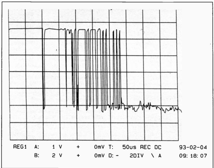
Fig. 7.5b. Switch bounce observed on the Mini Lab.
