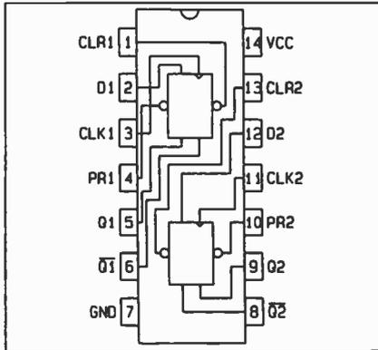
Fig. 7.7b. 74LS74 dual D-type flip-flop pin-out.
