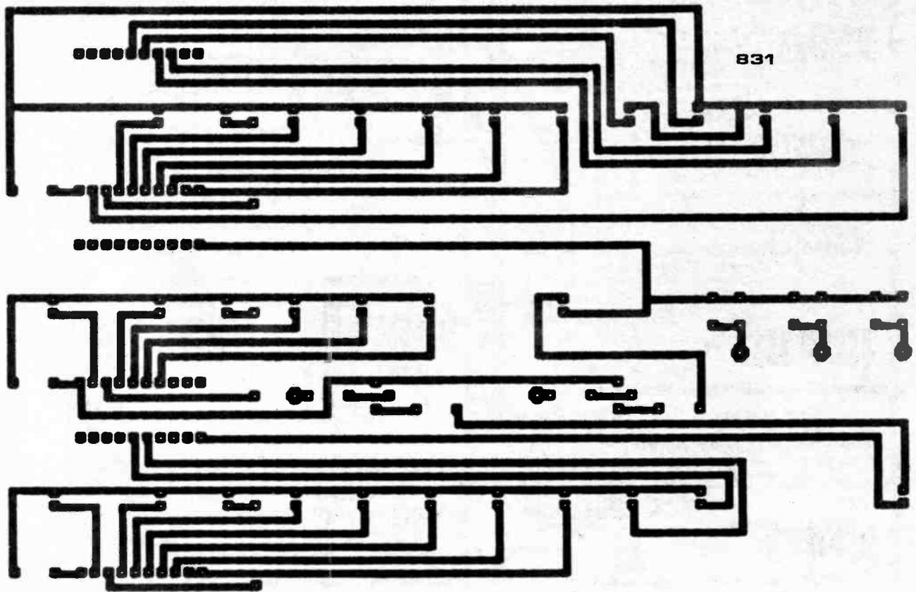
Fig. 7. Display printed circuit board component layout and full size copper foil master pattern. Note that the 10-way s.i.l. plugs PL1 to PL6 are mounted on the copper track side of the board, see Fig. 8.
