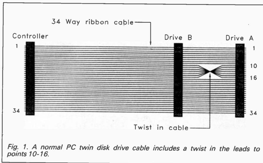
Fig. 1. A normal PC twin disk drive cable includes a twist in the leads to points 10-16.
