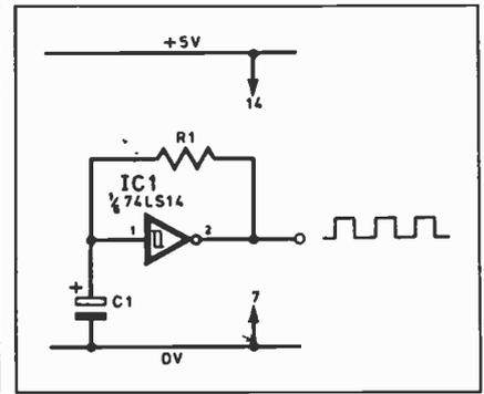
Fig. 7.9b. Using a Schmitt inverter to generate clock pulses.
