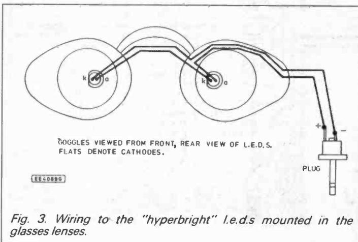
Fig. 3. Wiring to the "hyperbright" l.e.d.s mounted in the glasses lenses.
