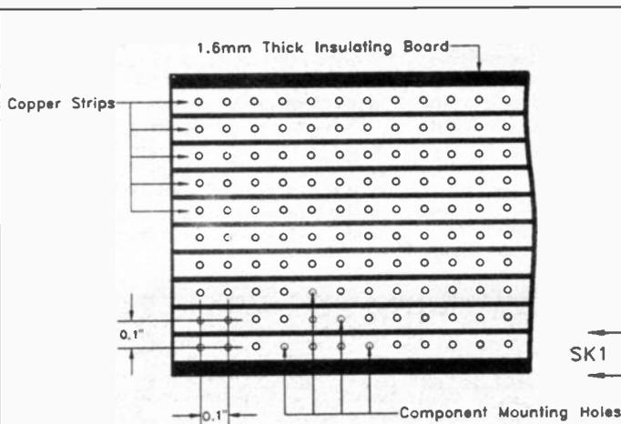
Fig. 1. Stripboard is basically very simple, but is extremely effective.
