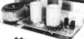
**OMP/MF 300 Mos-Fet** Output power 300 watts R.M.S. into 4 ohms, frequency response 1Hz - 100KHz -3dB, Damping Factor >300, Slew Rate 60V/uS, T.H.D. typical 0.001%, Input Sensitivity 500mV, S.N.R. -110 dB. Size 330 x 175 x 100mm.
