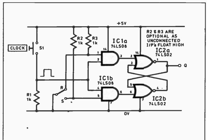
Fig. 7.6. Clocked SR flip-flop.
