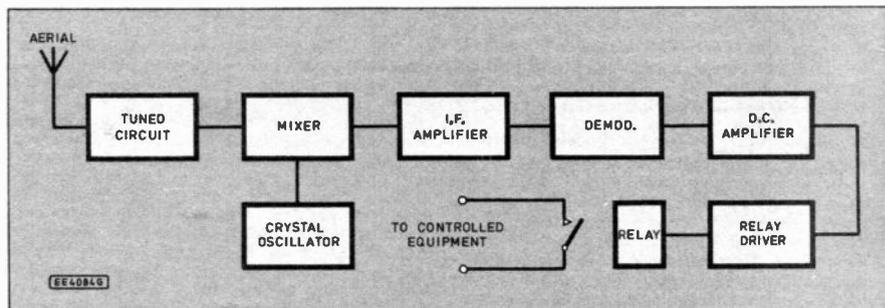
Fig. 1. The Superhet Radio Control Receiver block diagram.
