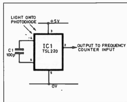
Fig. 7.17. Texas Instruments' light-to-frequency chip TSL220. For experimenters this could form the basis of many light-sensitive projects.
