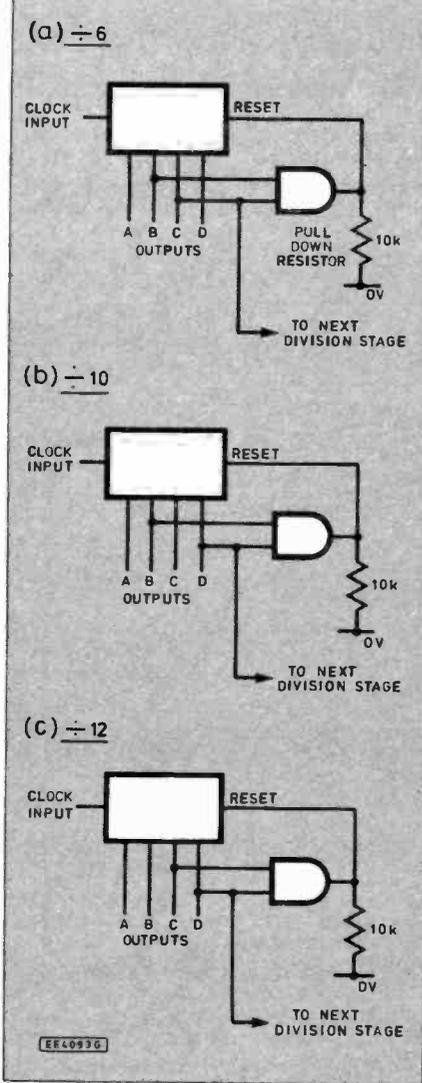
Fig. 4. The AND gate connections for  $\div 6$ ,  $\div 10$  and  $\div 12$  counters.
