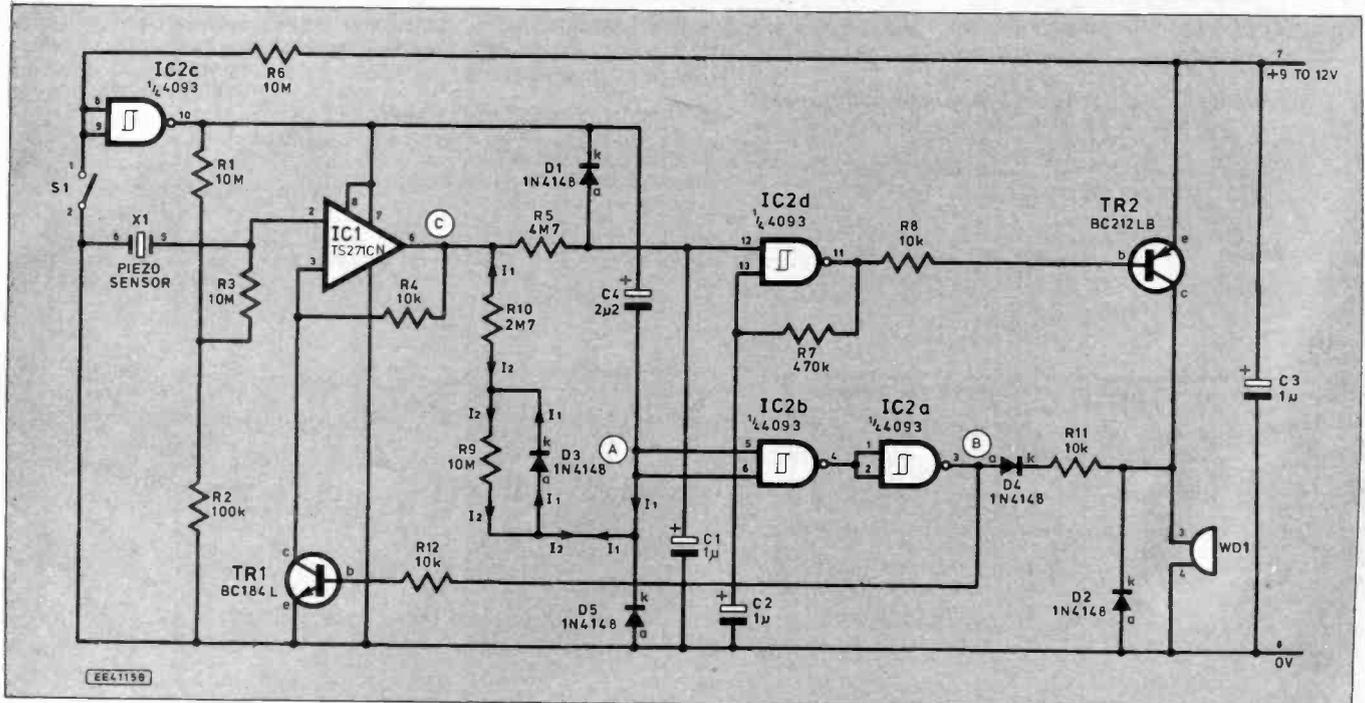
Fig. 1. Complete circuit of the Universal Alarm Module.
