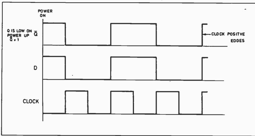
Fig. 7.10b. Timing diagram of the divide-by-two circuit.
