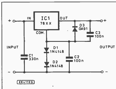
Fig. 2. Using a germanium diode as an output "protection" device.
