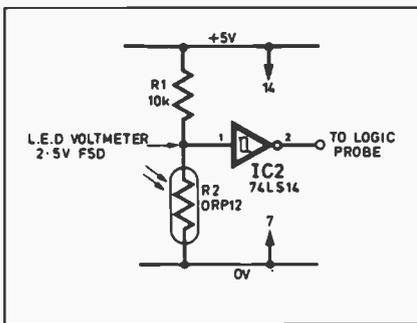
Fig. 7.3a. Light-sensor analogue-to-digital interface.
