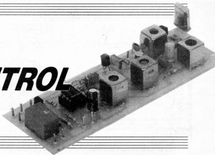
Improved operating range, up to 50 metres, and sensitivity is possible with the "superhet" receiver. No special test equipment needed for setting-up.
