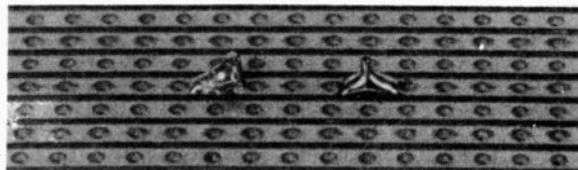
The right hand joint is a good one, with the solder covering the wire and track nicely. The joint on the left looks suspect.
