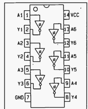
Fig. 7.2b. 74LS14 Hex Schmitt pin-out.
