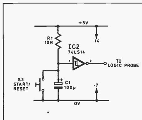
Fig. 7.2a. Time delay indicator.
