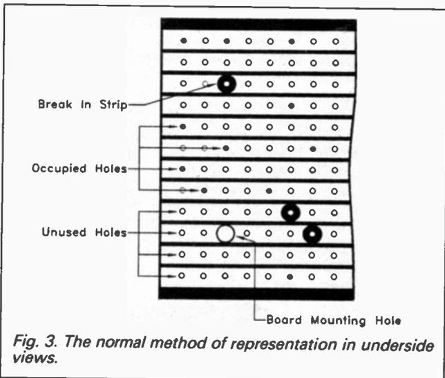
Fig. 3. The normal method of representation in underside views.
