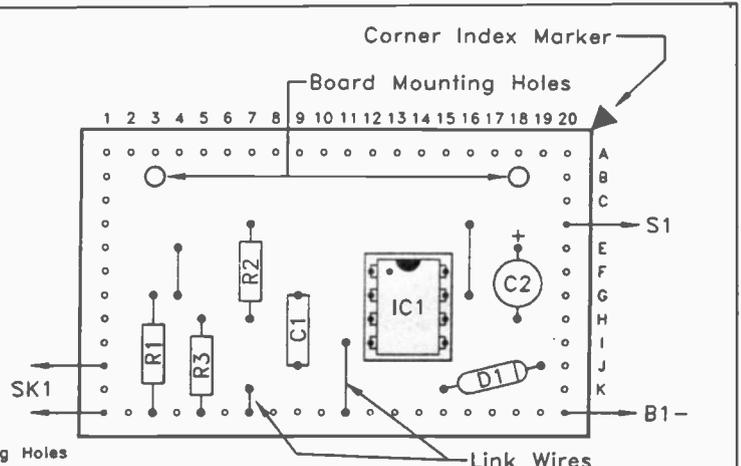
Fig. 2. Stripboard top views are often marked with identification numbers/letters for the columns and rows of holes.
