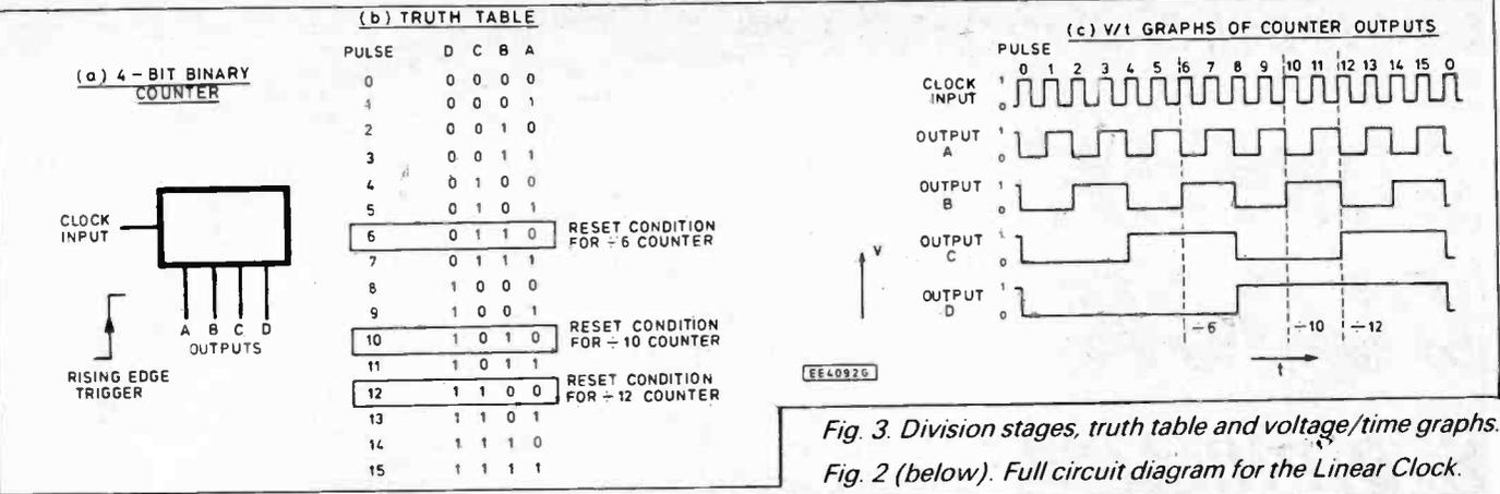
Fig. 3. Division stages, truth table and voltage/time graphs. Fig. 2 (below). Full circuit diagram for the Linear Clock.
