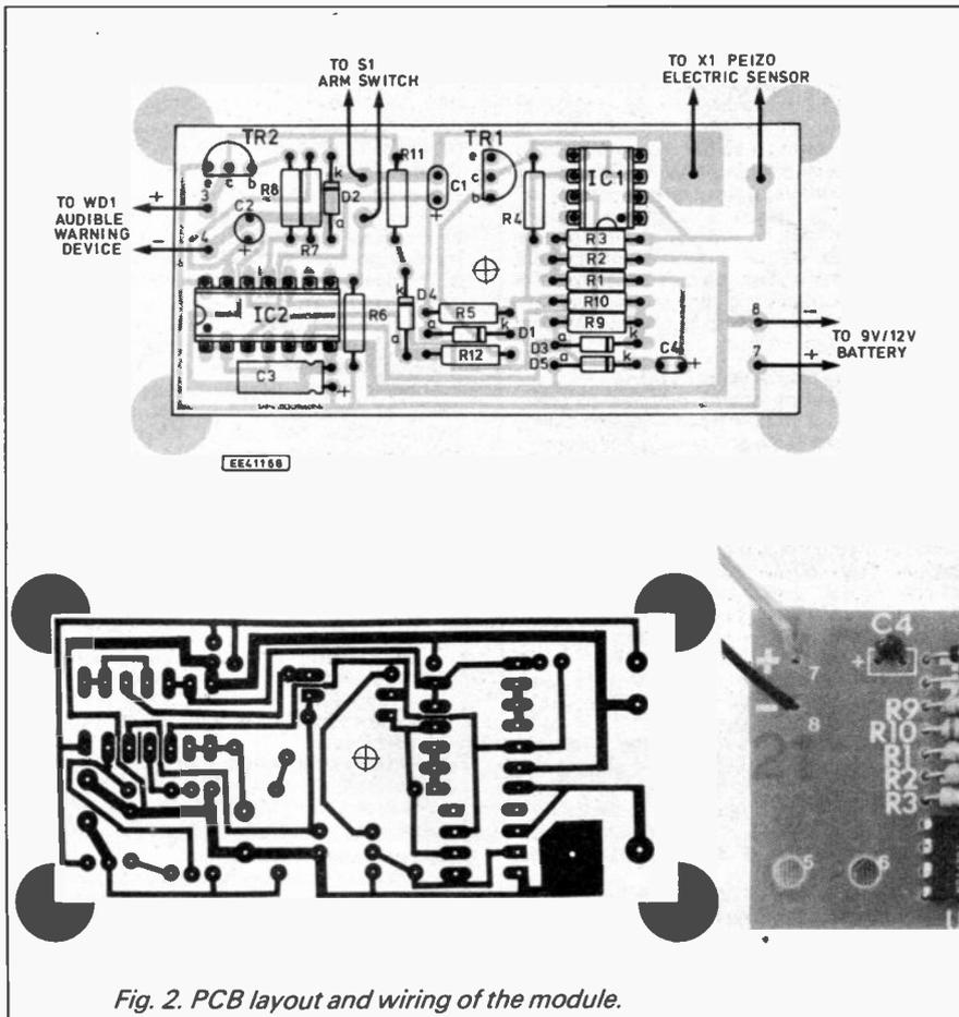
Fig. 2. PCB layout and wiring of the module.
