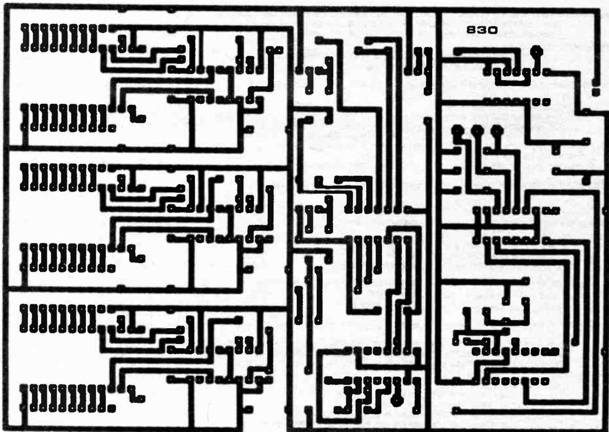
Fig. 6. Printed circuit board component layout and full size copper master pattern for the main Timing board. All i.c.s should be mounted in d.i.l. sockets and the wire links must be made with insulated wire; double check all link connections before moving on to the discrete components.
