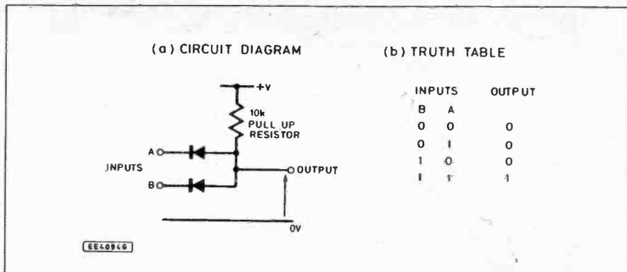
Fig. 5. The diode/resistor AND gate circuit and truth table.
