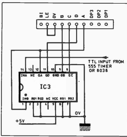
Fig. 7.13. Decoding a 4-bit binary number into decimal, using the Mini Lab Digital Display. Use both the 74LS93 and 74LS90 decoder chips in turn.
