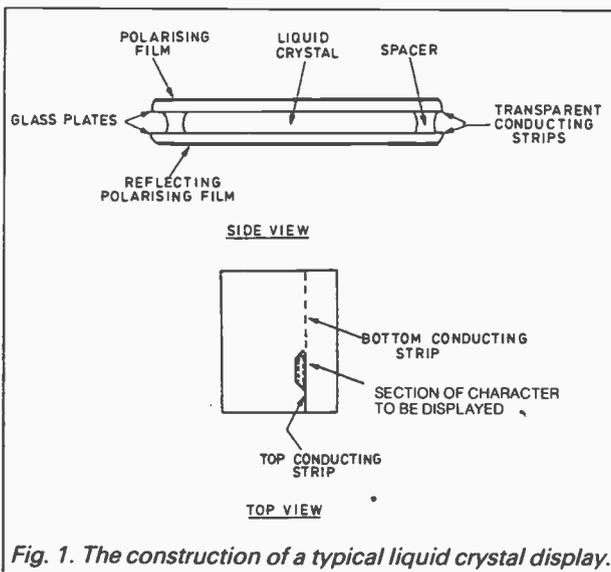
Fig. 1. The construction of a typical liquid crystal display.
