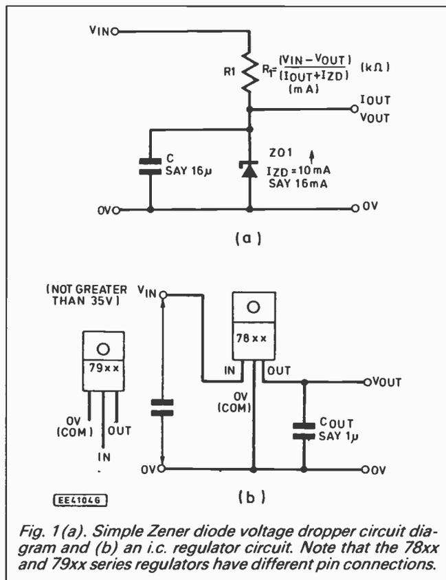
Fig. 1 (a). Simple Zener diode voltage dropper circuit diagram and (b) an i.c. regulator circuit. Note that the 78xx and 79xx series regulators have different pin connections.
