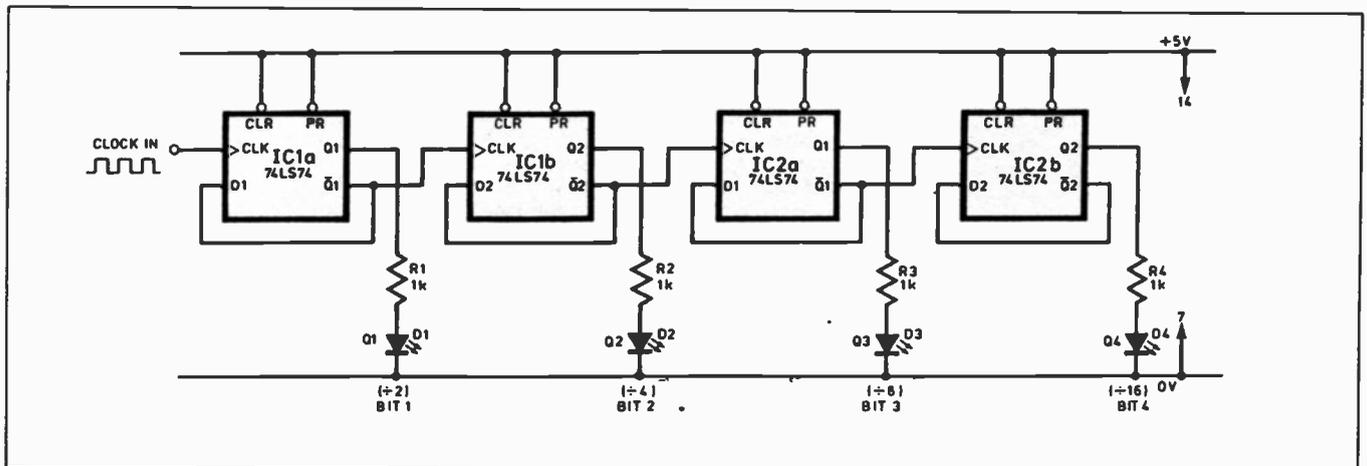
Fig. 7.12. A complete 4-Bit binary counter.
