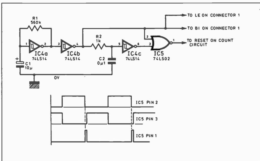
Fig. 7.16. A suggested digital frequency meter.
