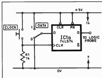
Fig. 7.8. Demonstration of the "D-type" latch.
