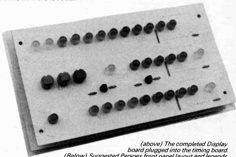
(above) The completed Display board plugged into the timing board.
