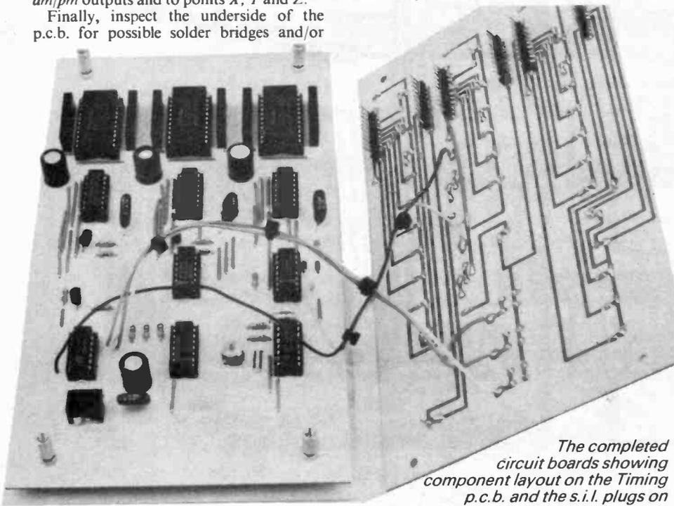
The completed circuit boards showing component layout on the Timing p.c.b. and the s.i.l. plugs on the track side of the Display p.c.b.
