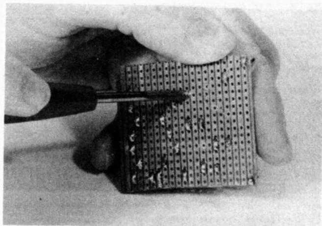
Stripboard (or Veroboard) tracks can be cut using the special tool available or a small (7mm or 8mm) hand held drill bit.
