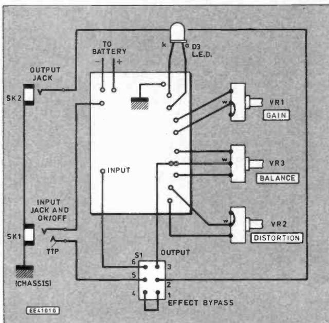
The completed unit. A solder tag should be inserted under the fixing bolt, and a lead taken from the tag to the Earth (Chassis) point for the jack sockets.
