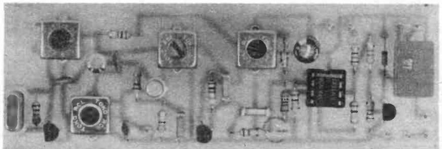
Fitting a printed circuit mounting HC-25U socket on the board and then plugging the crystal into this is a much neater solution. It also makes it much easier to change the crystal if you need to move the system to a different channel. However, if the receiver is likely to be subjected to a lot of vibration it is probably best to mount a pair of solder-pins on the board, and then carefully solder the crystal onto these.
