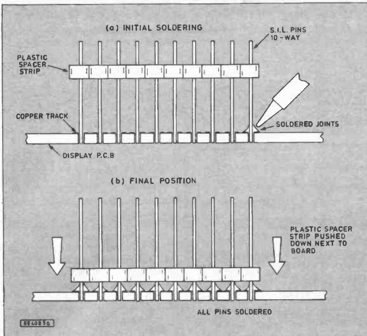
Fig. 8. Fitting s.i.l. pins to the track side of the display board.
