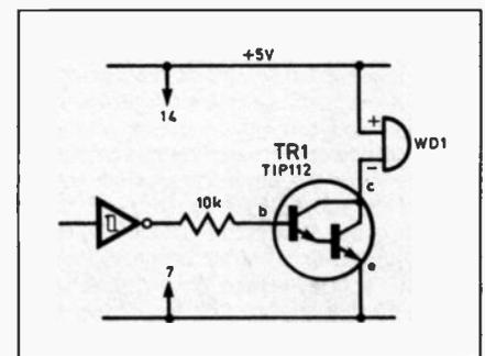
Fig. 7.4a. Driving a load through a buffer.
