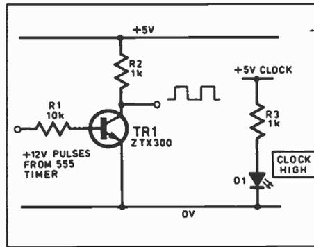
Fig. 7.9a. 12V to 5V TTL interface, for the 555 Timer.
