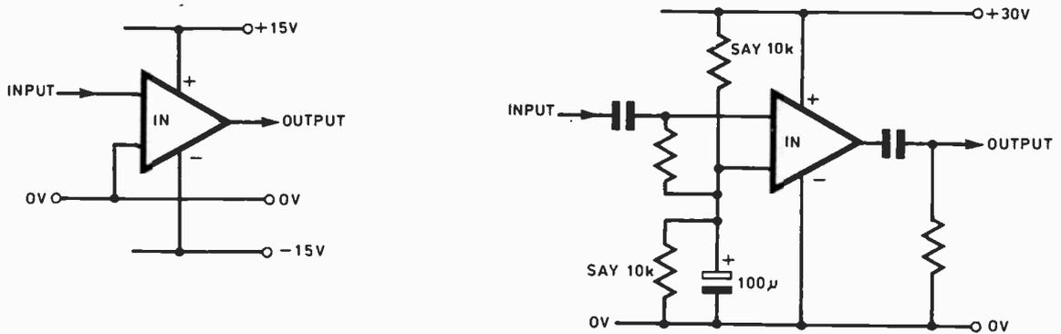
Fig. 3. An amplifier supplied by a pair of d.c. lines can often be rearranged to operate from a single supply line.
