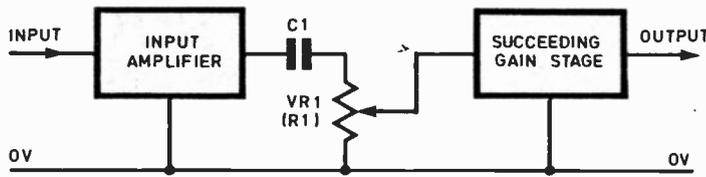
Fig. 6. Inserting a gain control (VR1) between the input amplifier and succeeding gain stage.
