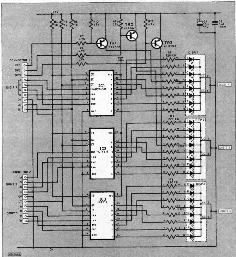
Fig. 1. Complete circuit diagram of the Display module.
