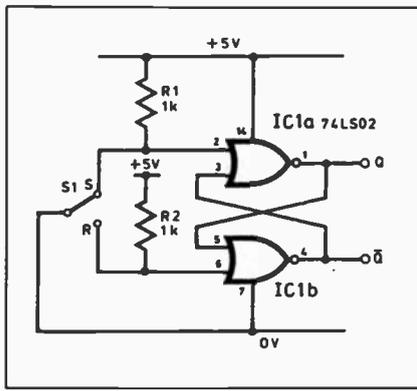
Fig. 7.5a. Bistable of "flip-flop".
