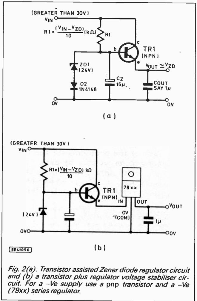
Fig. 2(a). Transistor assisted Zener diode regulator circuit and (b) a transistor plus regulator voltage stabiliser circuit. For a -Ve supply use a pnp transistor and a -Ve (79xx) series regulator.
