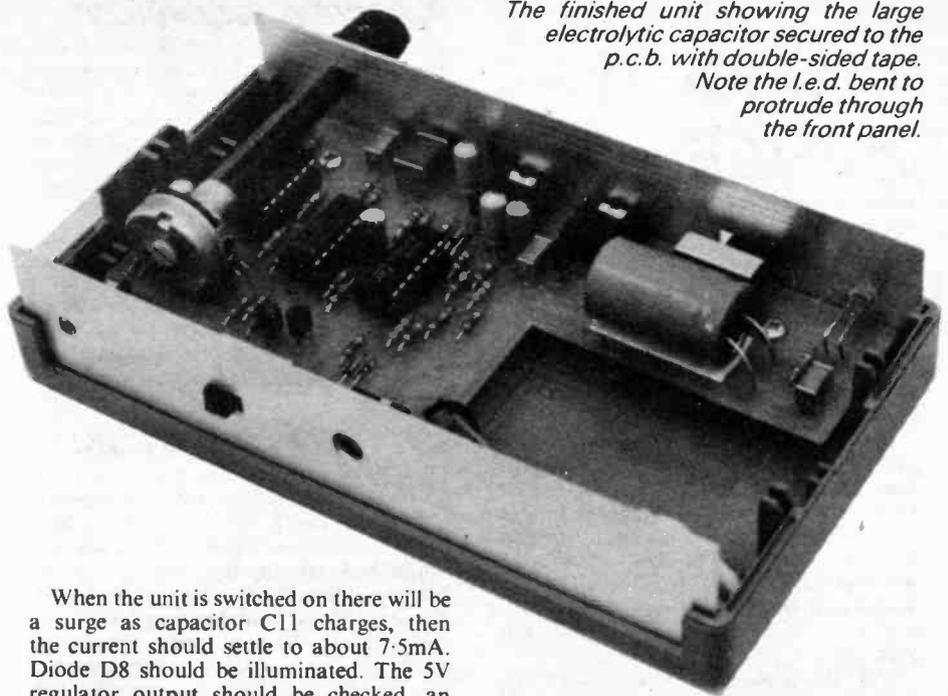
The finished unit showing the large electrolytic capacitor secured to the p.c.b. with double-sided tape. Note the l.e.d. bent to protrude through the front panel.
