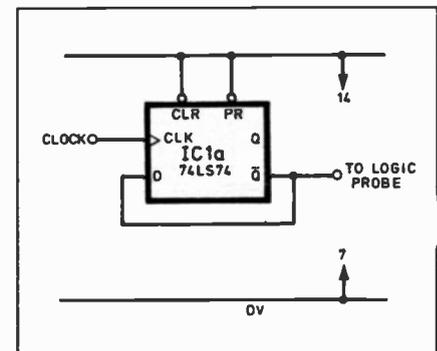
Fig. 7.10a. Divide-by-two function using a D-type flip-flop.
