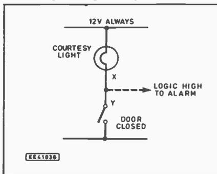
Fig. 1. Using the courtesy light switch to trigger the alarm. When the door is open a logic low is registered by the alarm.
