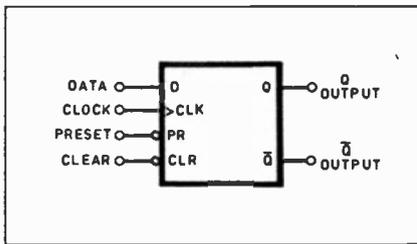
Fig. 7.7a. "D-type" flip-flop.
