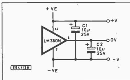
Fig. 3. Obtaining a split-supply voltage using the LM380N audio amp i.c. Note that pins 3, 4, 5 and 10, 11, 12 must be connected to the negative line.
