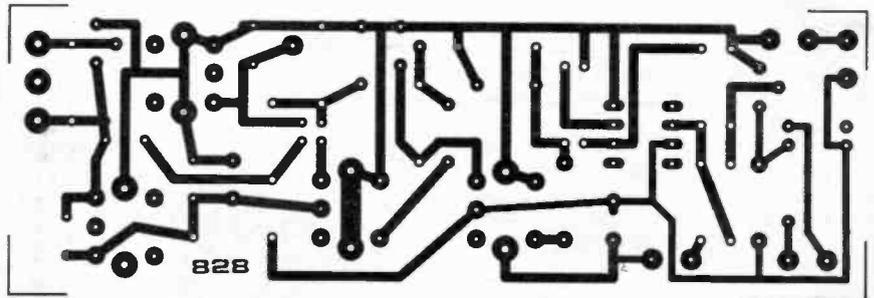
Fig. 3. Printed circuit board component layout and full size copper foil master pattern. As the metal "can" of transformer T4 completes the battery negative line (B1 -) connection, extra care should be taken to ensure that the mounting lugs are securely soldered to the board. The completed circuit board is shown in the photograph below.
