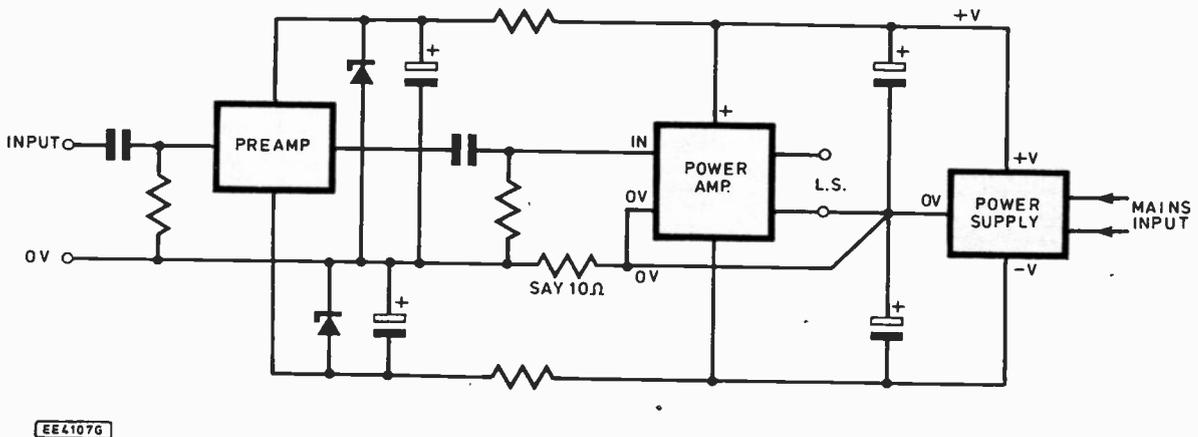
Fig. 4. Typical "0V" line connection between a preamplifier and a power amplifier.
