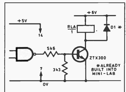
Fig. 7.4b. Using a bipolar transistor to buffer a gate.
