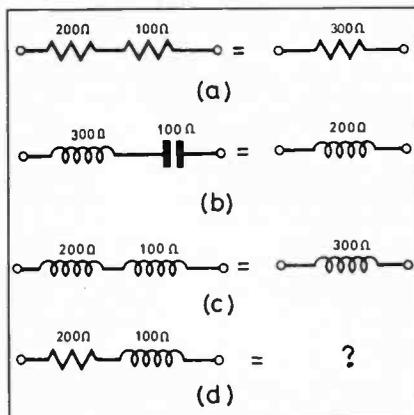
Fig. 1. Impedances in series and their simplified equivalents.
