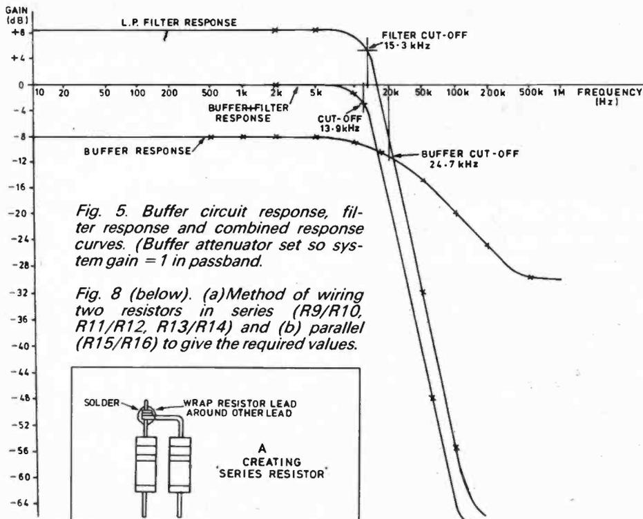
Fig. 5. Buffer circuit response, filter response and combined response curves. (Buffer attenuator set so system gain = 1 in passband.)
