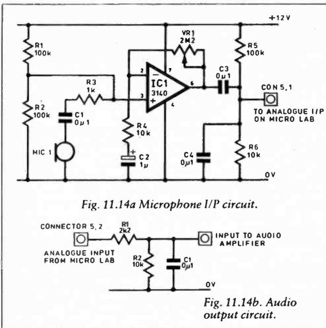
Fig. 11.14a Microphone I/P circuit.
