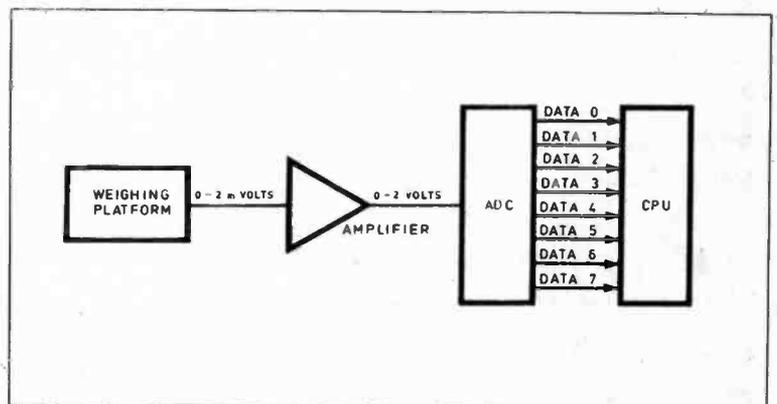
Fig. 11.2. ADC used in weighing application.
