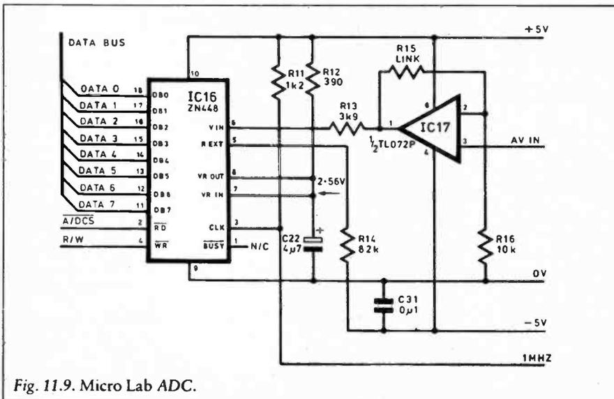
Fig. 11.9. Micro Lab ADC.
