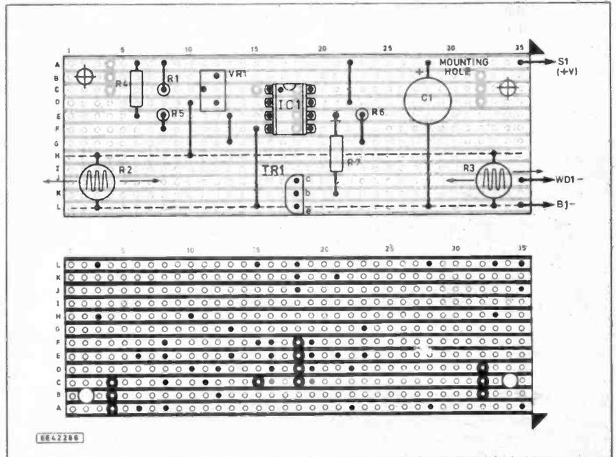
Fig. 2. Stripboard component layout and details of breaks required in the underside copper tracks. Layout of components inside the box is shown below.
