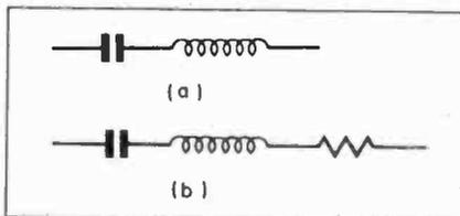
Fig. 2. Equivalent electrical circuit for capacitors.
