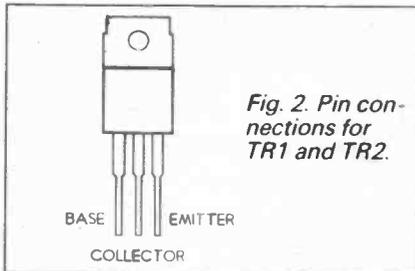
Fig. 2. Pin connections for TR1 and TR2.
