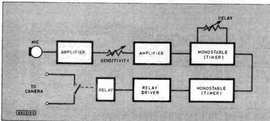
Fig. 1. The Sound Activated Camera Trigger block diagram.
