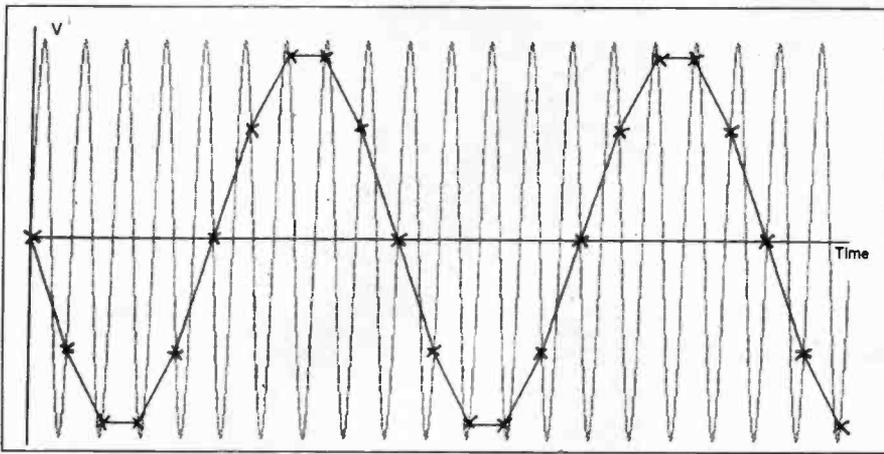
Fig. 11.12. Aliasing – A 10kHz signal sampled at 9kHz (x = sample) gives a 1kHz output signal.
