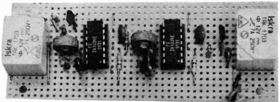
Component layout on the completed stripboard.
