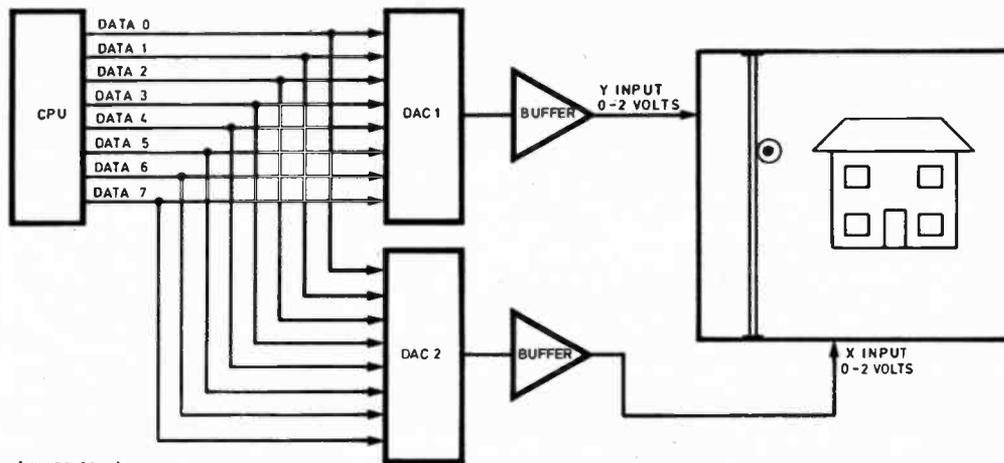
Fig. 11.3. DAC used in X-Y plotter.
