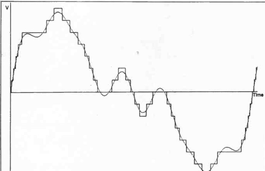
Fig. 11.13a. Waveform quantisation with 16 Levels.
