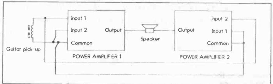
Fig. 5. Two amplifiers in a bridge configuration (20W output).
