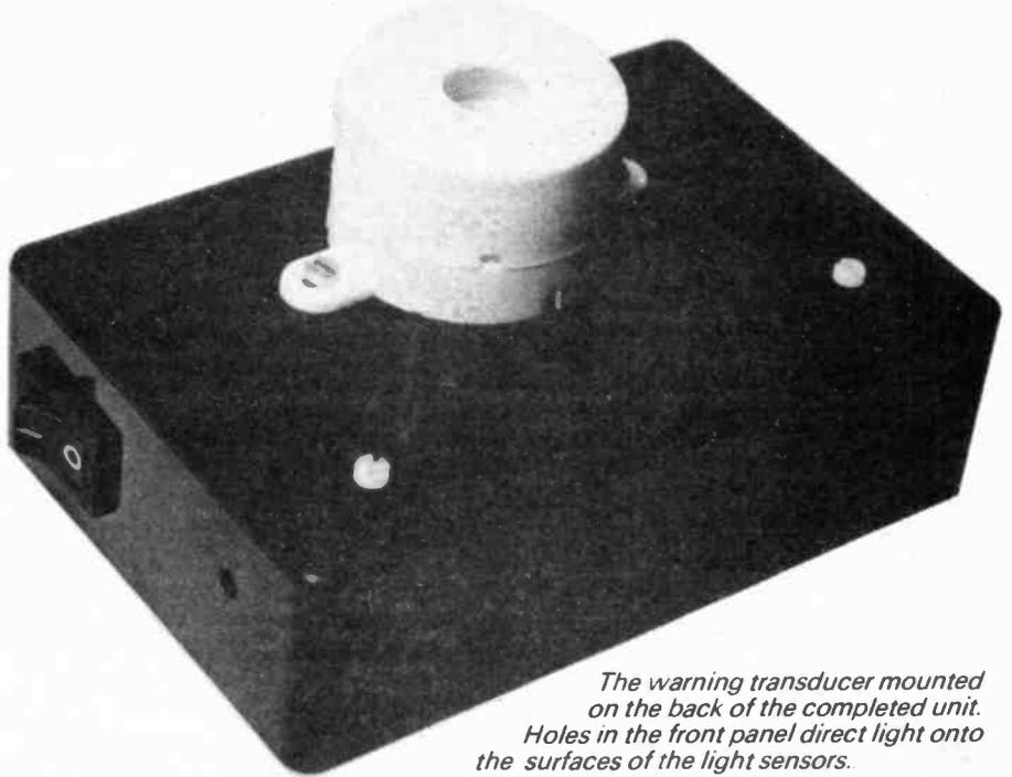
The warning transducer mounted on the back of the completed unit. Holes in the front panel direct light onto the surfaces of the light sensors.
