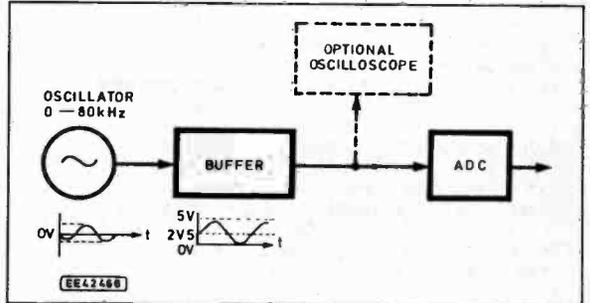
Fig. 13 (above right). Testing the effect of the software low pass filter.
