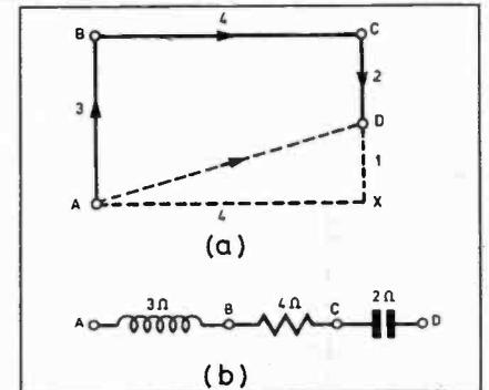
Fig. 3. A more complex circuit can be simplified by geometry. (a) The journey from A to B to C to D covers the "crow's flight" distance AD. This can be calculated from AX and DX. (b) Circuit equivalent to (a).
