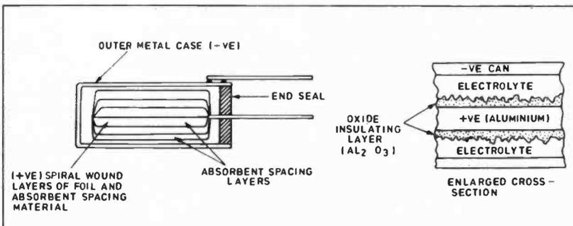
Fig. 4. Aluminium electrolytic capacitor (radial lead type).
