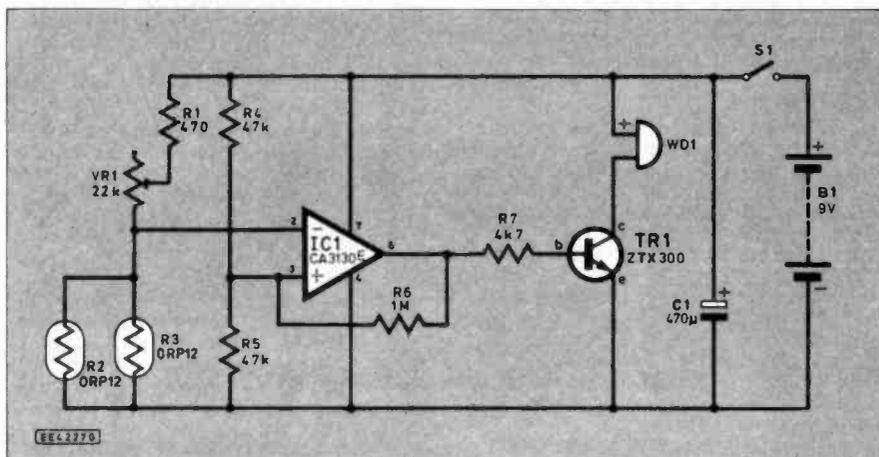
Fig. 1. Complete circuit diagram for the Light Work tester
