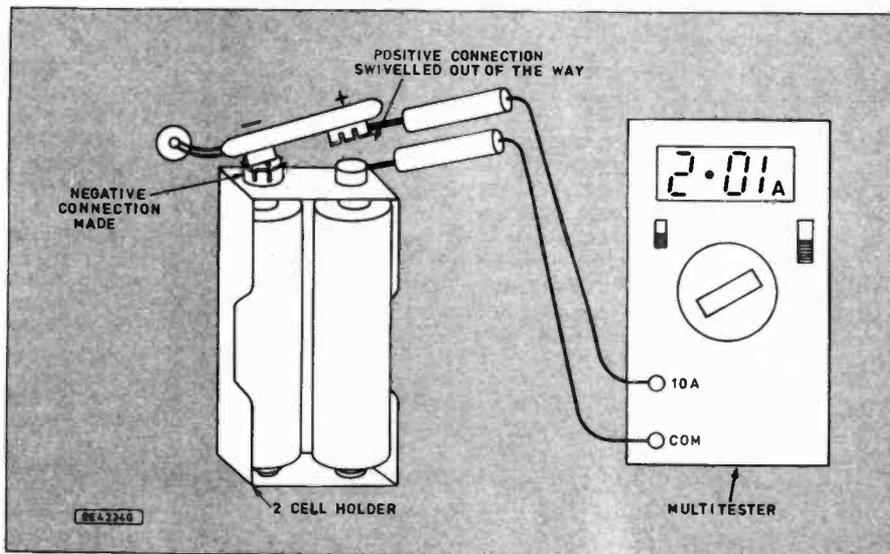
Fig. 4. Using test meter, set to amperes range, to check charging current.
