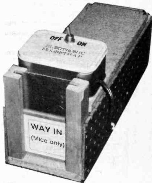
The finished Electronic Mousetrap with the Perspex "edible" top replaced with chipboard.
