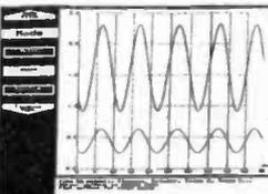
Storage oscilloscope with trigger and timebase. Traces can be printed and saved. Multiple meters onscreen. Real time spectrum analysis.
