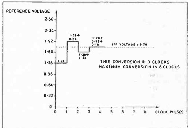
Fig. 11.8. Successive approximation ADC operation.
