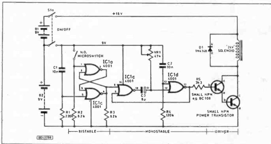
Fig. 1. Full circuit diagram of the Electronic Mousetrap.
