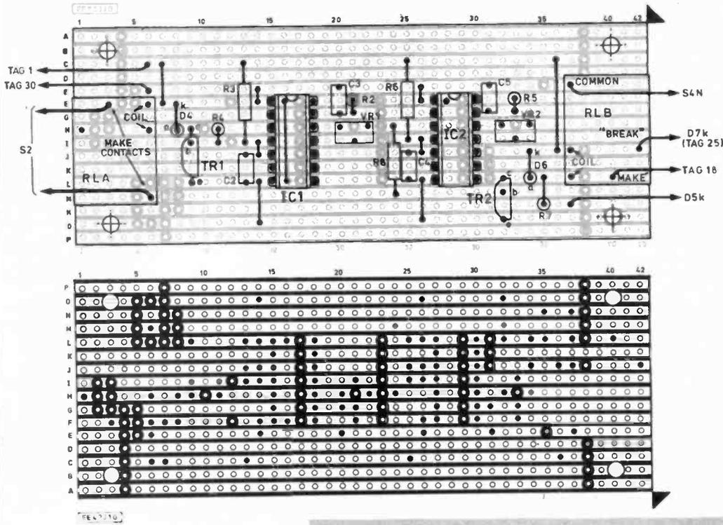
Fig. 2. (left). Striboard component layout and details of breaks required in the underside copper tracks.
