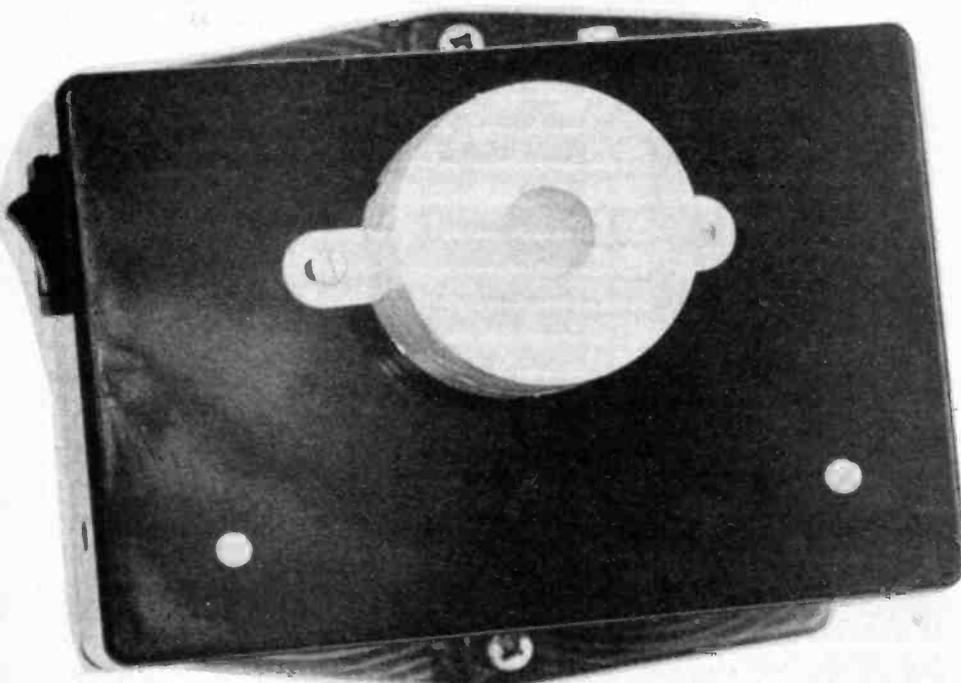
The completed Light Work mounted on a light cluster. Method of mounting can be by rubber suckers or Velcro strips.
