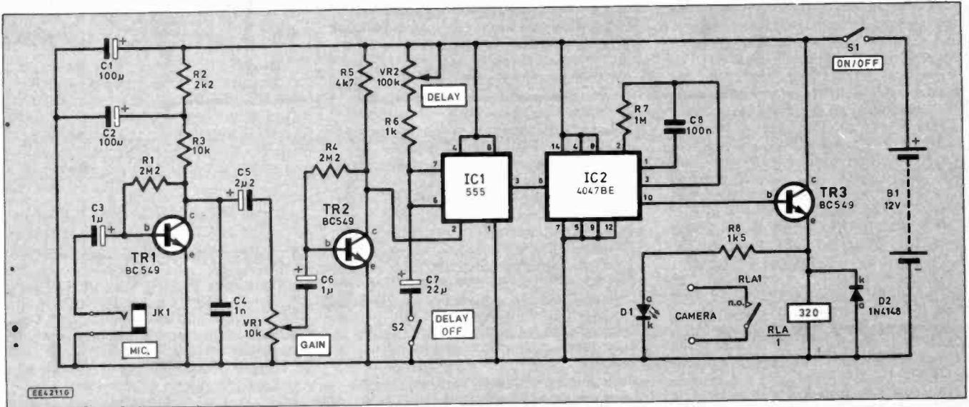
might seem to be an old fashioned method of controlling the camera, but the circuit that is being controlled is something of an "unknown quantity". The mechanical contacts of a relay should control any camera or motor drive properly, whereas semiconductor switching devices might fail to give satisfactory results.
