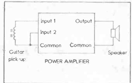
Fig. 4. Single-ended configuration (5W output).
