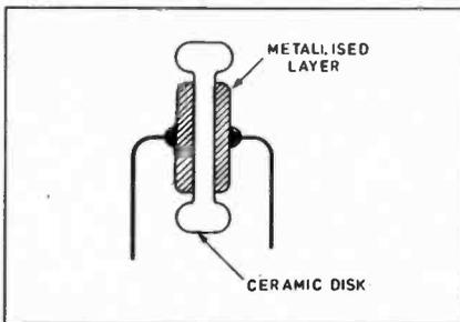
Fig. 3. Ceramic capacitor construction.
