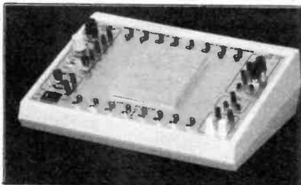
The model MS101 is a self contained mini lab which can be used without additional external equipment. The special features will enable you to move up the learning curve in digital electronics.
