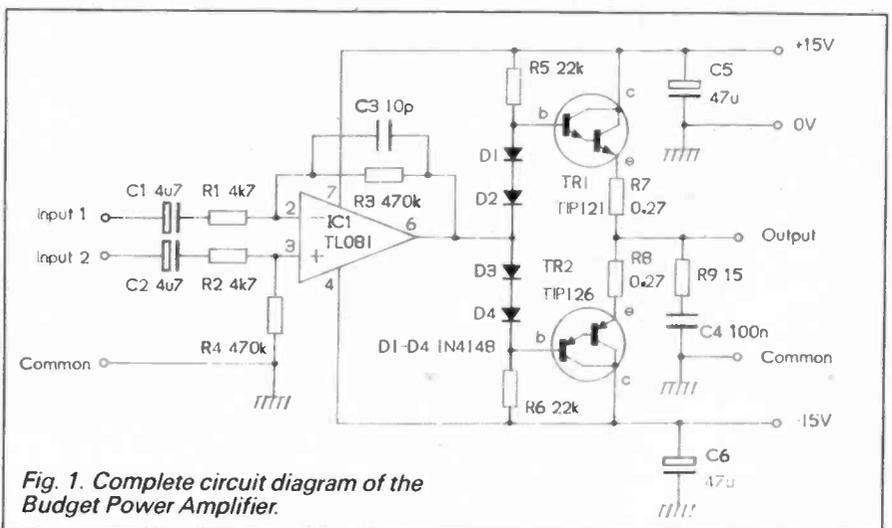
Fig. 1. Complete circuit diagram of the Budget Power Amplifier.
