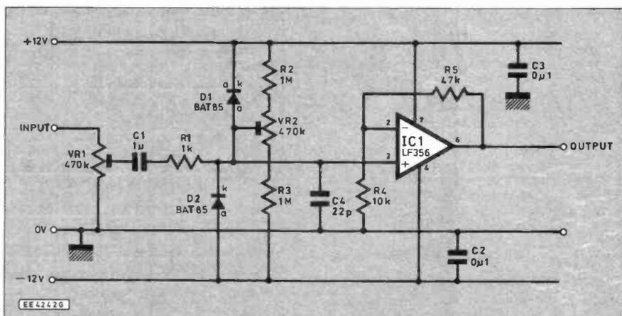
Circuit diagram for a simple Single I.C. Pre-amplifier (non-inverting).
