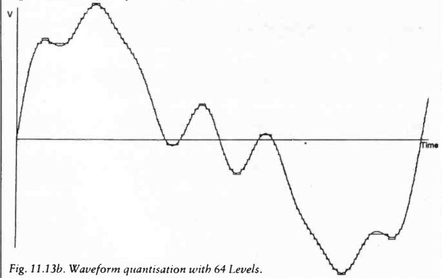
Fig. 11.13b. Waveform quantisation with 64 Levels.
