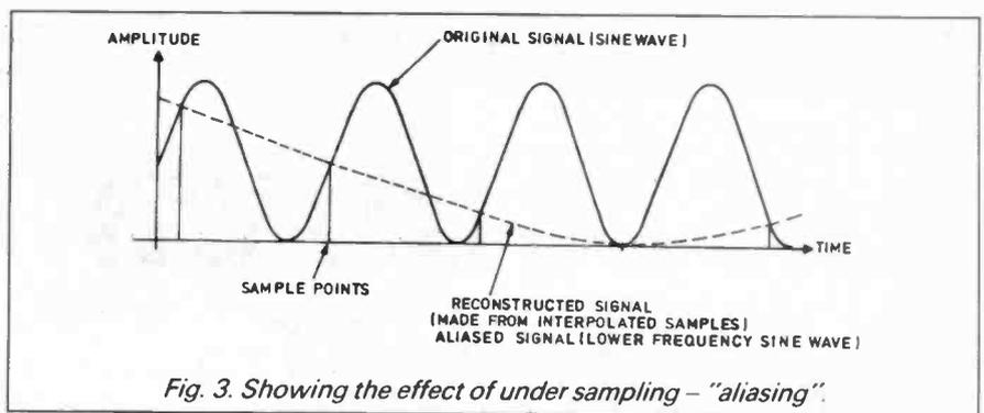
Fig. 3. Showing the effect of under sampling – "aliasing".
