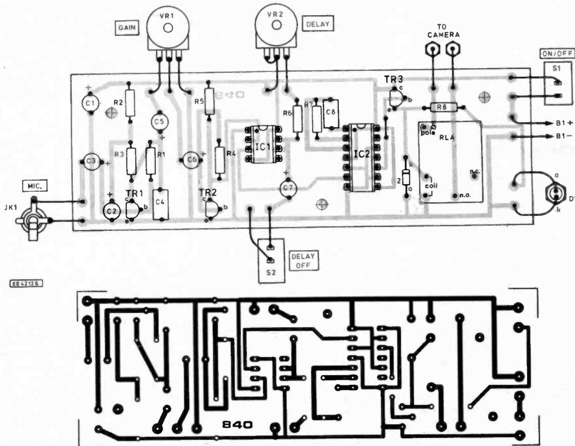
Fig. 3. Printed circuit board component layout and full size copper foil master pattern for the Sound Activated Camera Trigger unit.
