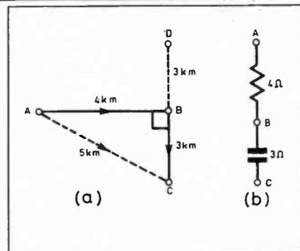
Fig. 2. A traveller's journey from A to C via B provides a good analogy for mixed impedances like Fig. 1d.
