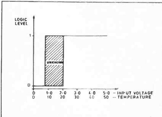
Fig. 11.1. CPU input level.
