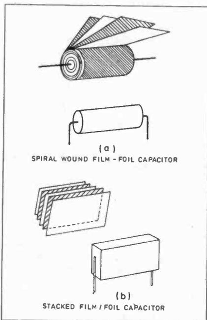
Fig. 1. Capacitor construction types.
