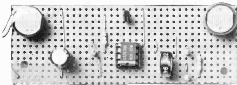
The completed circuit board showing the mountings of the radial capacitor and I.d.r.s.
