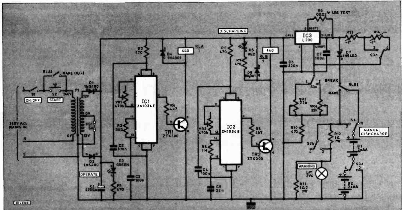
Fig. 1. Complete circuit diagram for the Charge-15 fifteen minute NiCad battery charger.
