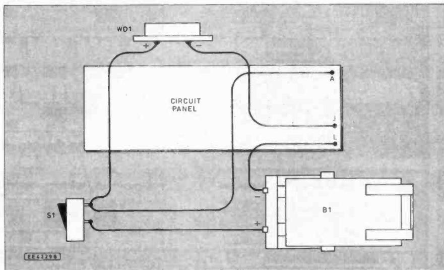
Fig. 3. Interwiring from the circuit board to battery holder, switch and warning buzzer.
