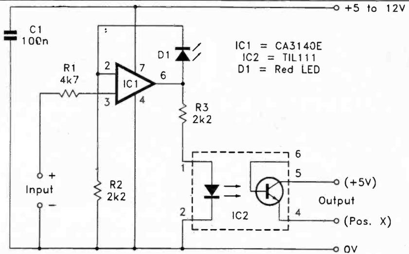
Fig. 2. A simple voltage to resistance converter. This is only suitable for non-critical applications.
