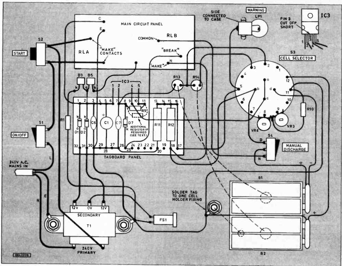
Fig. 3. Interwiring between the two boards and all off-board components. Connections to relay RLA "make" contacts are made by soldering 3A (minimum) mains wire direct to the relay tags.
