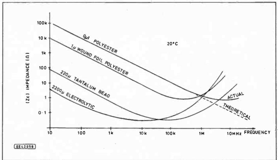
Fig. 5. Actual impedance vs. frequency of real-life capacitors.
