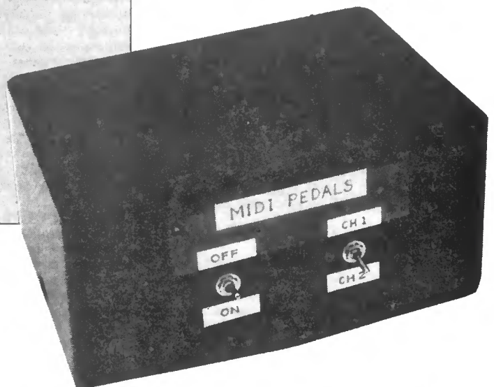
The completed keyboard scanner unit showing the MIDI Channel select switch and On/Off switch. These switches could be mounted on one of the side panels, away from any "flying feet."
