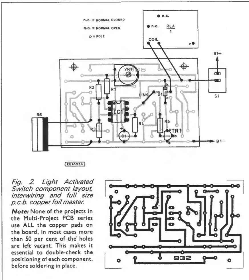
Fig. 2. Light Activated Switch component layout, interwiring and full size p.c.b. copper foil master.
