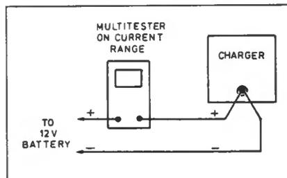
Fig. 6. Checking the current flow into a battery.
