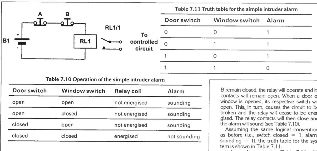
Fig. 7.4 Intruder alarm based on normally-closed switches and its truth tables.
