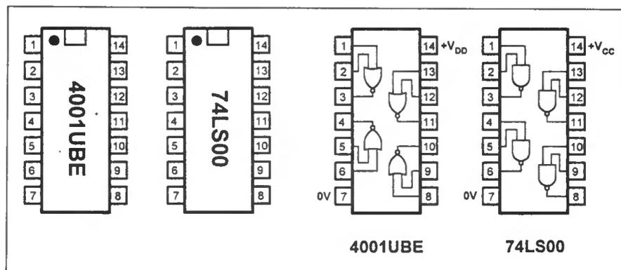
Fig. 7.18 Example of markings on digital integrated circuits.
