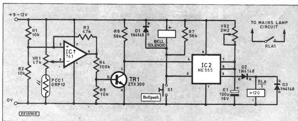
Fig. 1. Circuit diagram for a Doorbell-activated Porch Light.
