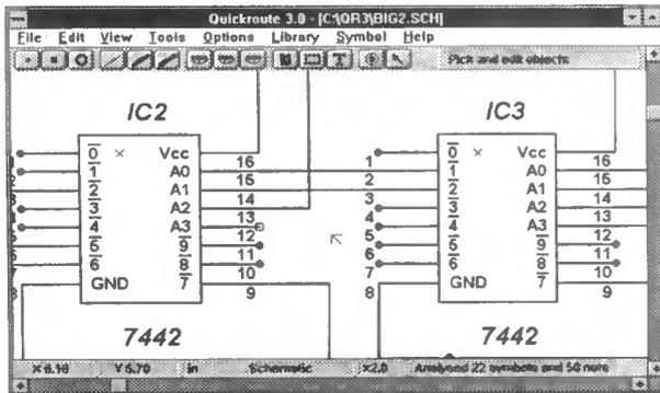
After schematic capture, components can be re-arranged prior to manual or automatic routing.
