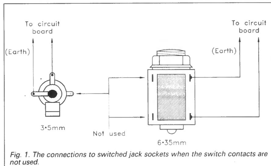
Fig. 1. The connections to switched jack sockets when the switch contacts are not used.
