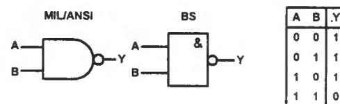
Fig. 7.8 Symbols and truth table for a two-input NAND gate.
