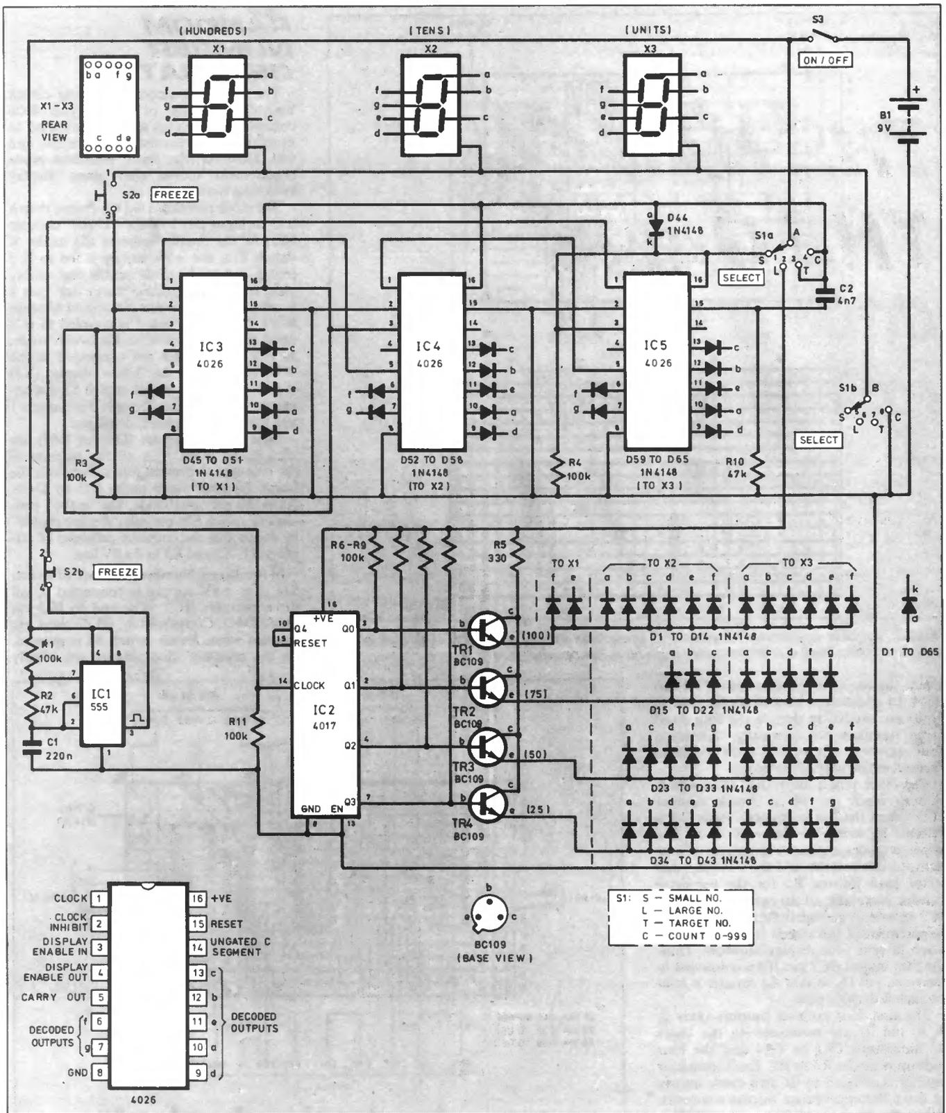
Fig. 1. Circuit diagram for the Counterspin games unit.
