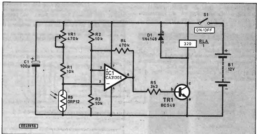
Fig. 1. Circuit diagram for the Light Activated Switch.
