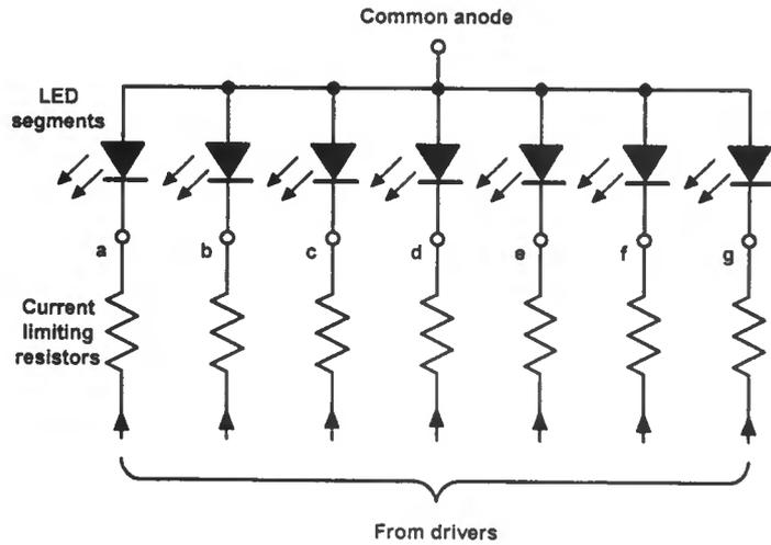
Fig. 7.29 Typical arrangement for a common-anode seven-segment display.
