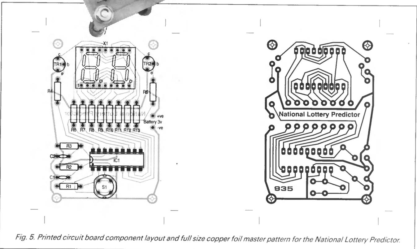
Fig. 5. Printed circuit board component layout and full size copper foil master pattern for the National Lottery Predictor.
