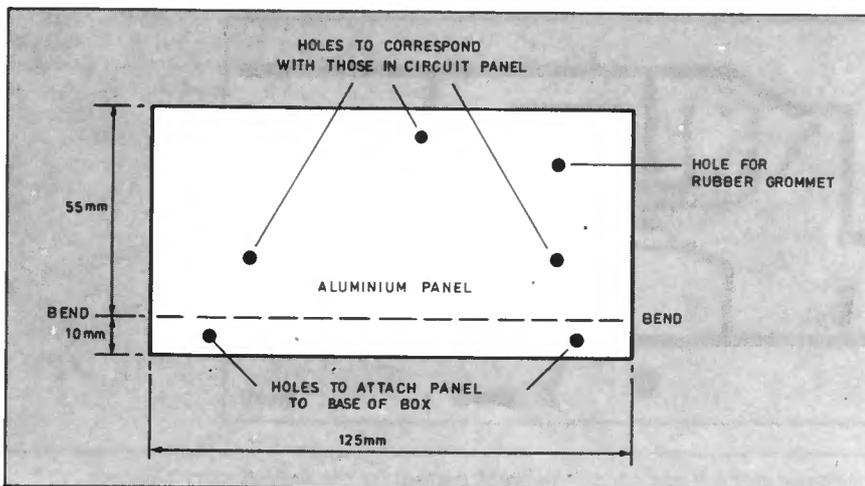
Fig. 3. Shaping the aluminium panel to which the p.c.b. is mounted.
