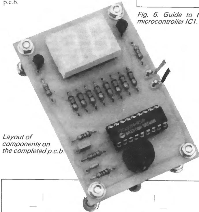
Layout of components on the completed p.c.b.
