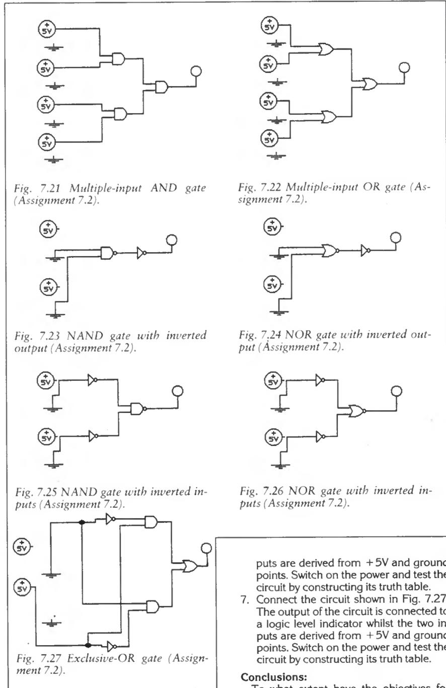
Fig. 7.21 Multiple-input AND gate (Assignment 7.2).
