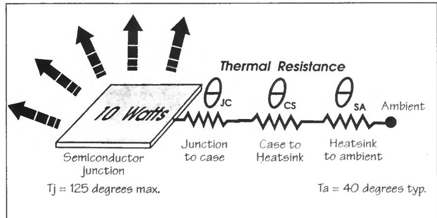
Fig. 2. Thermal resistance present in a heatsink system.
