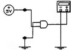
Fig. 7.16 Input connections for Assignment 7.1, A = 1 and B = 0.
