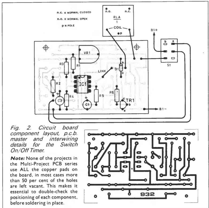
Fig. 2. Circuit board component layout, p.c.b. master and interwiring details for the Switch On/Off Timer.
