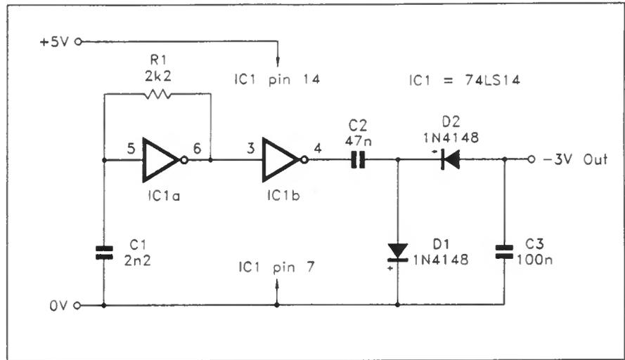
Fig. 3 The simple negative supply generator circuit diagram.
