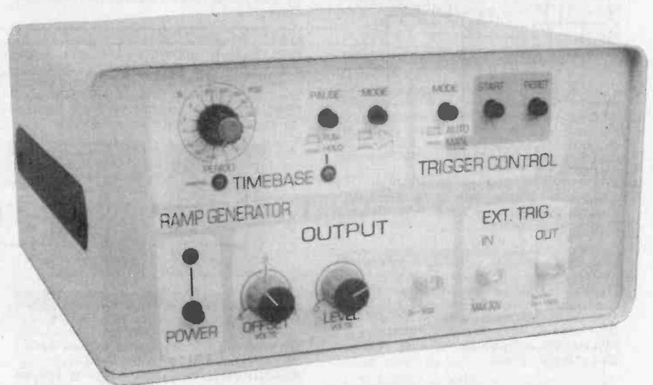
The 12-bit counter and digital-to-analogue converter (DAC) are responsible for converting the stream of digital pulses into a smooth ramping analogue waveform. The gated clock signal increments, or decrements, the counter, with the resulting 12-bit binary value being converted to an analogue voltage by the
