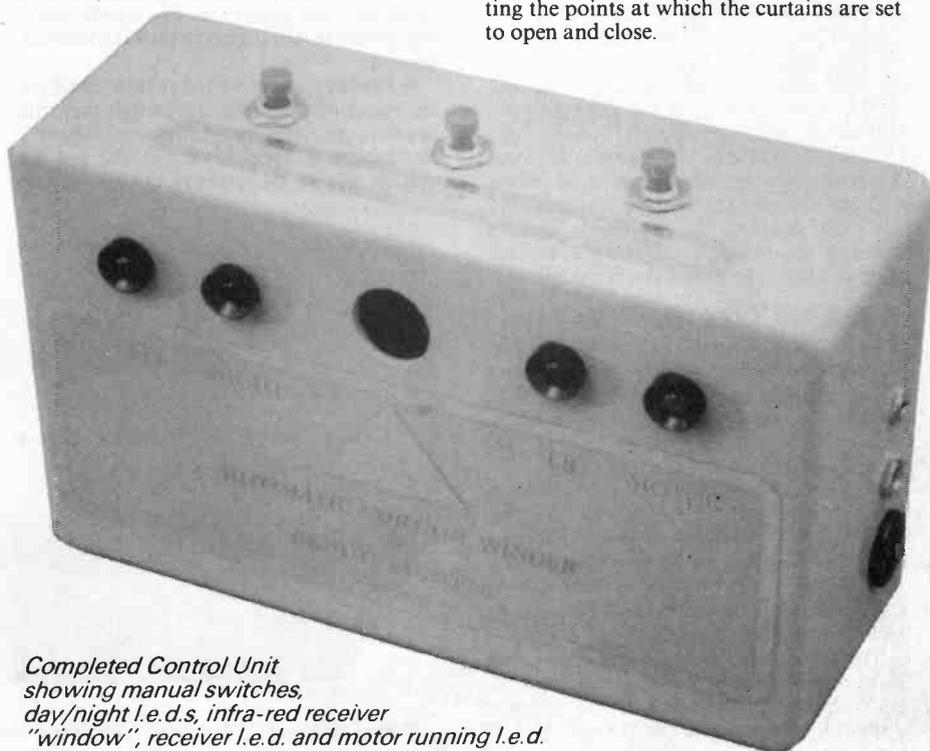
Completed Control Unit showing manual switches, day/night i.e.d.s, infra-red receiver "window", receiver i.e.d. and motor running i.e.d.
