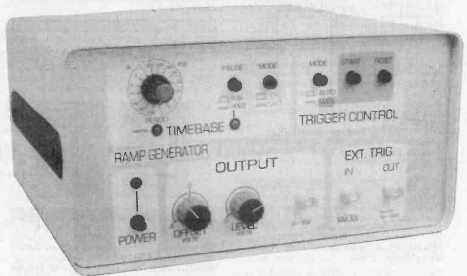
The 12-bit counter and digital-to-analogue converter (DAC) are responsible for converting the stream of digital pulses into a smooth ramping analogue waveform. The gated clock signal increments, or decrements, the counter, with the resulting 12-bit binary value being converted to an analogue voltage by the
