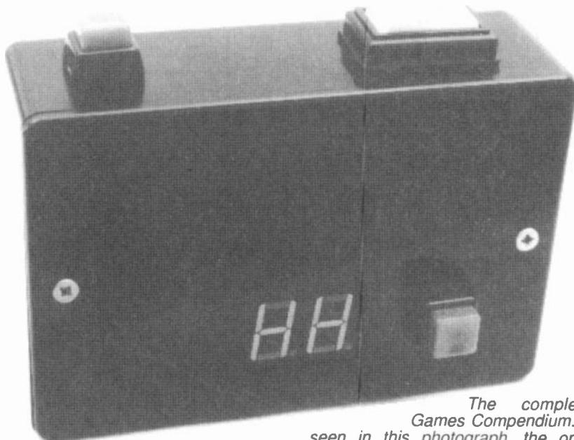
The completed Games Compendium. As seen in this photograph, the on-off switch is top right, the Choice switch is top left, and the Play switch alongside the l.e.d. display.
