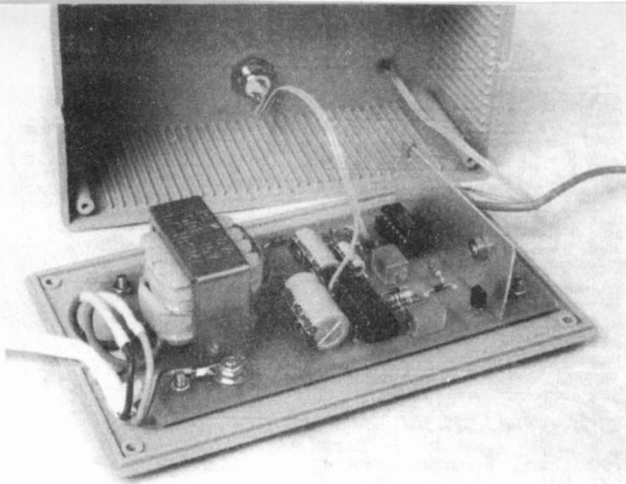
Switch the supply off. Remove the wire link from IC2 socket and place it across the connections for pins 3 and 16 of IC1's socket. This will apply a high signal to pin 4 of IC2, which can now be inserted in its socket. If the circuit is powered again, the l.e.d. should flash briefly at two-second intervals, showing that this part of the circuit is operating.
