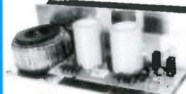
**OMP/MF 300 Mos-Fet** Output power 300 watts R.M.S. into 4 ohms, frequency response 1Hz - 100KHz -3dB, Damping Factor > 300, Slew Rate 60V/uS, T.H.D. typical 0.001%, Input Sensitivity 500mV, S.N.R. -110 dB. Size 330 x 175 x 100mm.
