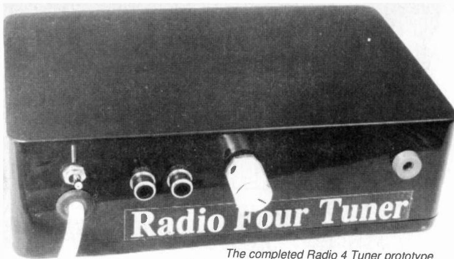
The completed Radio 4 Tuner prototype. The panel fuseholder is not shown on this model.
