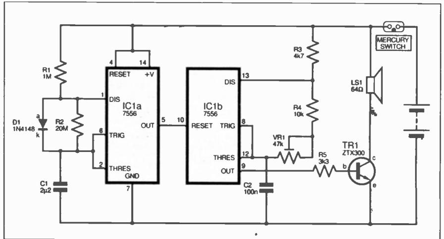
Fig. 2. Complete circuit diagram for the Mole-Ester.
