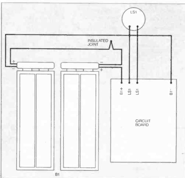
Fig. 4. Interwiring to the battery holders, speaker and circuit board.
