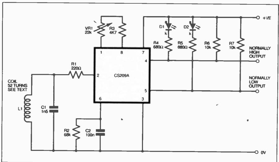
Fig. 10.4. Example circuit diagram for using the CS209A.
