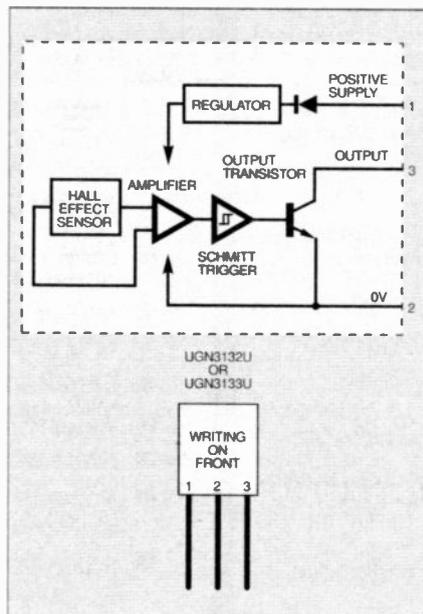
Fig. 10.1. Block diagram and pinout details for Hall effect sensors type UGN3132U and UGN3133U.
