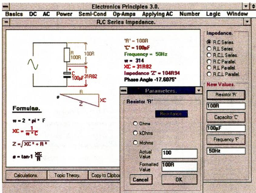
Fig. 5. Component values can be manually input via a dialogue box.
