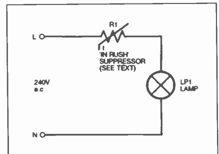
Fig. 1. Simple bulb protector.
