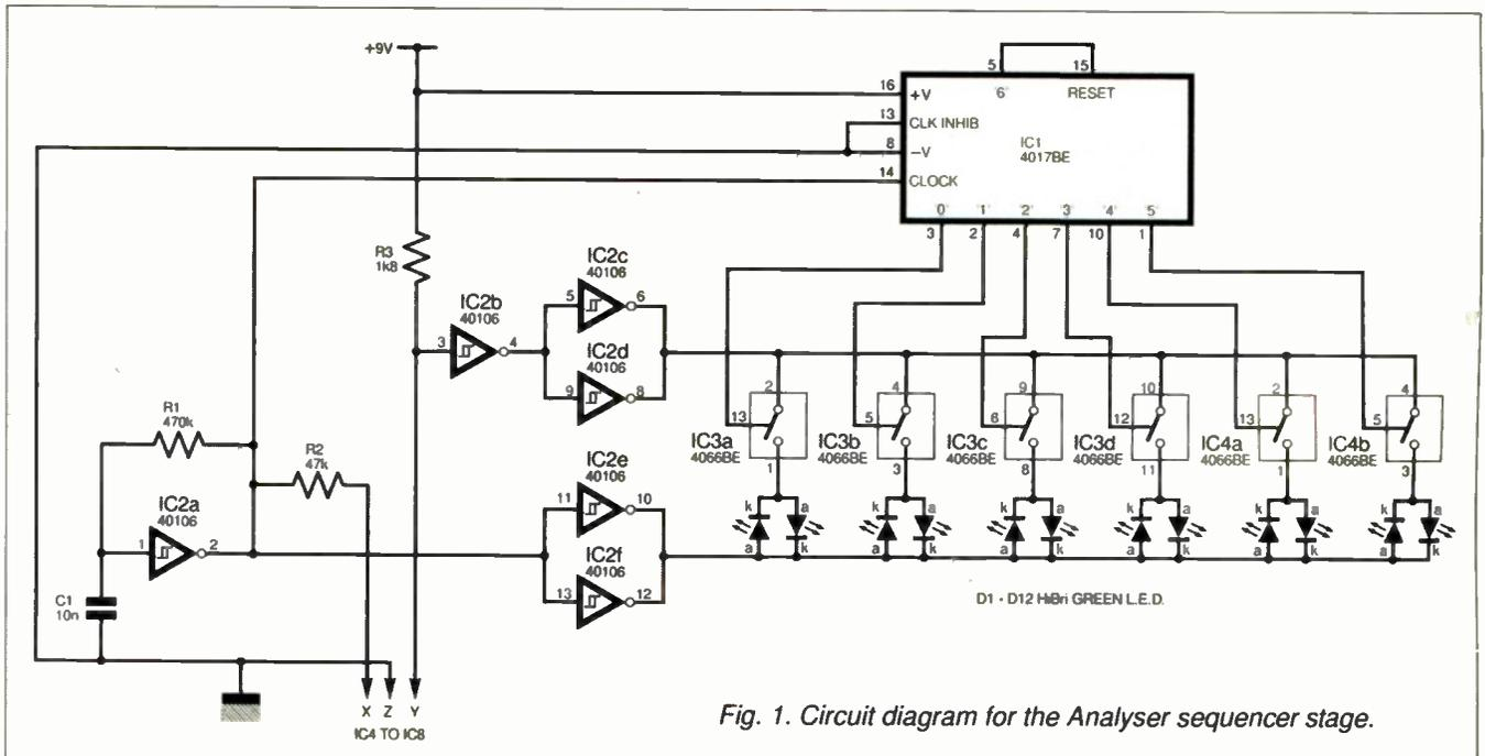
Fig. 1. Circuit diagram for the Analyser sequencer stage.
