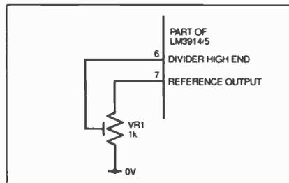
Fig. 10.11. Adjusting the bargraph response range.
