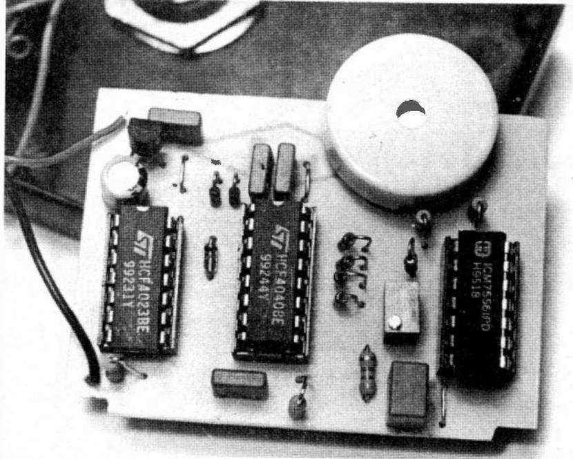
*Layout of components on the completed p.c.b. The supply voltage leads can be seen on the left. Note the two small cutouts on the p.c.b. to ease case mounting.*
