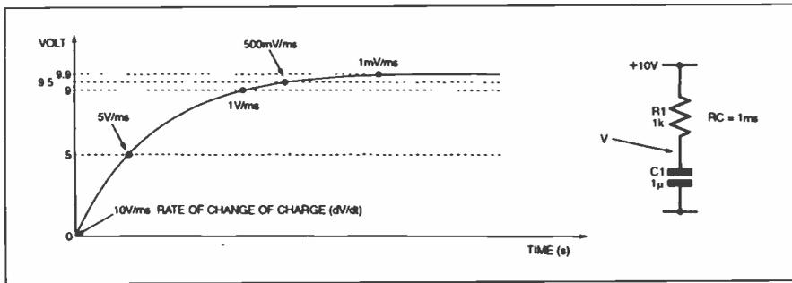
Fig. 2. Exponential charge curve of a basic R-C network.
