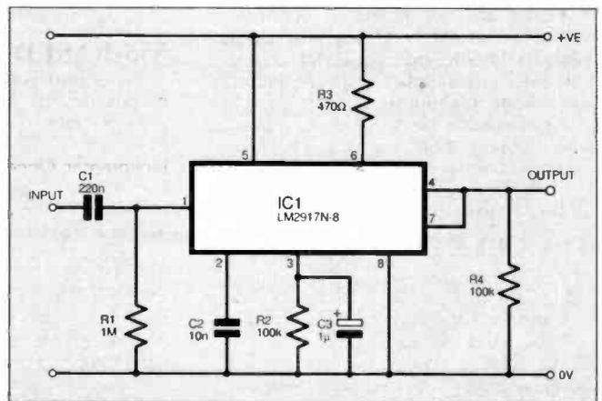
Fig. 10.9. Circuit for using the LM2917N-8 as a tachometer.
