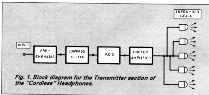
This applies a certain amount of high frequency boost to the signal. Complementary high frequency cut is used at the Receiver so that a flat frequency response is obtained overall.
