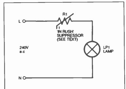
Fig. 1. Simple bulb protector.
