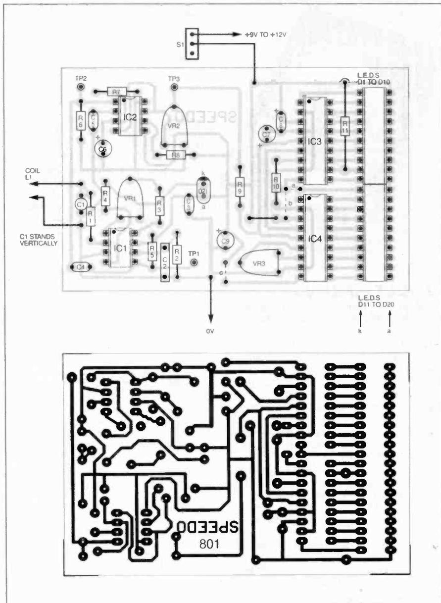
Fig. 3. Printed circuit board component layout and full-size underside copper foil master track pattern.
