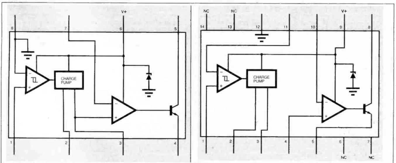
Fig. 10.8. Internal block diagrams of the LM2917N-8 (left) and LM2917N (right) tachometer i.c.s.
