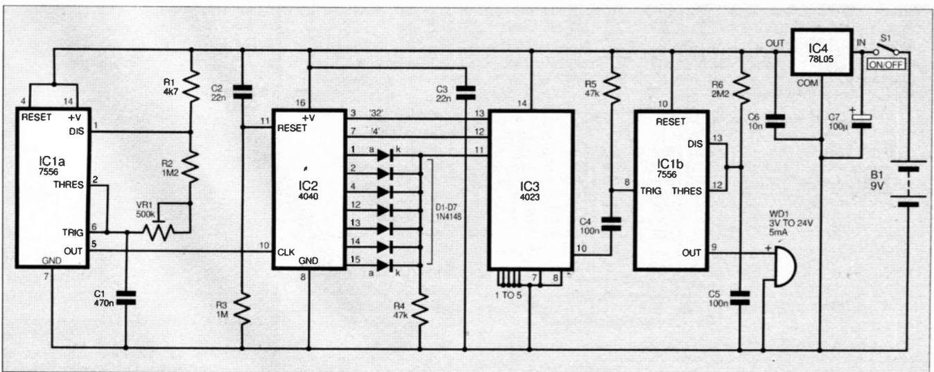
Fig. 2. Full circuit diagram, including voltage regulator, for the Mobile Miser.
