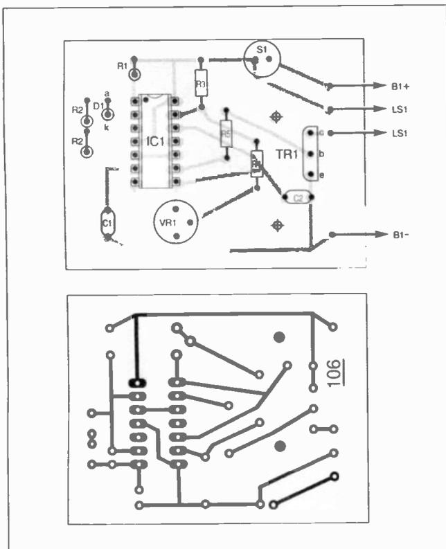
Fig. 3. Printed circuit board component layout and full size underside copper foil master pattern.
