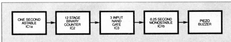
Fig. 1. Block diagram of the Mobile Miser system.
