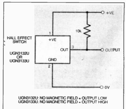
Fig. 10.2. Biasing the output.
