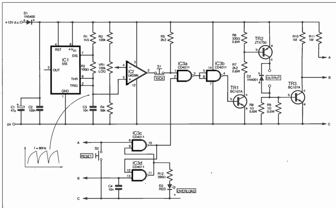
Fig. 1. Circuit diagram for the PWM Model Train Controller.
