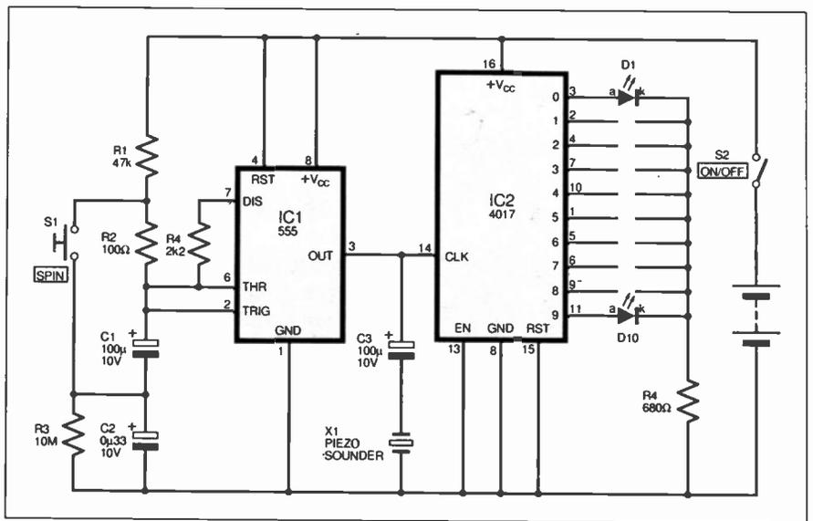
Fig. 3. The simple but flashy Mini Roulette circuit diagram.
