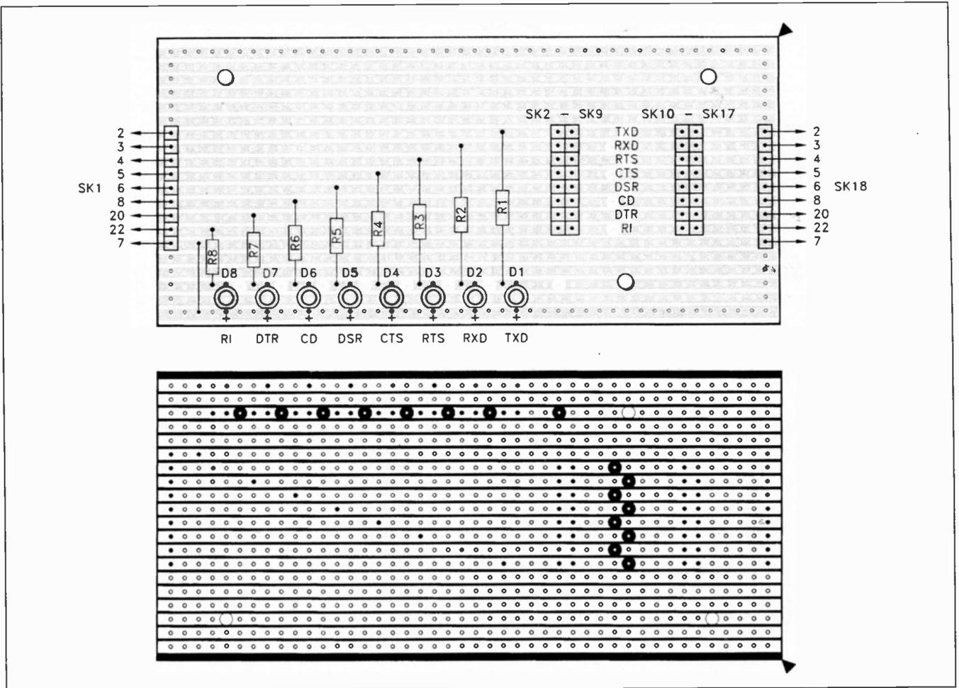
Fig. 2. Suggested stripboard construction of the circuit in Fig. 1.
