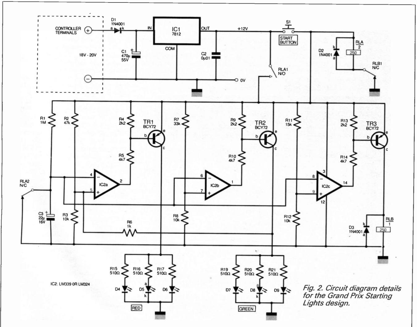
Fig. 2. Circuit diagram details for the Grand Prix Starting Lights design.
