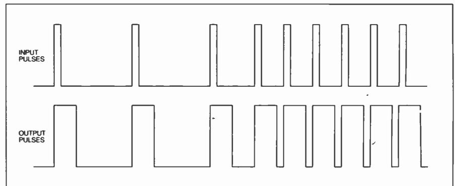
Fig. 10.6. Relationship of monostable input and output pulses.
