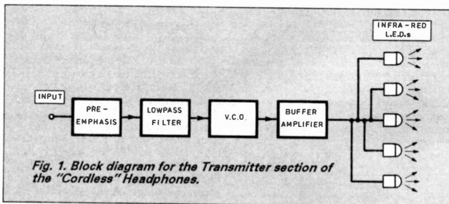
Fig. 1. Block diagram for the Transmitter section of the "Cordless" Headphones.
