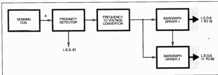
Fig. 1. Block diagram for the Bike Speedo.
