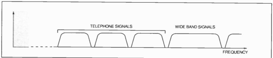
Fig. 1. Signals placed at different frequencies to send them down one link.
