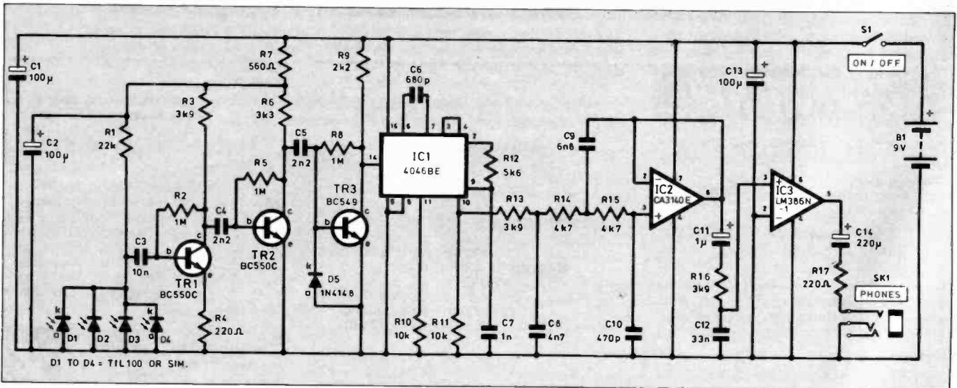
Fig. 5. Complete circuit diagram for the infra-red Receiver unit.
