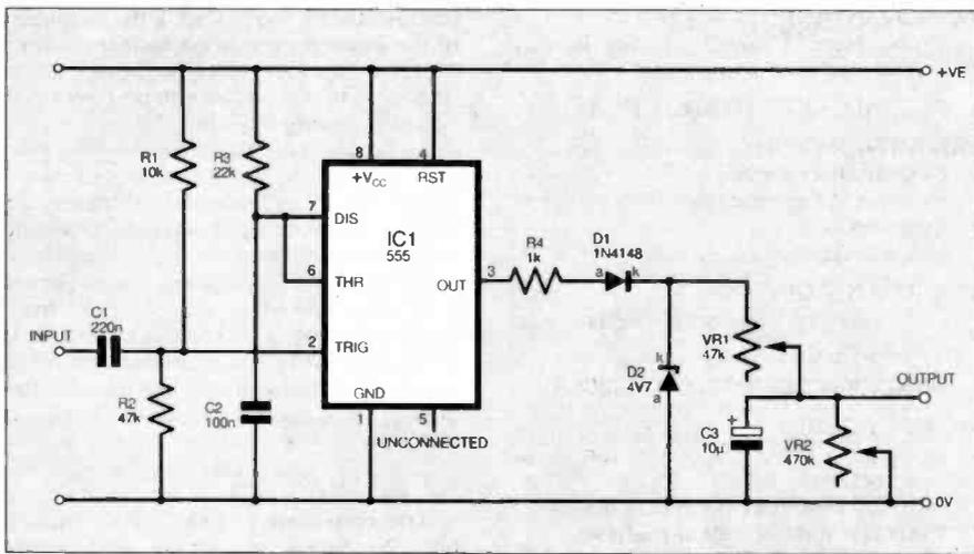
Fig. 10.7. Circuit diagram for a 555-based tachometer.
