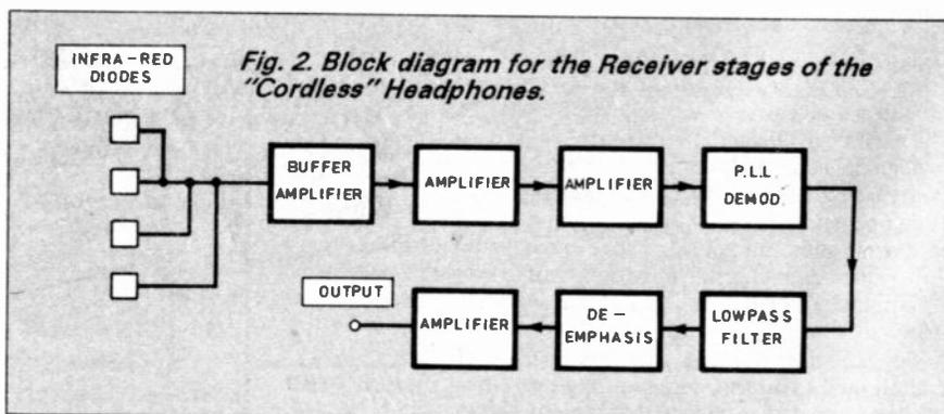
Fig. 2. Block diagram for the Receiver stages of the "Cordless" Headphones.
