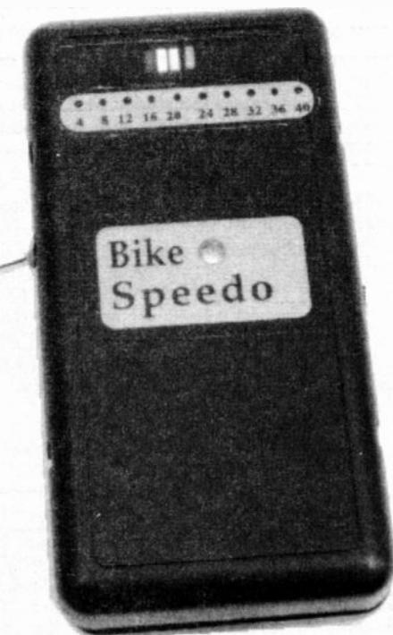
brand new bike, but the slightest imperfection in the geometry of the wheel could cause sensing problems. The chosen method of sensing the rotation was to use the proximity sensor i.c. type CS209A.
