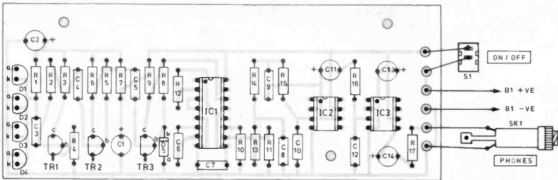
Fig. 8. (above) Circuit board component layout and wiring, and (right) actual size copper foil master for the Headphone Receiver.
