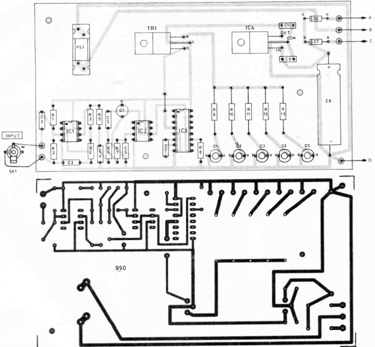
Fig. 6. Transmitter printed circuit board component layout, wiring and full size copper track master.
