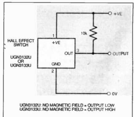
Fig. 10.2. Biasing the output.
