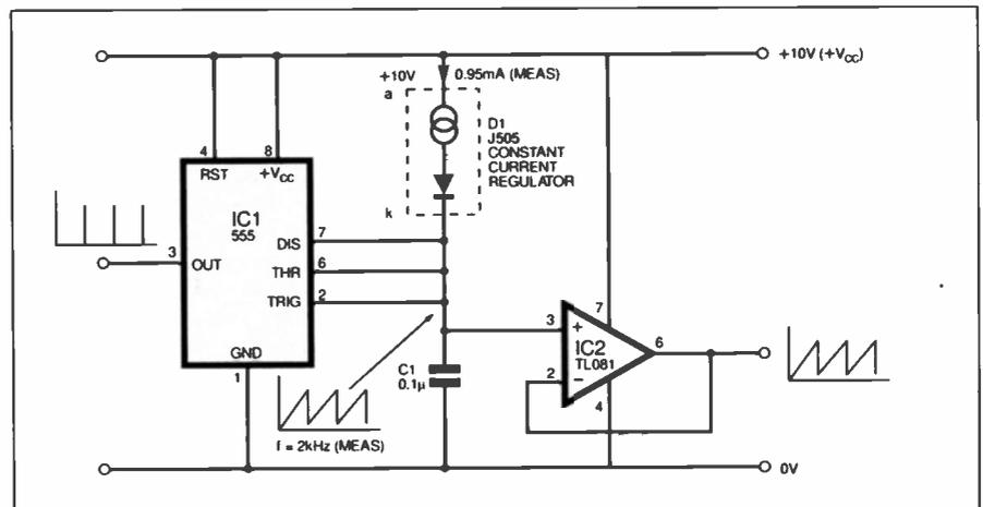
Fig. 4. Ramp generator using constant current regulator diode in a 555 oscillator.
