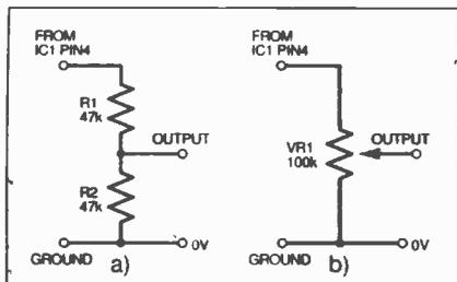
Fig. 10.10. Changing the output level from IC1 in Fig. 10.9.
