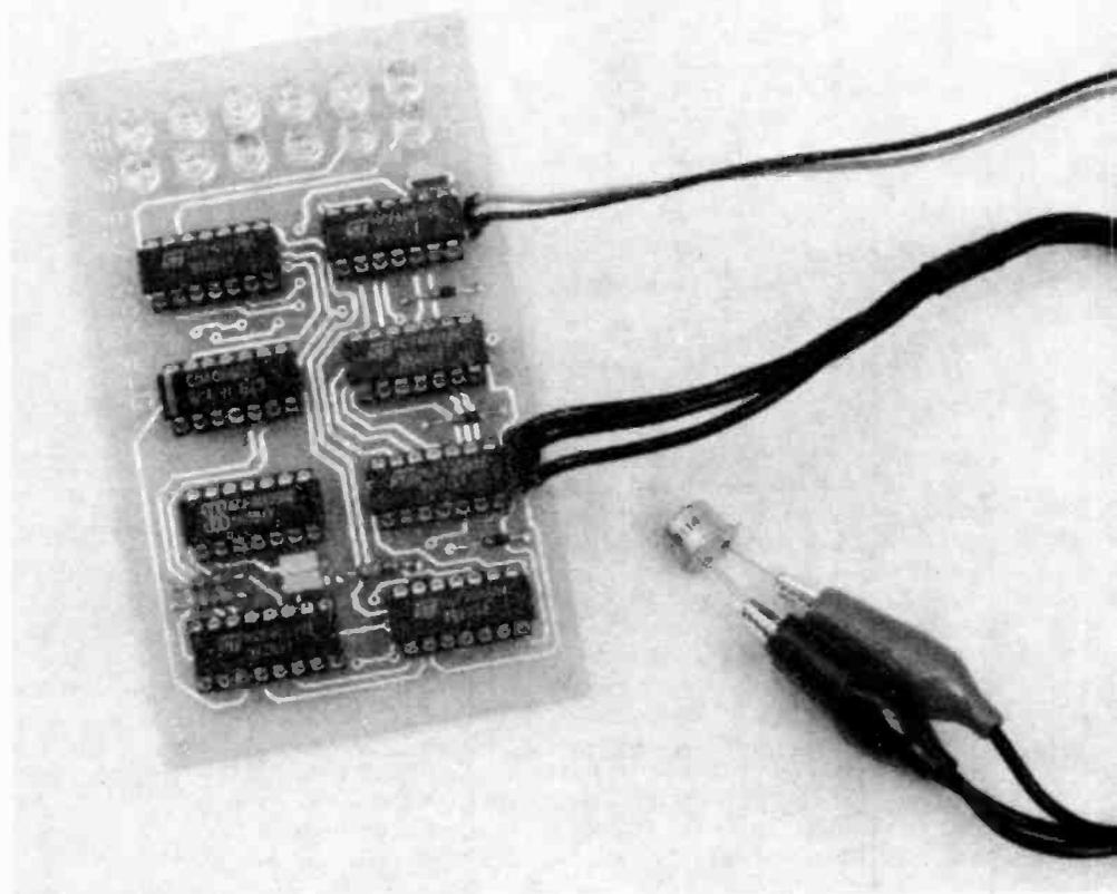
Completed Component Analyser p.c.b. with a transistor in the "jaws" of the croc-clips ready for testing.
