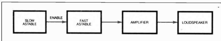
Fig. 1. Block diagram for the Mole-Ester.
