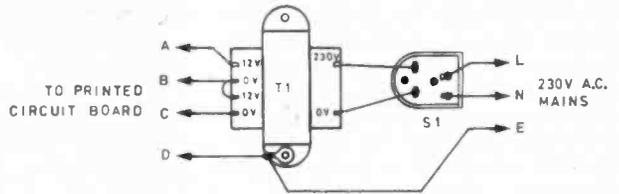
Fig. 7. Power supply wiring. Points A to D go to the p.c.b.
