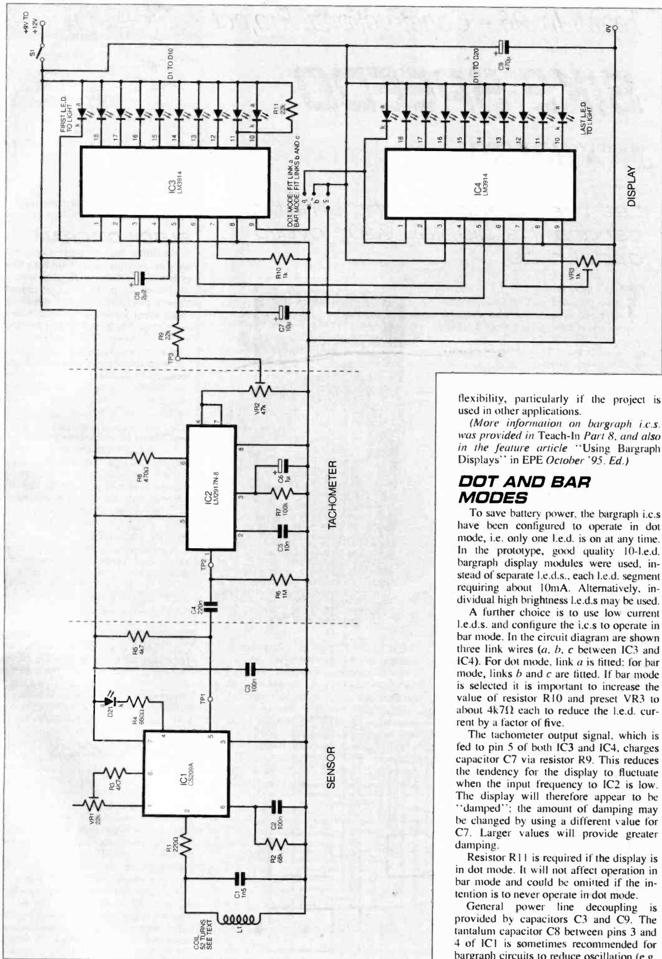
Fig. 2. Complete circuit diagram for the Bike Speed.
