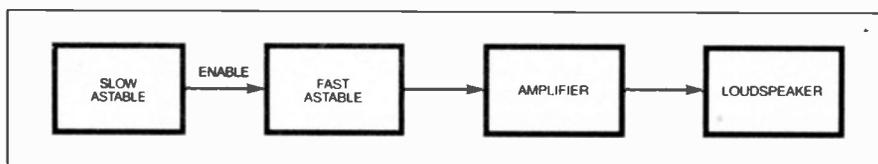
Fig. 1. Block diagram for the Mole-Ester.
