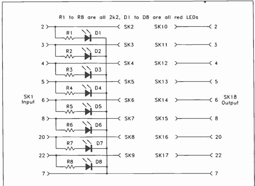
Fig. 1. The circuit diagram for a simple RS232C breakout box.
