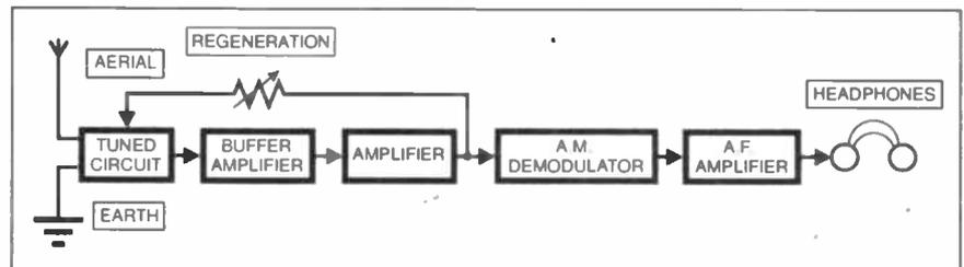
Fig.1. Block schematic diagram for the Simple SW Receiver.
