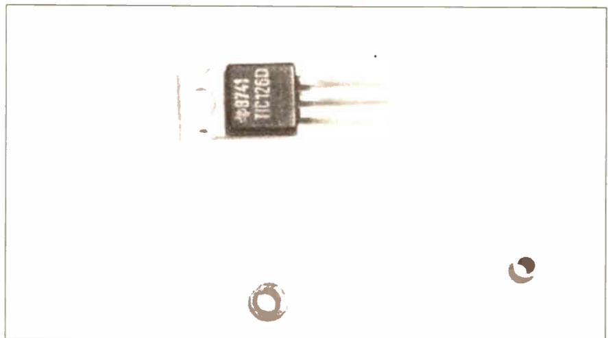
A TO220 transistor together with both mica (left) and plastic washers and a plastic bush.
