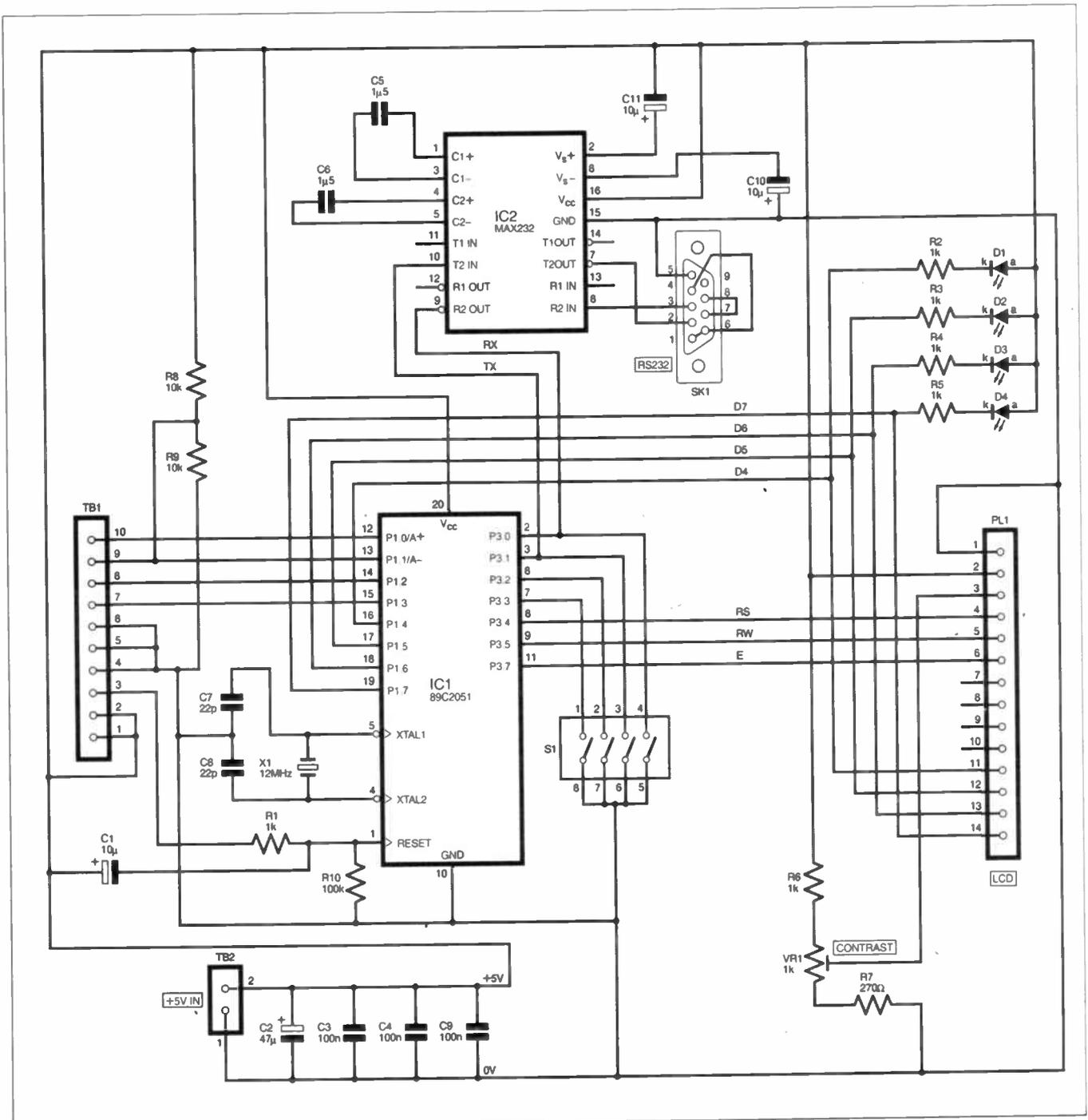
Fig.6. Circuit diagram for the Experimental Test Board.
