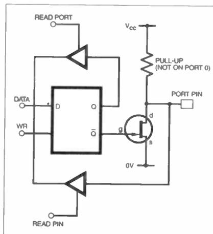
Fig.4. Typical port structure.
