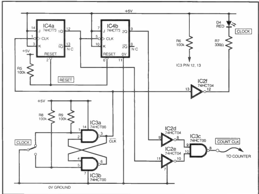
Fig.8.20. Assemble this Asynchronous 2-bit Counter, and link the Count CLK output to the clock counter of Fig.8.19.
