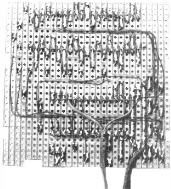
Underside of the stripboard showing interwiring. The wire used is Kynar covered type used for wirewrapping.
