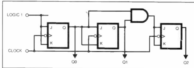
Fig. 8.13. A 3-bit synchronous up counter using JK flip-flops.
