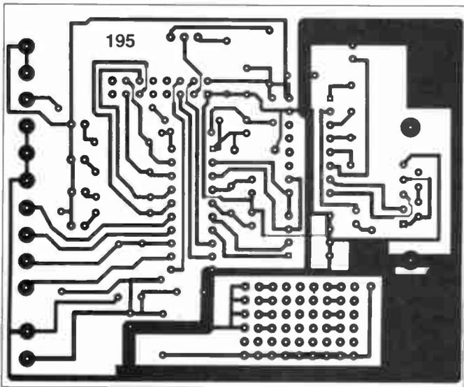
Fig.7. P.C.B. component layout and full size copper foil track master for the Experimental Test Board.
