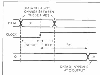
Fig. 8.17. Flip-flop setup, hold times and propagation delay.
