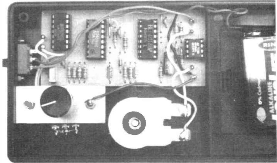
Completed unit showing components installed in the base of the case. Suggested methods for mounting the Frequency control and output coil are given in Fig.5 and Fig.6.
