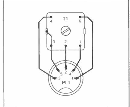
Fig.4. Pin connections from transformer T1 to the 5-way (180 degree) DIN plug.
