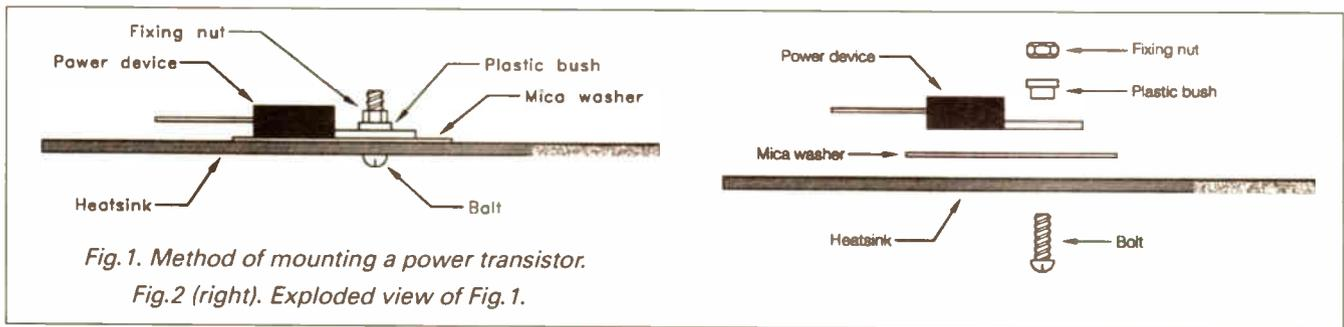
Fig. 1. Method of mounting a power transistor.
