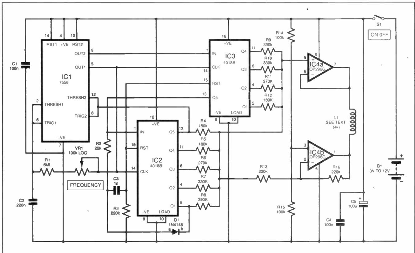
Fig.2. Complete circuit diagram for the EPE Mood Changer.
