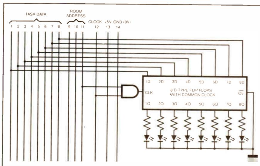
Fig.8.1. Command display circuit diagram.
