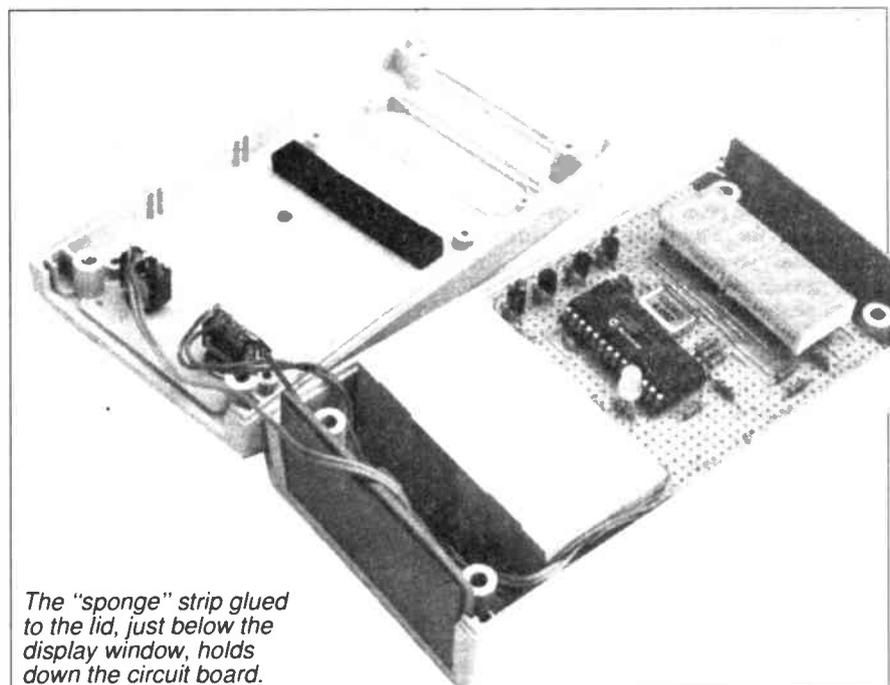
The "sponge" strip glued to the lid, just below the display window, holds down the circuit board.
