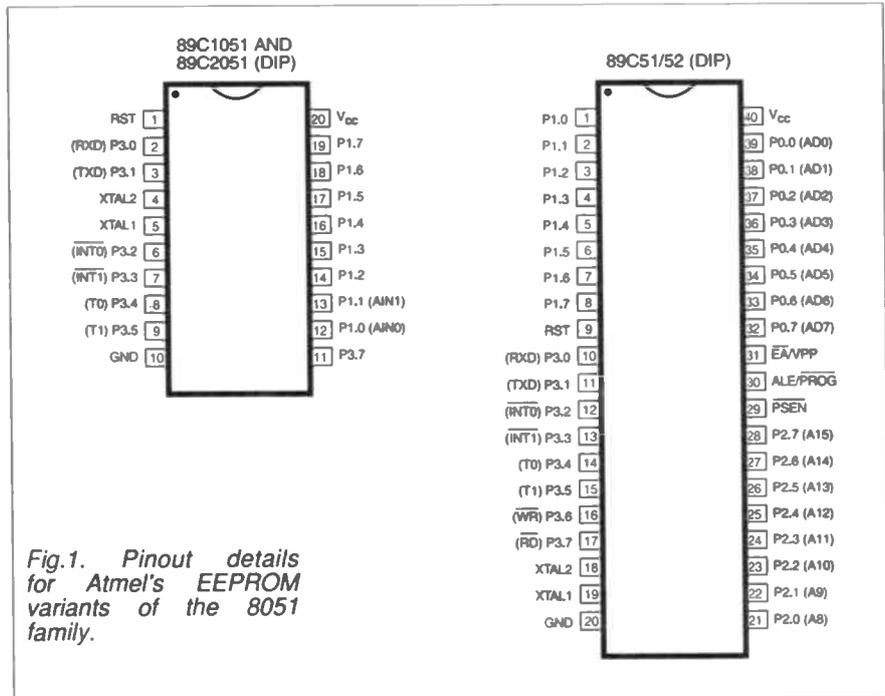
Fig.1. Pinout details for Atmel's EEPROM variants of the 8051 family.
