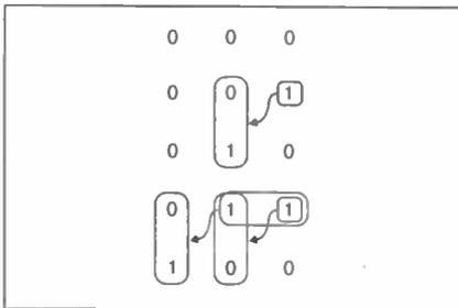
Fig. 8.12. When all lesser significant bits are 1 the next significant bit will toggle at the next clock input.
