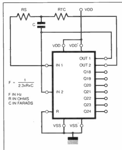
Fig.8.11 (above). Circuit for an RC oscillator circuit using a 4521 frequency divider i.c.
