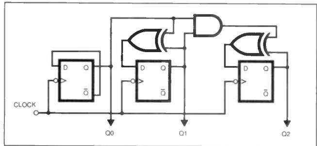
Fig. 8.16. Another 3-bit binary synchronous up counter. This one uses the toggle/hold circuit of Fig. 8.15
