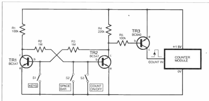
Fig.3. Typewriter word counter circuit.
