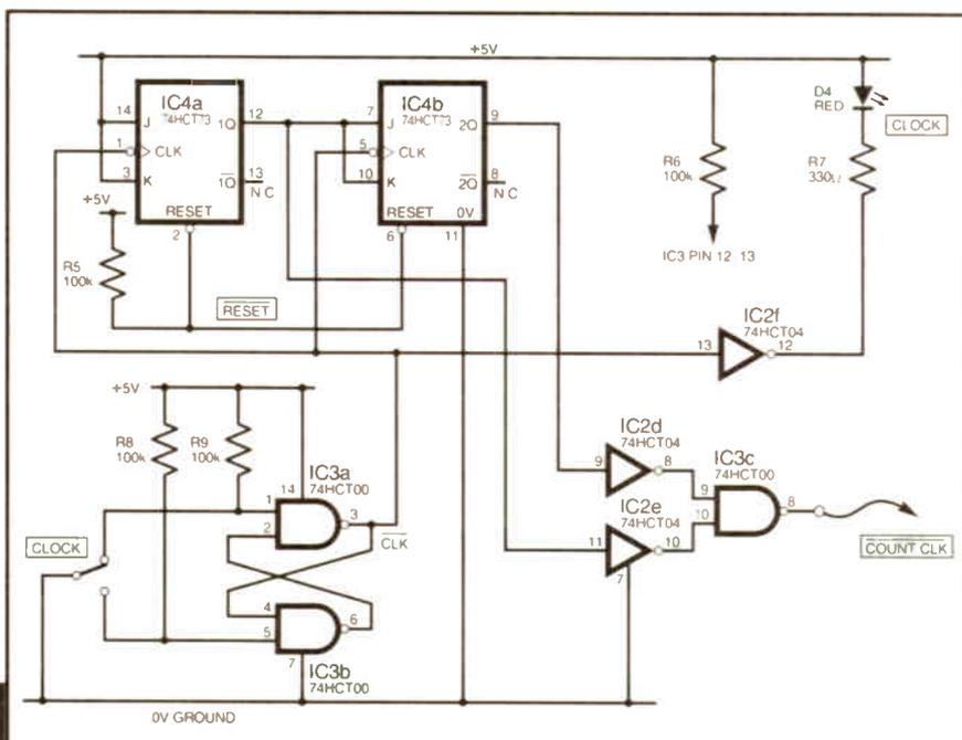
Fig.8.21. Modify the connections between IC4a and IC4b to form a Synchronous 2-bit Counter.
