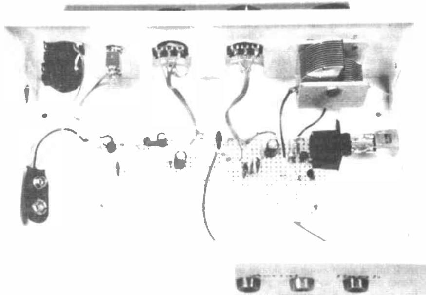
Completed Simple SW Receiver showing positioning of the circuit board and off-board components. Note the aerial and earth sockets are mounted on the rear panel.
