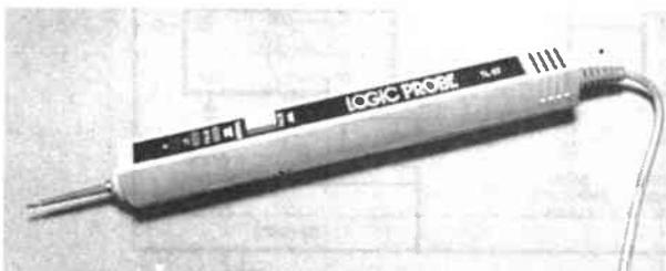
A useful piece of test equipment is the Logic Probe. The lead is terminated with a pair of crocodile clips.
