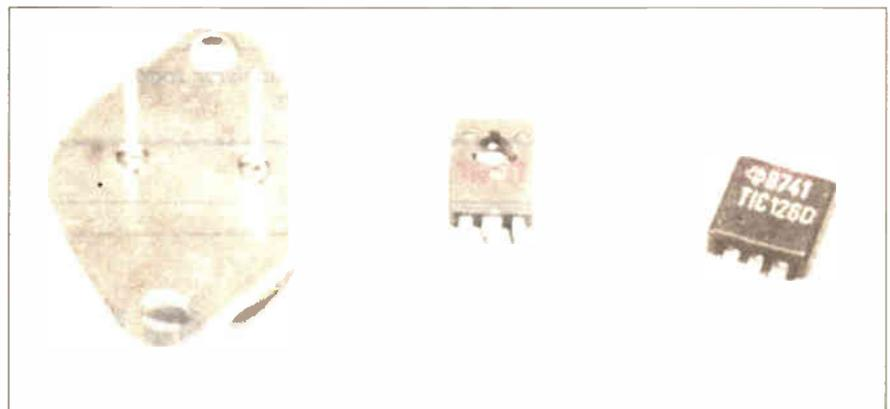
Various power transistors. From left to right the case styles are TO3, TO126 and TO220.
