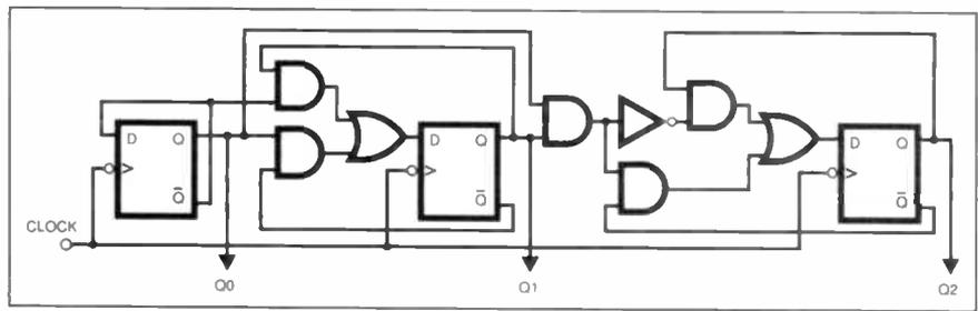
Fig. 8.14. A 3-bit binary synchronous up counter using D-type flip-flops.
