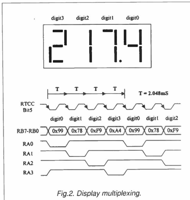
Fig.2. Display multiplexing.
