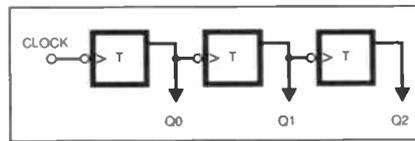
Fig.8.8. Asynchronous 3-bit binary counter using toggle flip-flops.
