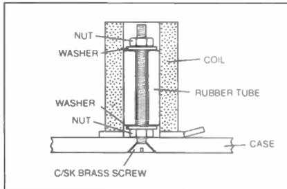
Fig.6. Coil mounting details.
