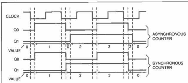
Fig.8.18. Timing diagram for asynchronous and synchronous counters.
