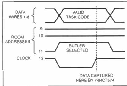
Fig.8.2. Command timing diagram.
