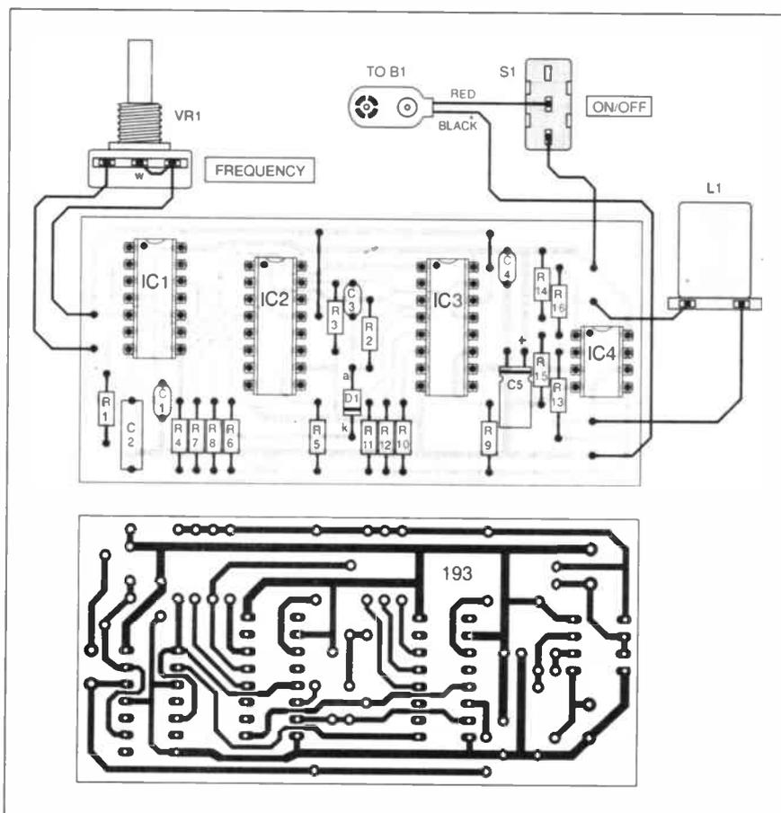
Fig.4. Printed circuit board component layout, off-board wiring and full size copper master pattern for the EPE Mood Changer.
