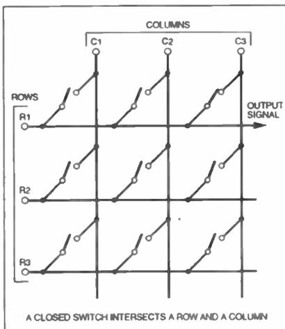
Fig. 1. 3 by 3 switch matrix.
