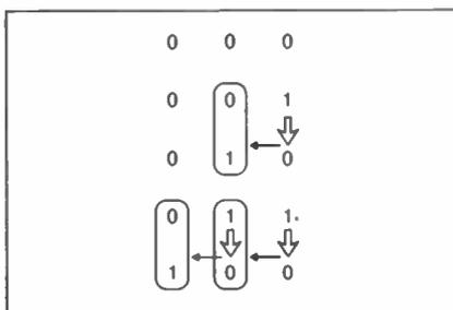
Fig.8.7. A 1→0 transition on one bit causes the next significant bit to toggle.
