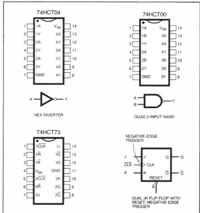
Pinout details for the MOS logic i.c.s used in the counter circuits.
