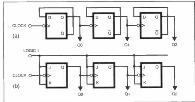
Fig.8.9. Asynchronous 3-bit binary up counters (a) using D-types, (b) using JKs.
