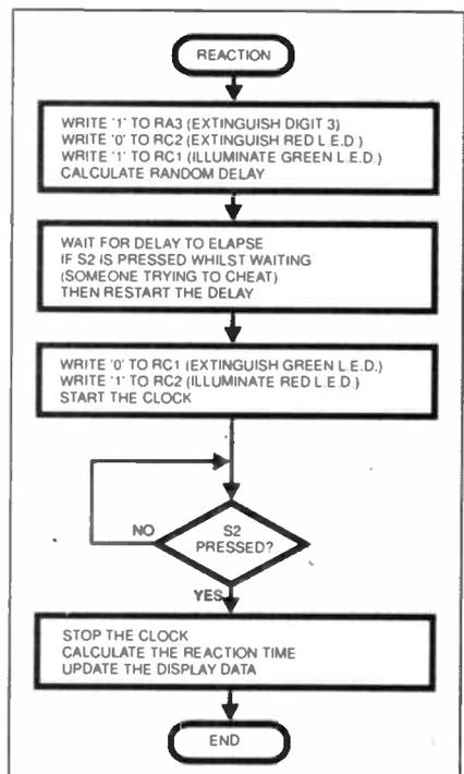
Fig.5. Software flow chart for reaction time.
