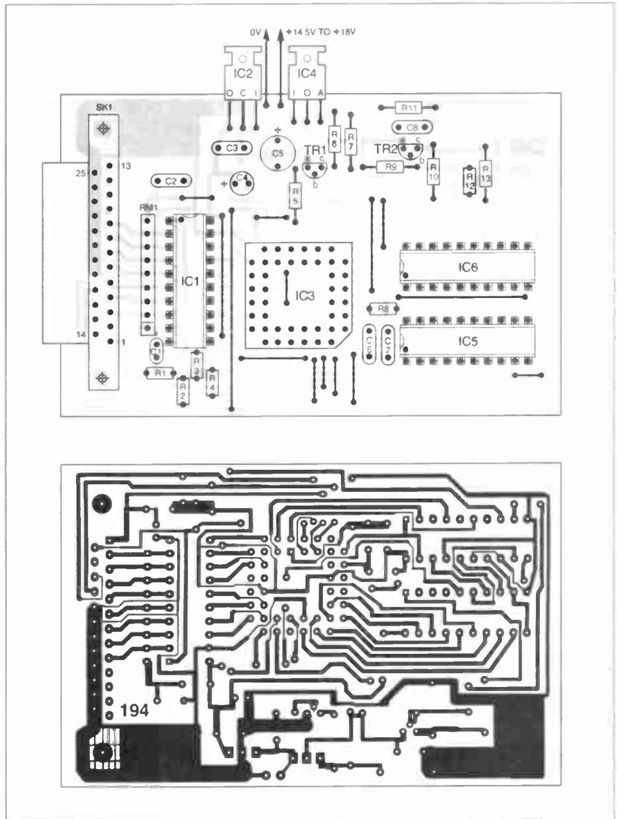
Fig.4. P.C.B. component layout and full size copper foil track master for the 2051/1051 programmer.
