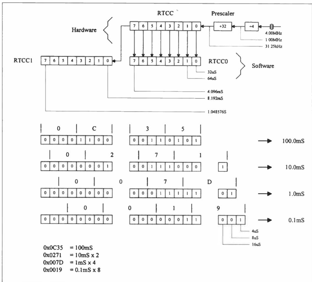
Fig.7. Calculating the reaction time.
