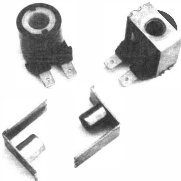
Producing an air-cored coil from a 230V solenoid coil salvaged from a washing machine three-way valve.
