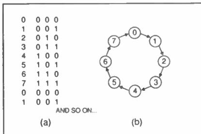
Fig.8.6. A 3-bit binary up counter (a) outputs, (b) state diagram.
