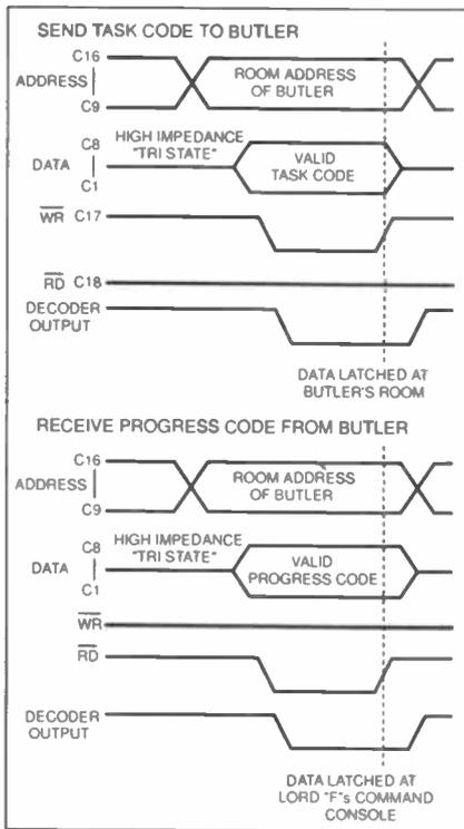
Fig.8.4 Read and Write timing diagrams for the Household Command System.
