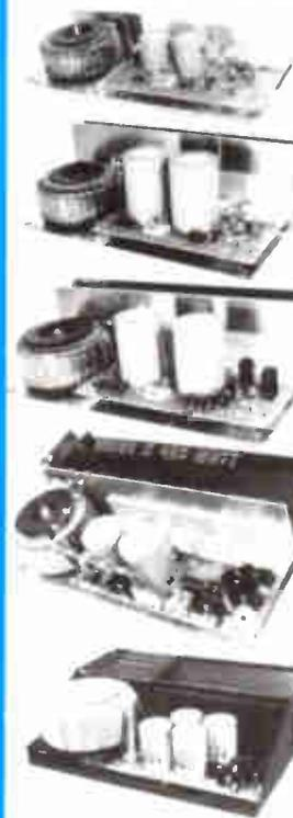
OMP/MF 100 Mos-Fet Output power 110 watts R.M.S. into 4 ohms, frequency response 1Hz - 100KHz -3dB, Damping Factor -300, Slew Rate 45V/uS, T.H.D. typical 0.002%, Input Sensitivity 500mV, S.N.R. -110 dB. Size 300 x 123 x 60mm.
