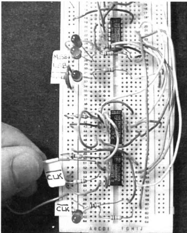
Building the synchronous/asynchronous counters, labelling the l.e.d.s and "toggling" the clock.
