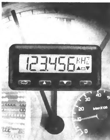
LASCAR Electronics have announced the introduction of their new family of intelligent digital panel meters, the C100 Counter, C110 Frequency Meter and C120 Timer.
