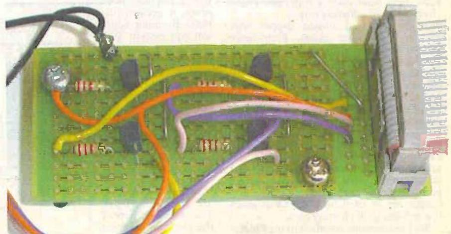
Fully assembled transistor board, complete with connector.
