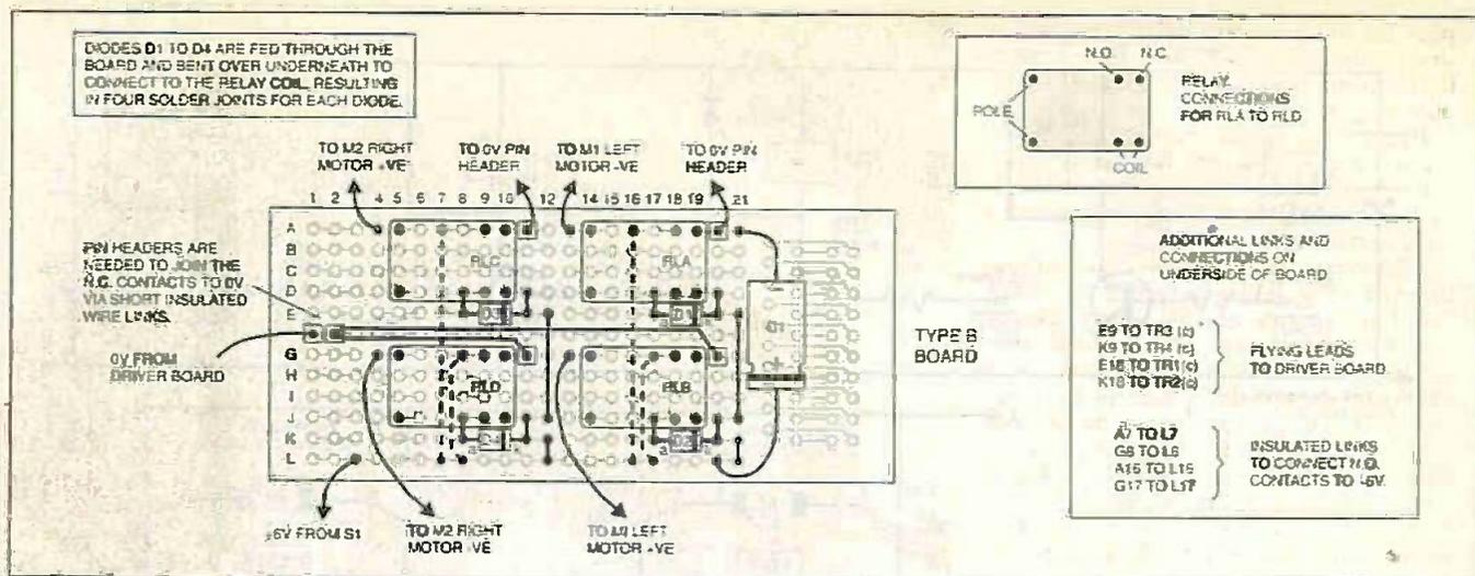
Fig.3. The four relays are also mounted on their own board and linked to the transistor board and motors as indicated.
