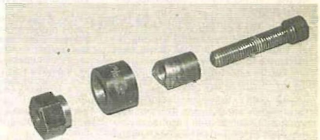
The four main parts of a chassis punch (above). The cutting blade (second right) is forced through the panel and into the die (second left). This produces very neat and accurate results.
