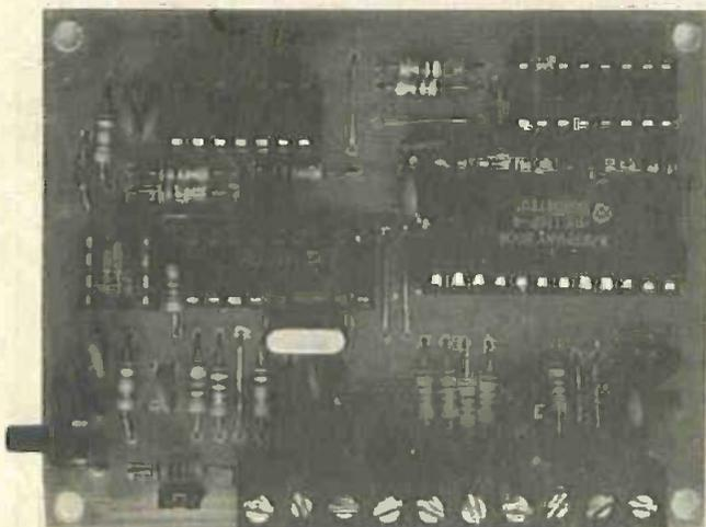
Layout of components on the finished p.c.b. The pushbutton function setting switch is on the bottom-left corner.
