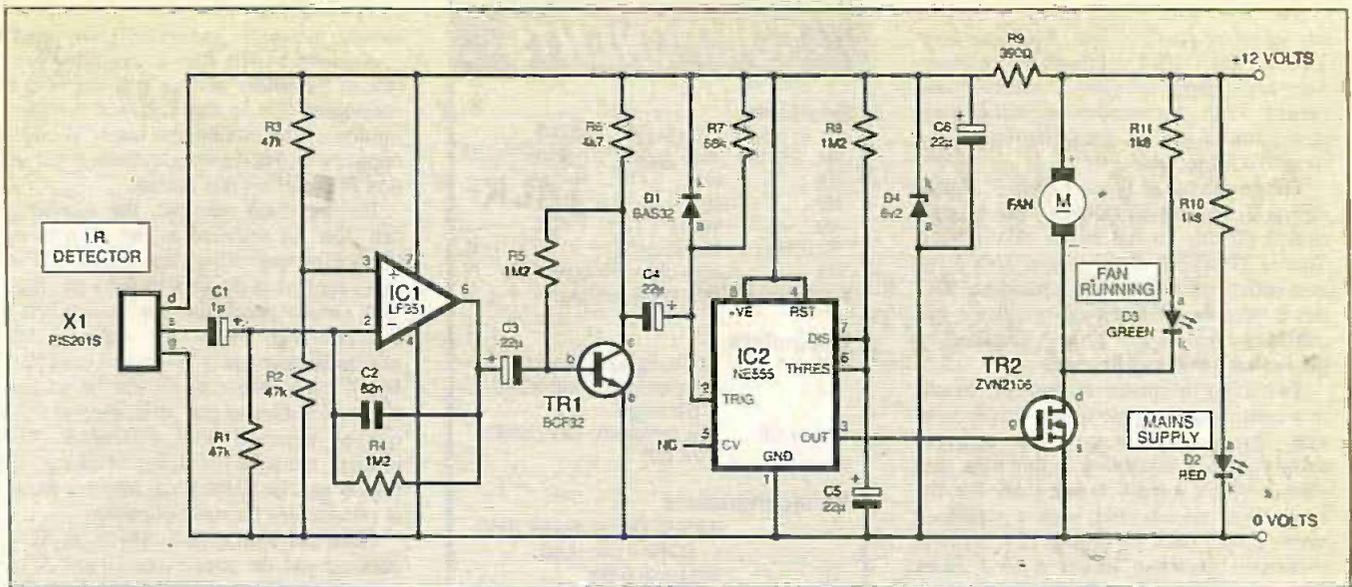
Fig. 1. Complete circuit diagram for the Smoke Absorber.
