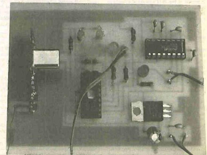
Completed a.m. receiver board. The f.m. adaptor p.c.b. replaces the a.m. module.
