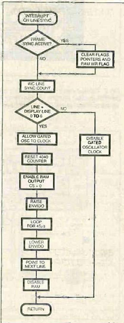
Fig.6. Simplified flowchart for the interrupt routine.
