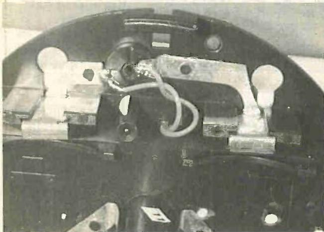
The original cord-operated switch has been removed from the lamp and the wires from the p.c.b. are soldered to its former position.
