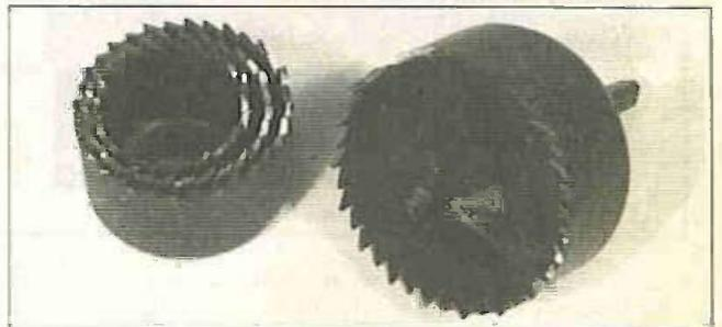
(Above) Hole-saws produce neat results and are quite fast. They work best in a power drill set to a slow speed. (Left) A reamer can turn a small hole into a larger one, up to about 30mm. The tank cutter (right) can handle holes having diameters from around 25mm to 120mm.
