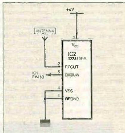
Fig. 19. Transmitter modification details for f.m. operation.
