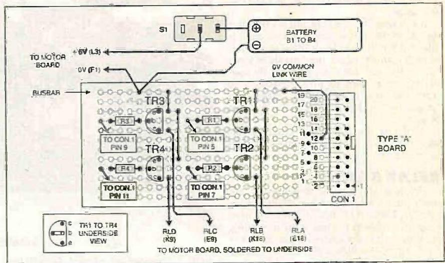
Fig. 2. The transistors are mounted on their own board.
