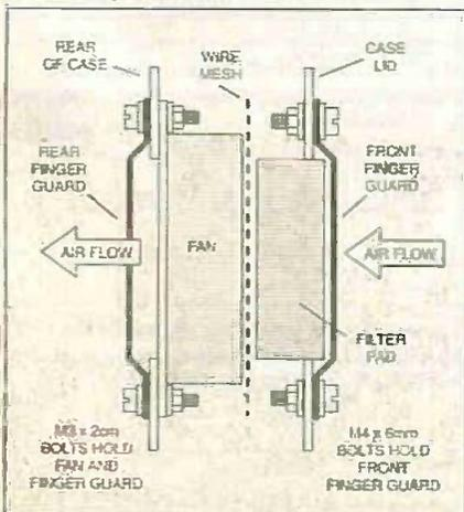
Fig. 5. Side-on view of the fan assembly.
