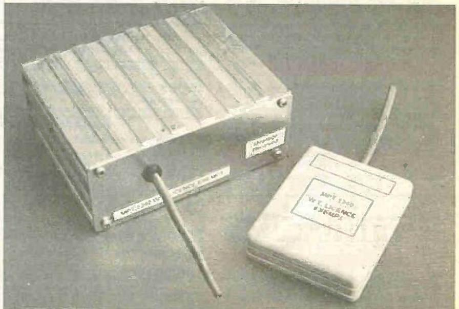
Completed Receiver module and Transmitter, with licence exempt label.
