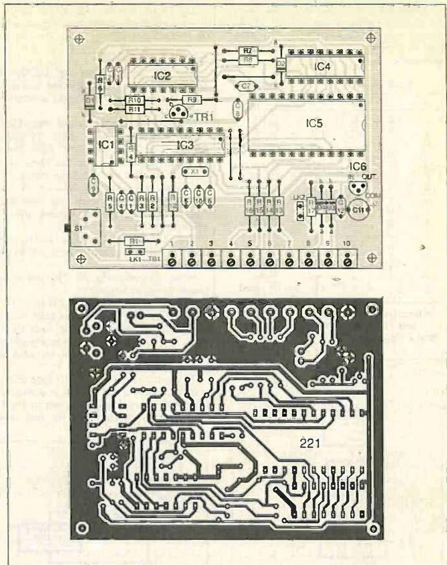
Fig.7. Printed circuit board topside component layout and full size underside copper foil master pattern for the Time and Date Generator. The right-angle 10-way screw terminal block (TB1) may have to be made up from "linkable" 2-way types.
