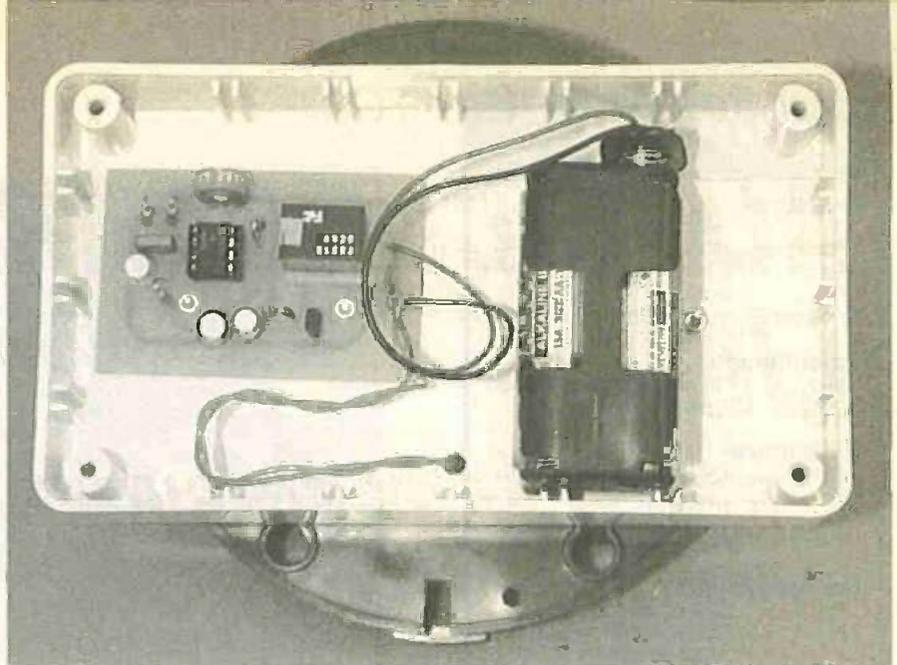
The circuit battery pack and printed circuit board mounted in position on the lid section of the box.
