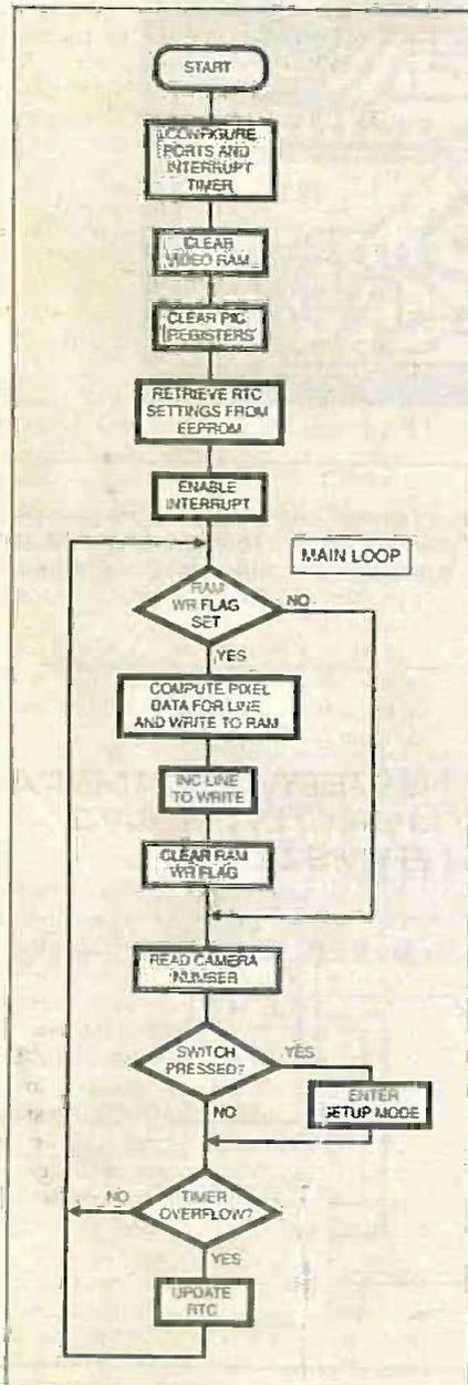
Fig.5. Setup and main loop initialisation flowchart.
