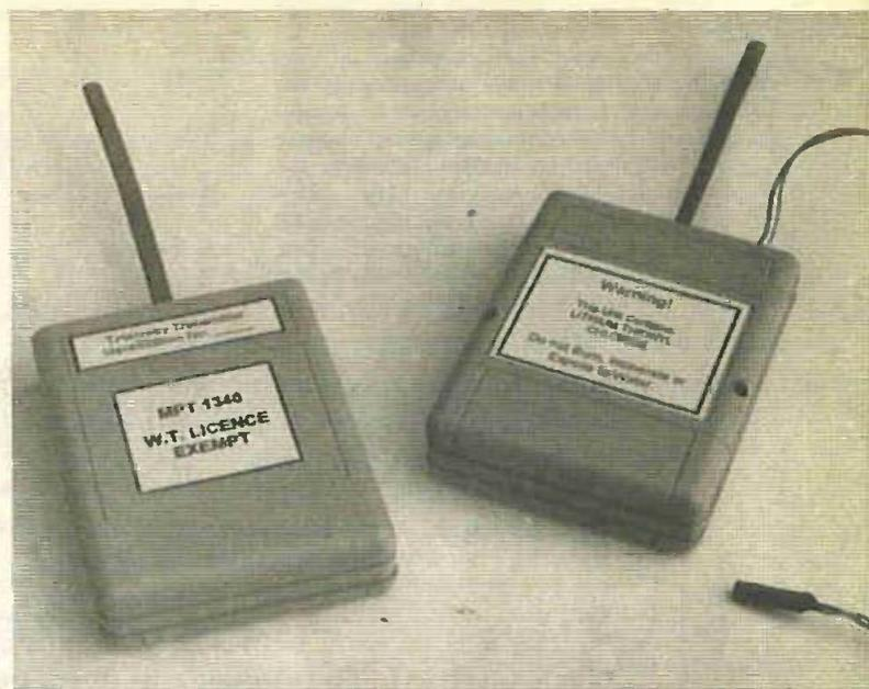
Two completed Transmitters. One with a remote thermistor sensor (right-hand corner), and the other showing the required "licence exempt" label.
