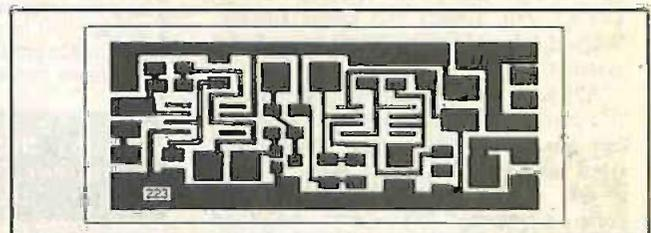
Fig. 3. Full-size topside (surface mount) copper foil master track pattern.
