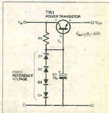
Fig. 2. A simple pre-regulator may help avoid excessive input-output voltage appearing across variable regulators. D1 and D2 are the Zener diodes.
