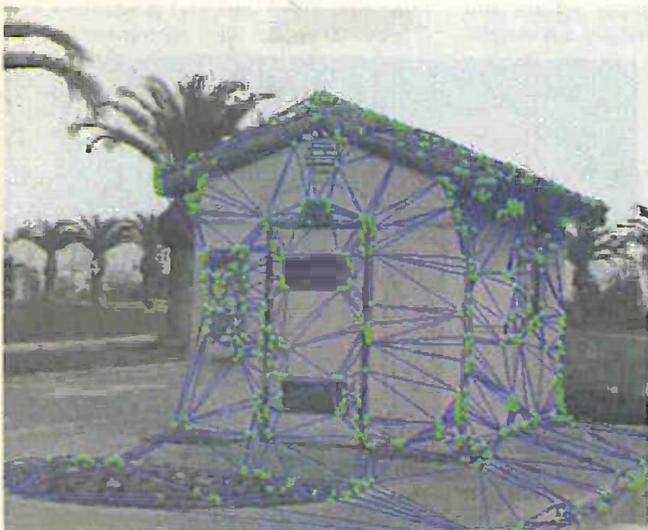
Fig.6. Polygonal mesh constructed from the data in the "point cloud".
