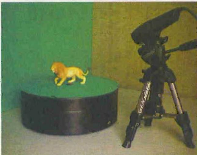
Fig.1. The 3Scan set-up with simple turntable and single video camera.
