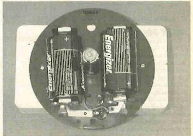
The D-cells and bulb replaced in the finished Auto Cupboard Light unit ready for receiving the light diffuser dome.
