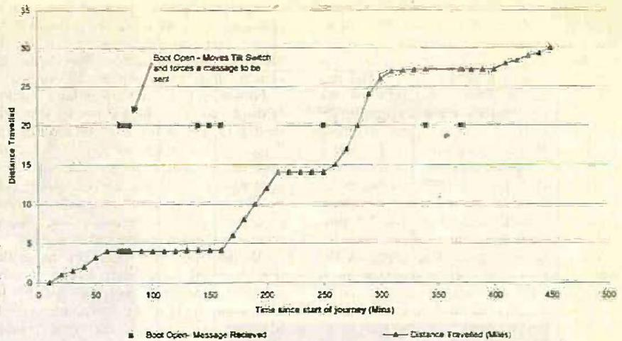
Fig. 16. Graph details from a boot sensor and a distance travelled sensor.
