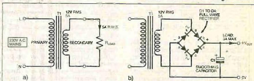
Fig. 1. Transformers must be derated when full-wave bridge rectifiers and smoothing capacitors are used. Makers' ratings usually assume a resistive load.
