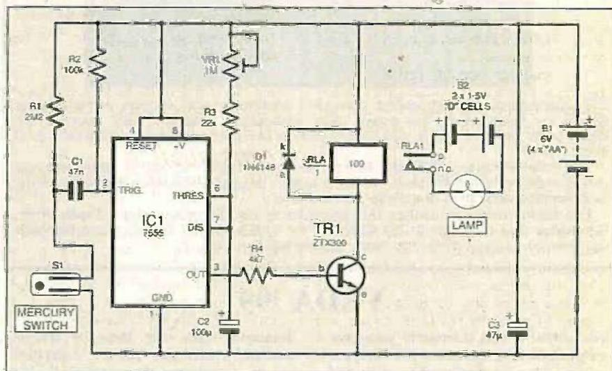
Fig.1. Complete circuit diagram for the Auto Cupboard Light. The power supply to the circuit is independent to that of the lamp.
