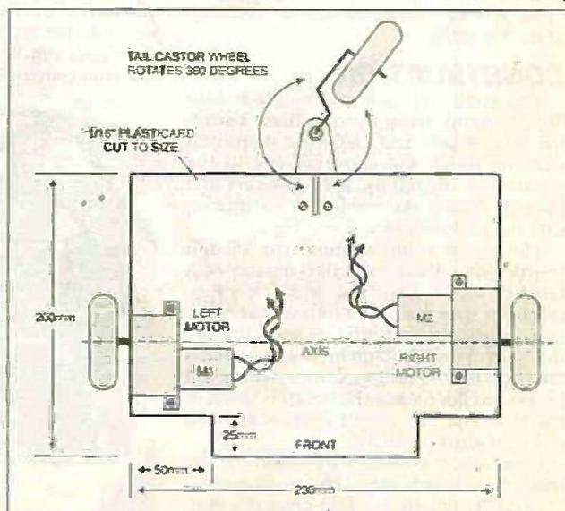
Fig.4. Dimensions of the PhizzyBot platform.
