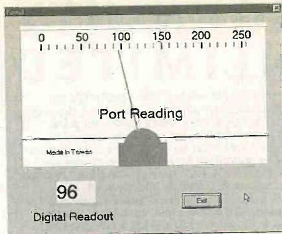
Fig.2. This virtual panel meter and digital readout requires just six lines of conventional BASIC code.
