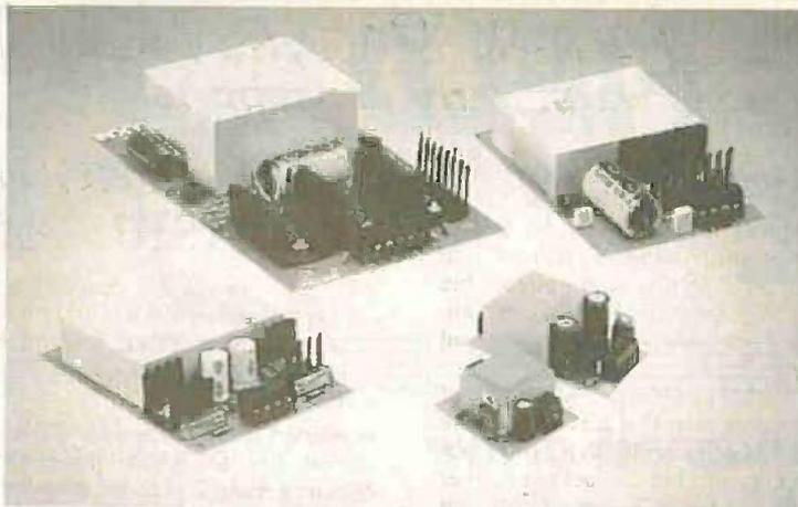
LASCAR Electronics has added a new miniature power supply to its existing (and excellent) low cost linear PSU range. The new PSU303 is a compact "open" mains power module featuring +5V (200mA) and -5V (50mA) fixed rails. It uses linear regulator i.c.s with over-current and over-temperature protection.
