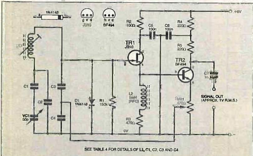
Fig.16. Circuit diagram for a narrow band Goral/Clapp variant of Colpitts oscillator.
