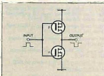
Fig. 1. Basic CMOS 4069 inverter.
