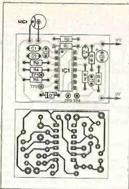
Fig.5. Printed circuit board component layout and full size copper foil master track pattern.
