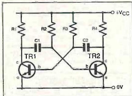
Fig. 2. A well recognised astable multivibrator circuit.
