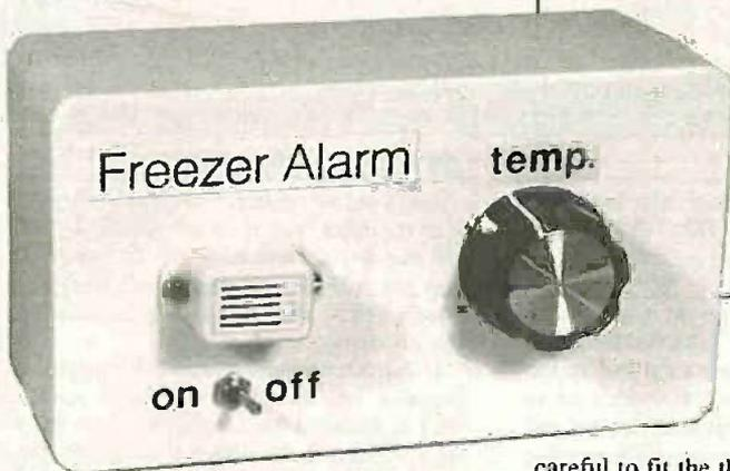
The use of a high value thermistor also helps to minimise the battery drain. Although R3 has a nominal resistance of 47 kilohms, this is its resistance at +25°C. In this application it will operate at a much lower temperature of around -20°C where its resistance is over ten times higher.
