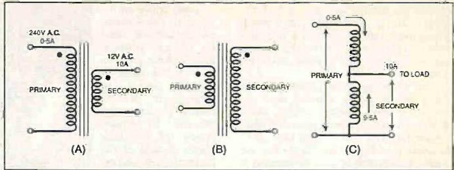
Fig.6a. Step-down transformer symbol. The "spot" indicates the direction of the windings. (b) Step-up transformer, and (c) auto-transformer.
