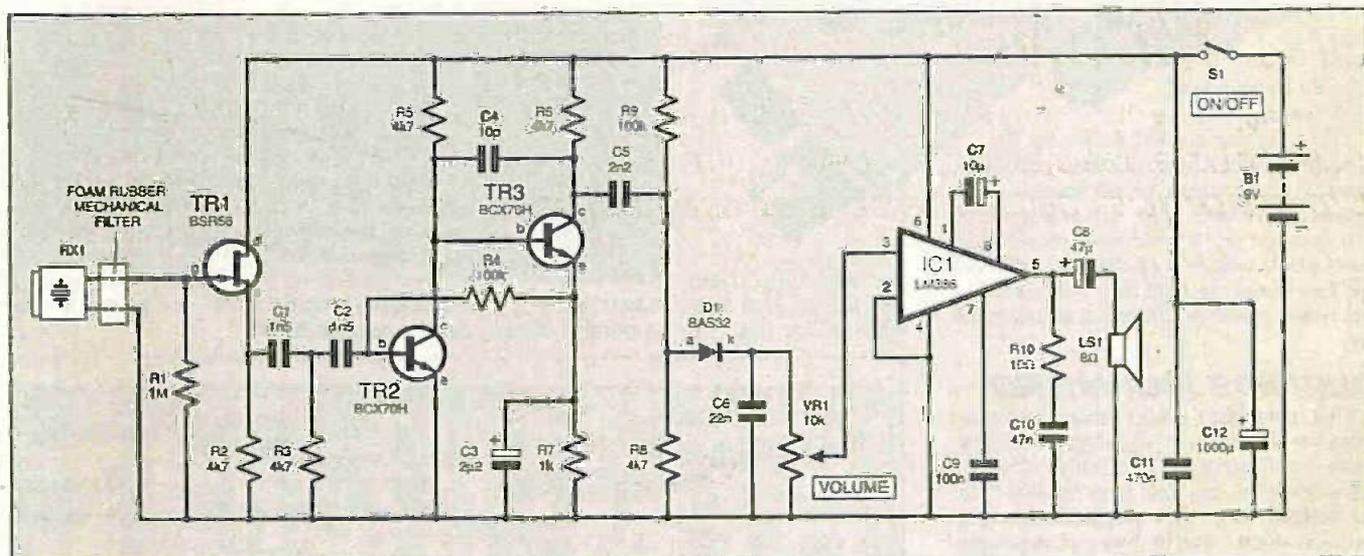
Fig.2. Full circuit diagram for the Ultrasonic Puncture Finder.
