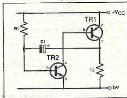
Fig. 3. Circuit diagram for the multivibrator part of the Lighting-Up Reminder.
