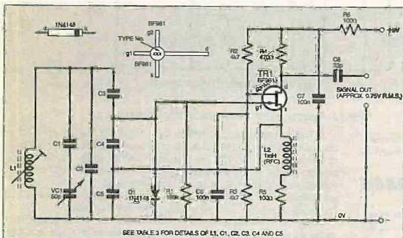
Fig.15. Circuit diagram for a narrow band Dow/Seiler variant of Colpitts oscillator.
