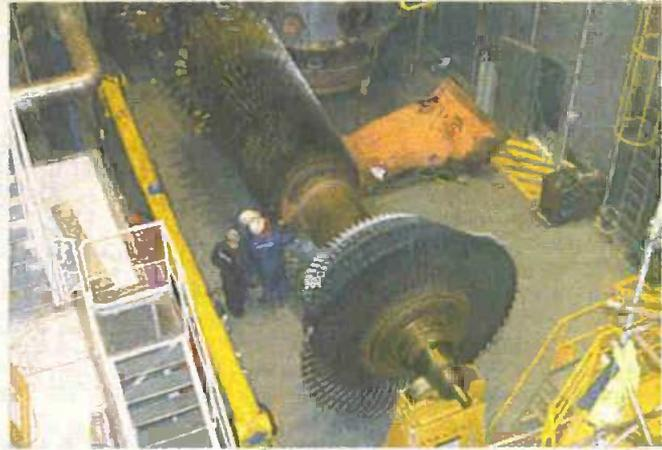
Aerial view showing gas turbine blades (largest, front) and air compressor (rear) on the shaft, undergoing inspection.
