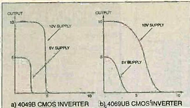
Fig.2. Comparison of switching slopes for buffered (a) and unbuffered (b) CMOS inverters.
