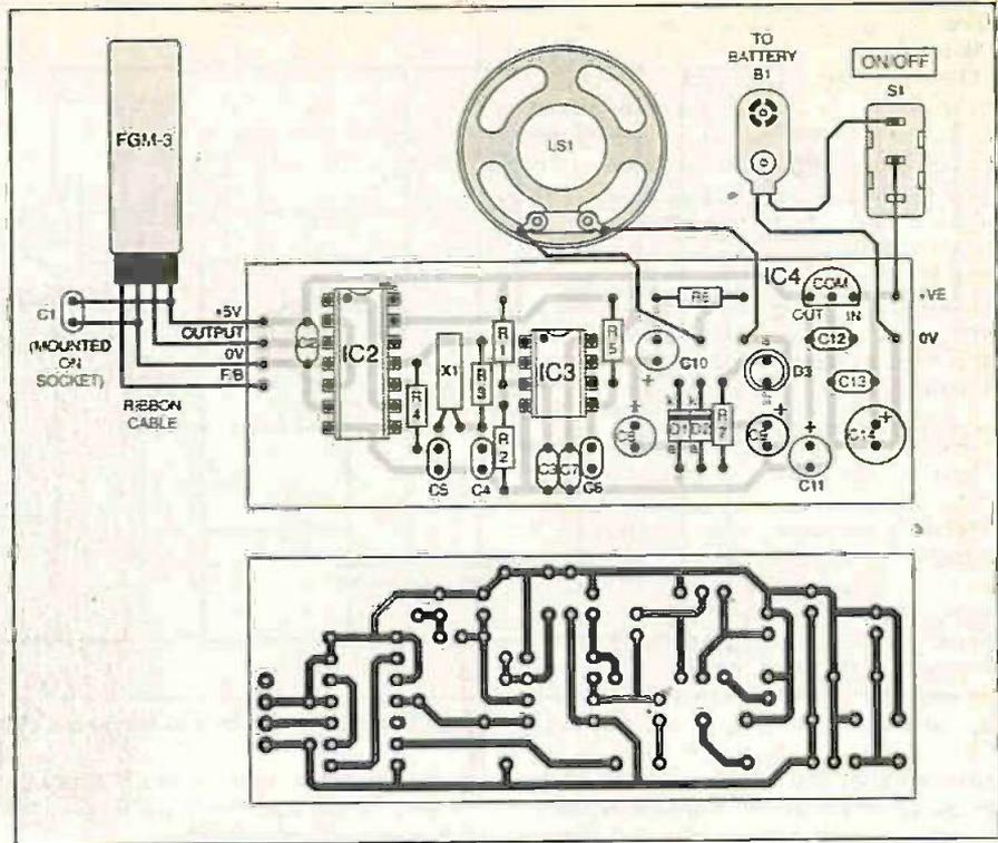
Fig.3. Component layout, full size copper foil master track pattern, and off-board interwiring details.
