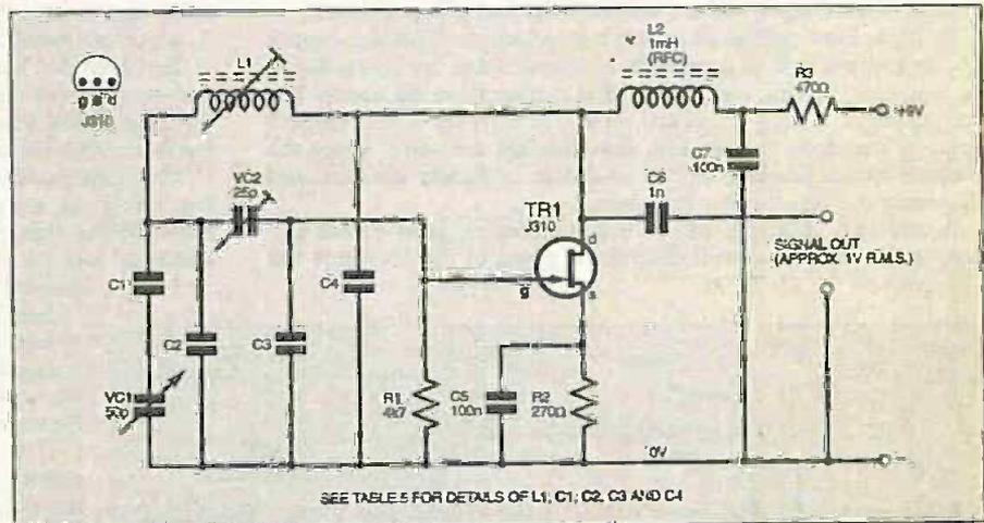
Fig.13. Narrow band Vackar oscillator using an f.e.t.
