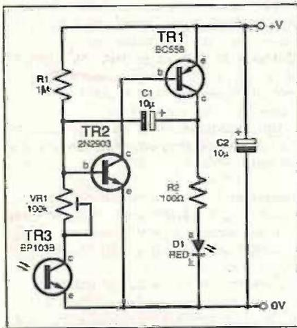
Fig. 1. Redrawn circuit diagram for the basic Lighting-Up Reminder, taken from the March '98 issue of *EPE*.
