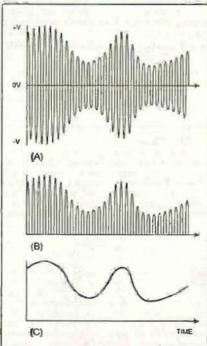
Fig. 1. Recovery of audio frequencies from an amplitude modulated signal. (a) 40kHz signal with low frequency amplitude variation (noise), (b) after diode detection before smoothing and (c) recovered audio (noise).
