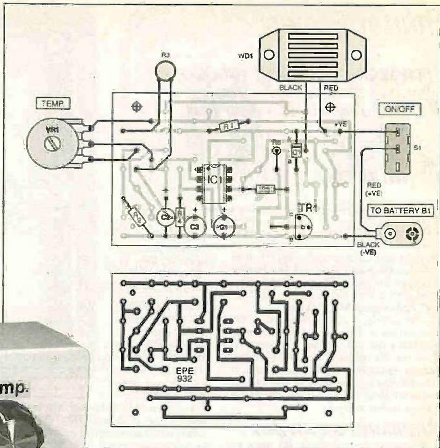
Fig. 2. Multi-project printed circuit board component layout, inter-wiring and full-size copper foil master. Double-check layout as not all holes are used.
