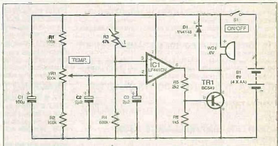
Fig.1. Complete circuit diagram for the Freezer Alarm. Component designated R3 is the thermistor temperature sensor.
