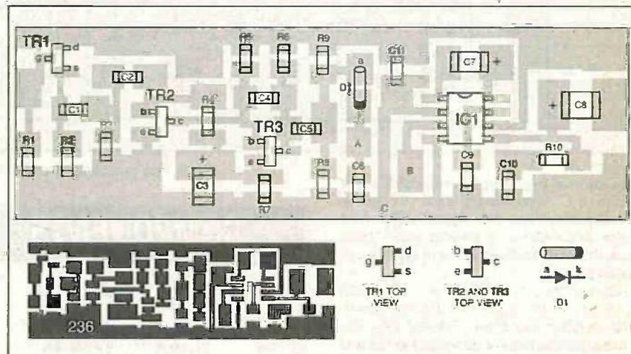
Fig.3. Layout of components on a twice-size surface mount printed circuit board and full size copper foil master pattern. The transistor and diode pinouts are also included.
