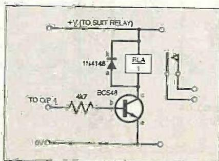
Fig.6. Interfacing to a relay.
