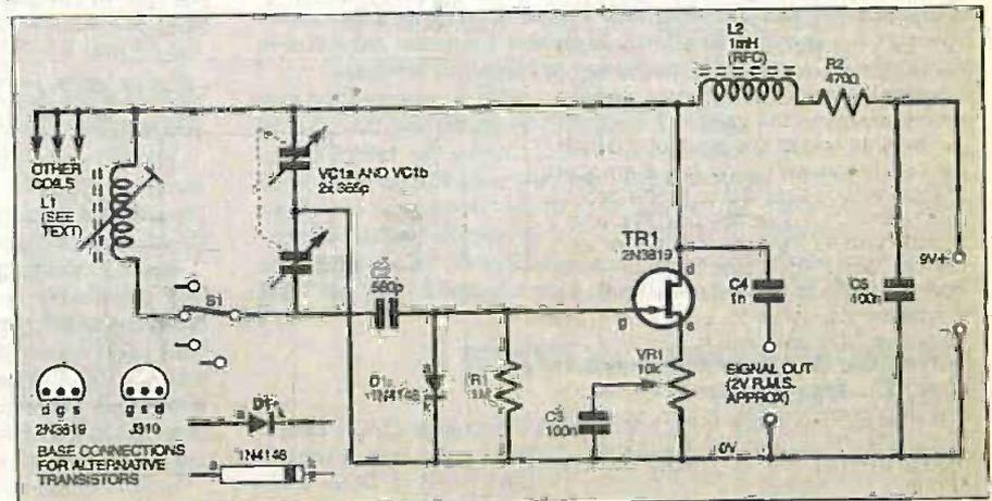
Fig.5. Circuit diagram for an r.f. oscillator, covering 150kHz to 15MHz, using an f.e.t.
