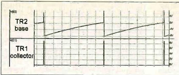
Fig.4. Screen waveform for a Lighting-Up style astable (9V supply, arbitrary timebase).
