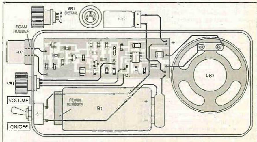
Fig.4. Positioning of components inside the small handheld case. Keep the ultrasonic transducer and loudspeaker as far apart as possible.
