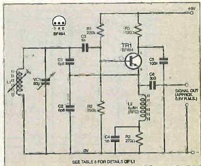
Fig.14. Circuit diagram for a v.h.f. Colpitts oscillator.
