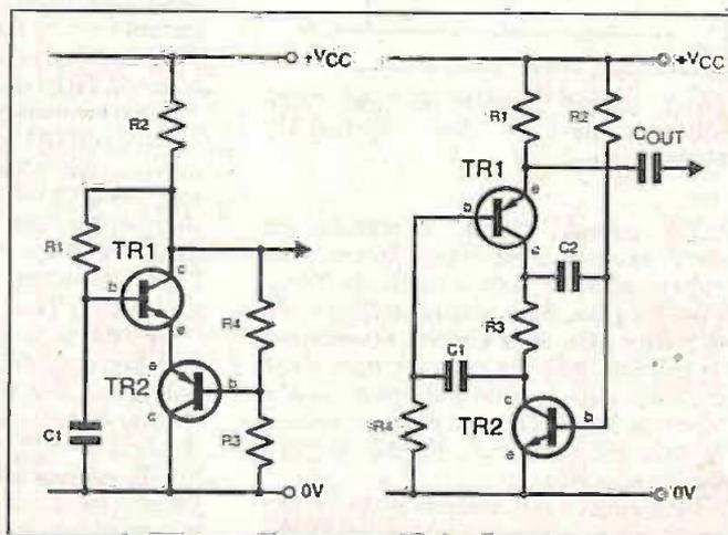
Fig.5. More complementary transistor multivibrator circuits. Can you figure out how they work?
