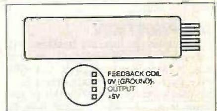
Fig.4. Connections for the FGM-3 sensor.
