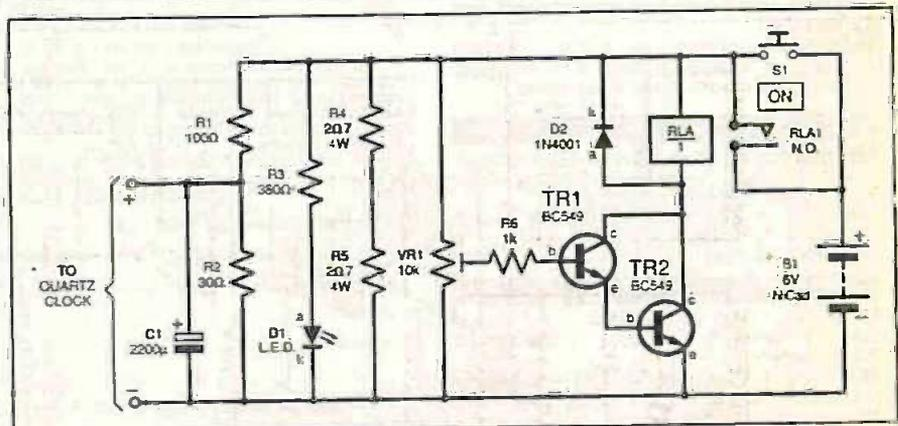
Fig. 3. Circuit diagram for a NiCad Discharge Unit.
