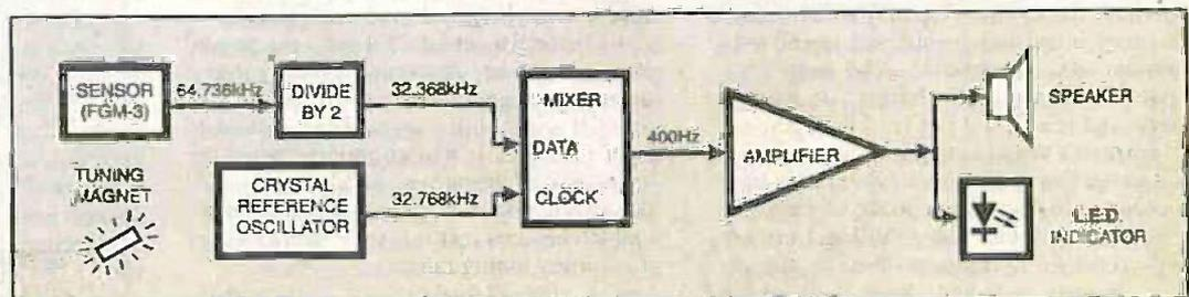
Fig. 1. Block diagram of the Magnetic Field Detective.
