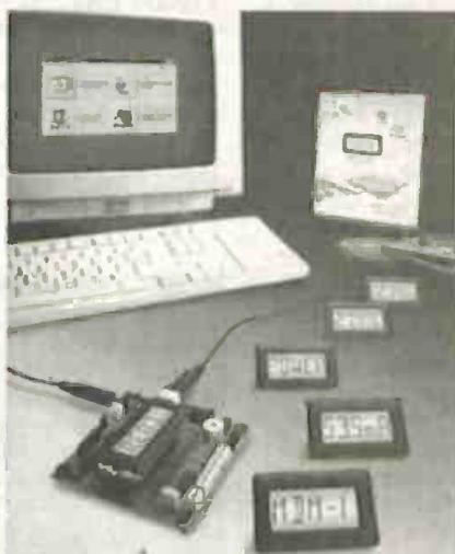
NEW from Lascar Electronics is a 5-digit starburst liquid crystal display module with an on-board Flash PICMicro. It has been designed as the building block for thousands of display and instrumentation applications.
