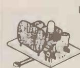
Uses "burst fire" technique to maintain temperature to within 0.5°C. Ideal for photography, incubators, wine making, etc.
