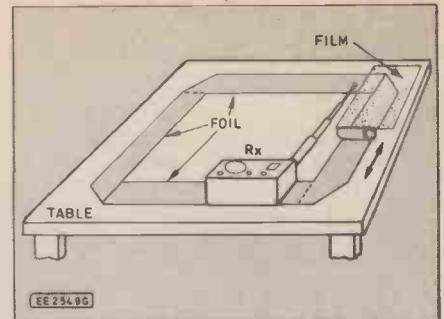
Fig. 6. Horizontal foil loop. The whip aerial must not make contact with the foil but should be extended over it as shown.
