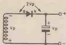
Fig. 4. During negative half-cycles when rectifier is non-conducting, the peak voltage stored in the capacitor in series with the negative voltage in the transformer winding imposes a reverse voltage of twice the peak or 2.8 times the r.m.s. across the rectifier.
