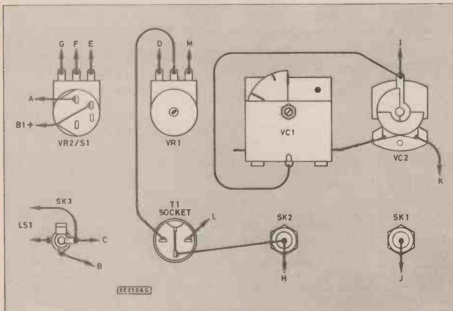
Fig. 3. Details of the wiring (use in conjunction with Fig. 2.).
