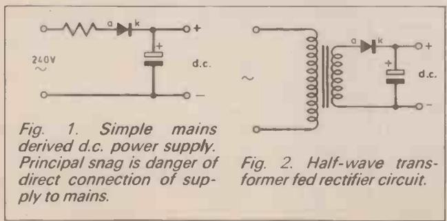
Fig. 1. Simple mains derived d.c. power supply. Principal snag is danger of direct connection of supply to mains.
