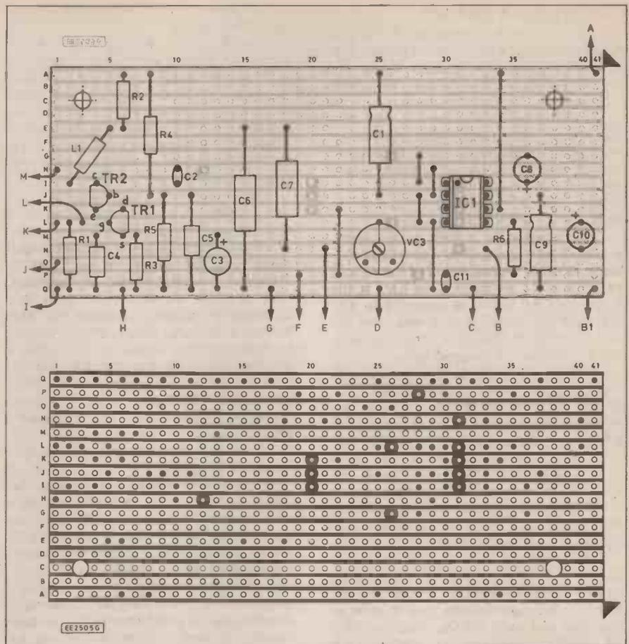
Fig. 2. Stripboard layout details
