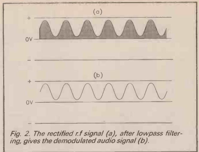
Fig. 2. The rectified r.f. signal (a), after lowpass filtering, gives the demodulated audio signal (b).
