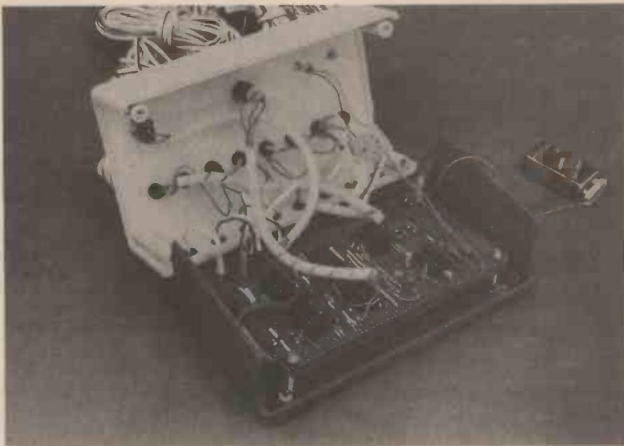
The early stripboard prototype version showing the "wiring looms" to the i.e.d.s.
