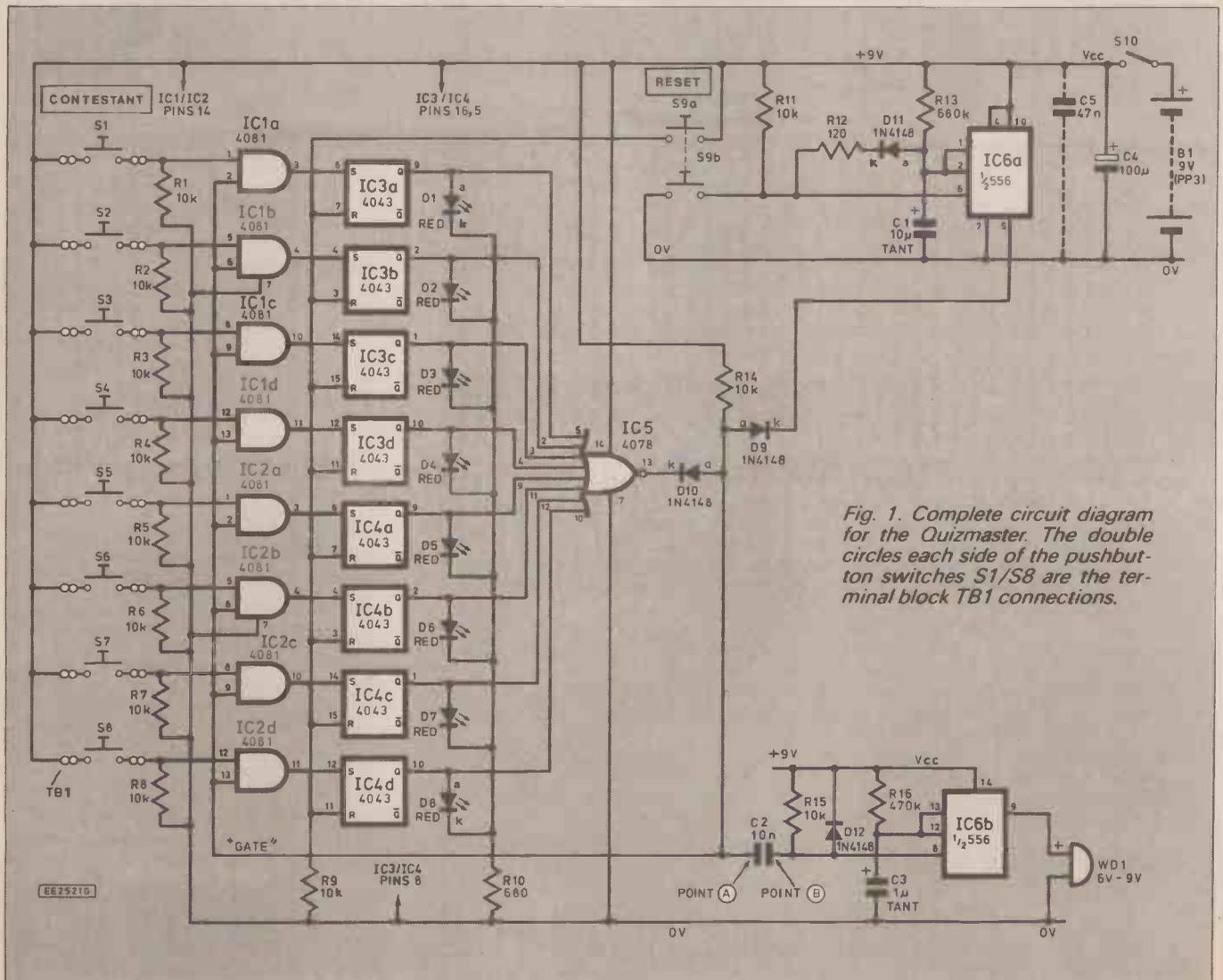
Fig. 1. Complete circuit diagram for the Quizmaster. The double circles each side of the pushbutton switches S1/S8 are the terminal block TB1 connections.
