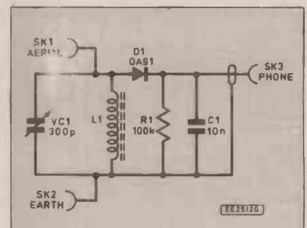
Fig. 3. The circuit diagram of the crystal set. It is purely passive — no battery is needed.
