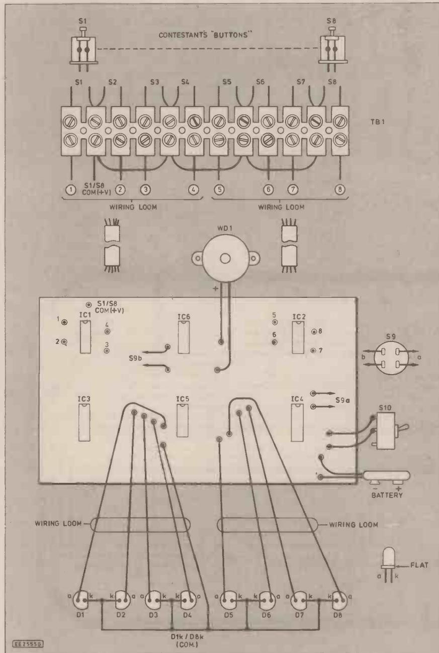
Fig. 5. Interwiring from the printed circuit board to the l.e.d.s, terminal block and contestant switches.
