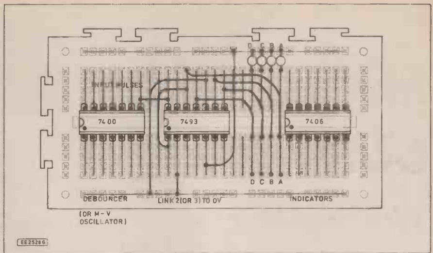
Fig. 6.4. Checking the binary counter.
