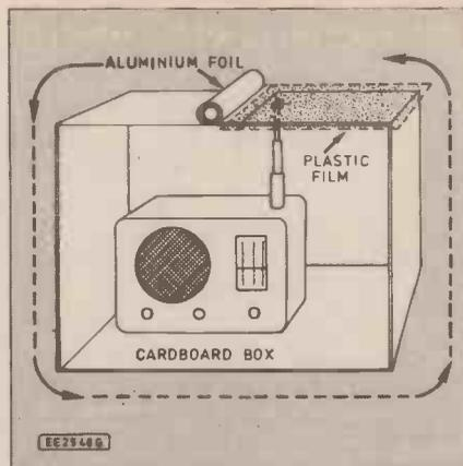
Fig. 5. Box loop. This is tuned by rolling the loose end of the foil over the plastic film.
