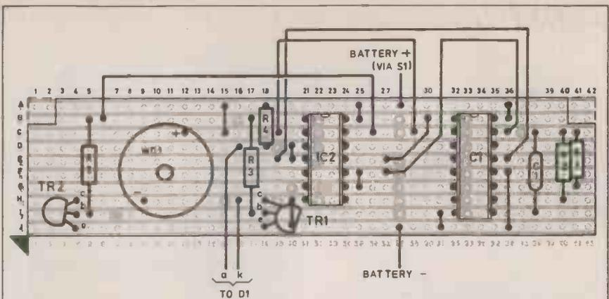
Fig. 3. Veroboard layout and wiring for the Auto Memo.
