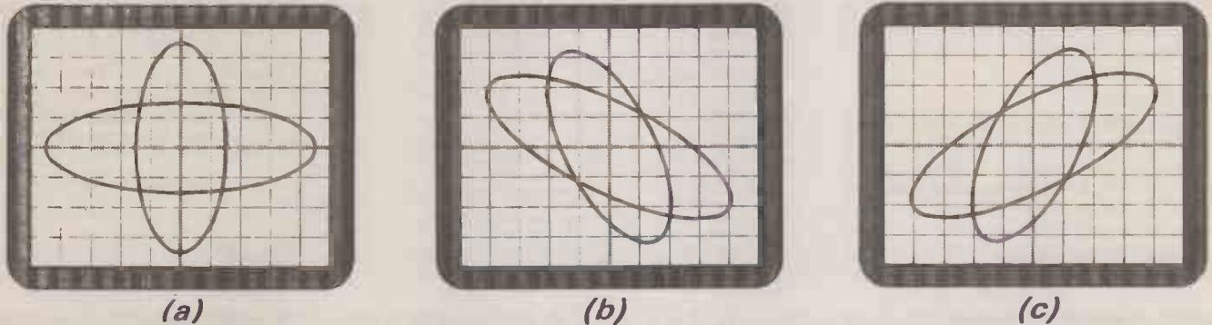
Fig. 3. Using an oscilloscope as a timing indicator. (a) indicates correct timing. While (b) and (c) show tuning errors in opposite directions.
