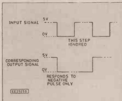
Fig. 6.1. Behaviour of binary divider
