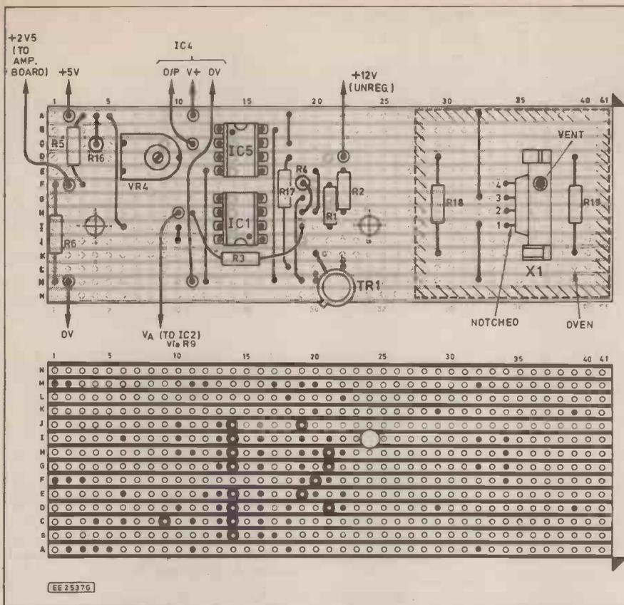
Fig. 6. Component layout and breaks in the underside copper tracks of the pressure sensing/amplifier board.
