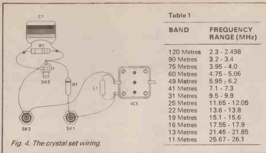
Fig. 4. The crystal set wiring.
