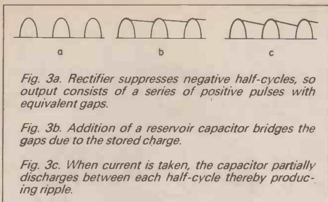
Fig. 3a. Rectifier suppresses negative half-cycles, so output consists of a series of positive pulses with equivalent gaps.
