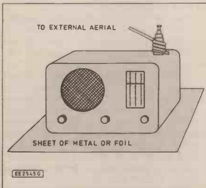
Fig. 2. Where no aerial terminals exist an external aerial can be coupled by wrapping its insulated downlead round the built-in whip aerial. Note that no direct connection is made. Placing the receiver on a sheet of metal often improves reception.
