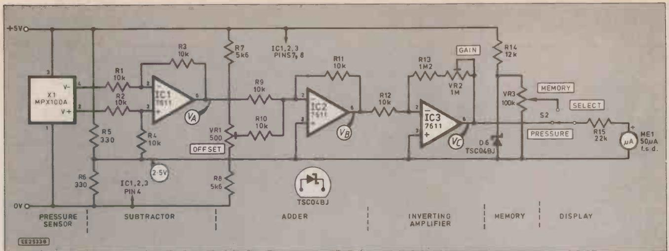
Fig. 2. Pressure-sensing and amplifying circuit diagram for the Electronic Barometer
