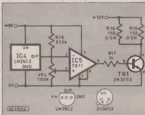
Fig. 3. Thermostat circuit diagram for the "oven".
