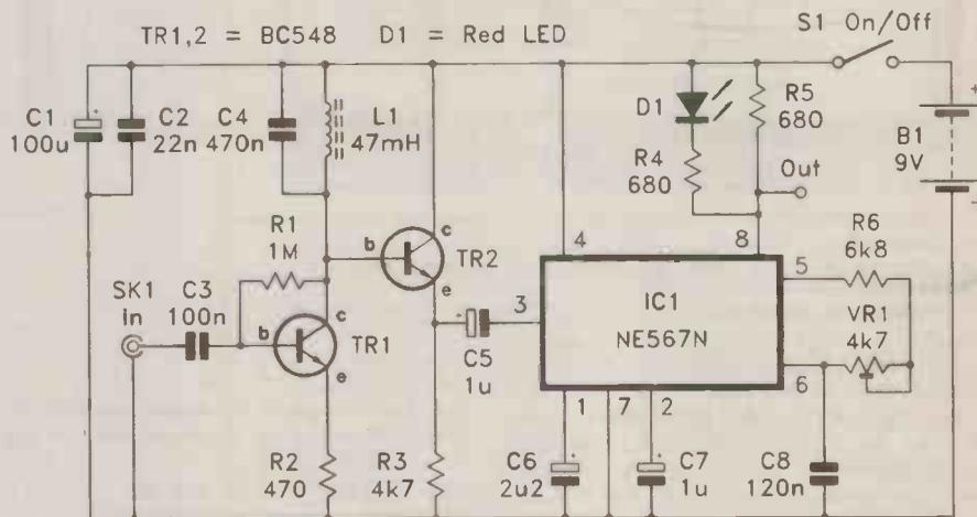
Fig. 1. A simple CW Tone Decoder based on a phase-locked-loop i.c.
