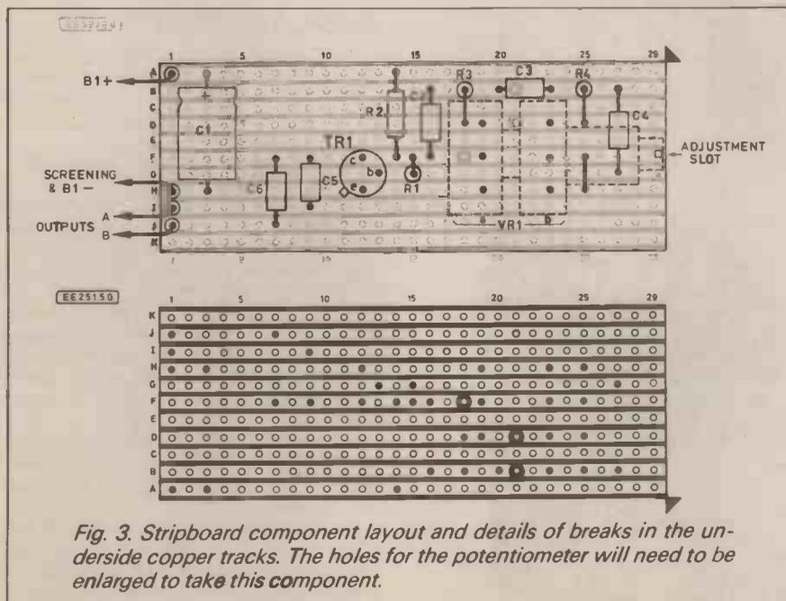
Fig. 3. Stripboard component layout and details of breaks in the underside copper tracks. The holes for the potentiometer will need to be enlarged to take this component.
