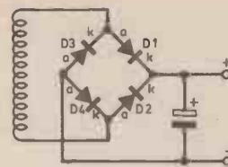
Fig. 7. A bridge circuit provides full-wave rectification without a transformer centre tap.
