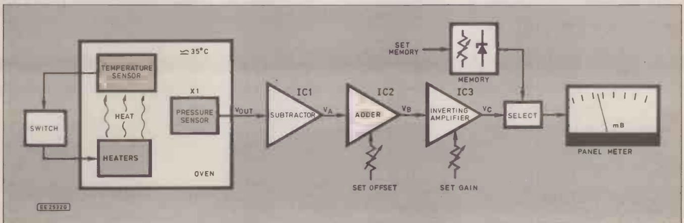
Fig. 1. System block diagram for the Electronic Barometer
