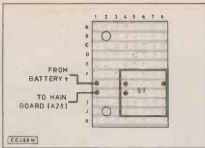
Fig. 4. Circuit board for S1.
