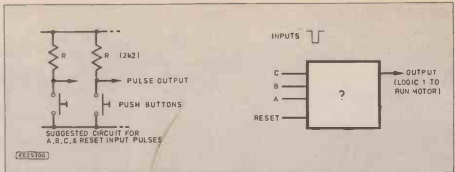
Fig. 6.6. Motor control example. To start the motor, A must be pressed first, then B and C together.
