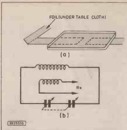
Fig. 8(a). Concealed table-top loop. A thin table cloth (not shown) conceals the foil, and provides a dielectric. A metal tray moved over the gap in the foil tunes the loop. (b) Equivalent loop circuit plus receiver coupling coil.
