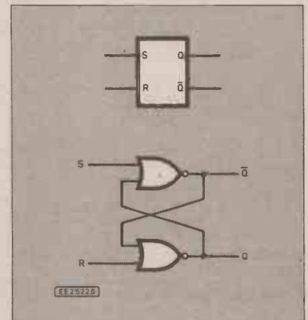
Fig. 2. Block and circuit schematic for the RS latch.
