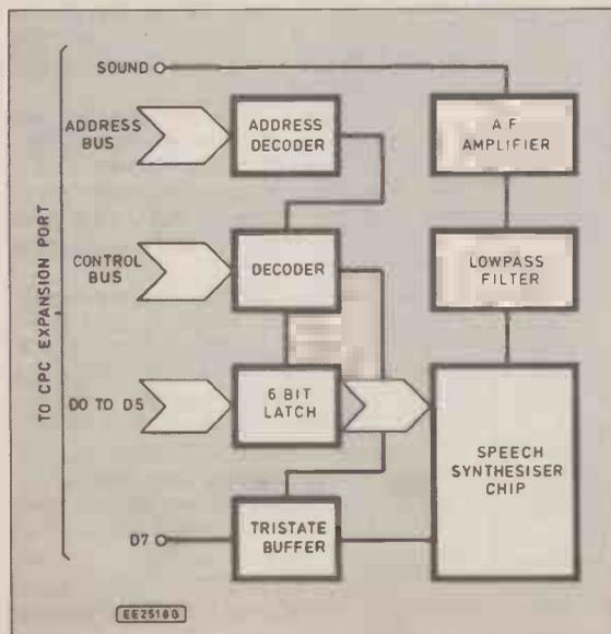
been produced. Timing loops are not really a viable alternative as the allophones have various durations from 10ms to 420ms. An accurately timed flow of data is essential if a good quality output is to be achieved.
