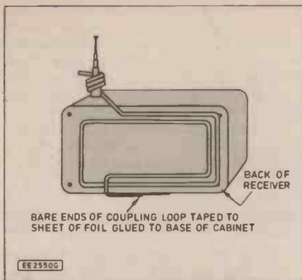
Fig. 7. How to attach a coupling loop to the receiver.
