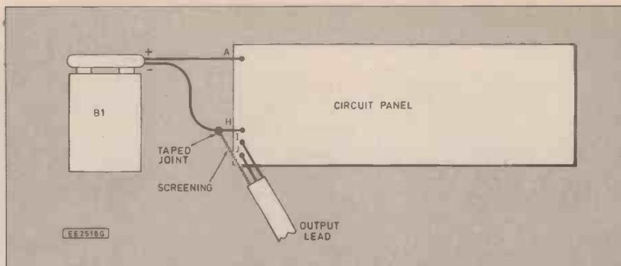
Fig. 4. Interwiring from the circuit battery board to the screened output lead and battery.
