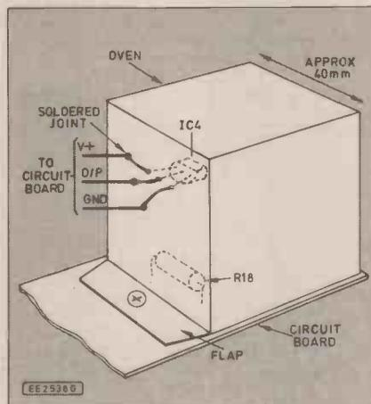
Fig. 7. Mounting the temperature sensor in the "oven".
