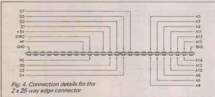
Fig. 4. Connection details for the 2 x 25 way edge connector.
