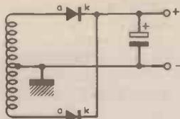
Fig. 5. A full-wave rectifier circuit using a centre-tapped winding.
