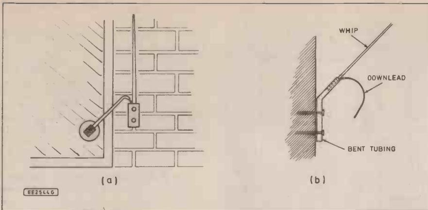
Fig. 1(a). External whip aerial with capacitive coupling through the window glass. (b) Simple mounting bracket.
