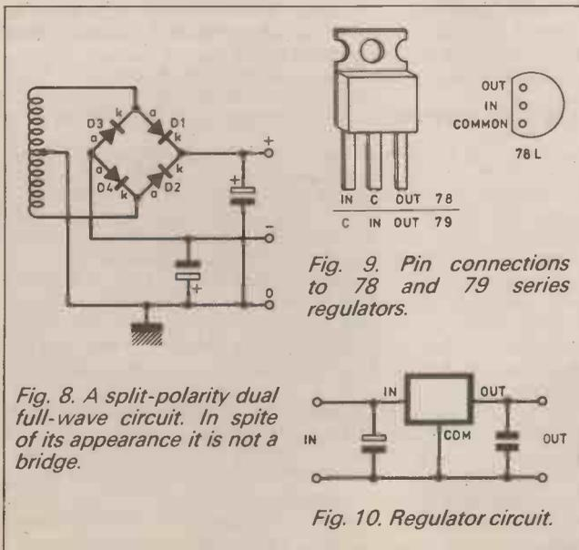
Fig. 8. A split-polarity dual full-wave circuit. In spite of its appearance it is not a bridge.
