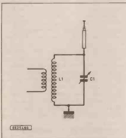
Fig. 3. In many receivers the built-in whip is connected directly to the live side of the signal-frequency tuned circuit L1/C1.
