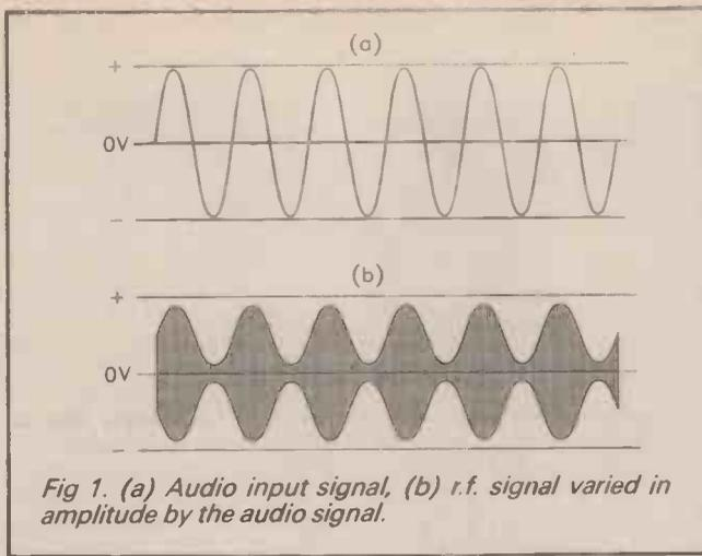
Fig 1. (a) Audio input signal, (b) r.f. signal varied in amplitude by the audio signal.
