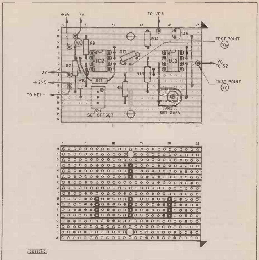
Fig. 8. Component layout and details of breaks in the underside copper tracks of the adder/inverter board.
