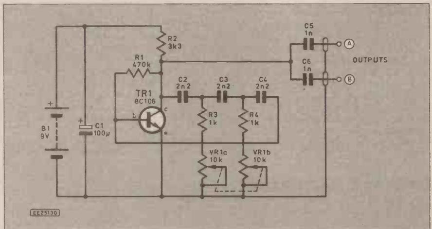
Fig. 1. Complete circuit diagram for the Azimuth Adjustment Aid.
