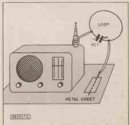
Fig. 4. Coupling arrangements for a tuned loop aerial.
