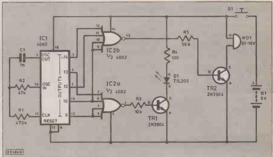
Fig. 1. Circuit diagram of the Auto Memo
