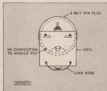
Fig. 4. Method of fitting the Toko coils to three-way DIN plugs
