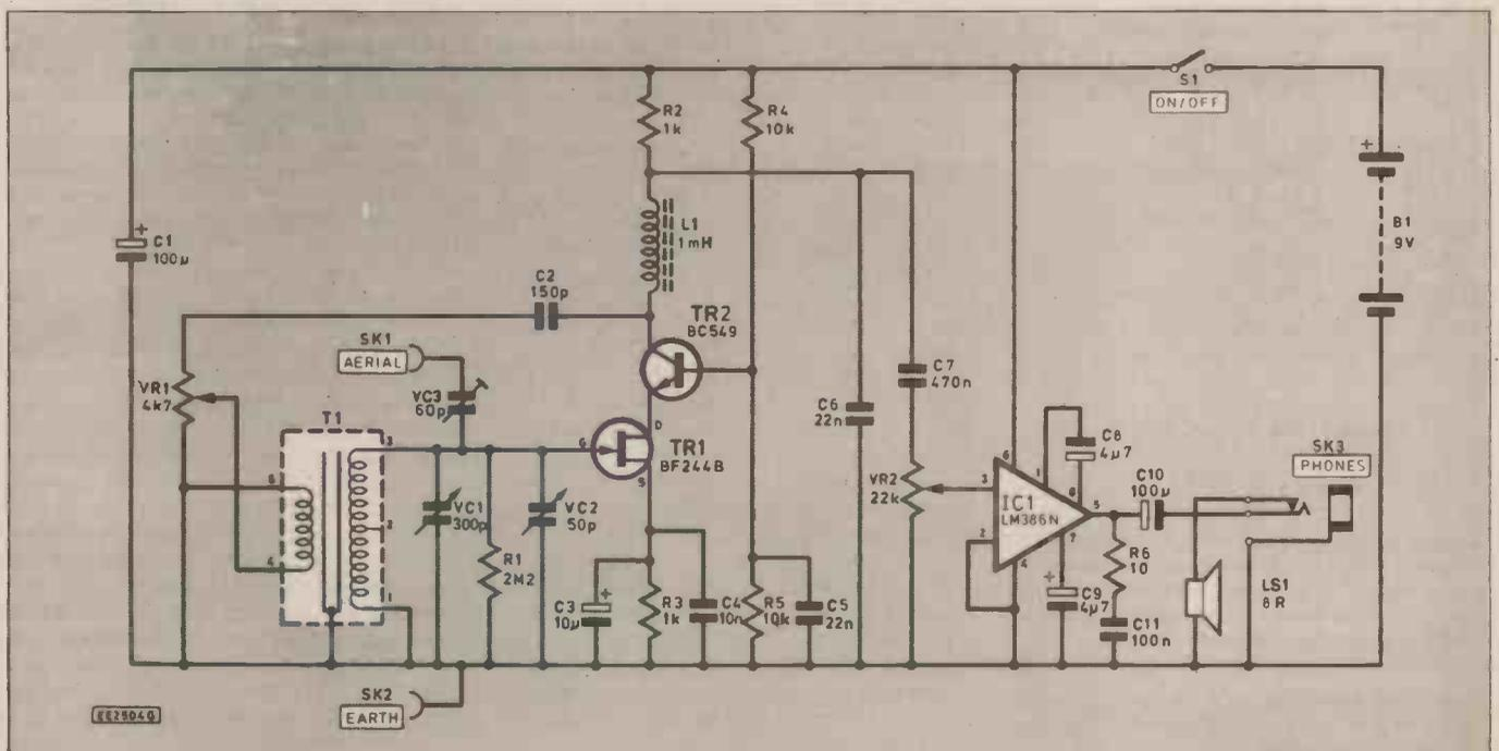
Fig 1. Full circuit diagram of the T.R.F receiver
