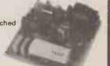
This small PCB, just 50 x 50mm will accept 8-24V input and give a stable 5V DC at up to 2A output. The 6 transistor circuit provides current overload protection, thermal cut-out and excellent filtering. Offered at the remarkably low price of just..... £5.00
