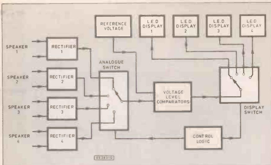
Fig. 2. Block diagram for the "cost saving" time division multiplexing system.
