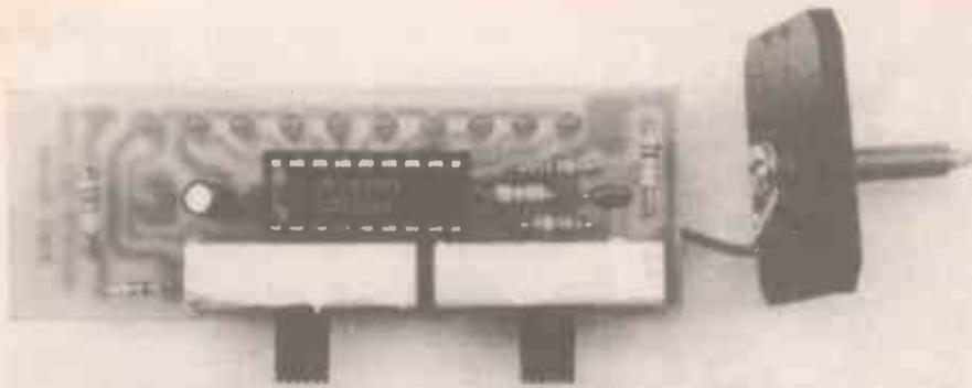
The completed circuit board with the slide switches soldered in position. Resistor R1 is mounted track side - see photo below.
