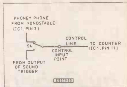
Fig. 5. Fitting a mode select switch to the Phoney Phone (Aug '90).
