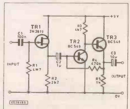
Fig. 2.9. Adding an f.e.t. input stage to obtain a very high input impedance
