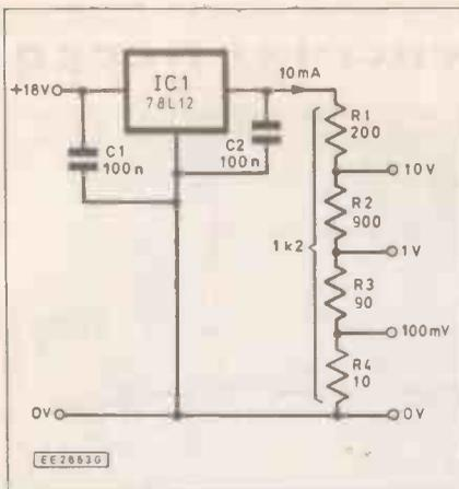
Fig. 2.22. Voltage calibrator circuit (solution to last month's Design Problem)
