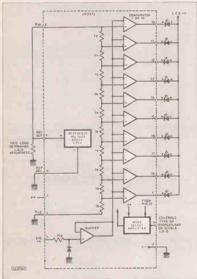
Fig. 2. Internal circuit details for the LM3914N i.c.
