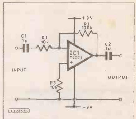
Fig. 2.17. Practical inverting amplifier
