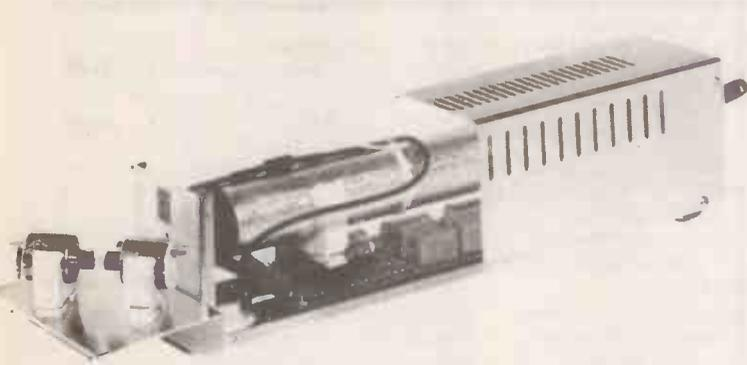
An almost infinite number of circular patterns can be projected onto a wall or ceiling with this super laser show equipment.
