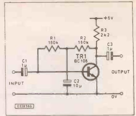
Fig. 2.5. Reducing the amount of a.c. feedback
