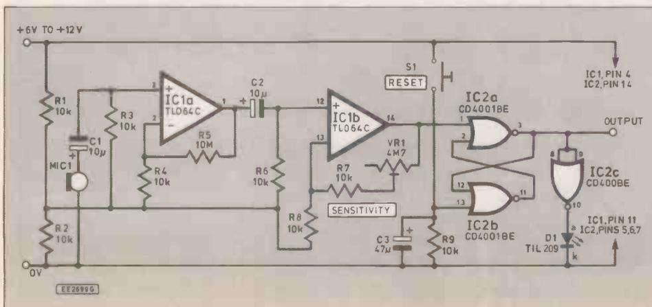
the second amplifier is normally about 1V, so satisfies this requirement. The other input of the bistable is connected to the 0V rail through resistor R9.
