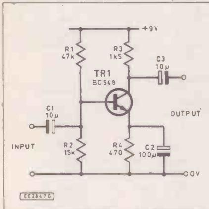
Fig. 2.6. Emitter stabilised common-emitter amplifier stage
