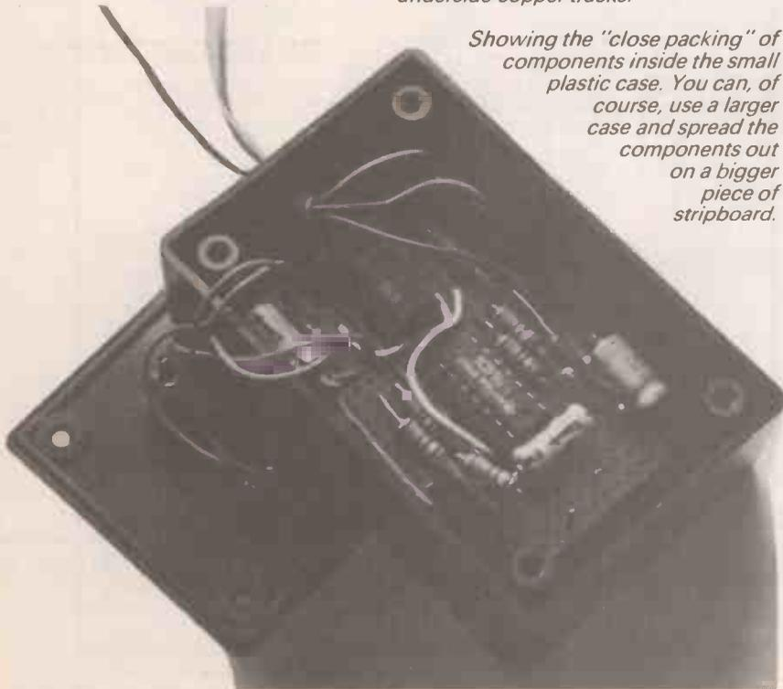
is connected to the case. If so, this is the terminal to be wired to the solder pin at A10. The "earthed" case shields the microphone element from interference.
