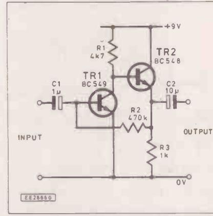
Fig. 2.7. Two-stage amplifier with low-impedance output
