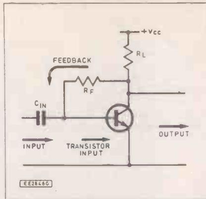
Fig. 2.4. Feedback path in the simple common-emitter stage
