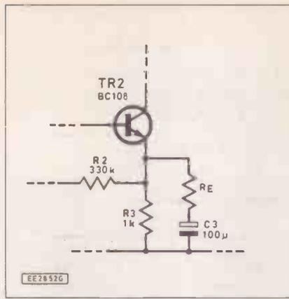
Fig. 2.12. Modification to the general purpose transistor amplifier module in order to permit gain setting
