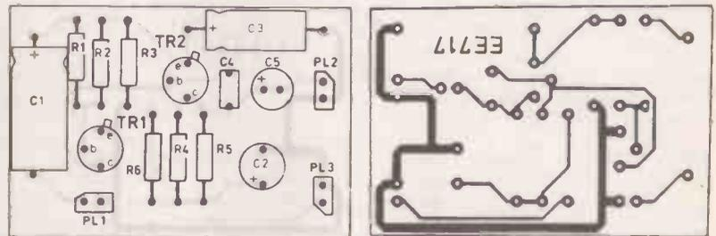
Fig. 2.14. P.C.B. layout for the general purpose transistor amplifier module
