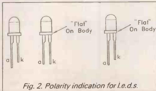
Fig. 2. Polarity indication for l.e.d.s.
