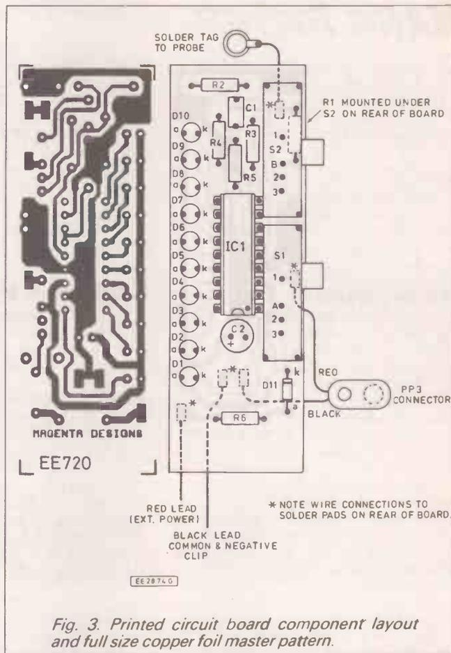
Fig. 3. Printed circuit board component layout and full size copper foil master pattern.
