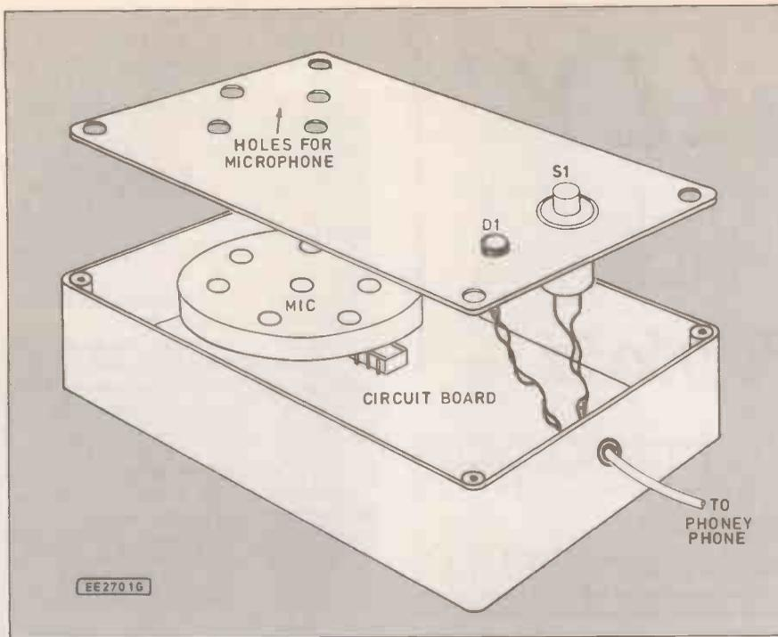
Fig. 4. Guide to the layout of components inside the small plastic case. The microphone insert sits above IC1 and is held in place with a piece of Bluetack.
