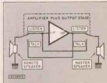
Fig. 1. Block diagram of a basic intercom
