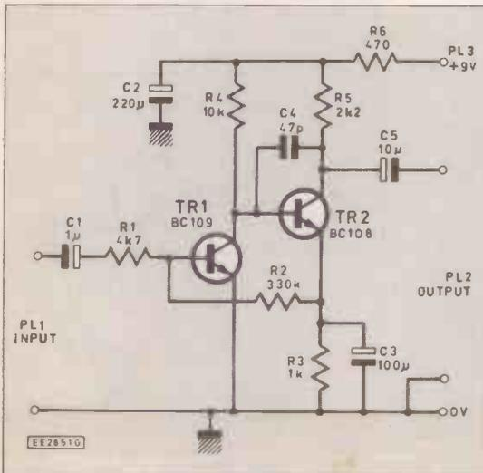
Fig. 2.11. General purpose transistor amplifier module
