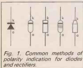
Fig. 1. Common methods of polarity indication for diodes and rectifiers.
