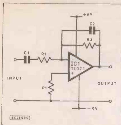
Fig. 2.19. Bandwidth limited inverting operational amplifier
