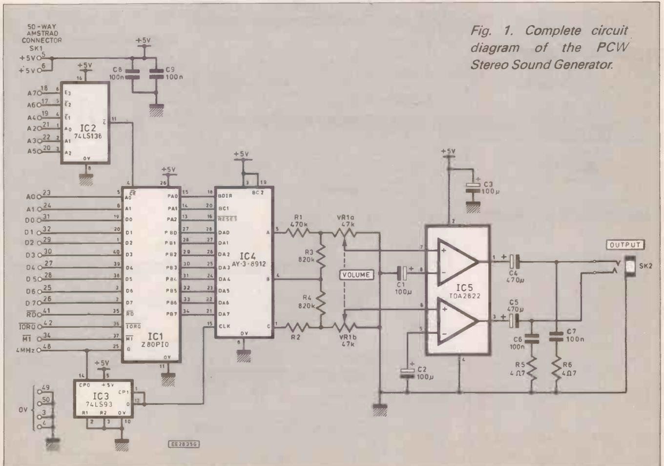
Fig. 1. Complete circuit diagram of the PCW Stereo Sound Generator.
