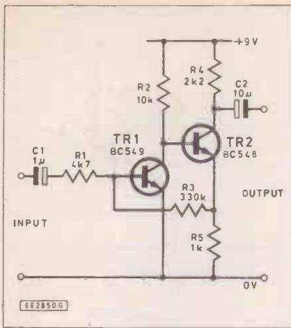
Fig. 2.10. Two-stage high gain amplifier
