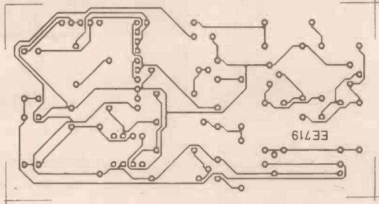
Fig. 5. P.C.B. layout for the simple intercom.
