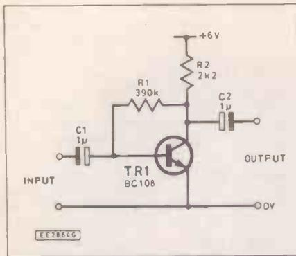
Fig. 2.3. Simple common-emitter amplifier stage
