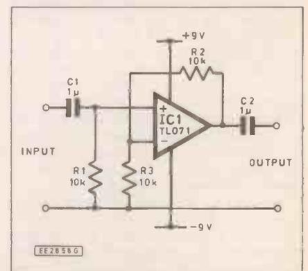
Fig. 2.18. Practical non-inverting amplifier
