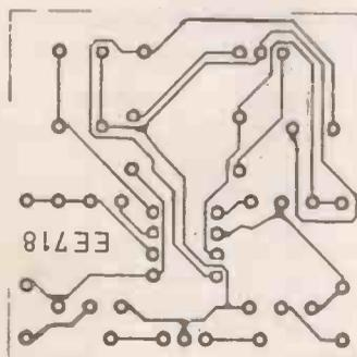
Fig. 2.21. P.C.B. layout for the general purpose operational amplifier module
