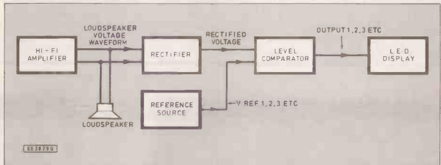
Fig. 1. Spatial Power Display block diagram and waveforms (below) showing the basic principle of operation
