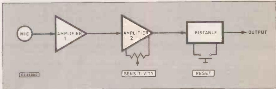
Fig. 1. Block diagram for the Sound Trigger.
