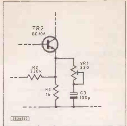
Fig. 2.13. Modification to the general purpose transistor amplifier module in order to permit variable gain adjustment
