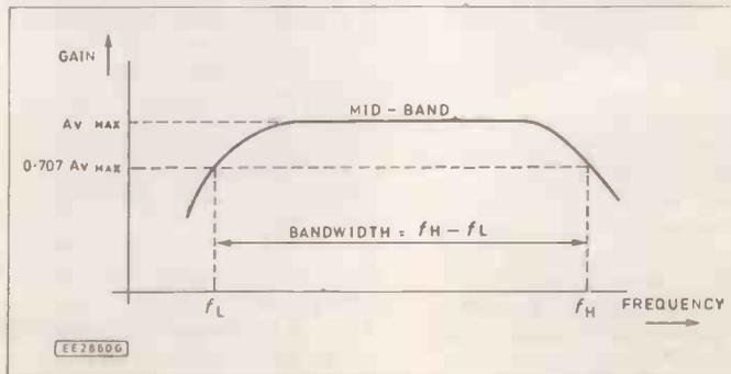
Fig. 2.1. Typical frequency response for a small-signal amplifier
