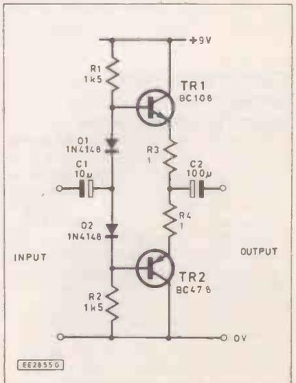
Fig. 2.15. Low-power complementary output driver for use with low impedance loads.
