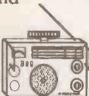
SW1 7-23MHZ, SW2 3-7.2MHZ AFC, direction finder, fine tuning mains or battery.
