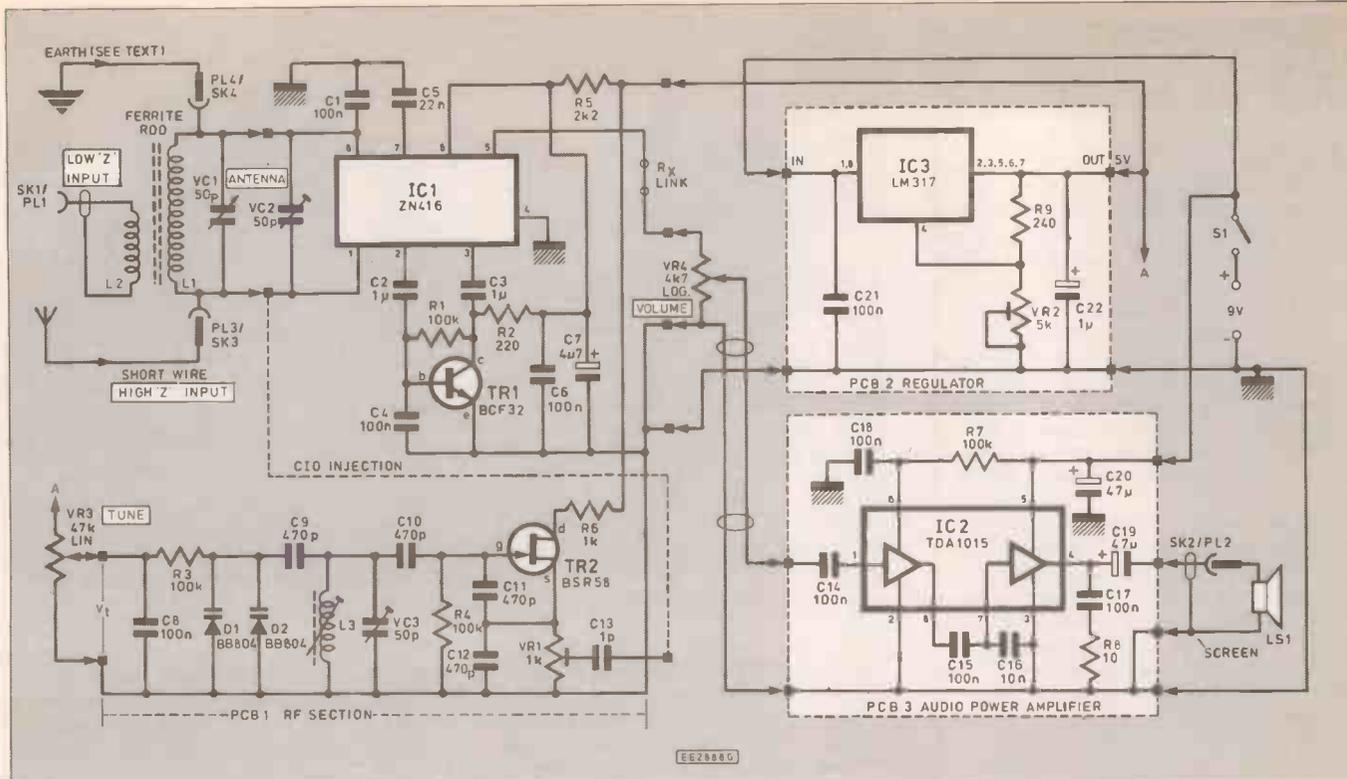
Fig. 4. Complete circuit diagram of the Gingernut. The three printed circuit boards are indicated by the dotted section.
