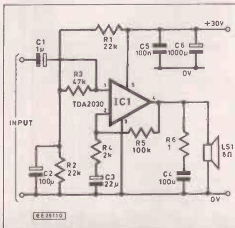
Fig. 3.20 TDA2030 power amplifier (single supply)
