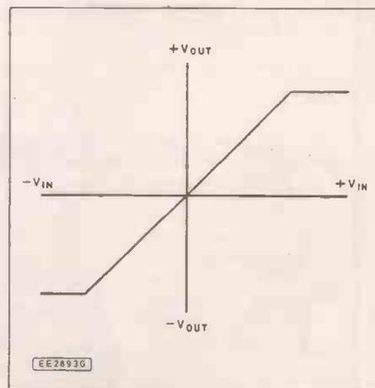
Fig. 3.1 Transfer characteristic for a typical power amplifier
