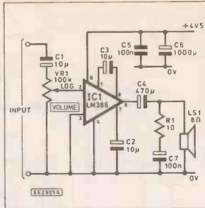
Fig. 3.14 I.C. audio power amplifier based on an LM386
