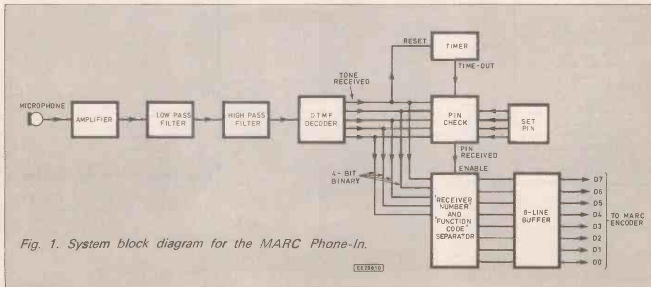
Fig. 1. System block diagram for the MARC Phone-In.
