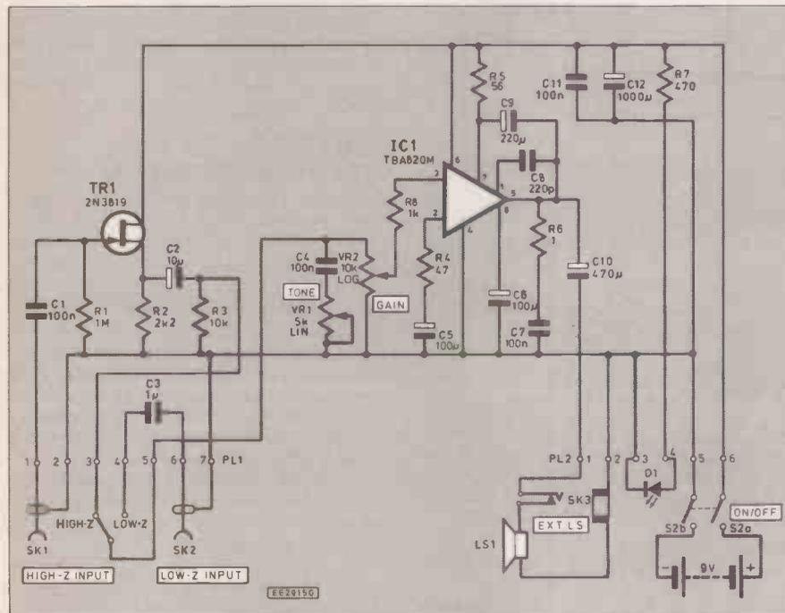
Fig. 2. Complete circuit of the Bench Amplifier/Signal Tracer
