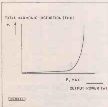
Fig. 3.4 Relationship between total harmonic distortion and output power (note the onset of clipping)
