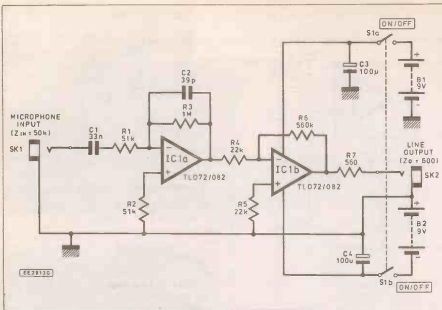
Fig. 3.21 Microphone preamplifier (solution to last month's Design Problem)
