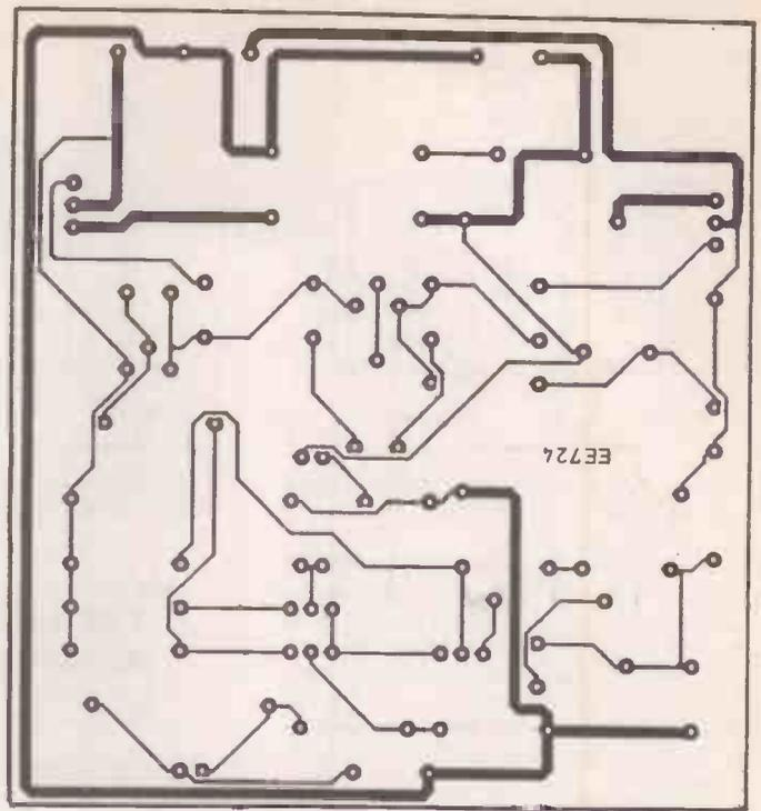
Fig. 3.12 P.C.B. layout for the high quality power amplifier module
