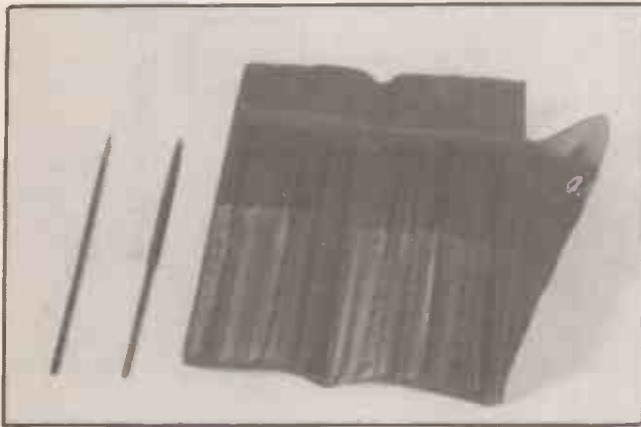
*A set of miniature files is one of the most useful items for electronic project construction.*
