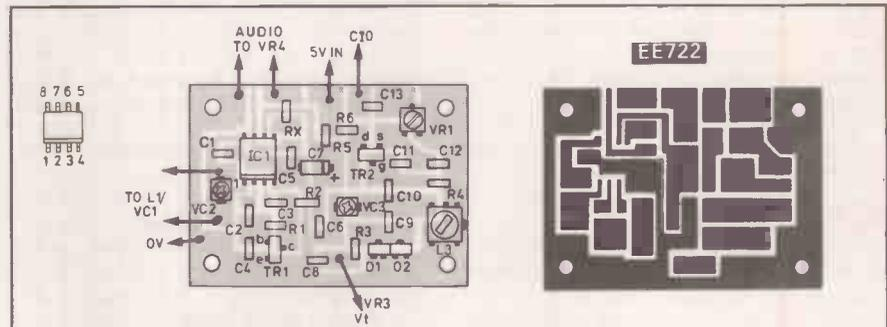
Fig. 5. Component layout and full size copper foil master pattern for the r.f. stages.
