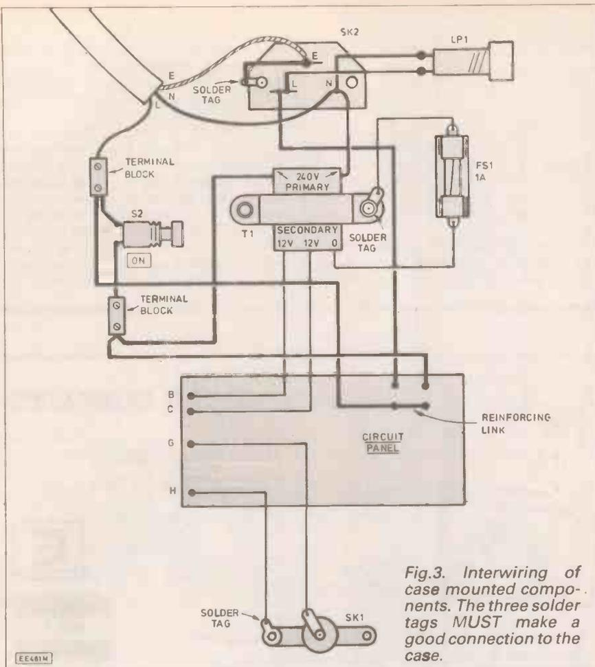
Fig. 3. Interwiring of case mounted components. The three solder tags MUST make a good connection to the case.
