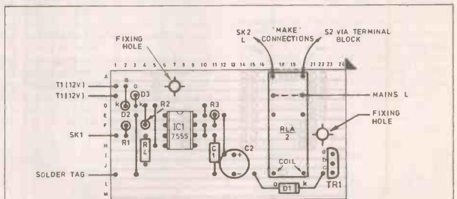
Fig. 2. Veroboard layout and wiring.
