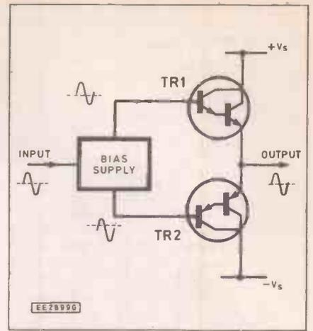
Fig. 3.7 Complementary output stage based on power Darlington transistors
