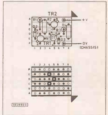
Fig. 3. Component layout and details of breaks required in the underside copper tracks.
