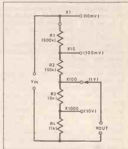
Fig. 3. (a) Step attenuator for millivoltmeter, with resistance values for an impedance of one megohm.
