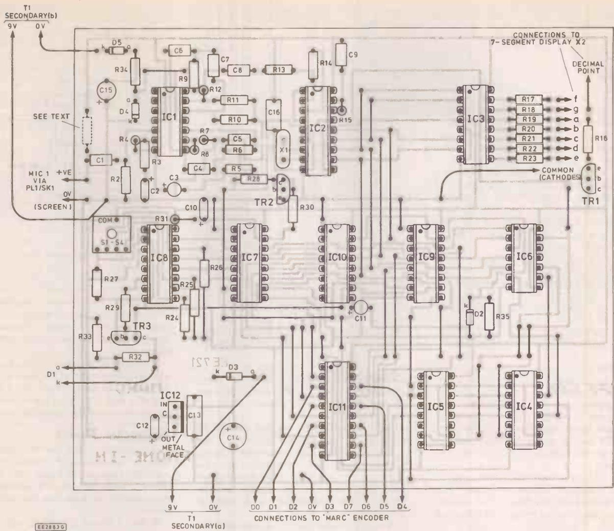
Fig. 3. Printed circuit board component layout and full size copper foil master pattern.
