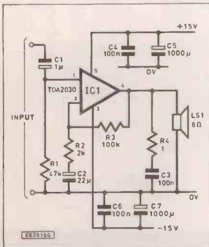
Fig. 3.19 TDA2030 power amplifier (dual supply)
