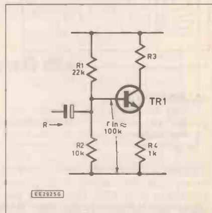
Fig. 2. A calculator with a reciprocal function makes it easy to find the a.c. input resistance of this amplifier.
