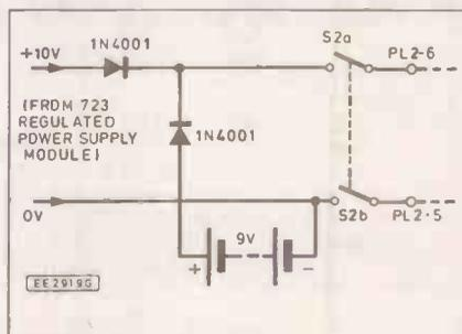
Fig. 7. Modifications for dual mains/battery operation
