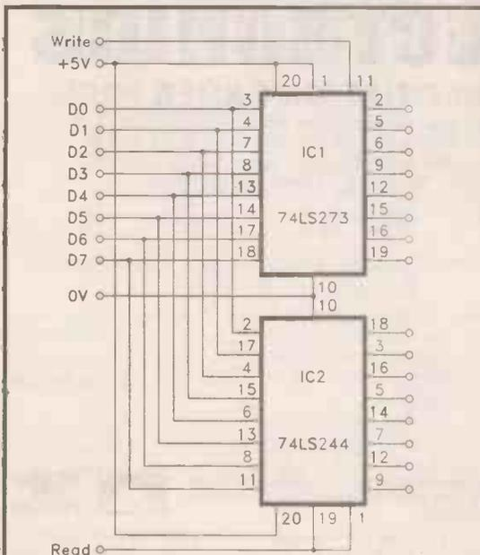
Fig. 1. Simple circuit for providing 8-bit input and output ports for use with the address decoder circuits provided last month.
