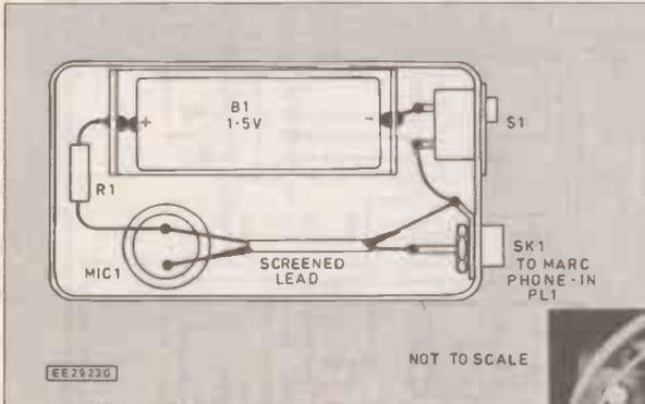
Fig. 4. Layout and wiring of the microphone pick-up unit.
