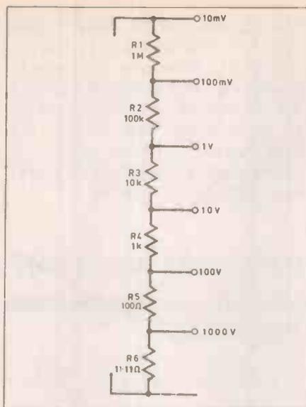
requirement becomes 1M, 100k, 10k, 1.11...k. True, the input resistance is now 1.11M, but who cares, so long as it's high? The only awkward value is 1.11...k. A bit of fiddling with my calculator shows that it is obtained exactly from 1.2k and 15k in parallel (both E12 values).
