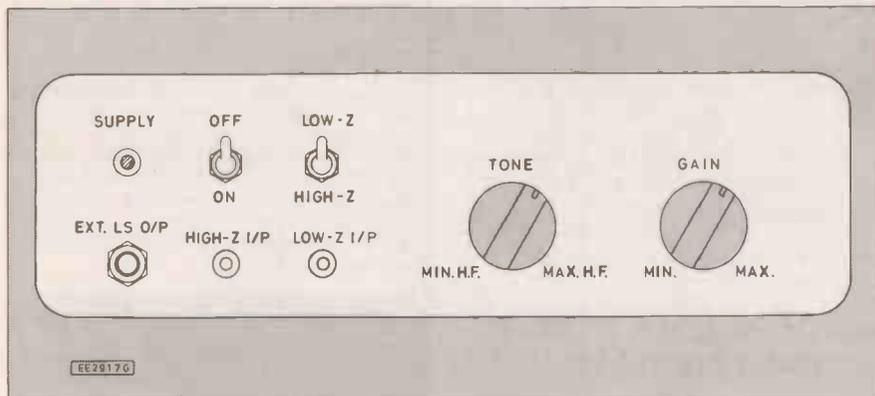
Fig. 4. Recommended front panel layout
