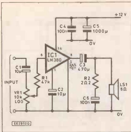
Fig. 3.13 Simple i.c. audio power amplifier using an LM380
