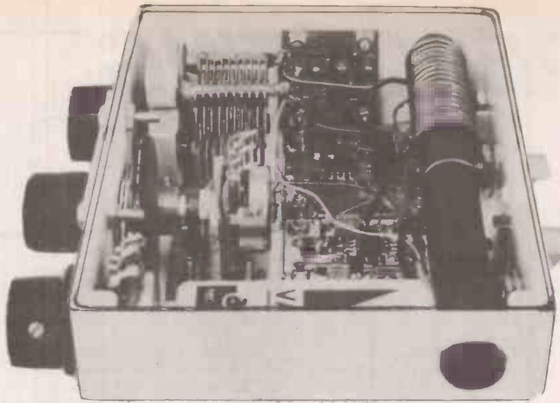
follow it down with the v.f.o. to make sure the whole band is covered. VC2 and L1 may be adjusted to get most of the band in the higher tuning voltage range. The tuning dial can be calibrated at least every 50kHz or so. The scale will not be linear being compacted at the low end.
