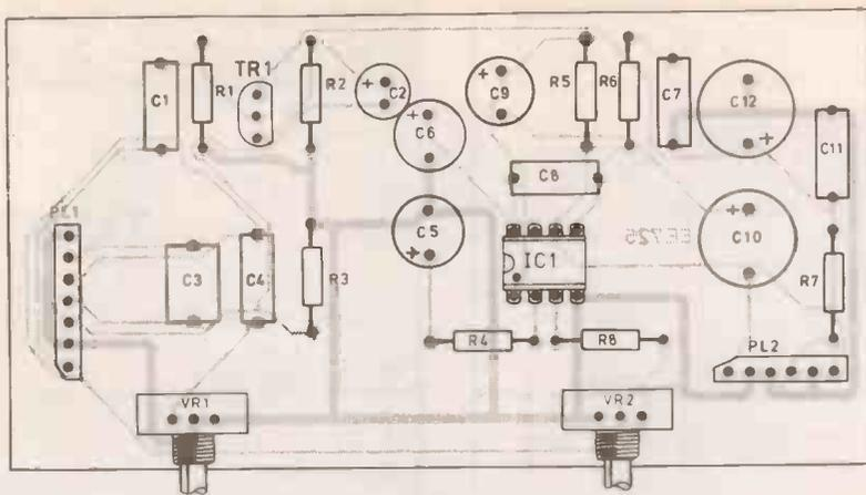
EE2016G Fig. 3. P.C.B. copper foil and component layout
