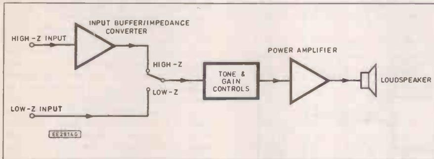
Fig. 1. Block diagram of the Bench Amplifier/Signal Tracer
