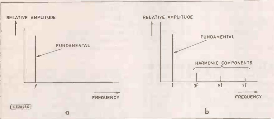
Fig. 3.3(a) Frequency spectrum associated with the output signal in Fig. 3.2(a)
