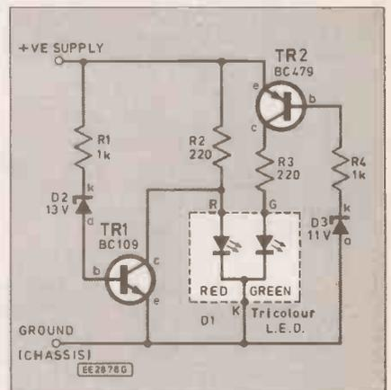
Fig. 1. Full circuit diagram for the Vehicle Voltage Monitor.
