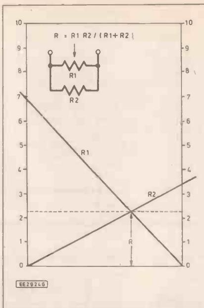
Fig. 1. Parallel resistance calculator. The lines between 0 and R1, 0 and R2 intersect at a height which gives R.
