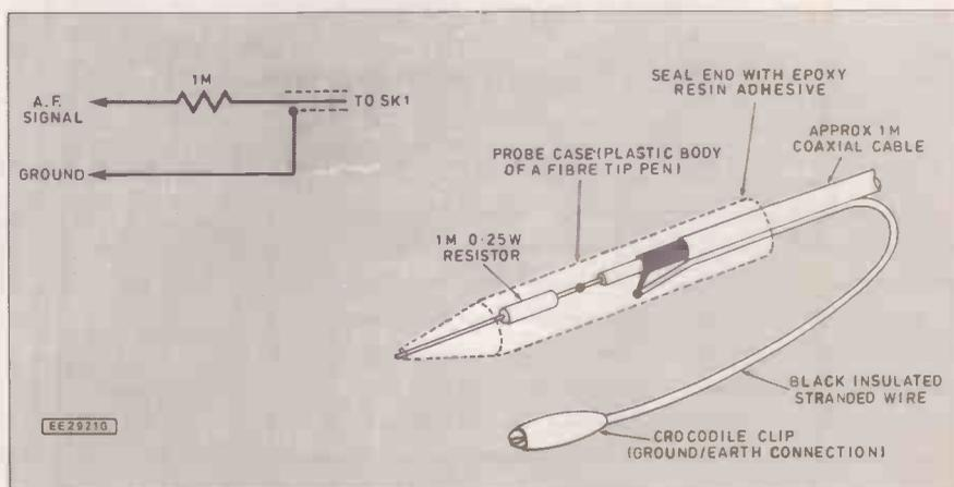
Fig.8. Input probe
