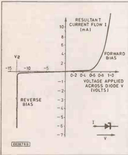
Fig. 2. Zener diode characteristics.
