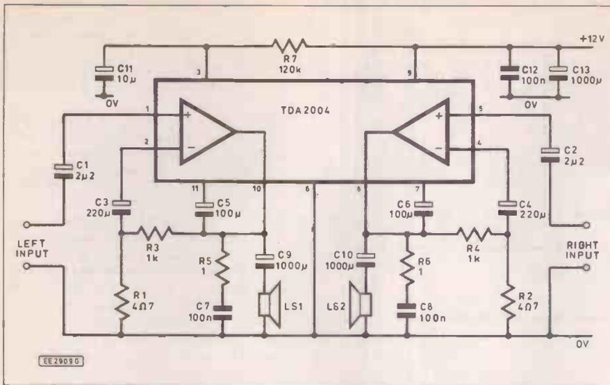
Fig. 3.18 TDA2004 stereo power amplifier
