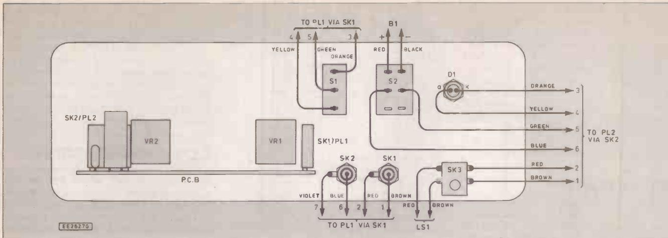
Fig. 5. Internal wiring of the Bench Amplifier/Signal Tracer
