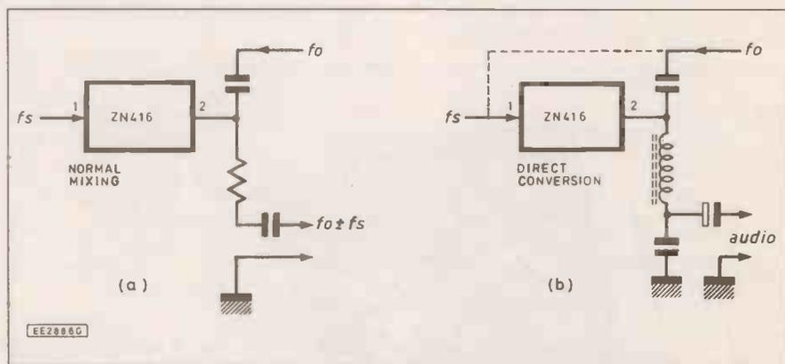
Fig. 2. Using the ZN416 detector as a high level mixer. (a) Normal mixing and (b) direct conversion.
