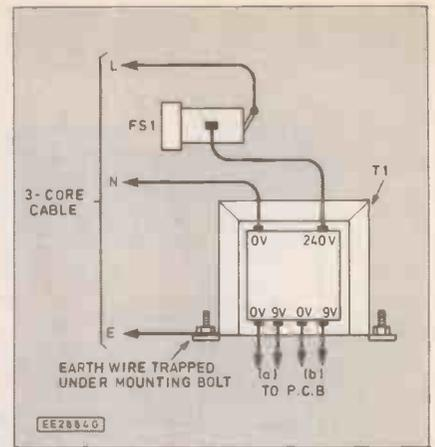
Fig. 5. Wiring details for the mains transformer T1.
