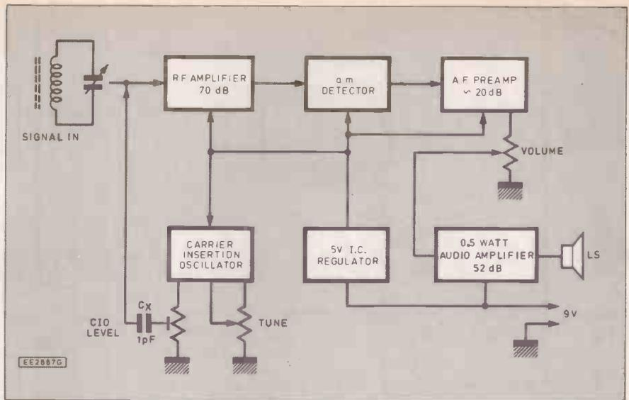
Fig. 3. Block diagram of the Gingernut receiver showing the major functional elements.
