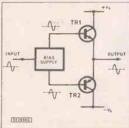
Fig. 3.6 Complementary output stage based on conventional bipolar transistors
