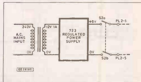
Fig. 6. Modifications for mains operation
