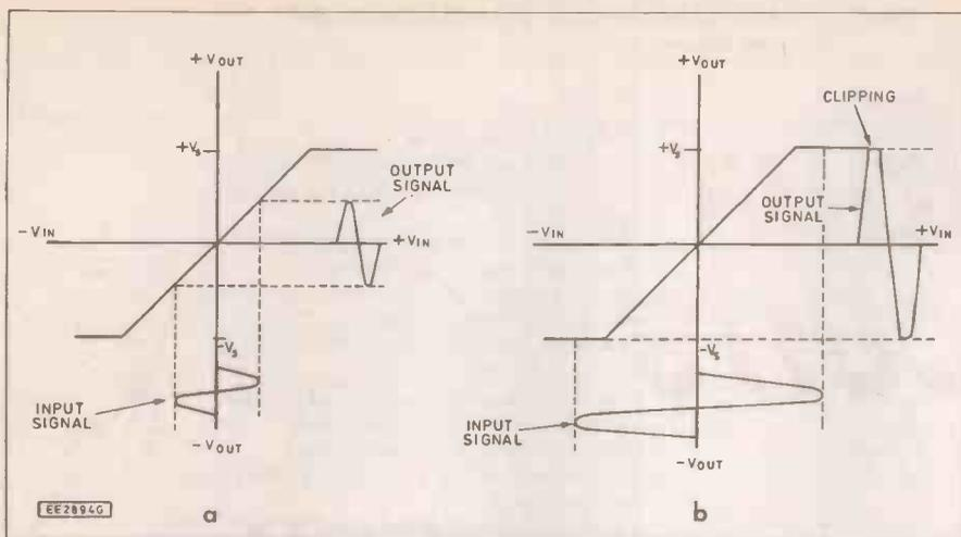
Fig. 3.2(a) Effect of Fig. 3.1 on a sinusoidal input signal of moderate amplitude
