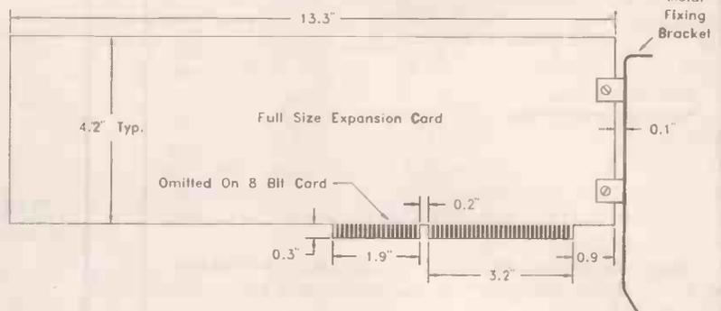
Fig. 2. Basic mechanical details of a full length PC expansion card.
