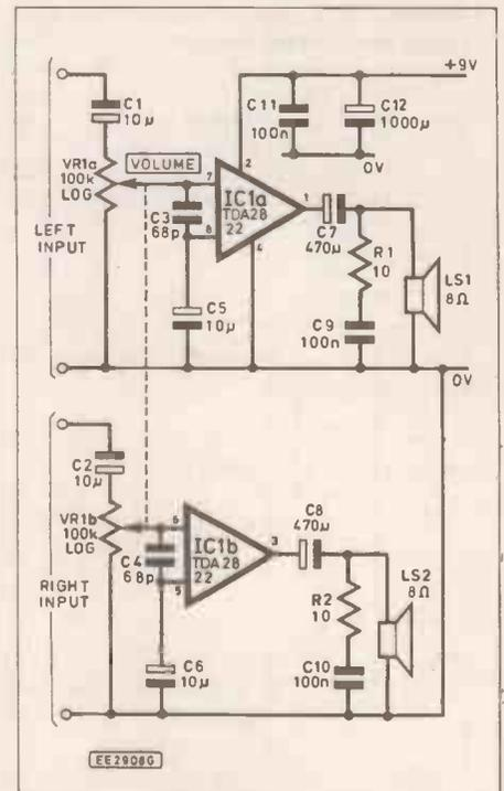
Fig. 3.17 Simple stereo amplifier based on the TDA2822
