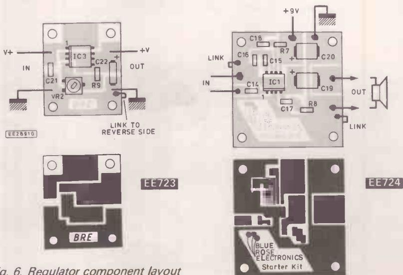
Fig. 6. Regulator component layout and master pattern.
