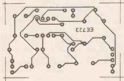
Fig. 3.16 P.C.B. layout for the TBA820M power amplifier module
