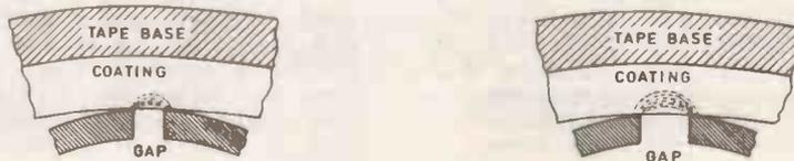
**Fig. 1.** A wide recording head gap produces a field that penetrates deeper into the tape coating than a narrow one because the radius of the field is proportional to it.
