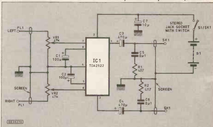
Fig. 1. Complete circuit diagram of the Camcorder Headphone Amplifier. The text refers to S1/SK1.
