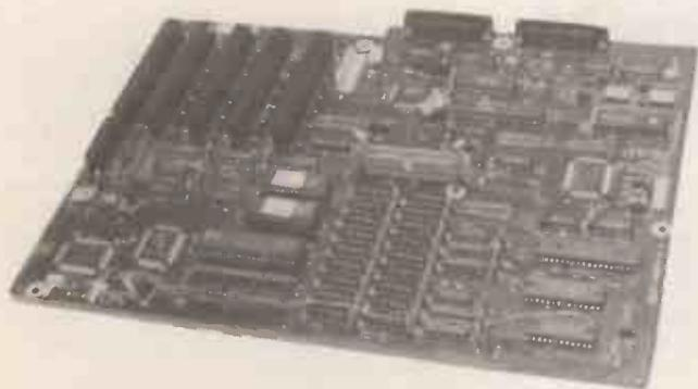
**A double-sided p.c.b. combining many dual-in-line (d.i.l.) and four surface-mounted (SM) devices. This is the main board of a Victor Personal Computer.**
