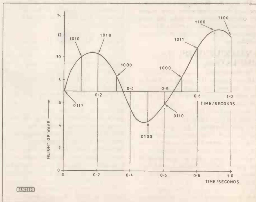
Fig. 5. Sampling the height of an analogue wave.
