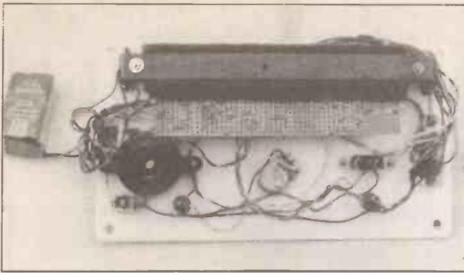
The buzzer and board mounted on rear of front panel.
