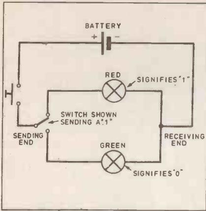
Fig. 6. Binary sending circuit.
