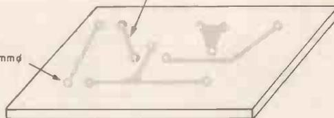
**Fig. 9.** After etching is completed, the resistant transfers are removed to expose the copper tracks underneath. Holes are drilled with a mini-drill to accommodate component leads and the completed p.c.b. can be protected with a coat of spray-on lacquer.
