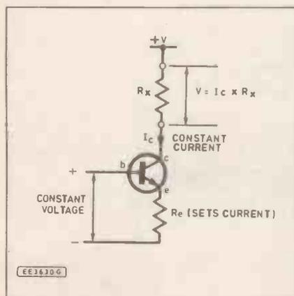
Fig.1 Basic principle of the linear scale ohmmeter.
