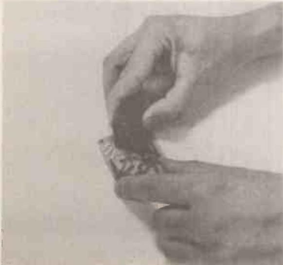
The etched board is rinsed with clean water and then the Alfac transfers can be removed with the cleaner block.
