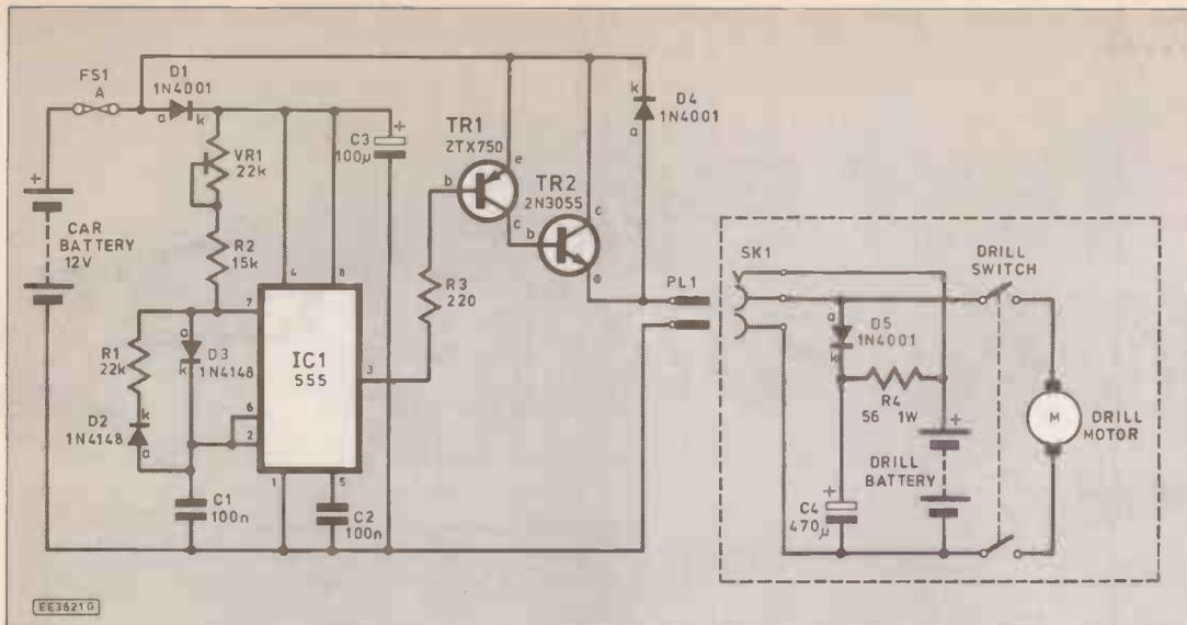
Fig. 1. Circuit diagram of the Cordless Drill Charger/PSU.
