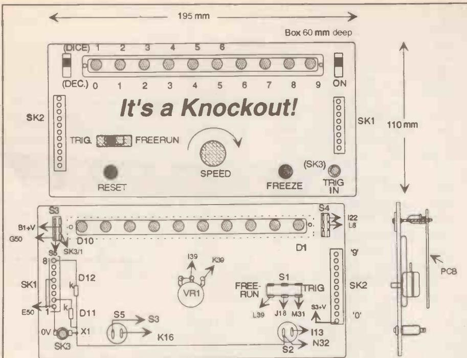
Fig. 3. Front panel layout and wiring from panel mounted components to circuit board. Letters and numbers are board grid references.
