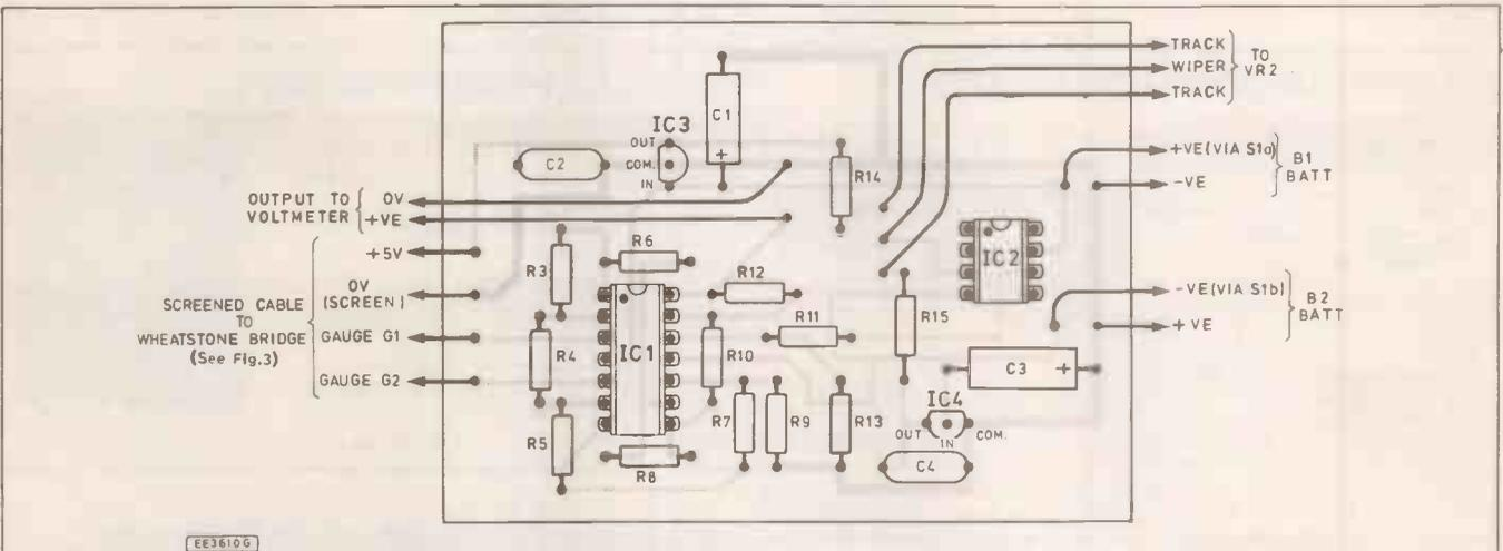
Fig. 4. Printed circuit board component layout, full size copper foil master pattern and photograph of the completed circuit board.
