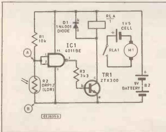
Fig. 1. Motor Control circuit.
