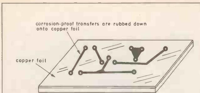
Fig. Fig. 6. Etch-resistant transfers are applied to the clean copper foil, in the desired layout of the copper track pattern. This is the "direct etch" and simplest method, of producing a p.c.b.
