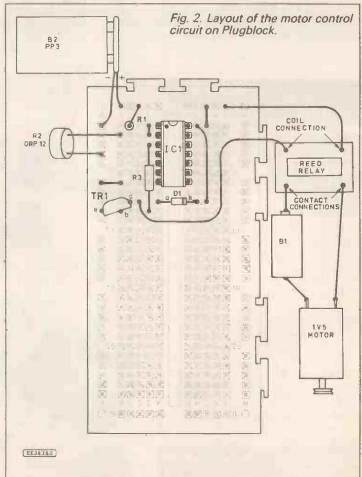
Fig. 2. Layout of the motor control circuit on Plugblock.
