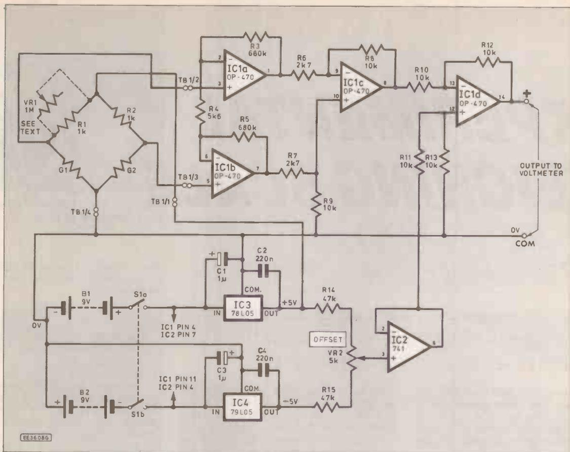
Fig. 2. Complete circuit diagram for the Experimental Weighing Scale. Preset VR1 may be needed to balance or "zero" the bridge.
