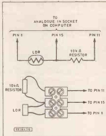
Fig. 8. L.D.R. circuit connected to a BBC Micro.
