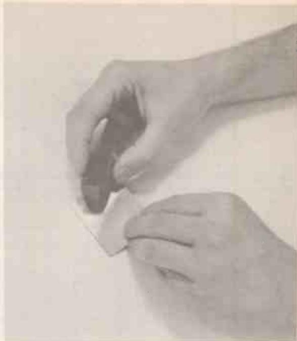
**Copper-clad board, cut to size, being cleaned with an abrasive cleaning block.**
