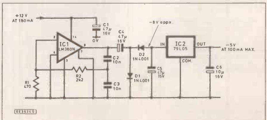
Fig.5 Complete -5V 100mA power supply based on an LM380.
