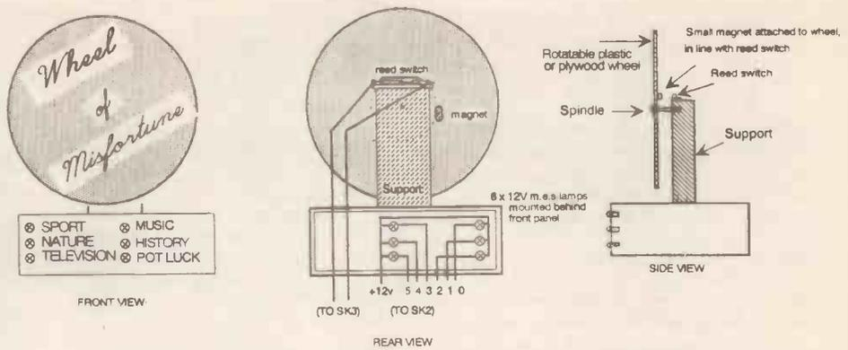
Fig. 6. Assembly and wiring to the Wheel of Misfortune display.
