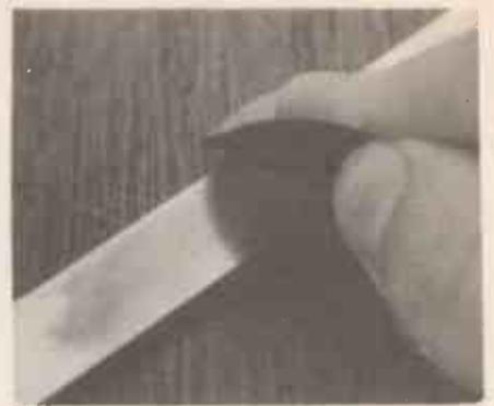
Photo 2 (above) – Using a wet/dry paper disc to abrade the metal strip.
