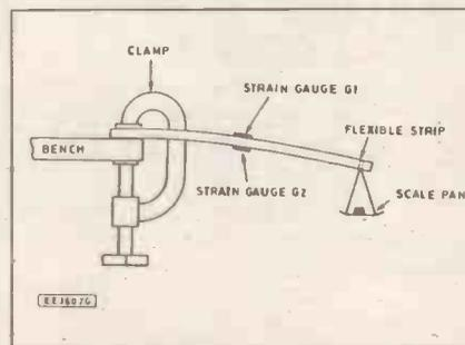
Fig. 1. Experimental "cantilever" type Load Cell set up.
