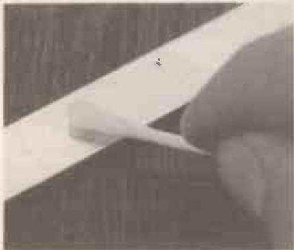
Photo 3 – Cleaning the surface with weak detergent and a "cotton bud".
