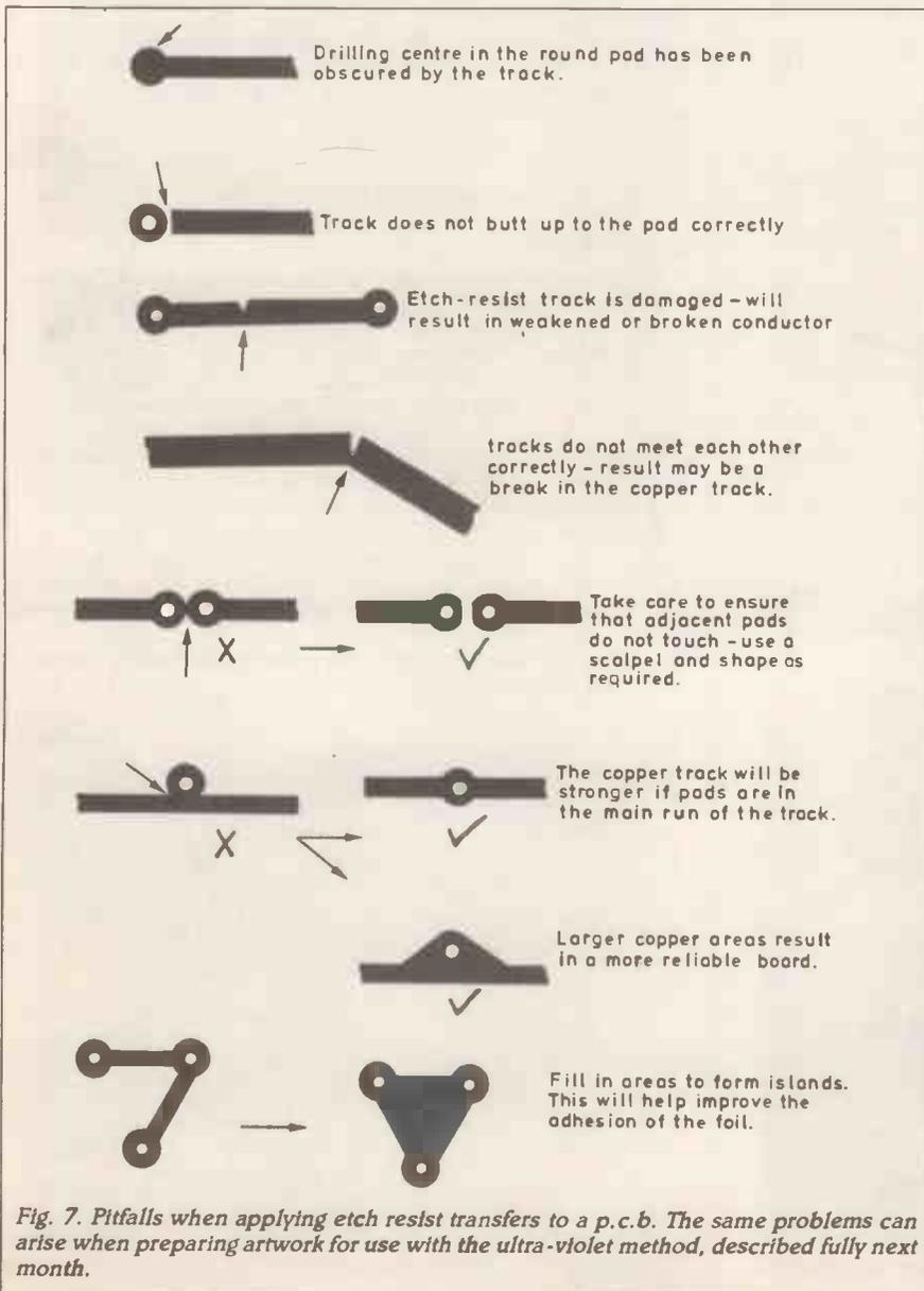
Fig. 7. Pitfalls when applying etch resist transfers to a p.c.b. The same problems can arise when preparing artwork for use with the ultra-violet method, described fully next month.
