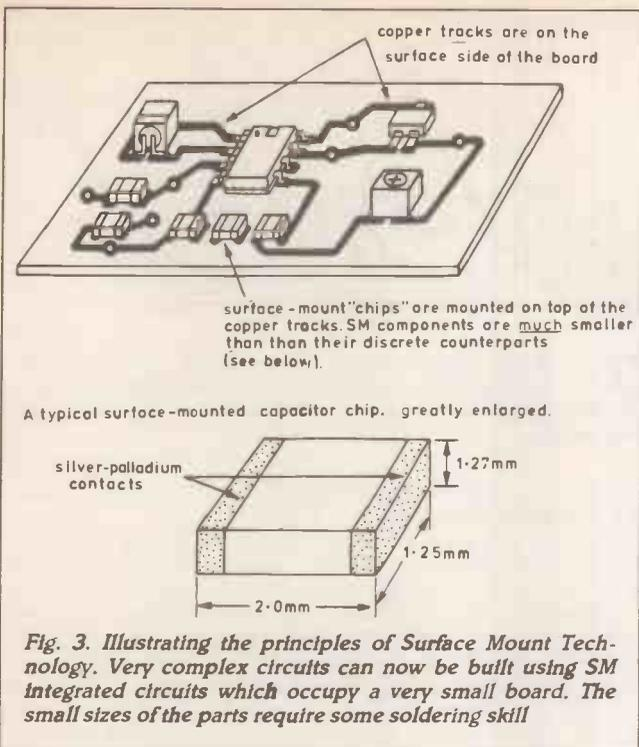
**Fig. 3. Illustrating the principles of Surface Mount Technology. Very complex circuits can now be built using SM Integrated circuits which occupy a very small board. The small sizes of the parts require some soldering skill**
