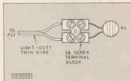
Fig. 4. Suggested method of mounting the thermistor inside a small box using a two-way terminal block.
