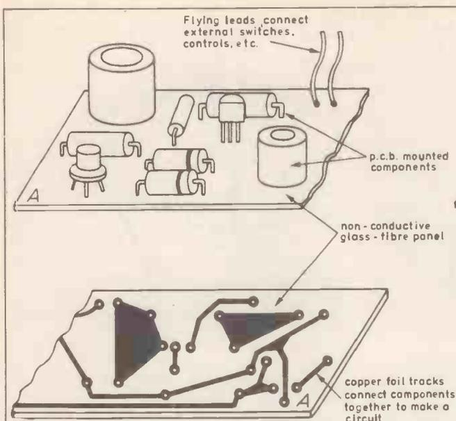
**Fig. 1. Single-sided printed circuit board where the copper tracks are all on one side of the board. The components are soldered to the copper pads to form a complete circuit.**
