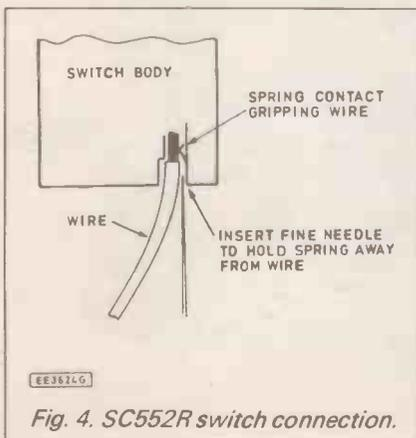
Fig. 4. SC522R switch connection.
