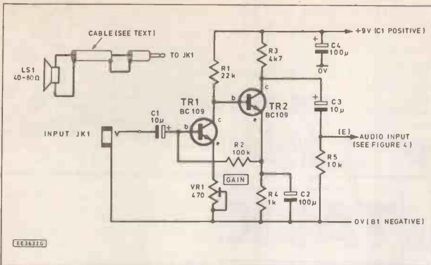
Fig.3 Additional pre-amplifier for use with the EE Telesound in order to provide "baby listening" facilities.
