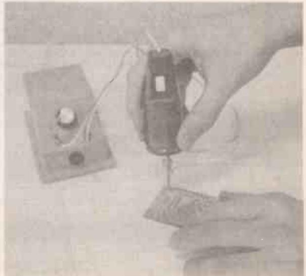
Drilling the board with a low-voltage mini drill; note the mains adaptor.
