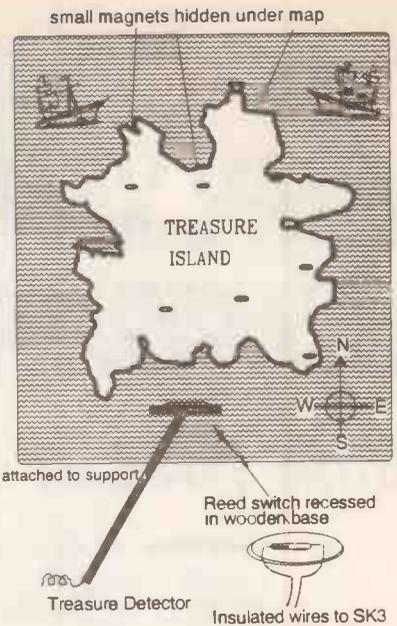
Fig. 8. Buried Treasure map layout and detector head.
