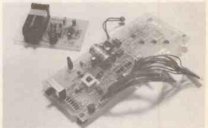
**(Left) Typical single-sided printed circuit board – note the p.c.b.-mounted battery holder. (Right) A double-sided p.c.b. – the copper tracks on the upper side and the through-pins can clearly be seen.**
