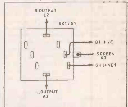
Fig. 3. Wiring of SK1/S2.
