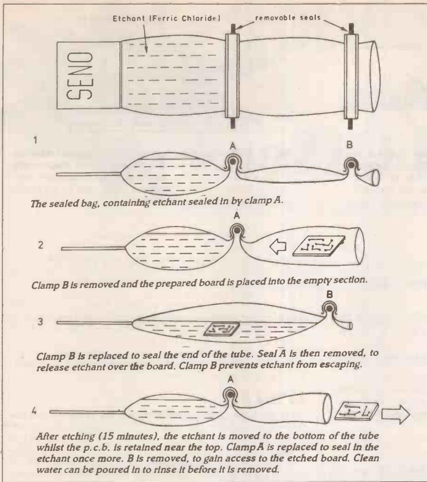
With use the Ferric Chloride solution will eventually become laden with iron, slowing down the etching time and when the etchant has finally been exhausted, a neutralising powder (supplied) is added to the solution which is eventually transformed into a solid mass for safe disposal.
