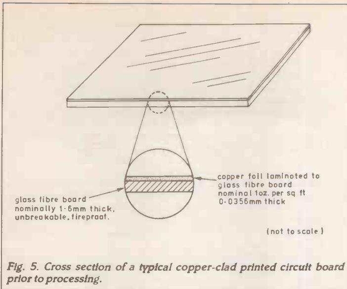
**Fig. 5. Cross section of a typical copper-clad printed circuit board prior to processing.**
