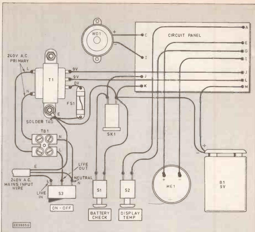
Fig. 3. Interwiring from the circuit board to the case mounted components. Mains 3A wire should be used for connecting the illuminated On/Off switch to the screw terminal block TB1. The completed unit, with cover removed, is shown in the photograph below. The thermistor is housed separately in a small plastic box.
