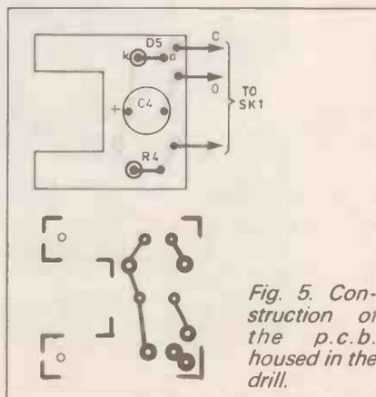
Fig. 5. Construction of the p.c.b. housed in the drill.
