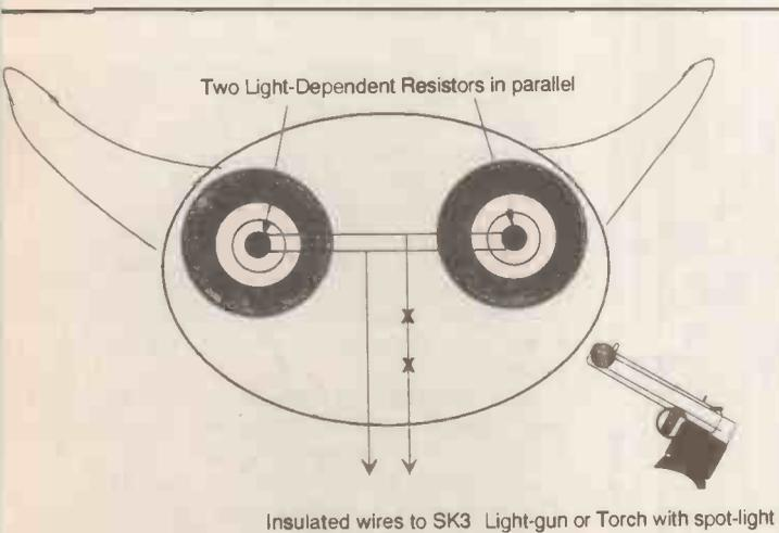
Fig. 7. Wiring to the two LDR "eyes" of the Bull's Eyes display. If ambient light causes premature triggering, insert a 5k potentiometer (wiper and one outer tag) at points "X".
