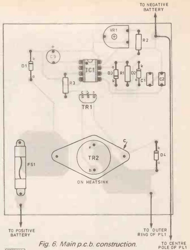
Fig. 6. Main p.c.b. construction.
