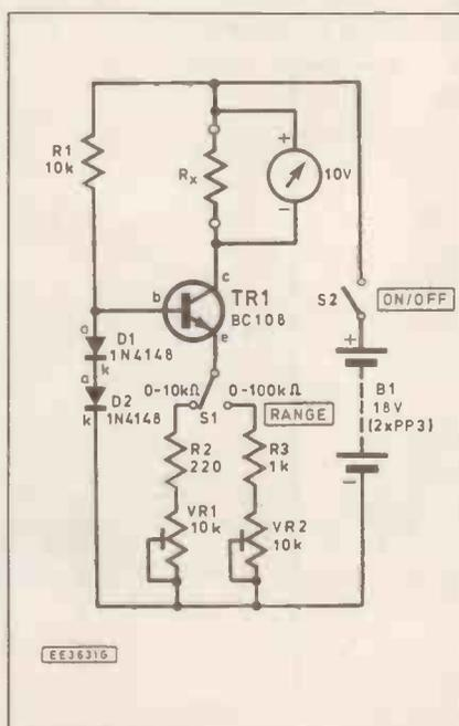
Fig.2 Complete circuit of the linear scale ohmmeter.
