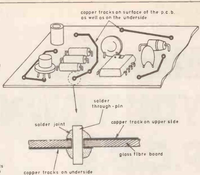
**Fig. 2. Double-sided p.c.b. where some copper tracks are placed on the surface of the board, and are connected to the main track pattern underneath by using through-pins.**
