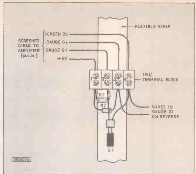
Fig. 3. Using a 4-way terminal block (TB1) to make up the Wheatstone bridge. This is connected to the p.c.b. using multi-cored screened cable.
