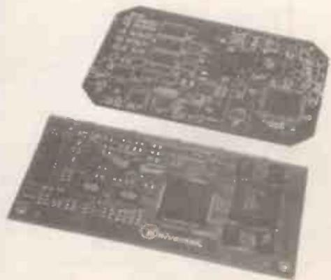
**(Below) A surface-mounted p.c.b. – note the flat-pack SM integrated circuits and the tiny capacitor and resistor “chips”. (Above) A commercial 4-level multi-layer p.c.b. prior to fitting with components. The darker tracks which can just be seen are actually within the board itself.**
