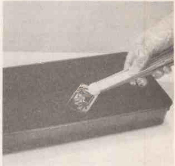
Removing the p.c.b. from the etching solution. Gloves and goggles are sensible precautions.
