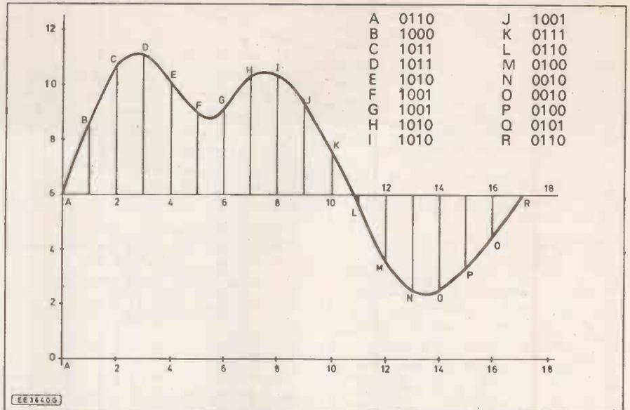
Fig. 7a. Master wave and the representative binary numbers.
