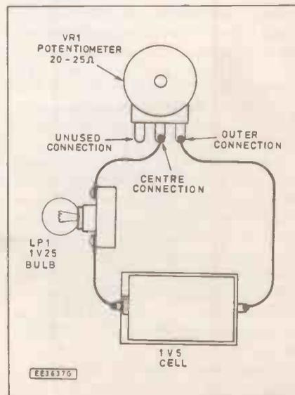
Fig. 3. Practical layout for the analogue circuit.
