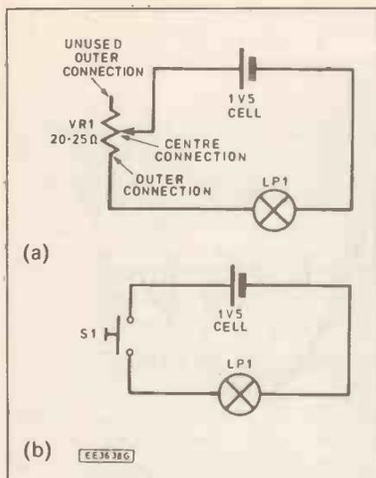
Fig. 4. Analogue (a) and digital (b) circuits.
