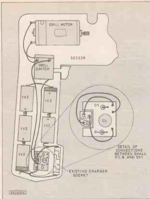
Fig. 3. Modification to the SC522R drill.
