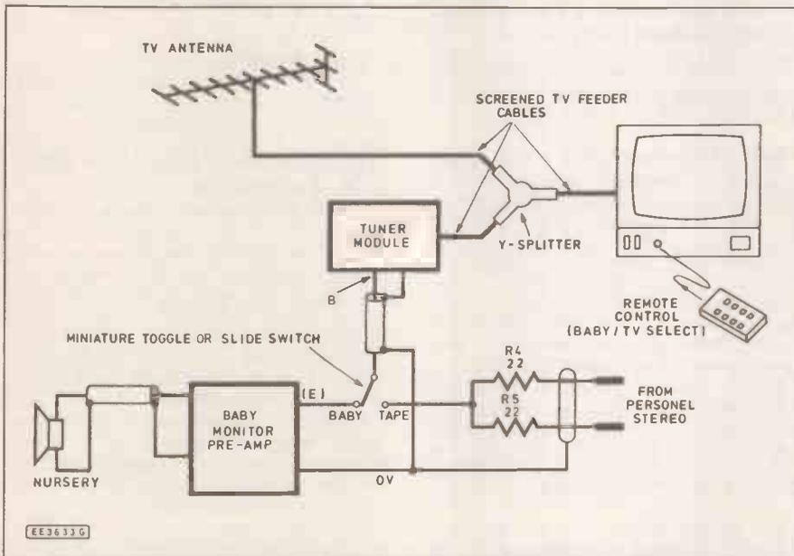
Fig.4 Method of connecting the EE Telesound to provide switching between TV programmes and baby listening.
