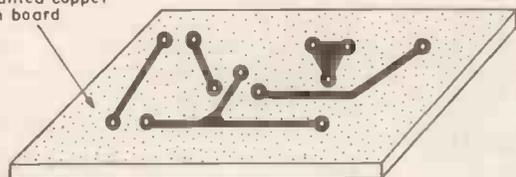
**Fig. 8.** The board, with etch-resist transfers applied, is placed into a corrosive liquid (Ferric Chloride) which removes all the copper except that protected by the resist. Notice the layer of copper foil has disappeared from the cross-sectional view (compare against (Fig. 6).
