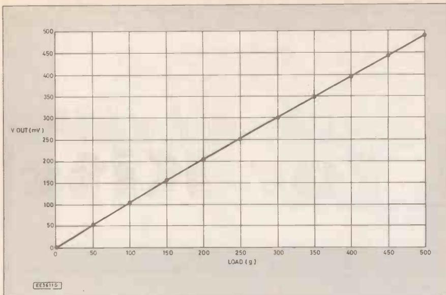
Fig. 5. Typical calibration graph. This is produced by hanging a series of known masses on the Load Cell and recording the output voltage in each case
