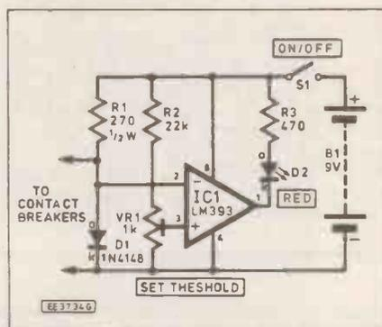
Fig. 2 Simple instrument for sensing the state of the contact breakers
