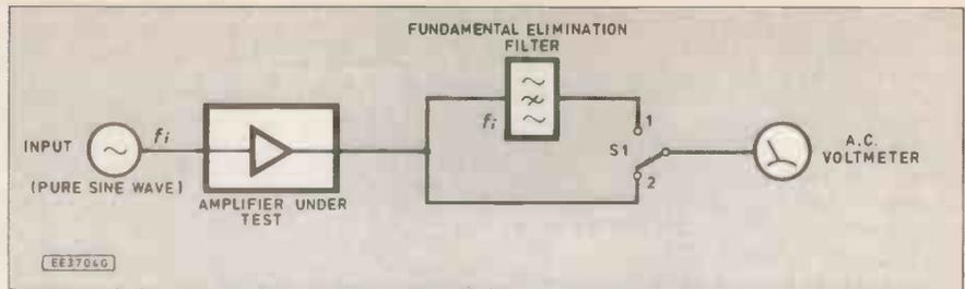
Fig. 1. Distortion factor measurement setup.
