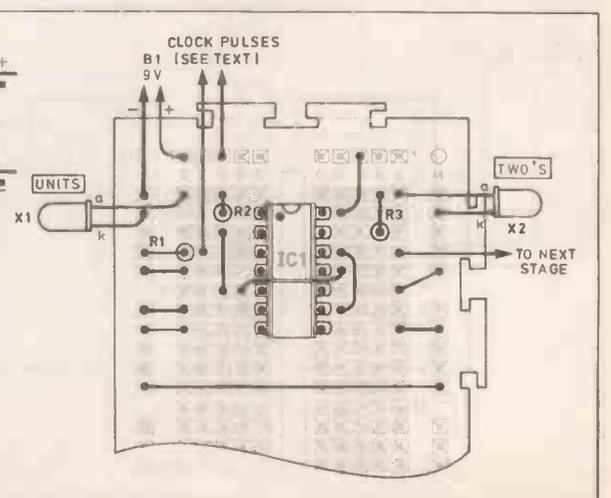
Fig. 17. (right) 2-bit binary counter construction.
