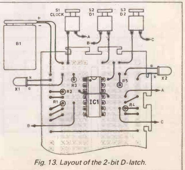
Fig. 13. Layout of the 2-bit D-latch.
