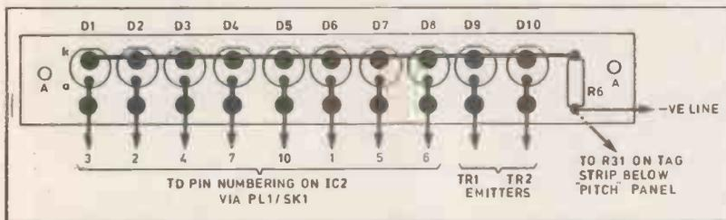
Fig. 4. Using a small board to wire the wicket l.e.d.s. This board could be made from stripboard.
