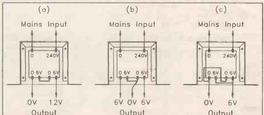
Fig. 1. Methods of connecting twin secondary windings (a) in series (b) pseudo-centre tap (c) parallel.
