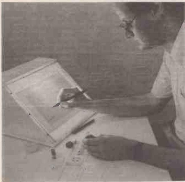
Photo 1. Designing your own artwork starts by drafting a rough component layout diagram, referring to the circuit diagram and manufacturer's data as required. Here, the EE Light Box (next month) is being used, which proves invaluable in the following stages.
