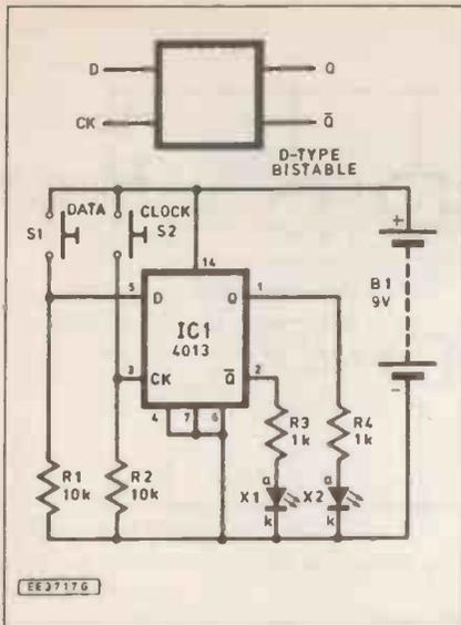
Fig. 10. D-type bistable symbol and a practical circuit.
