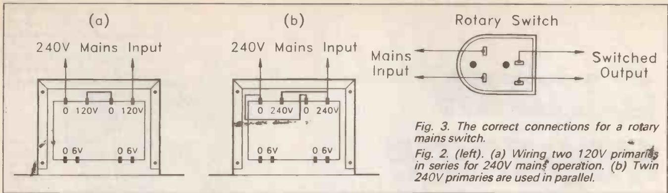
Fig. 3. The correct connections for a rotary mains switch.
