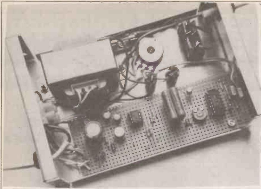
The complete circuit board mounted inside the metal case. The metal case must be "Earthed" through the mains lead, see Fig. 3.
