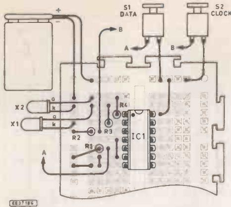
Fig. 11. D-type bistable construction.
