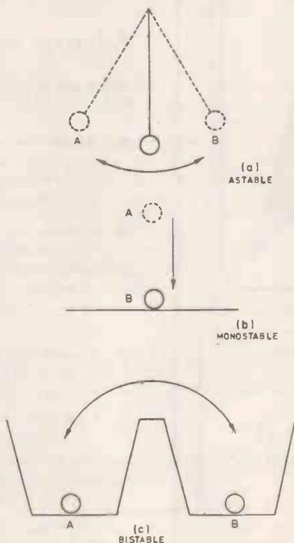
Fig. 1. Mechanical models of the multivibrator family.
