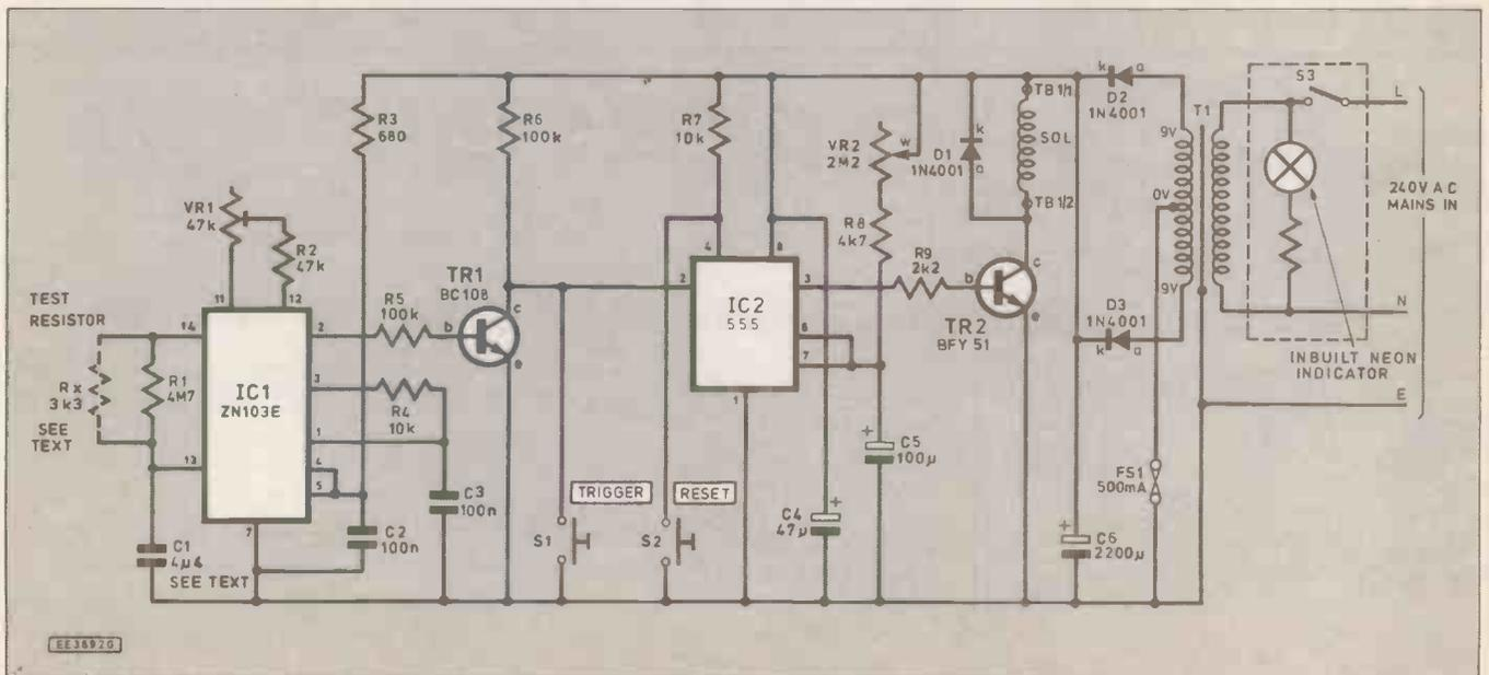
and pin 3, change state – pin 2 going from low to high and pin 3 from high to low. With the values of C1 and R1 specified, the time taken to do this is nominally 24 hours. Preset potentiometer VR1, in conjunction with fixed resistor R2 connected between IC1 pins 11 and 12, provide an adjustment which will be used to trim the timing period for best accuracy at the end of construction.
