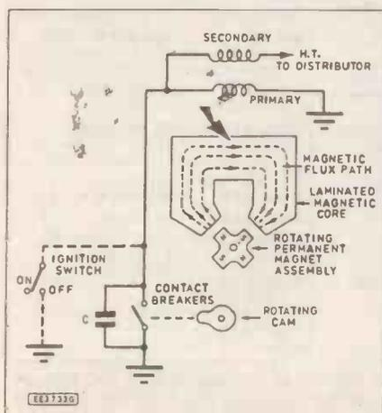
Fig. 1 Basic magneto arrangement (note that the transformer windings are wound on the laminated steel core)
