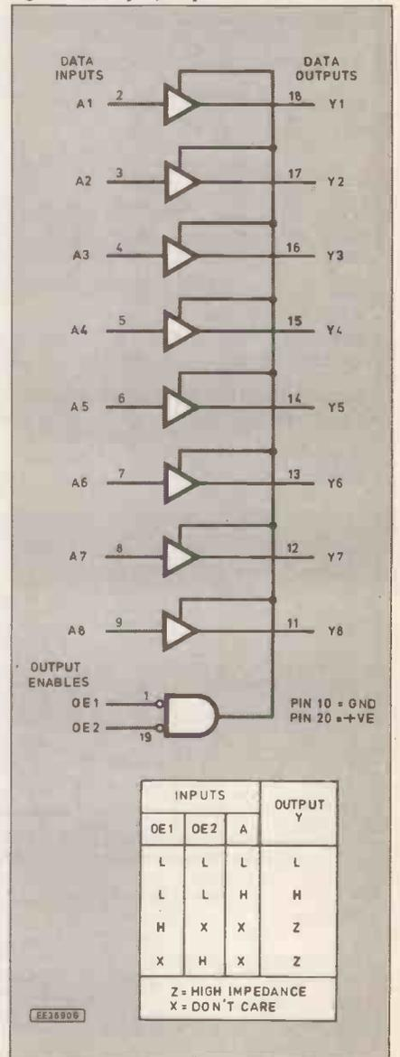
Fig. 3. Functional logic diagram and truth table for the 74C541.
