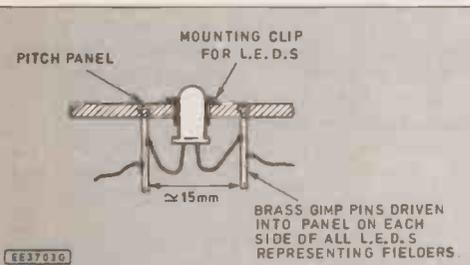
Fig. 6. How the "fielders" are mounted and wired on the pitch panel.
