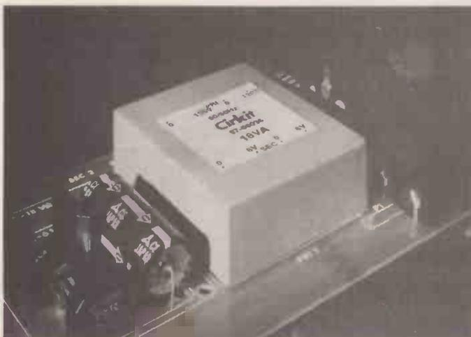
Wound on twin double section bobbins to provide maximum isolation - 4kV - between windings and near toroidal characteristics.
