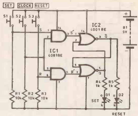
Fig. 8. Clocked S-R bistable.
