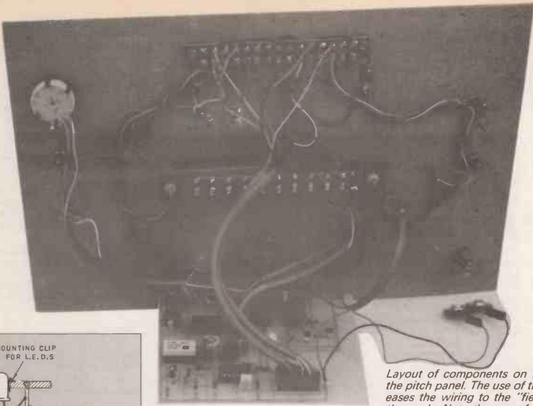
Layout of components on the rear of the pitch panel. The use of the tag strip eases the wiring to the "fielders" and the p.c.b. Note the use of the header connections on the p.c.b.
