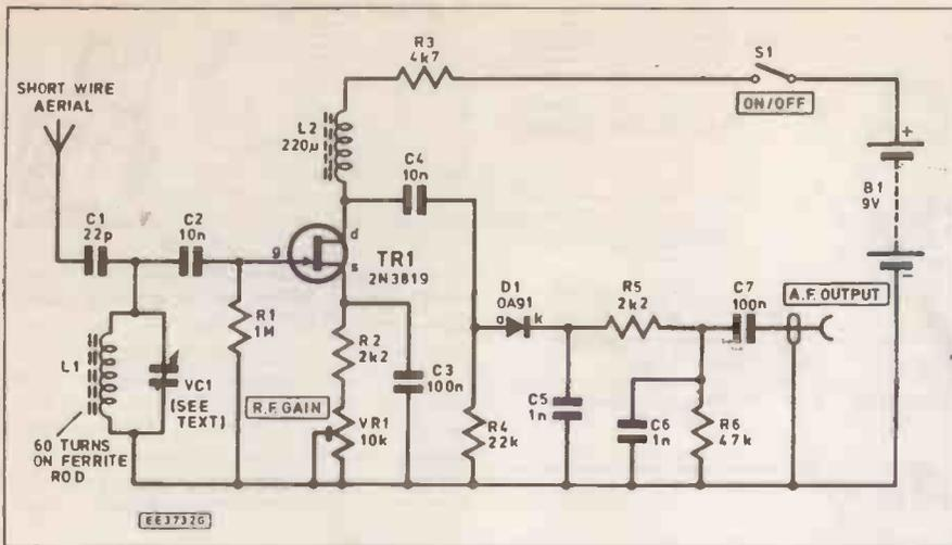
Fig. 4 Circuit of the simple a.m. tuner
