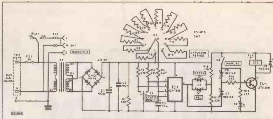
The circuit diagram of the UV Exposure Timer which is used here to demonstrate the approach taken in designing your own p.c.b. A photograph of the completed project is also shown.
