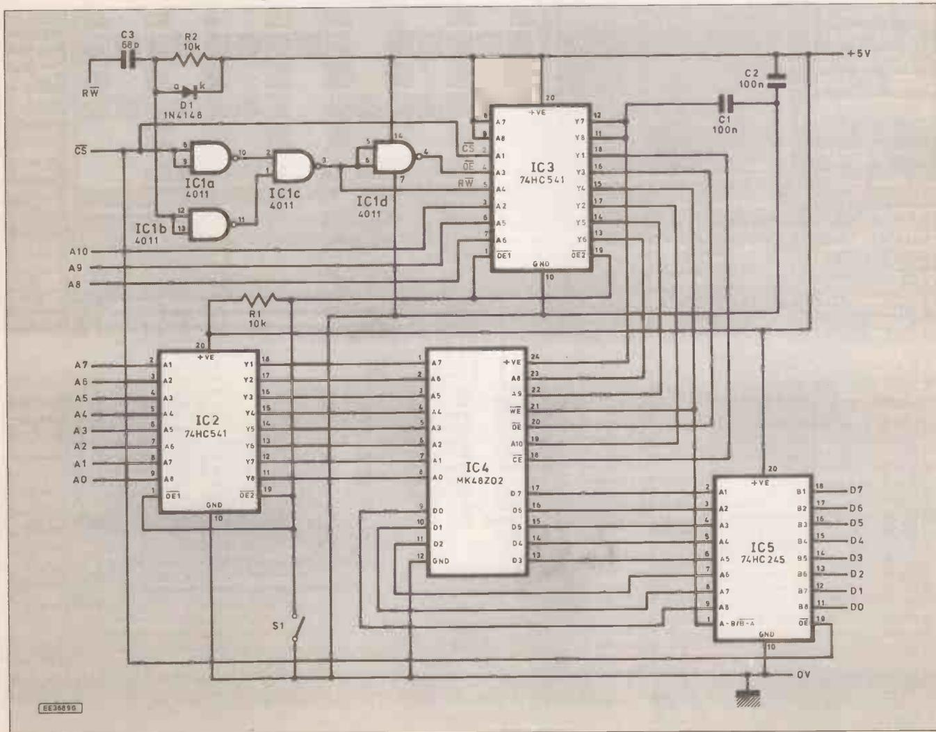
lines must both be low. When reading from the SRAM,  $\overline{CS}$  must again be low, but  $\overline{RW}$  must be high.
