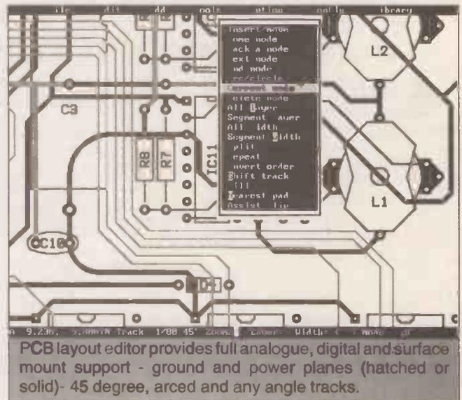
PCB layout editor provides full analogue, digital and surface mount support - ground and power planes (hatched or solid) - 45 degree, arced and any angle tracks.
