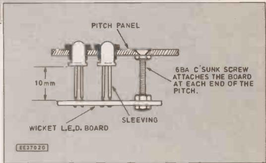
Fig. 5. How the l.e.d.s are mounted on the subsidiary "wicket" board and fixed to the pitch panel.
