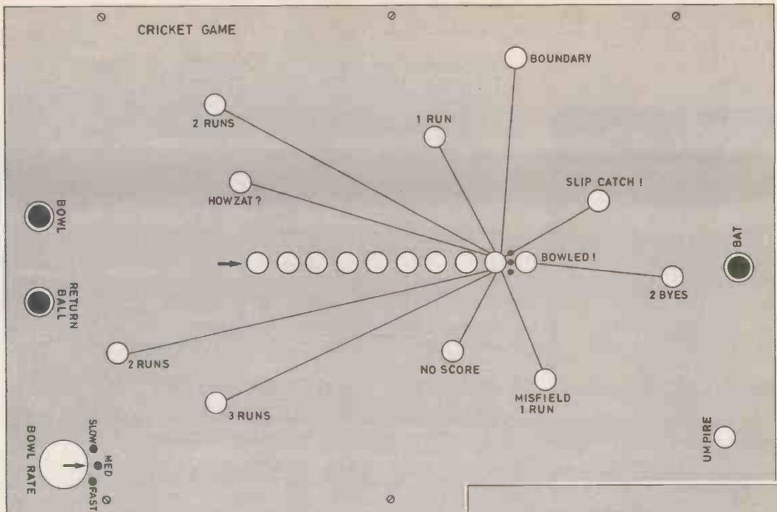
Fig. 3. Suggested field layout. The "wicket" l.e.d.s are spaced 10mm apart.
