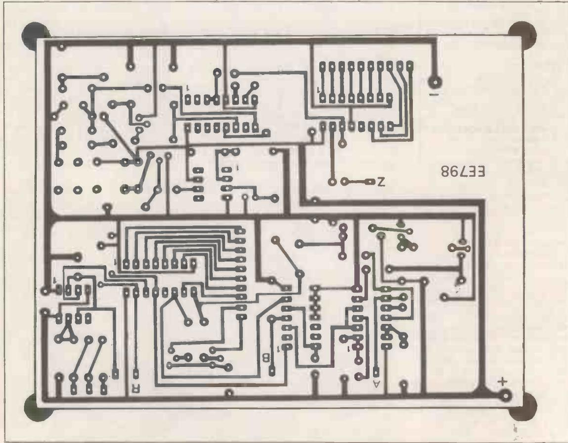
Fig. 2. Printed circuit board component layout and full size copper foil master pattern for the Cricket Game.
