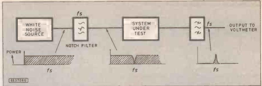
Fig. 5. Intermodulation measurement by "noise in slot" method.
