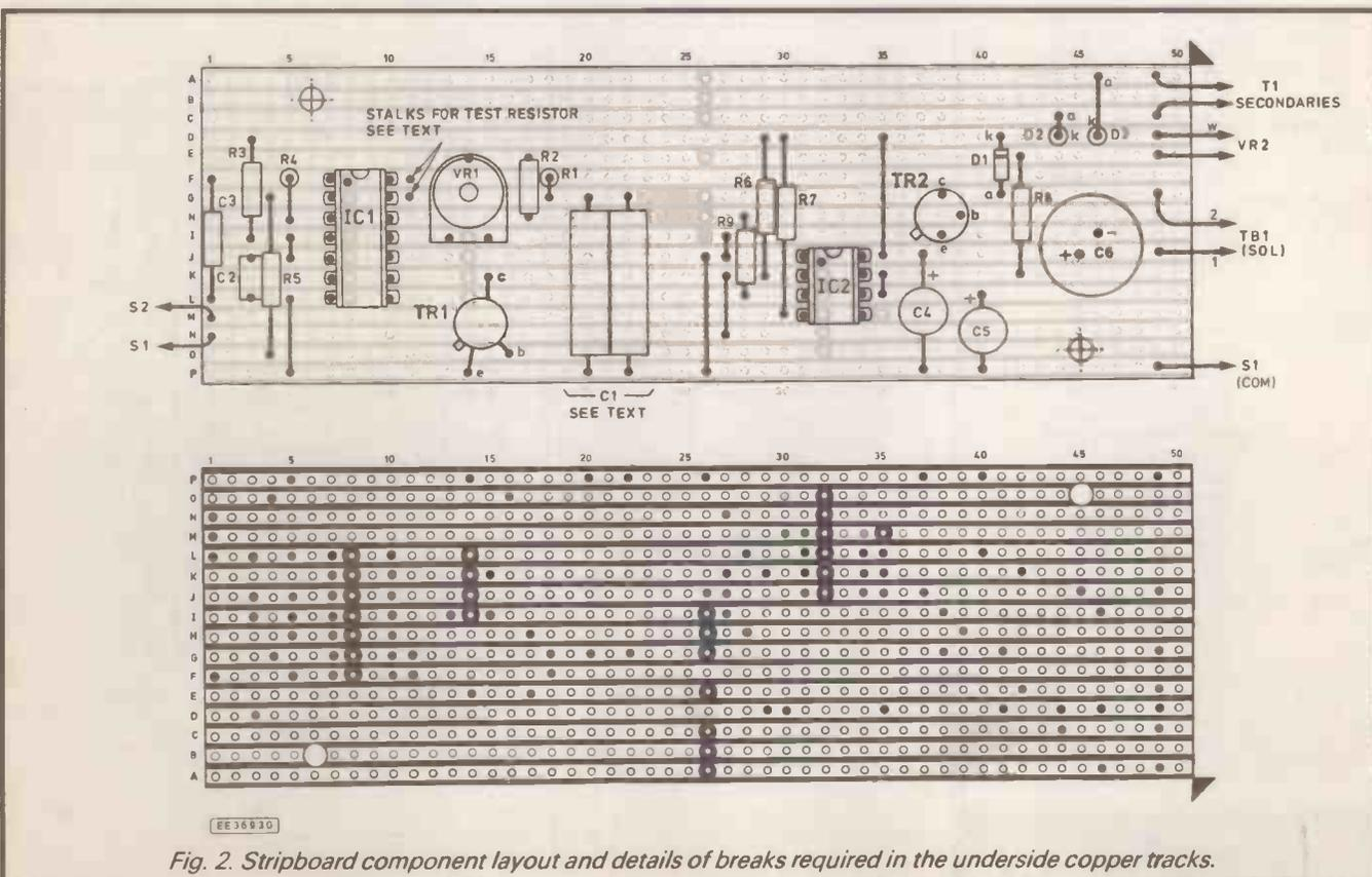
Fig. 2. Stripboard component layout and details of breaks required in the underside copper tracks.
