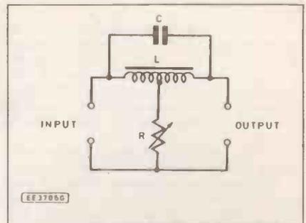
Fig. 3. Bridged-T trap.
