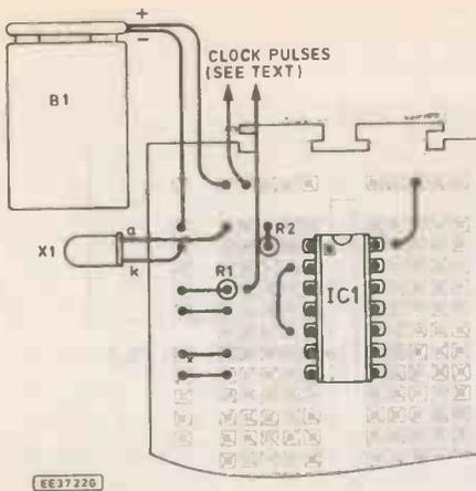
Fig. 15. Construction of the toggling circuit.
