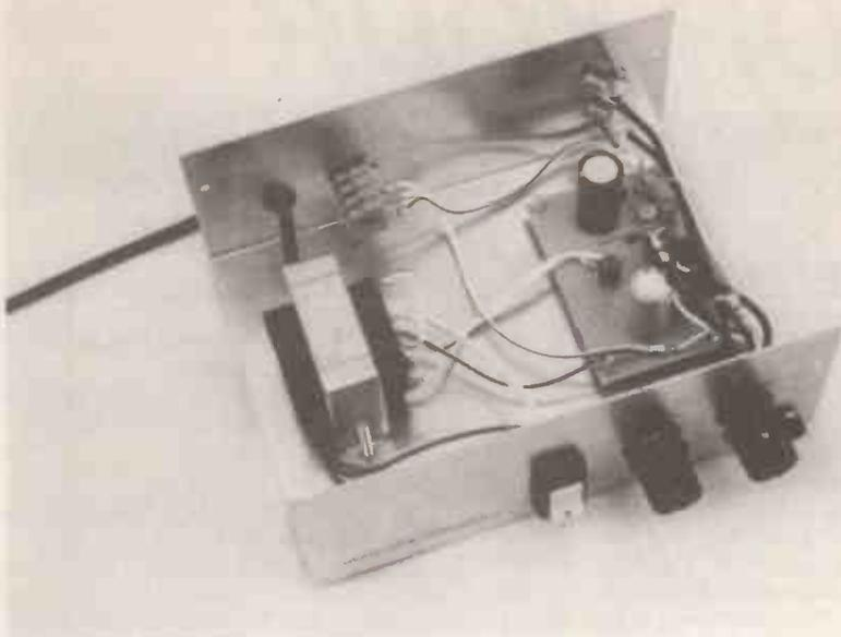
case is shown in Fig. 3. As you can see it's quite simple due to the fact that only the controls, input/output sockets, transformer and board mounting holes are required. The main point to note here is that the mains entry hole needs to be fitted with a 10mm cable clamping grommet.
