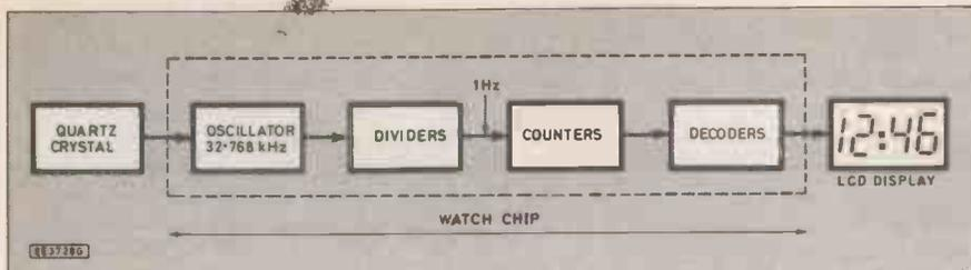
The working parts of a digital watch.
