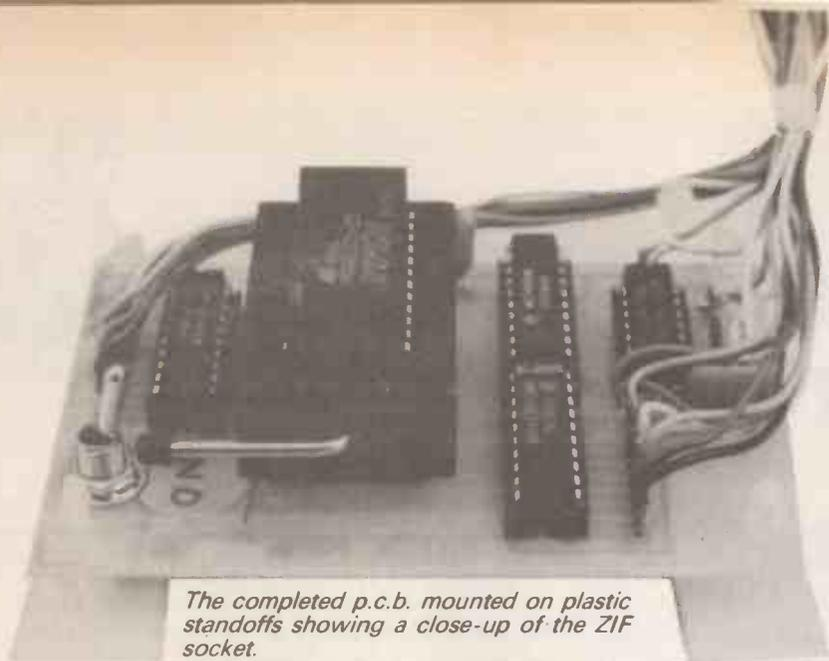
The completed p.c.b. mounted on plastic standoffs showing a close-up of the ZIF socket.
