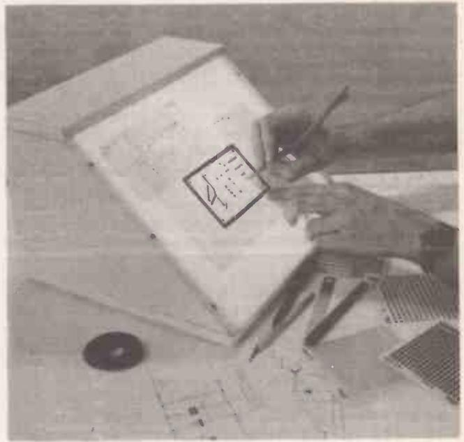
Photo 2. Starting to prepare the master artwork using Alfac rub-down transfers. Also on the Light Box is the author's rough draft - the proposed copper track layout shows through the paper so that an "X-Ray" view of the rough version is seen.
