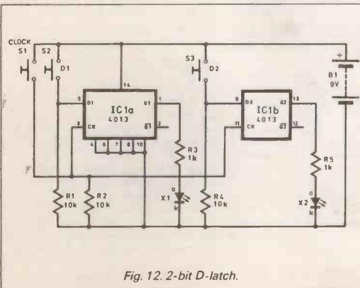
Fig. 12. 2-bit D-latch.
