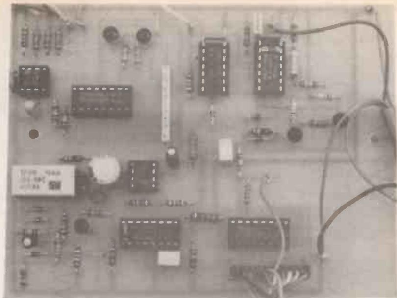
turning transistor TR5 on and operating the relay which closes RLA1 contacts. This closure is only momentary because of the differentiating action of the coupling components capacitor C6 and resistor R21, and the rest of the circuit is then activated in the way already explained.
