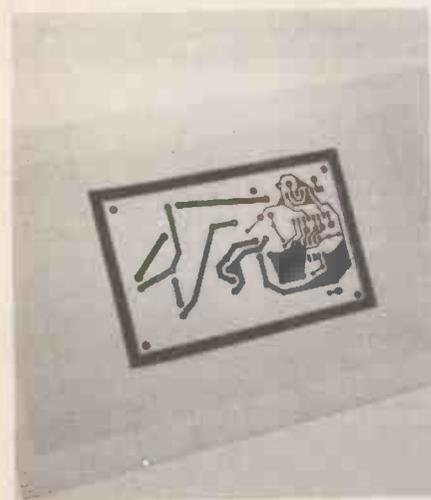
*Photo 3. The completed artwork on the light box - the precision 0.1in. matrix grid is also visible. This view is actually equivalent to seeing the copper track pattern "through" the board from the component side.*
