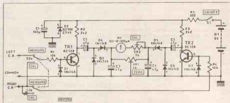
Fig. 3 Circuit of the experimental pulse comparator
