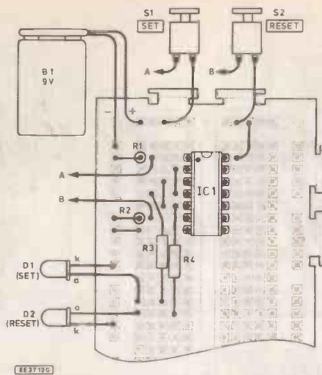
Fig. 5. Practical S-R bistable construction.
