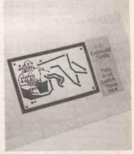
*Photo 5. The artwork is turned over and clearly labelled "Copper Track View Side" - this is your first sight of the actual copper foil pattern which will be etched into your p.c.b.!*
