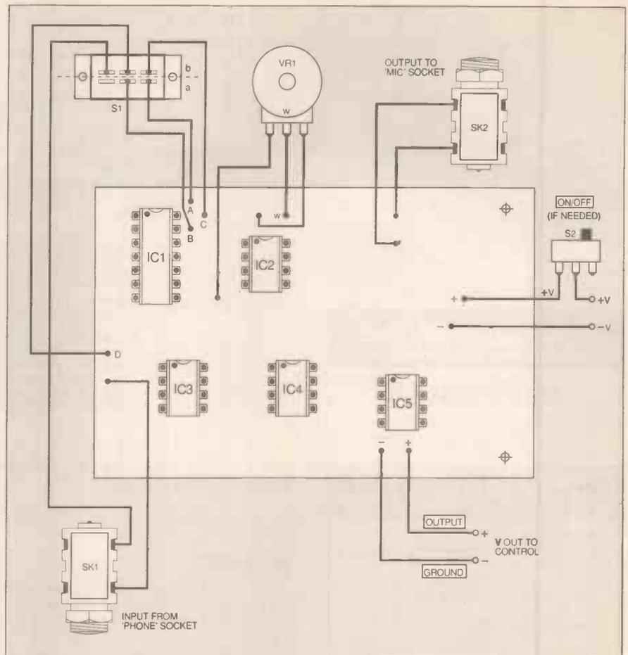
Fig. 4. Interwiring from the printed circuit board to off-board components.
