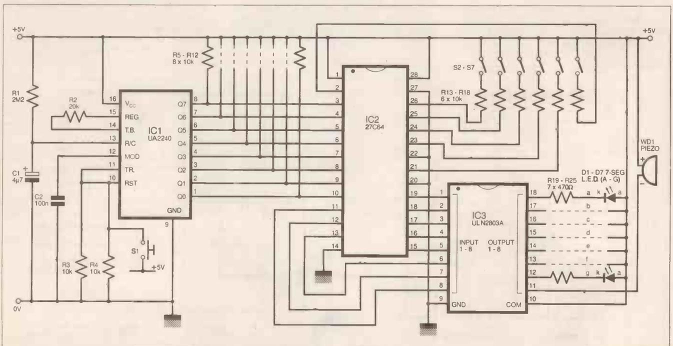
Fig. 4. Circuit diagram for a Programmable Timer/Sequencer.
