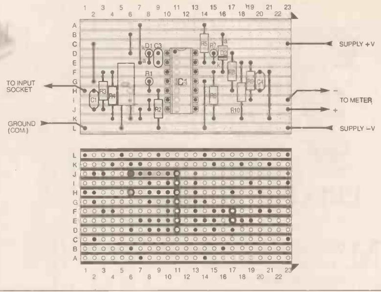
Fig. 6. Signal Level stripboard component layout and details of underside breaks required in copper tracks.
