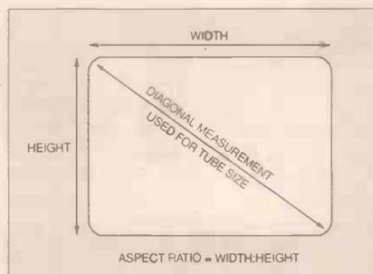
Fig. 23. Aspect ratio and size.
