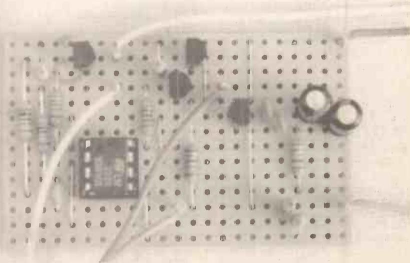
Layout of components on the Loop Interface stripboard.
