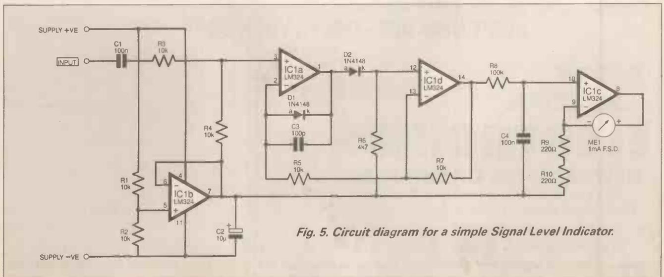
Fig. 5. Circuit diagram for a simple Signal Level Indicator.
