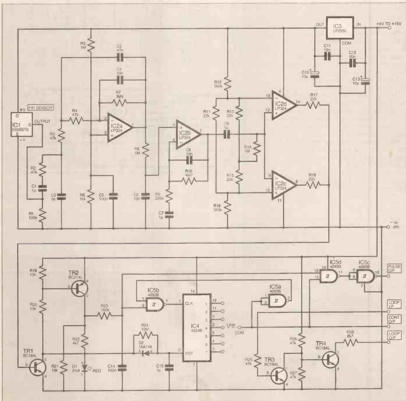
Fig. 1. Complete circuit diagram for the pulse-counting Versatile PIR Detector Alarm.
