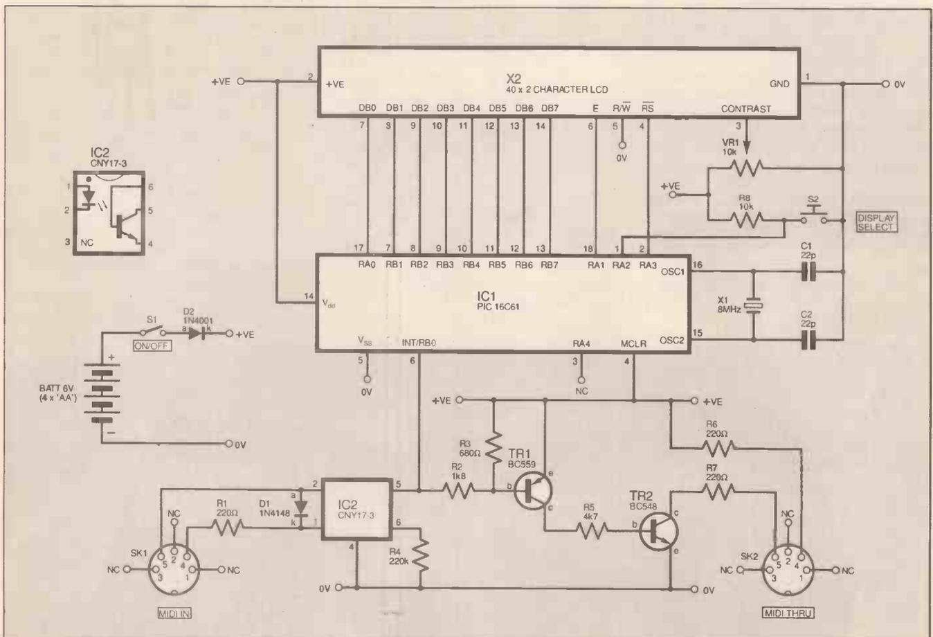
Fig. 4. Complete circuit diagram for the MIDI Analyser. Note that switch S2 is a push-to-make and release-to-break type.
