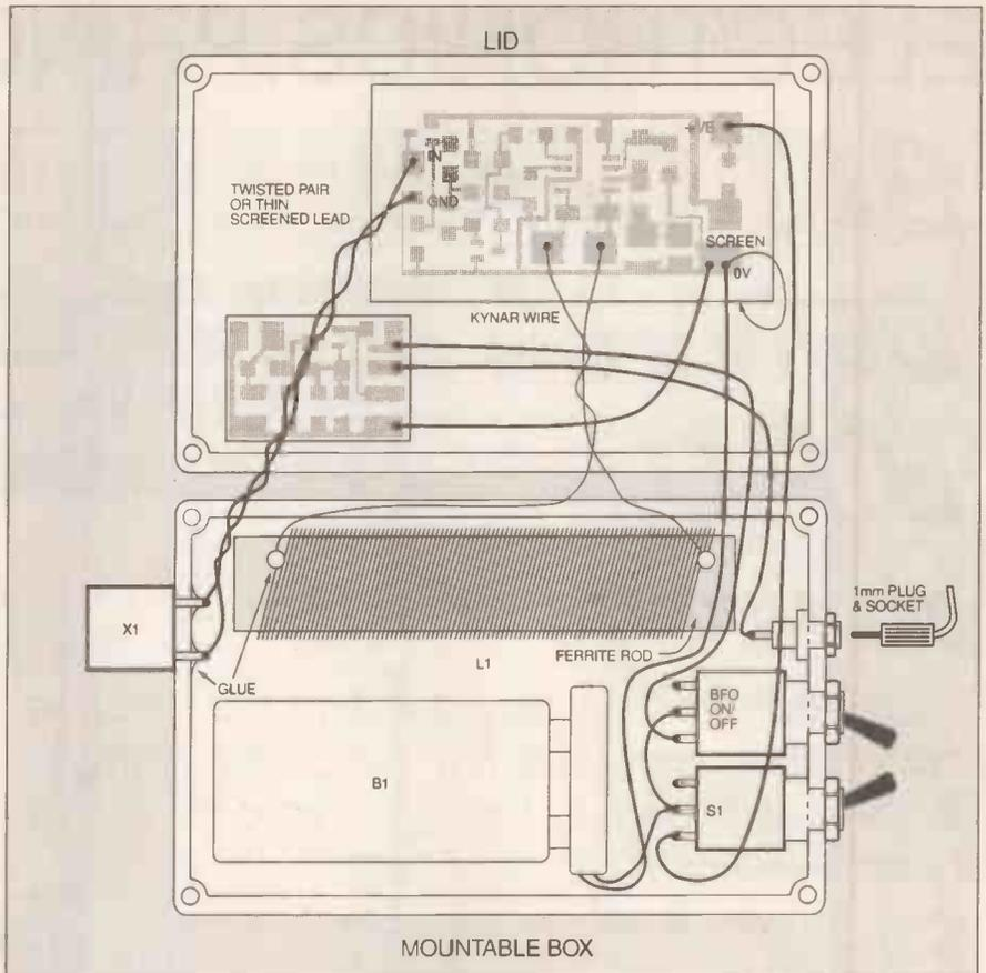
Fig. 3. Wiring the B.F.O. board, additional switch and output socket into last month's small Bat Band Converter case.
