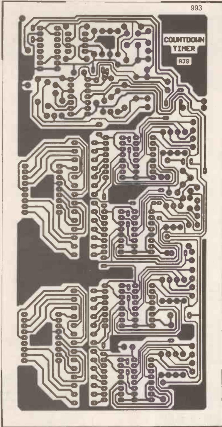
Fig. 6. Full-size underside copper foil track master pattern.
