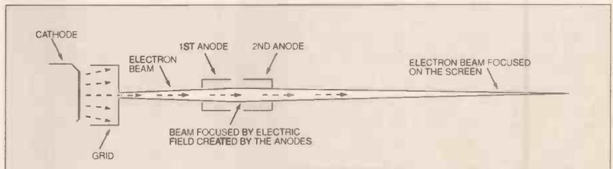
Fig. 19. Anodes in the electron gun.
