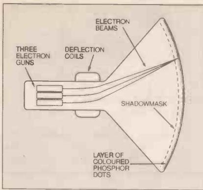
Fig. 25. Construction of a colour tube.
