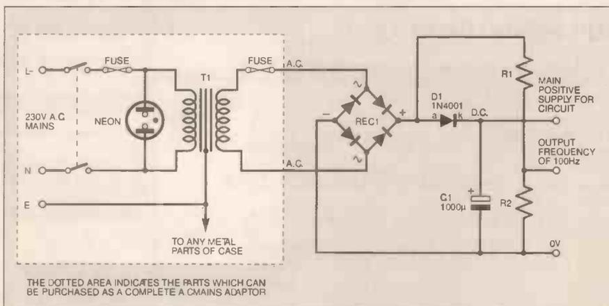
Fig. 7.1. Deriving a 100Hz signal from an a.c. power supply. Typical values for R1 and R2 would be: 10k and 47k respectively.
