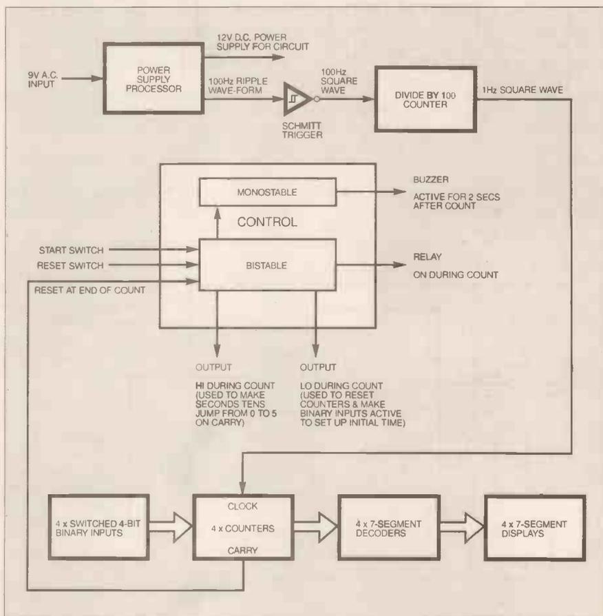
Fig. 1. Block diagram for the Countdown Timer. The relay is optional.
