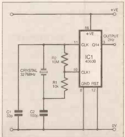
Fig. 7.5. Combined crystal oscillator and counter circuit.
