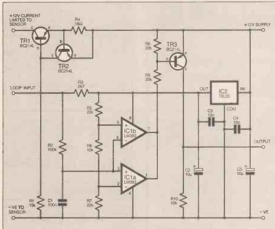
Fig. 5. Circuit diagram for the Loop Interface.
