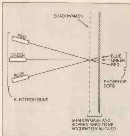
Fig. 26. Operation of the shadowmask.
