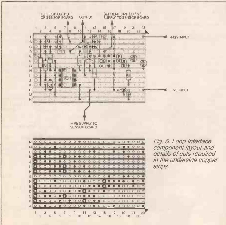
Fig. 6. Loop Interface component layout and details of cuts required in the underside copper strips.
