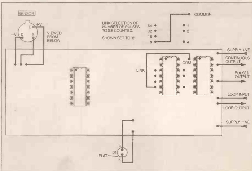
Fig. 3. Interwiring connections to Sensor board and link to select pulse count details.
