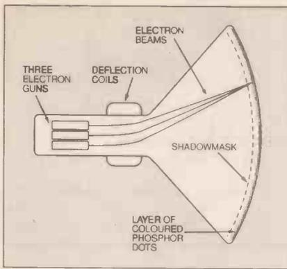
Fig. 25. Construction of a colour tube.
