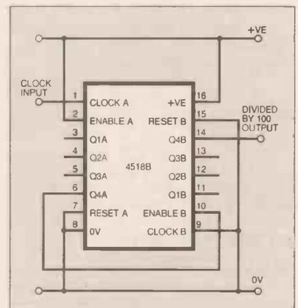
Fig. 7.8. A divide-by-100 circuit.
