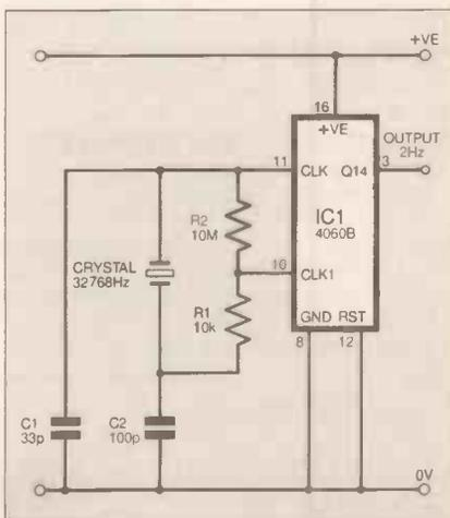
Fig. 7.5. Combined crystal oscillator and counter circuit.
