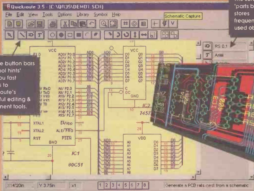
Multiple button bars with 'tool hints' give you fast access to Quickroute's powerful editing & placement tools.
