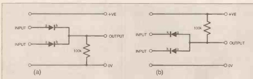
Fig. 7.6. (a) A diode OR gate. (b) A diode AND gate.
