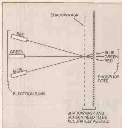
Fig. 26. Operation of the shadowmask.
