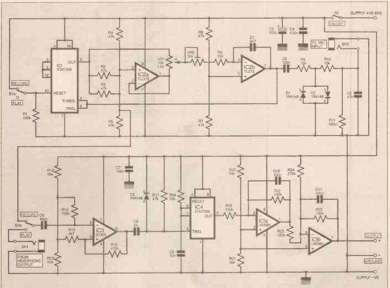
Fig. 2. Complete circuit diagram for the Tape Controller. The Record/Play switch is a double-pole "slider" type.
