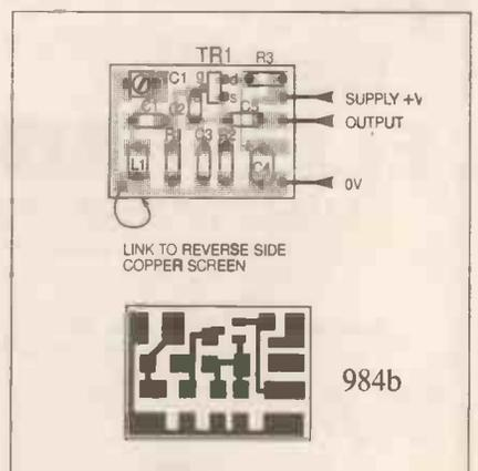
Fig. 2. Printed circuit board component layout and copper foil master pattern.
