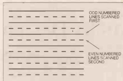
Fig. 24. Interlacing of screen scan.
