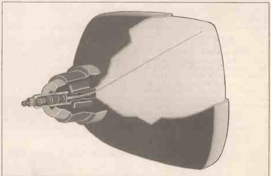
*Cutaway view of a modern c.r.t.* This illustration and the title photograph, courtesy of Philips Test and Measuring Instruments.
