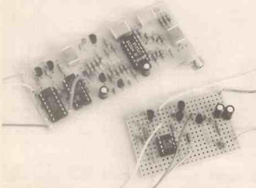
Complete Sensor p.c.b. and Loop Interface strip board.
