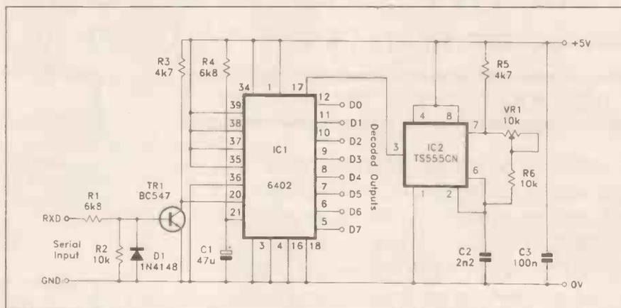
Fig. 1. Circuit diagram for the RS232C to parallel data converter.
