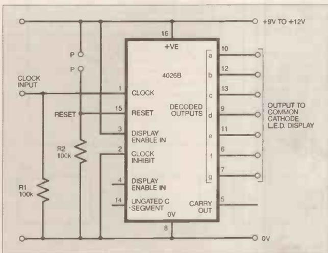
Fig. 7.10. The 4026B i.c. is a combined counter and 7-segment l.e.d. display driver. Points P are for a reset function.
