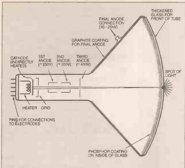
Fig. 18. Simplified diagram of a c.r.t. In essence, only one anode is required.
