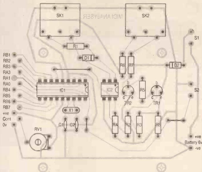
Fig. 5. Printed circuit board component layout and actual size copper foil master for the MIDI Analyser.
