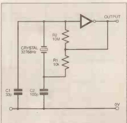
Fig. 7.4. A simple crystal oscillator circuit.
