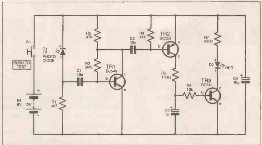
Fig. 3. Circuit diagram for the Remote Handset Tester.
