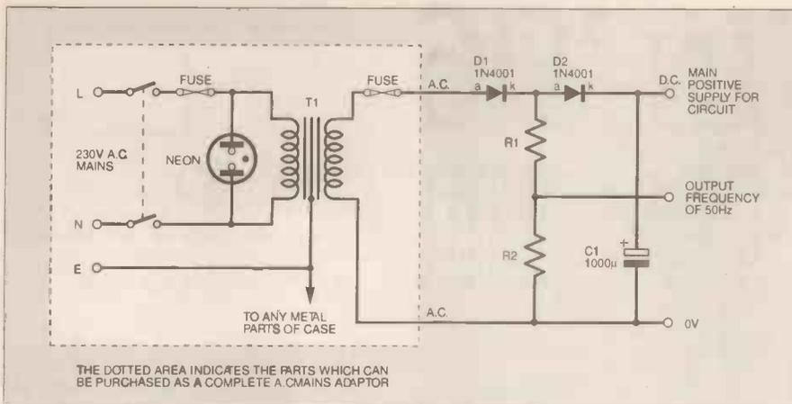
Fig. 7.2. Deriving a 50Hz signal from an a.c. power supply.
