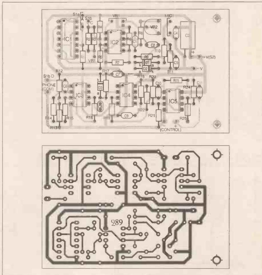
Fig. 3. Tape Controller printed circuit board component layout and full size copper foil master pattern.
