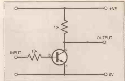
Fig. 7.7. A simple transistor inverter.
