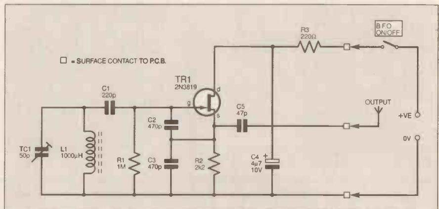
Fig. 1. Complete circuit diagram for the B.F.O.
