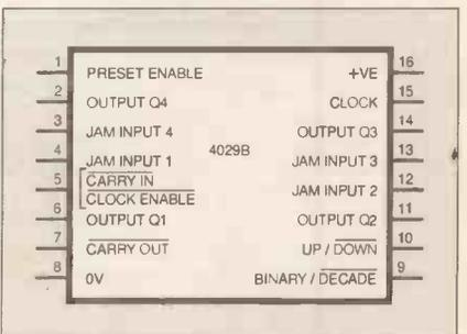
Fig. 3. Pinouts of the 4029B counter i.c.
