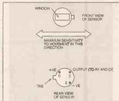
Fig. 4. Sensor pinout and sensitivity details.
