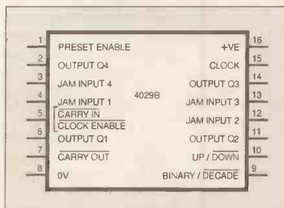
Fig. 3. Pinouts of the 4029B counter i.c.
