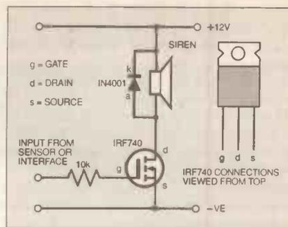
Fig. 7. Simple circuit diagram for interfacing to a warning Siren using a power MOSFET.
