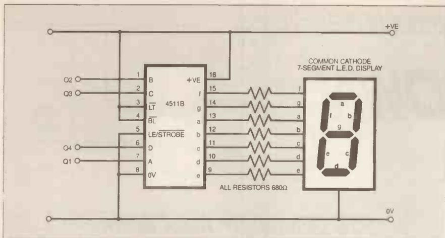
Fig. 7.9. The 4511B i.c. converts a BCD input code into a format suitable for driving a seven-segment l.e.d. display.
