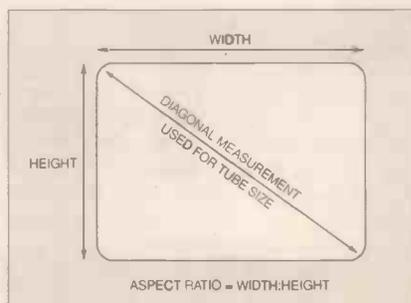
Fig. 23. Aspect ratio and size.
