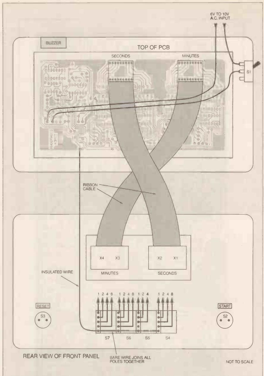
Fig. 7. Interwiring of the p.c.b. to the case-mounted components not shown in Fig. 5.
