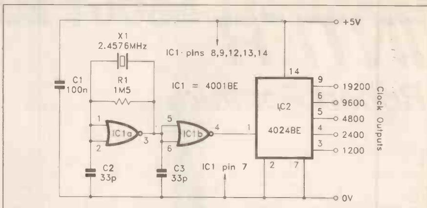
Fig. 2. Circuit diagram for a simple crystal controlled baud rate generator.
