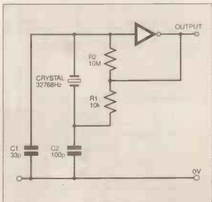
Fig. 7.4. A simple crystal oscillator circuit.
