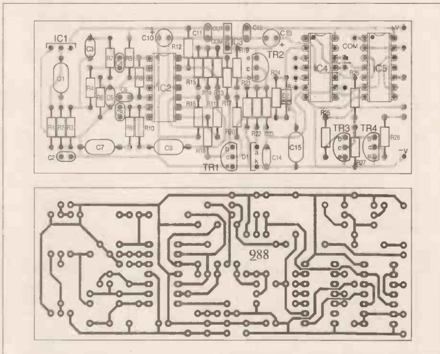
Fig. 2. Sensor printed circuit board component layout and actual size underside copper foil master pattern.
