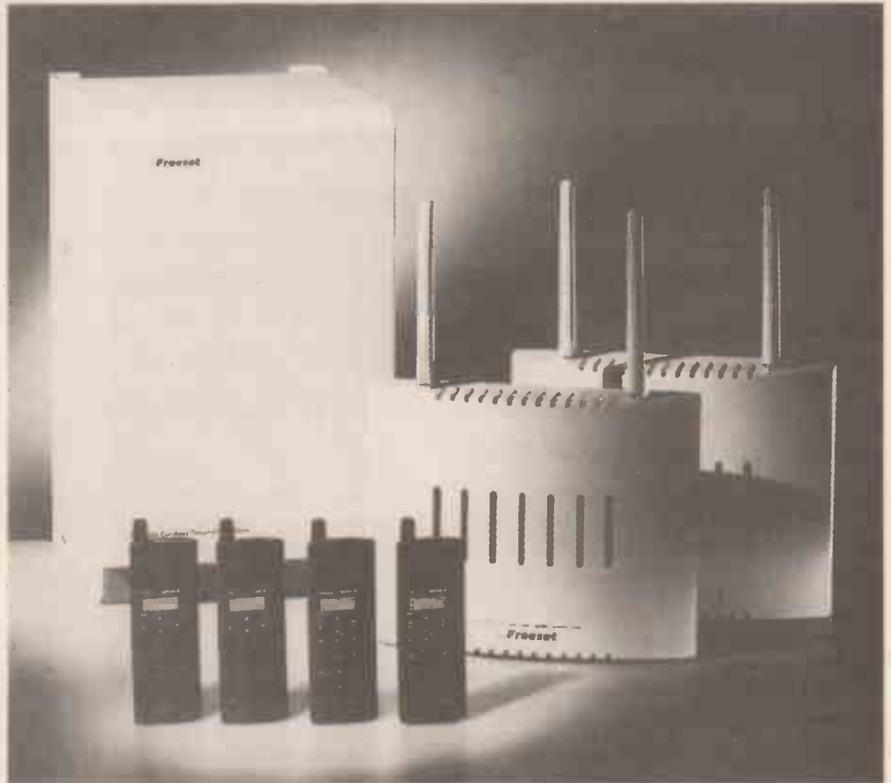
*Freeset is a unique digital cordless phone system comprising a radio exchange, base stations and portable handsets.*
