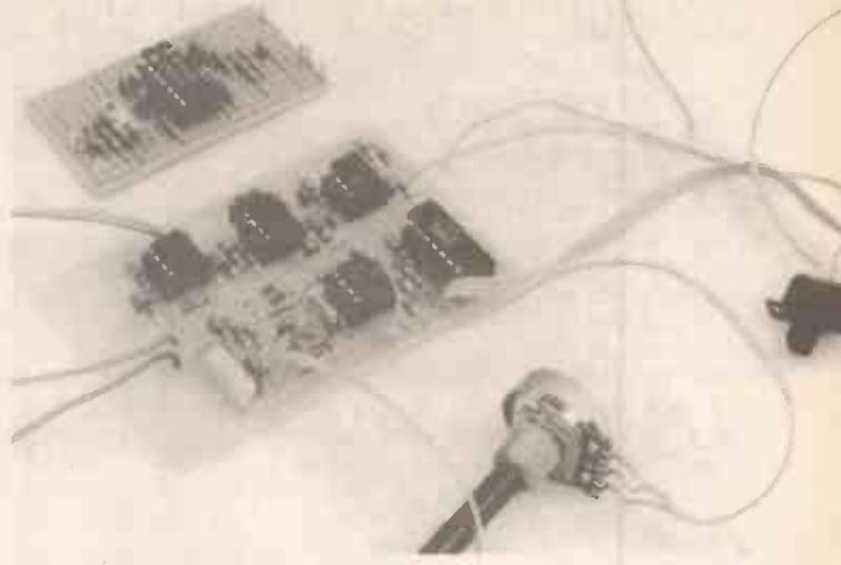
Completed Tape Controller board together with the Signal Level Indicator board.
