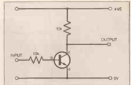
Fig. 7.7. A simple transistor inverter.
