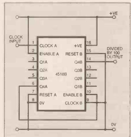
Fig. 7.8. A divide-by-100 circuit.
