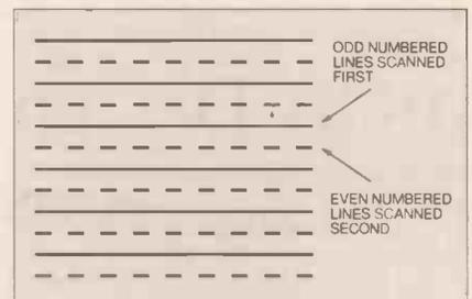
Fig. 24. Interlacing of screen scan.
