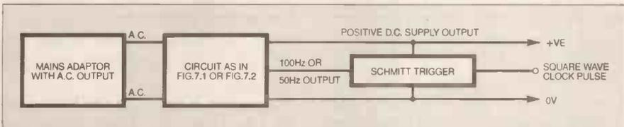
Fig. 7.3. A Schmitt trigger improves the clock waveform shape.
