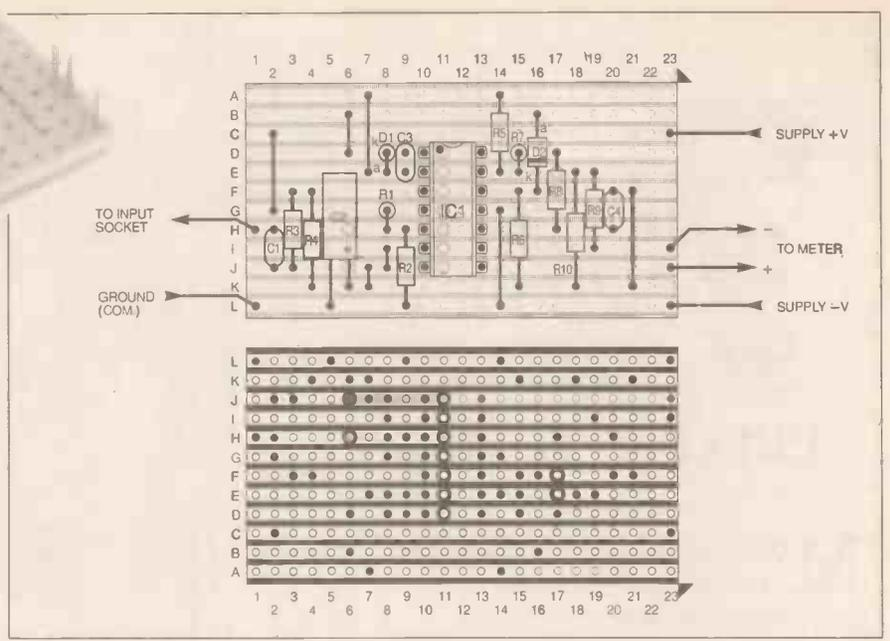
Fig. 6. Signal Level stripboard component layout and details of underside breaks required in copper tracks.
