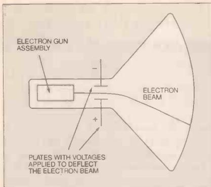
Fig. 21. Electrostatic deflection.
