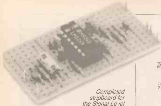
Completed stripboard for the Signal Level Indicator.
