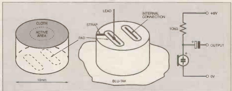
Fig. 2. Condenser (electret) microphone. The negative terminal is identified by the strap which connects it to the case. Two pads are provided for leads. These are loaded with solder, which conceals the internal connections shown. To solder a lead, press the mike into some Blu-tack. Then melt the solder on the pad, and stand a vertical wire outside the internal connection, as drawn. To lift the mic. from the Blu-tack, rock gently. Output is taken from a series resistor, as indicated.
