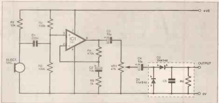
Fig. 8.4. Circuit diagram for the audio input module which produces a d.c. output voltage relative to the input signal amplitude.
