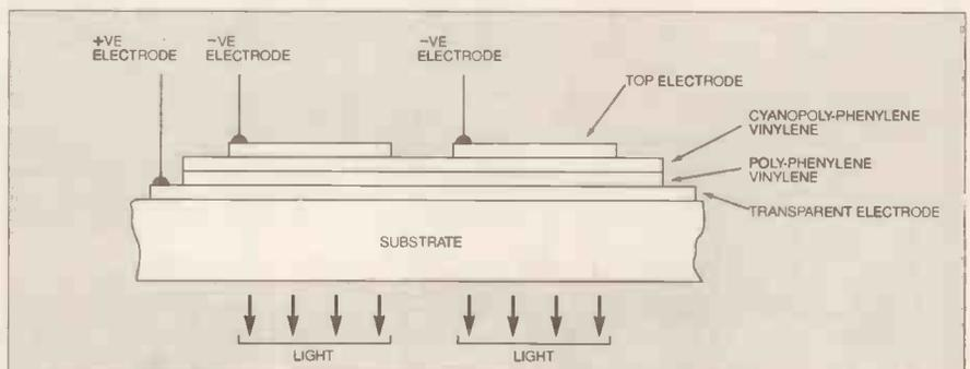
Fig. 1 The structure of a light emitting polymer display.
