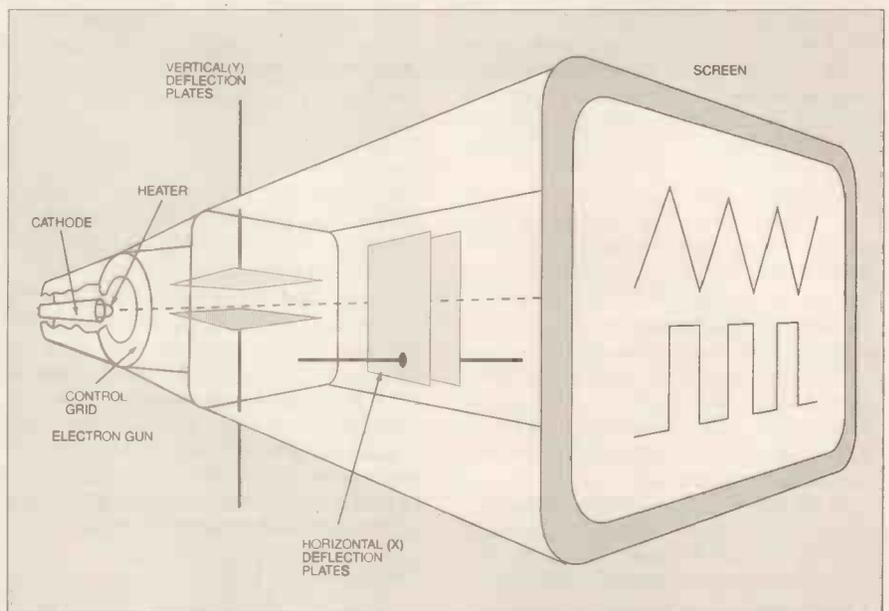
Fig. 1. Basic details of a cathode ray tube as used in an oscilloscope, excluding focussing and acceleration anodes.
