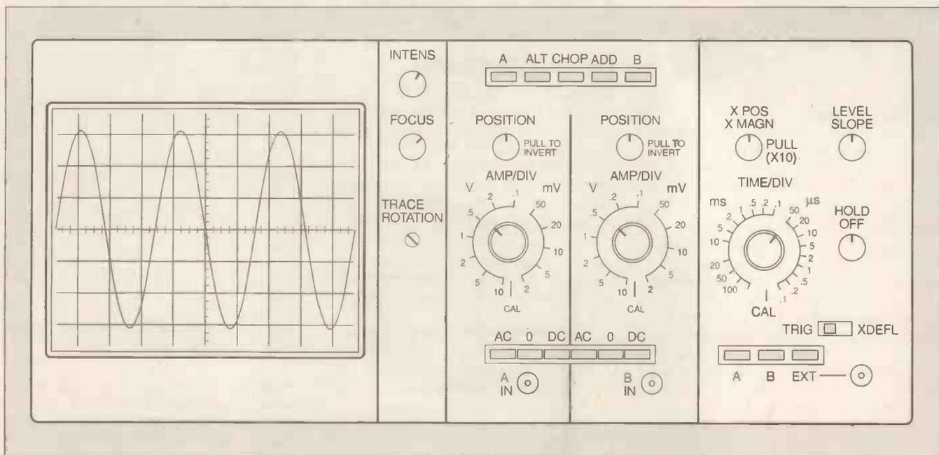
Fig. 5. Stylized layout of the basic controls on a typical dual-trace oscilloscope.
