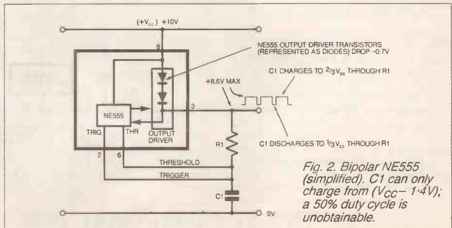
Fig. 2. Bipolar NE555 (simplified). C1 can only charge from ( $V_{cc} - 1.4V$ ); a 50% duty cycle is unobtainable.
