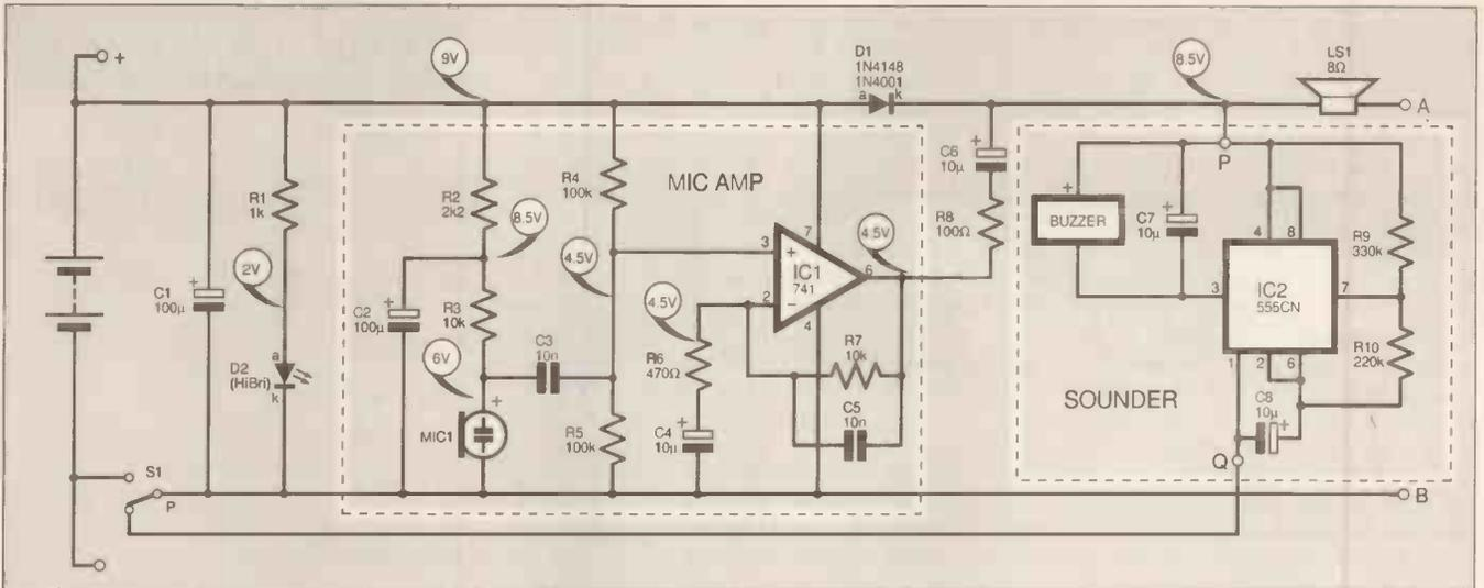
Fig. 4. Complete Home Telephone link Circuit diagram. The voltages marked should appear when the phone is lifted, if the test meter negative lead is connected to the B wire. Nothing should be attached at A and B. Speaking into the mic. should raise the voltage at P.
