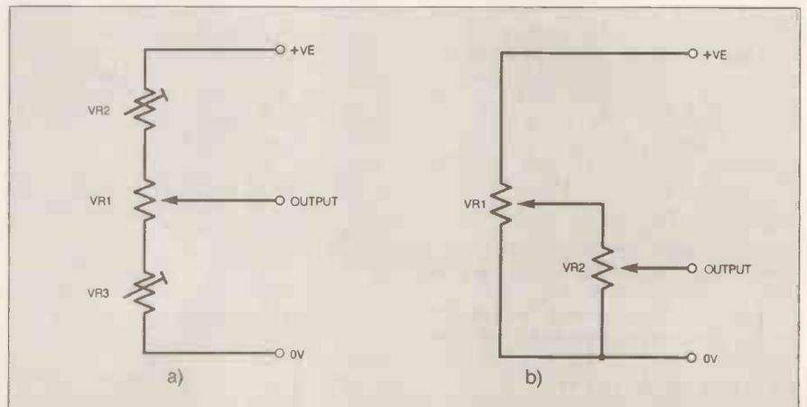
Fig. 8.8. Two methods for restricting the output voltage range from a potentiometer.
