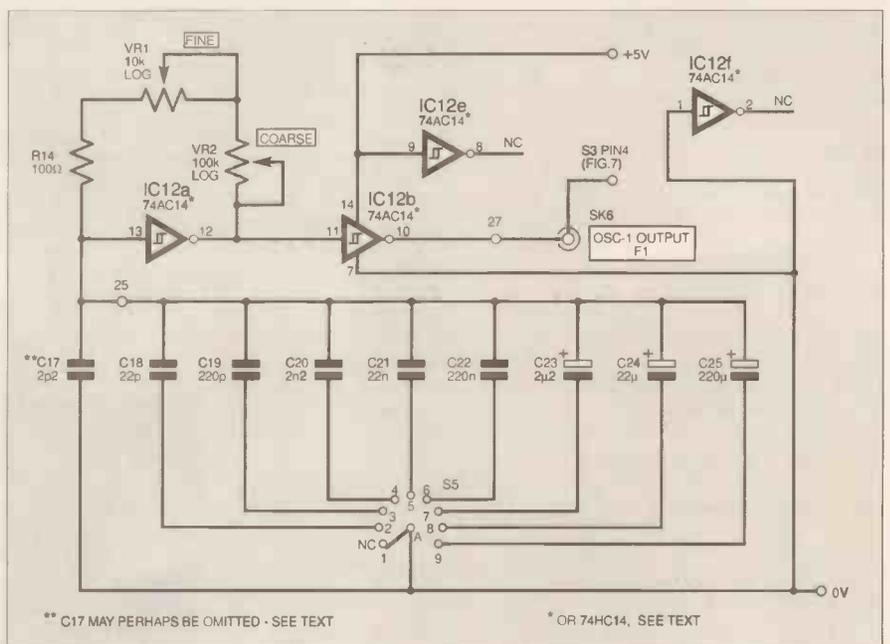
Fig. 2. Circuit diagram for Oscillator-1.
