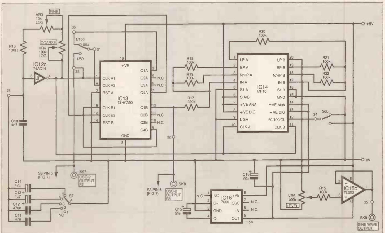
Fig. 3. Circuit diagram for Oscillator-2 and Sinewave filter stages.
