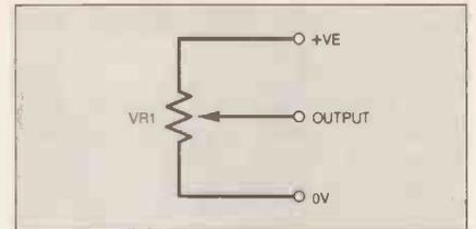
Fig. 8.6. A potentiometer can be used for position-to-voltage sensing.
