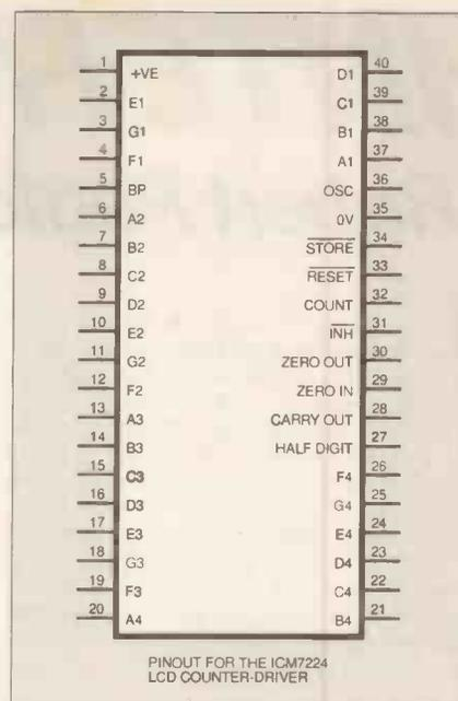
PINOUT FOR THE ICM7224 LCD COUNTER-DRIVER
