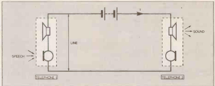
Fig. 1. Simultaneous two-way communication. Speech at either microphone modulates the circulating current, reproducing the sound in both earphones.
