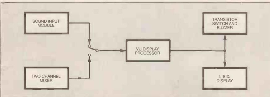
Fig. 1. Block diagram for the VU Display and Alarm.
