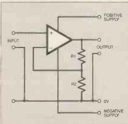
Fig. 8.1. Circuit diagram for an op.amp non-inverting amplifier.
