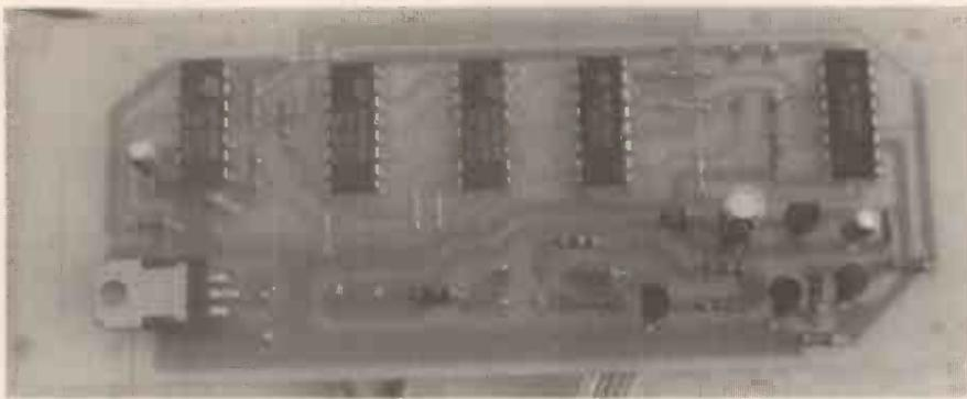
Component layout on completed circuit board. The power MOSFET TR1 has been carefully bent horizontally with the p.c.b.
