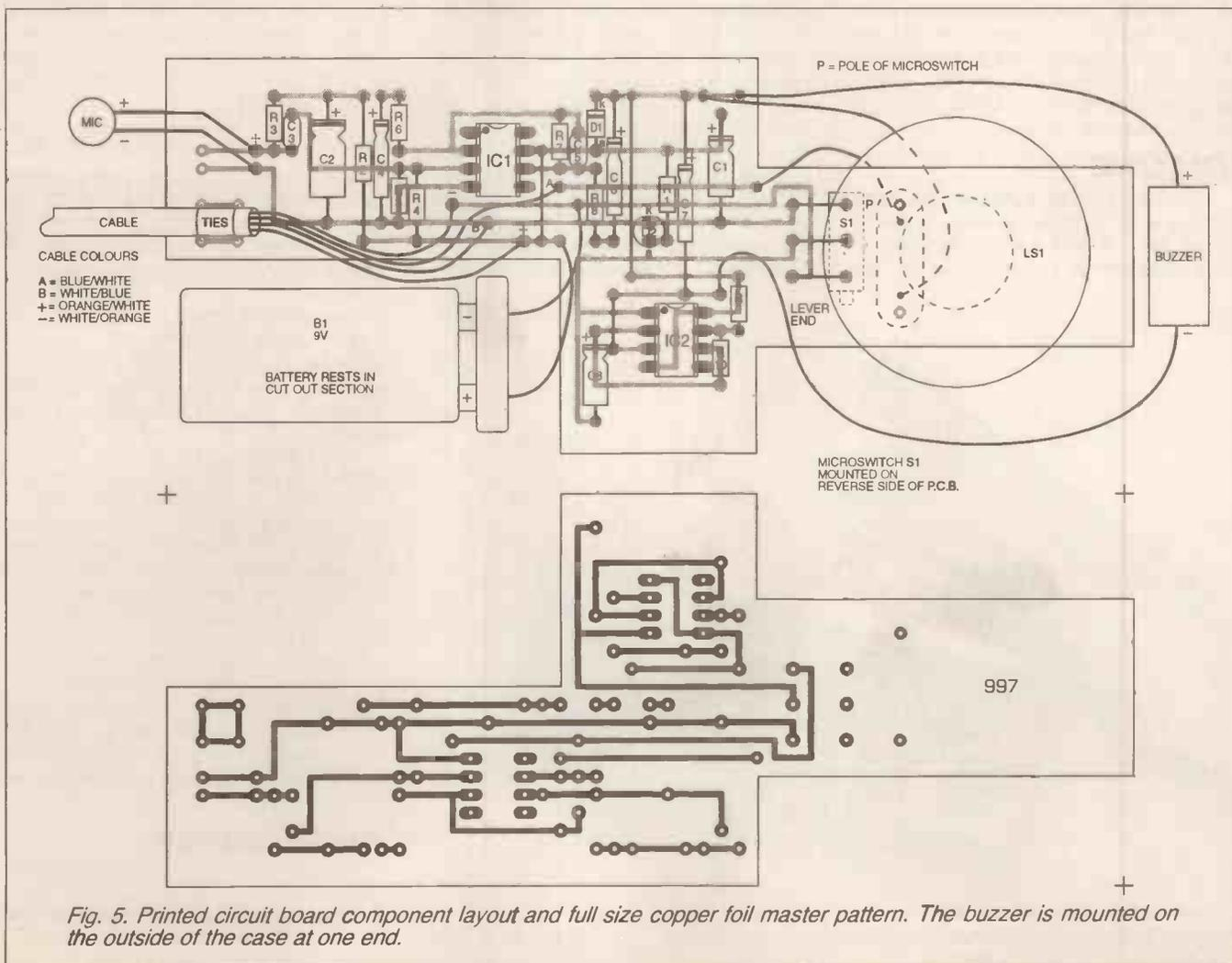
Fig. 5. Printed circuit board component layout and full size copper foil master pattern. The buzzer is mounted on the outside of the case at one end.
