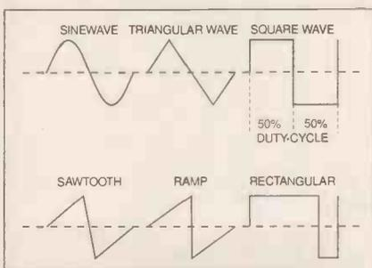
Fig. 6. Idealised standard waveforms.
