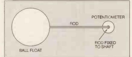
Fig. 8.7. Using a potentiometer to sense water level changes.
