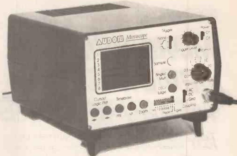
With positive or negative triggering selected, the sweep commences when the appropriate type of transition is detected on the Channel 8 input. However, trigger pulses are ignored until the unit has been "cocked" by pressing the Sample button. This avoids unwanted multiple triggering of the unit.
