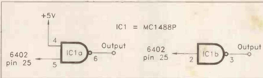
Fig. 4. Using the driver in the MC1488P.
