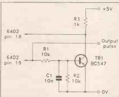
Fig. 1. Circuit which generates a strobe pulse each time a fresh byte of data is available.
