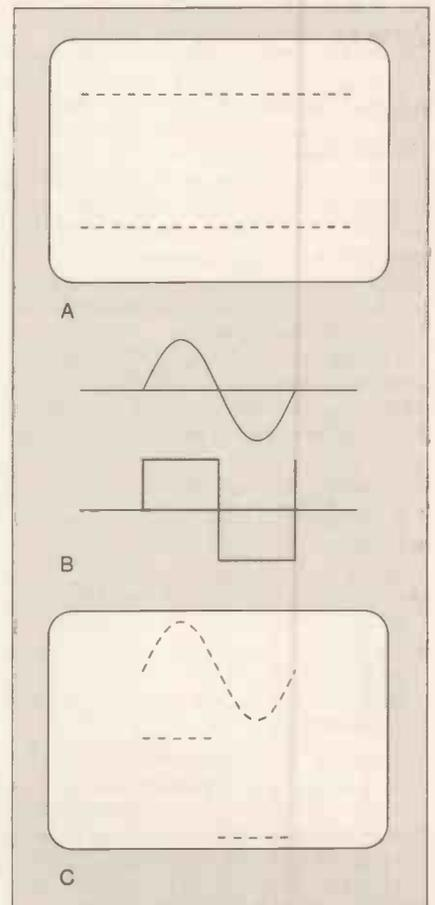
Fig. 3. Timebase presentation of signals on a dual-trace oscilloscope.
