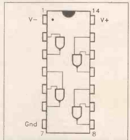
Fig. 3. Pinout details for the MC1488P quad line driver.
