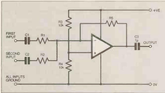
Fig. 8.5. Basic 2-channel op.amp mixer circuit.
