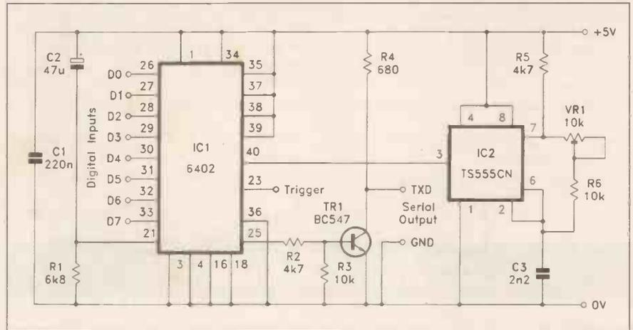
Fig. 2. The serial transmitter circuit. The trigger input is pulsed low to transmit a byte of data.
