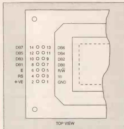
Fig. 4. Pinouts for the l.c.d. module.
