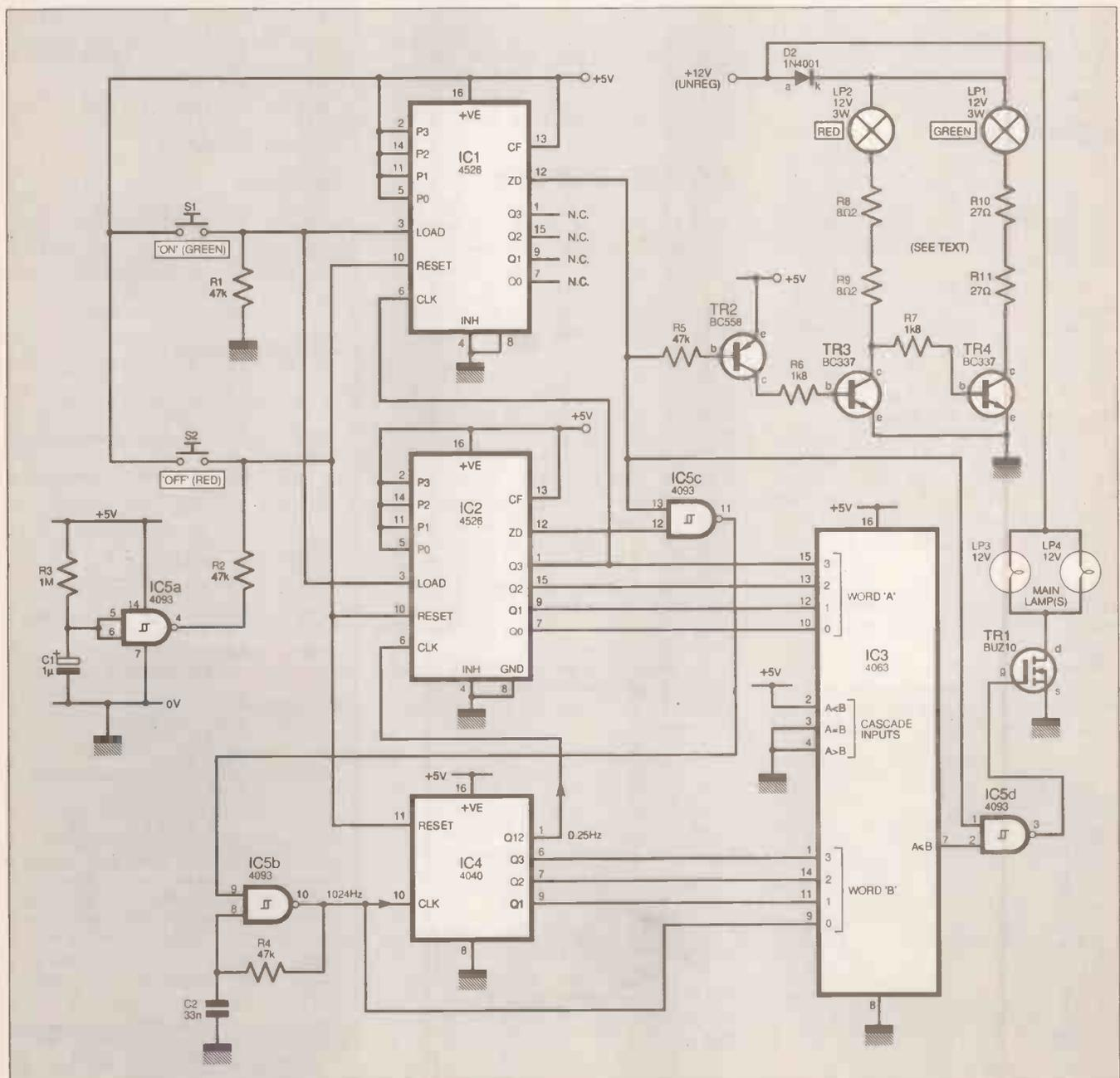
Fig. 1. Main control circuit diagram for Sarah's Light. Switches S1 and S2 are combined with indicator lamps LP1 and LP2.
