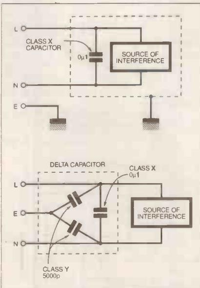
Fig. 4. Suppressor capacitors help prevent interference generated by equipment, feeding into the mains supply, and reduce electromagnetic interference.
