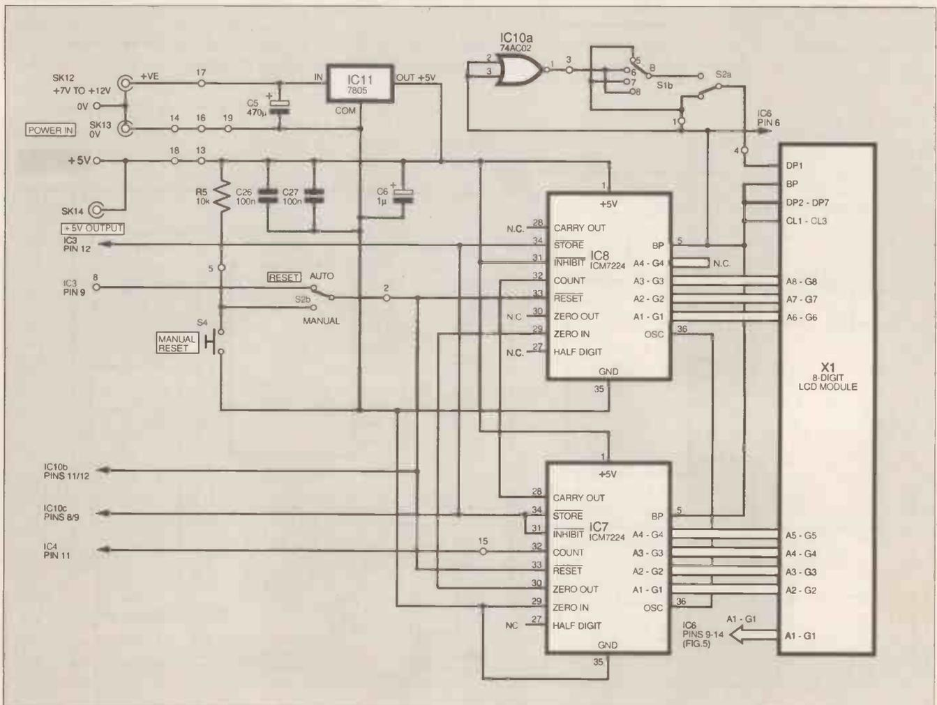
Fig. 4. Circuit diagram for l.c.d. digits 2 to 7 counter/driver, display and power supply.
