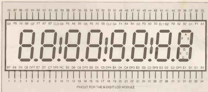
Fig. 8. Pinouts for the 8-digit l.c.d. module and (right) the ICM7224 counter/driver.
