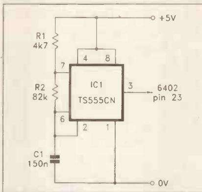
Fig. 5. A circuit which provides regular triggering to the 6402 UART.
