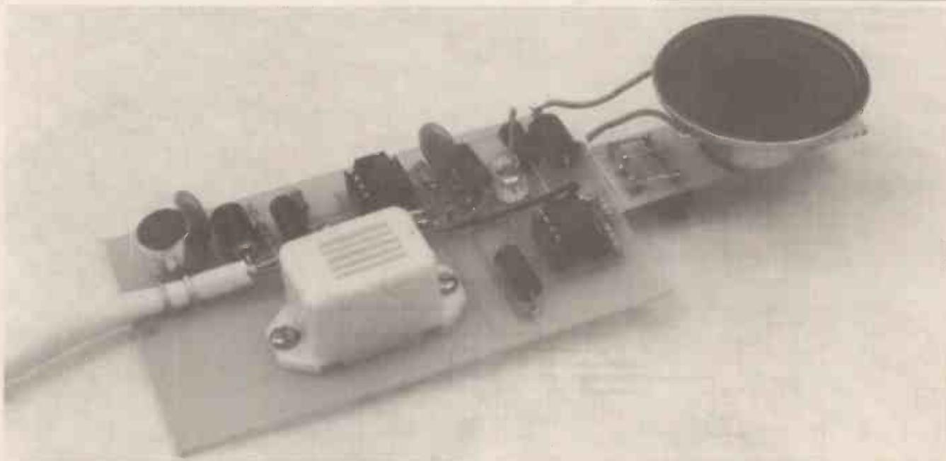
The first prototype phone built on a printed circuit board. This prototype was not intended to be housed in a case so the microphone and buzzer were mounted directly on the p.c.b. When inserted in the case, the p.c.b. has to be cut to take the battery, the microphone mounted inside the lid and the buzzer on the outside of the case.
