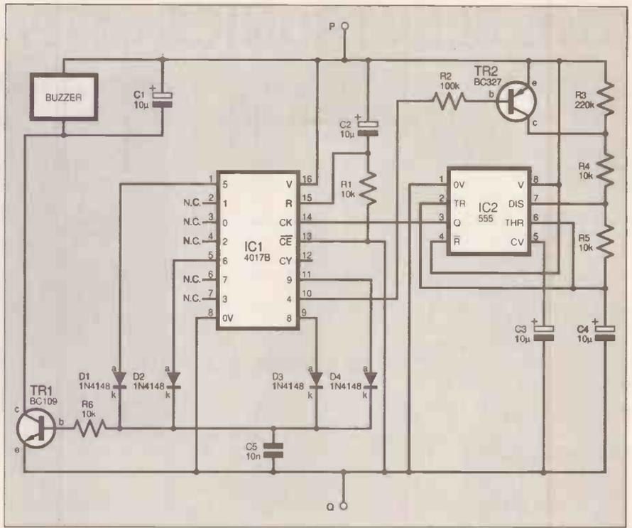
Fig. 6. Circuit for producing the familiar BT ringing cadence. The 555 timer period is 0.2 sec., and the 4017 IC1 sounds the buzzer at counts 5 + 6 and 8 + 9. Count 4 is stretched. This circuit replaces components between points P and Q in Fig. 4 if required.
