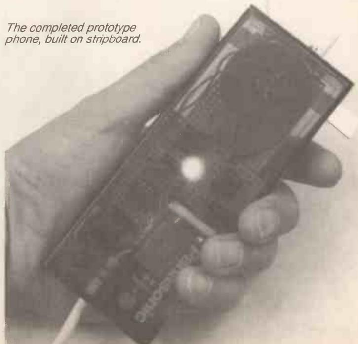
The completed prototype phone, built on stripboard.
