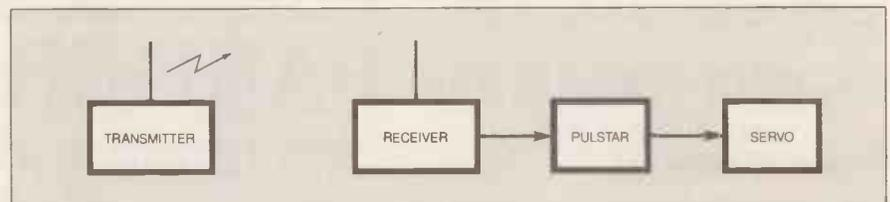
Fig. 1. Block diagram showing how PulStar fits into an R-C system.
