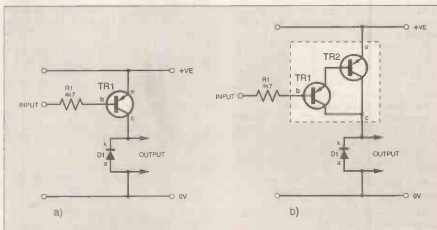
Fig. 8.210. Two examples of a *pn*p switch: (a) a single transistor and (b) a Darlington transistor.
