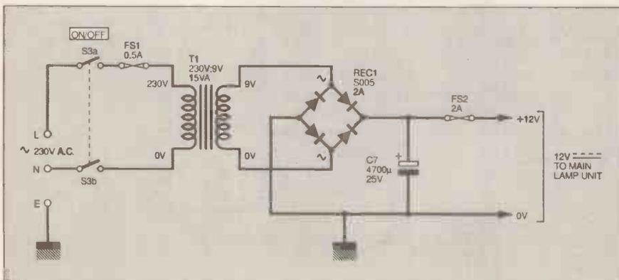
Fig. 3. Circuit diagram for a suggested mains driven power supply.
