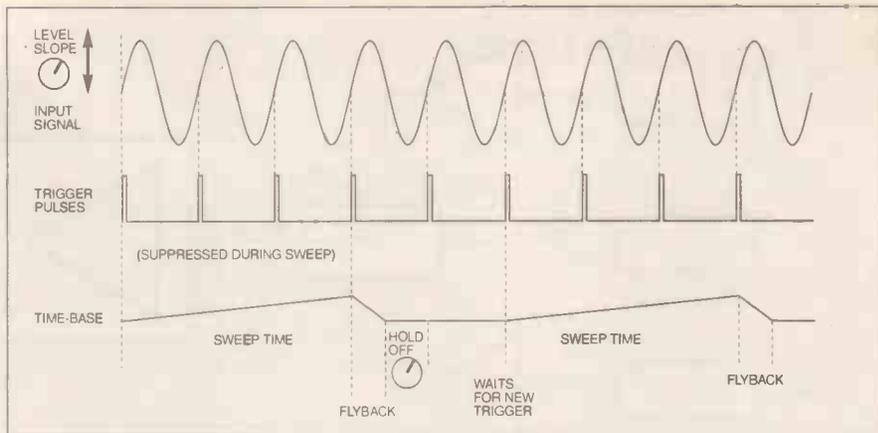
Fig. 4. Timebase generator output waveforms.
