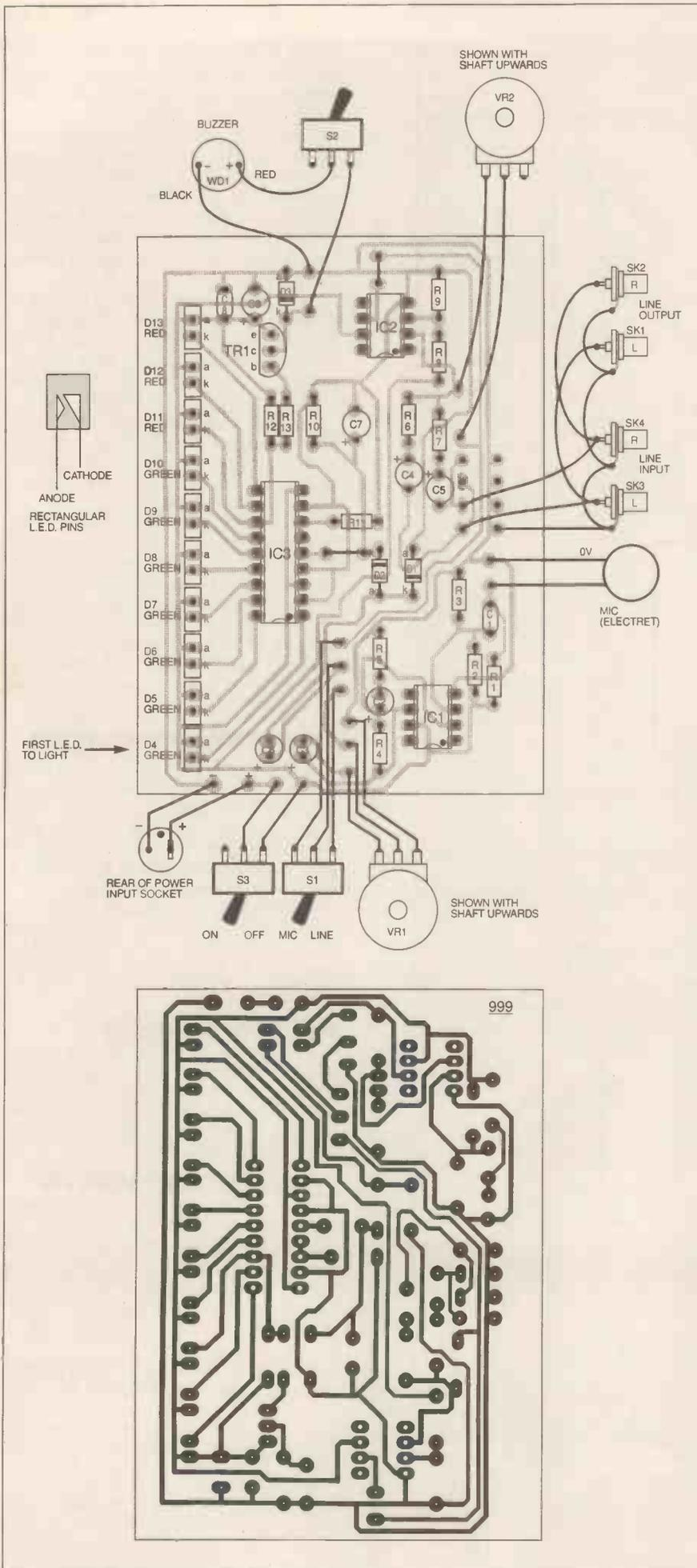
Fig. 3. Printed circuit board component layout and full-size underside copper foil track master pattern.
