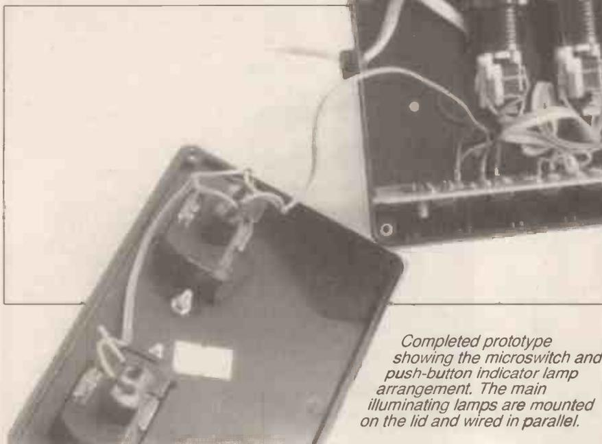
Completed prototype showing the microswitch and push-button indicator lamp arrangement. The main illuminating lamps are mounted on the lid and wired in parallel.
