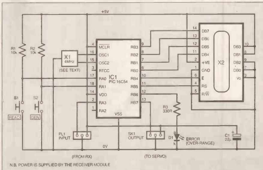
Fig. 2. Complete circuit diagram for PulStar.
