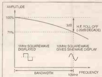
Fig. 8. Frequency response of a 10MHz oscilloscope.
