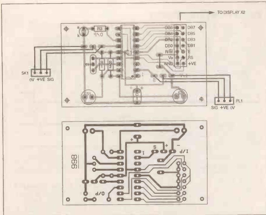
Fig. 3. Printed circuit board component layout and full size copper foil master track pattern for PulStar.
