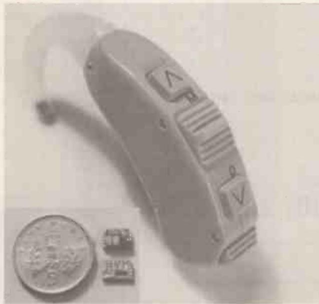
The hearing instrument worn behind the ear (BTE) has two controls to select the user's required programme needs. The inset shows how small the unit's control boards are.
