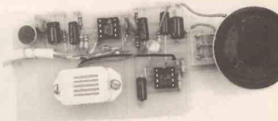
The microphone insert and buzzer are not mounted on the p.c.b. in the final version. The board is carefully cut to make space for the battery and the microphone is glued to the inside lid of the case – see below.
