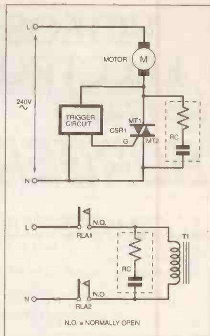
Fig. 3. Typical RC snubber applications
