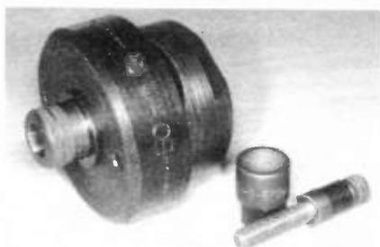
Q-Max sheet metal punches come in a variety of sizes ( $\frac{3}{8}$  and 50mm shown here).
