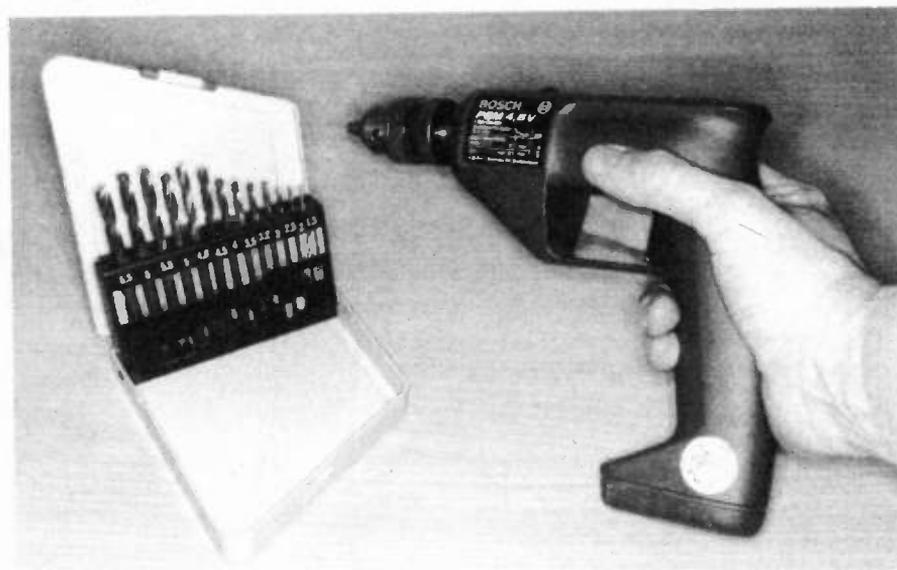
*If you're serious about project building, you will need a set of high speed steel (HSS) twist drills and preferably a rechargeable drill.*
