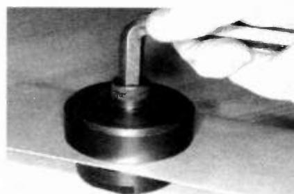
Using an Allen hex key, the punch is tightened up until the two halves make a clean cut in the panel.
