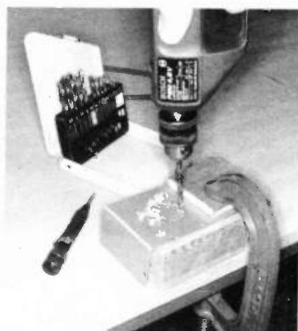
Using a G-clamp to hold the work piece, with wood blocks to prevent scratches.
