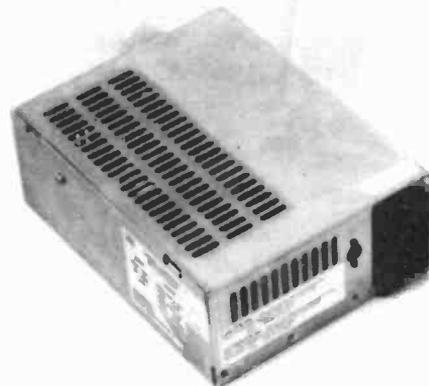
Over the years, we've had many different switch mode power supplies, but this latest unit is without doubt one of the finest we've ever seen! Made by Astec, it is a totally enclosed steel cased unit measuring 175x136x65mm, which has incorporated in it a switched and fused IEC mains inlet. Inside, the PCB is 160x80mm with output pins fitted on one end. A connector to these pins to extend the outputs to the exterior of the case is provided.
