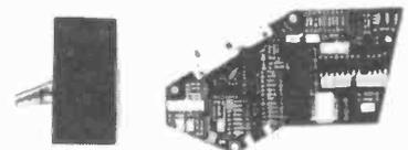
**Z1438** Control panel from sheet feeder. 90x45mm. PCB fitted with 4 illuminated push switches (all with yellow LED), and separate green LED.
