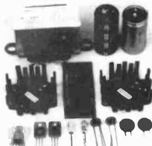
**Z4190** Disk Drive Power Supply Kit. Ideal for powering single 3 1/2" or 5 1/4" drive. Mains input, stabilised smoothed outputs, 12V @ 1A and 5V @ 1A. Simple, easy to assemble kit with full instructions, at an excellent price **£5.95**
