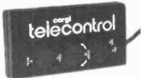
**Z4133** Corgi telecontrol. Neat 2 part black plastic case 100x60x25mm with 3 red control switches, 2W, 3W and 8W, believed to come from a low cost game. 1m long 5 core lead attached. **60p**
