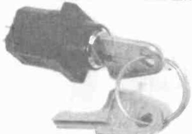
**Z2168** Superb quality British made (TOK). Gold plated DPCO contacts. Key can be removed in either position. PC mounting or clip fix - needs 15x15mm cut-out. Ideal for alarms etc.
