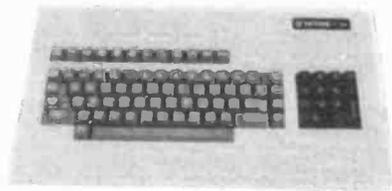
**Z8842** Tatung VT4100 keyboard. Cased 85 key units with separate numeric keypad. With circuit. Has 2 or 3 broken key tops. 450 x 65 x 125mm.
