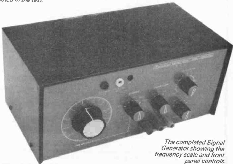
The completed Signal Generator showing the frequency scale and front panel controls.
