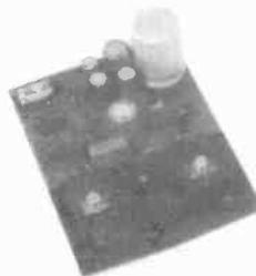
**Z469** AL30A amp. Panel 90 x 64mm. 10W RMS with 30V supply. Popular audio amp module, these are ex-equip, but believed to be working.
