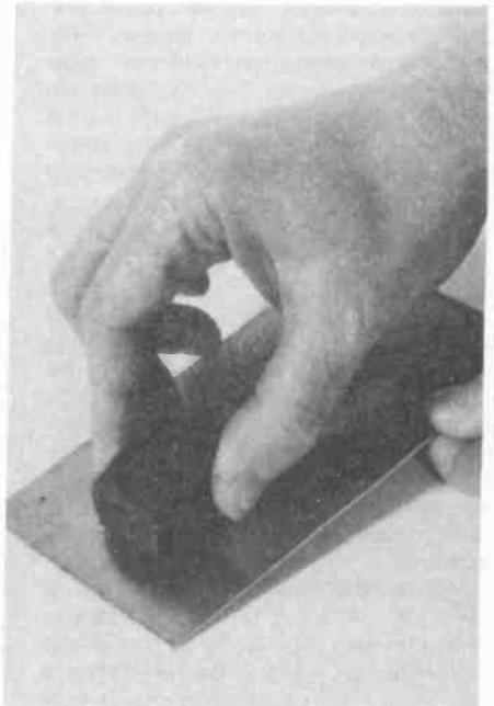
*Cleaning the board with an abrasive block.*
