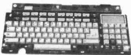
**Z8852** Keyboard: Superb brand new keyboard 392x181 with LCD displaying 1 line of 10 characters and a further line with various symbols. 100 keys, inc separate numeric keypad. Chips on board are 2x74HC05, 80C48. LCD + driver chips are easily removable from board. Looks like it was used with a comms package.
