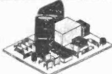
A simple yet highly versatile Infra Red remote control kit with a multitude of uses in the home or car. Operates from 9-15V dc or 240V ac and switches a 3A relay on and off alternately each time the transmitter is operated at ranges up to 20ft (6m). Responds only to the transmitter frequency. Great for lights, TV, alarm controls etc.
