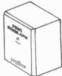
**Z5155** Mini Power Stereo using 2 x LA4140 chips and 6 transistors giving 600mW output Amp. Neat silver cased unit. 88 x 58 x 68mm with LED on front for use with personal stereo. Input lead supplied. Just add 4 x AA batteries (supplied) or 6V PSU and connect speakers!
