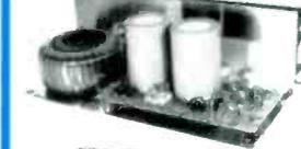
**OMP/MF 200 Mos-Fet Output power 200 watts R.M.S. into 4 ohms, frequency response 1Hz - 100KHz -3dB, Damping Factor >300, Slew Rate 50V/uS, T.H.D. typical 0.001%, Input Sensitivity 500mV, S.N.R. -110 dB. Size 300 x 155 x 100mm.
