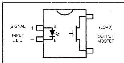
*Fig.1. A photovoltaic MOSFET-type of solid-state relay in a dual-in-line package.*
