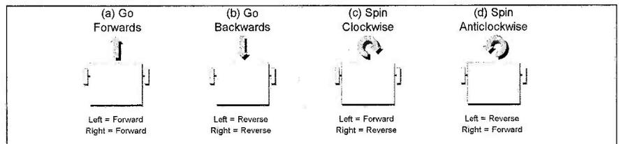
Fig.2: Cases where both motors are active
