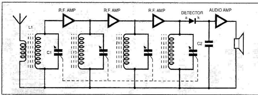
Fig. 10. Simplified T.R.F. (tuned radio frequency) receiver.
