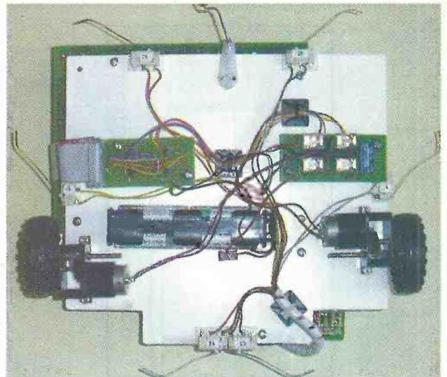
Rear view of the platform showing microswitches positioned in relation to other components.
