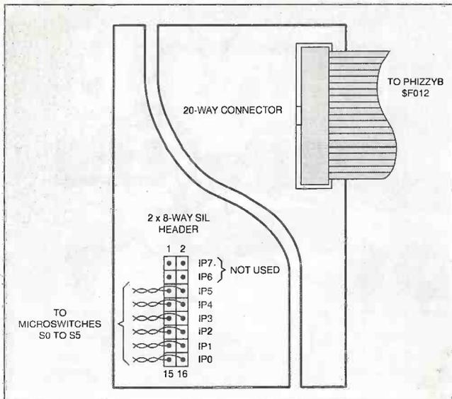
Fig.3. Interconnections to the interrupt driven switch module.
