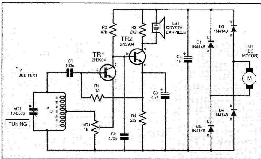
Fig.2. Complete circuit diagram for the Mechanical Radio.
