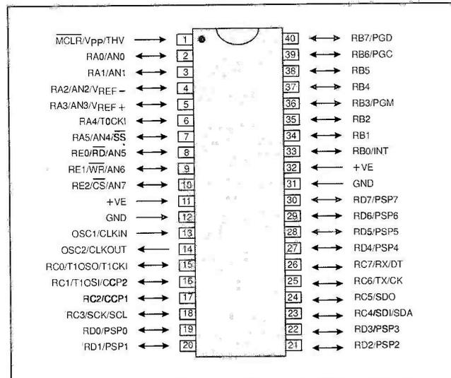
**Fig.2. Pinout details for the PIC16F874/877 microcontrollers.**
