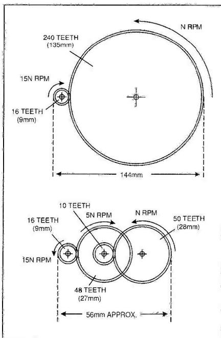
Fig.3. Gear trains with 1:15 ratio.
