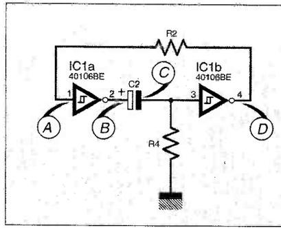
Fig.4. Simplified monostable timer circuit.
