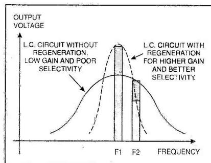
Fig. 12. Response of single tuned circuit with and without regeneration.
