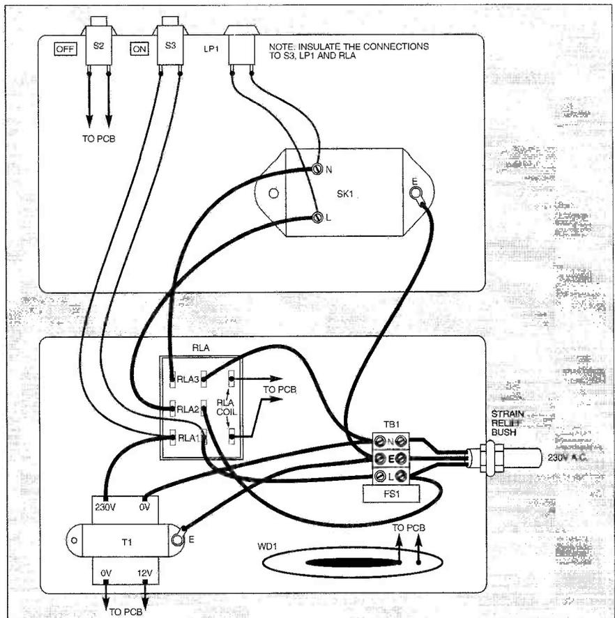
Fig.6. Interwiring of the p.c.b. to all other components. All earth leads must connect back to TB1.
