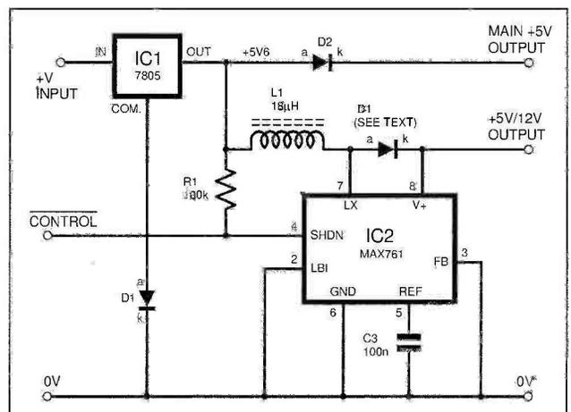
Fig.5. Circuit diagram for a 5V/12V switchable supply from a 5V input.
