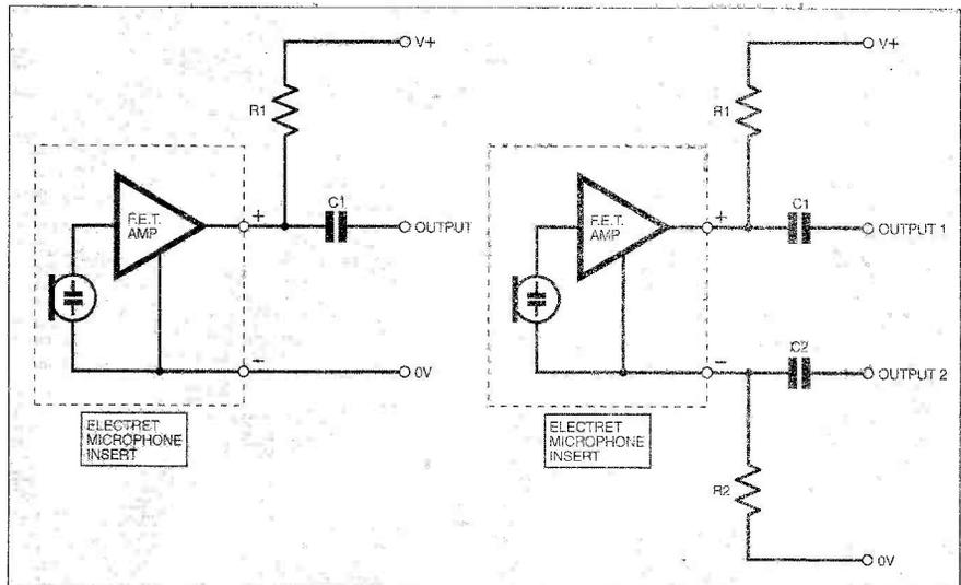
Fig. 4. (left) Normal method of using an electret microphone insert, and (right) producing differential output signals.
