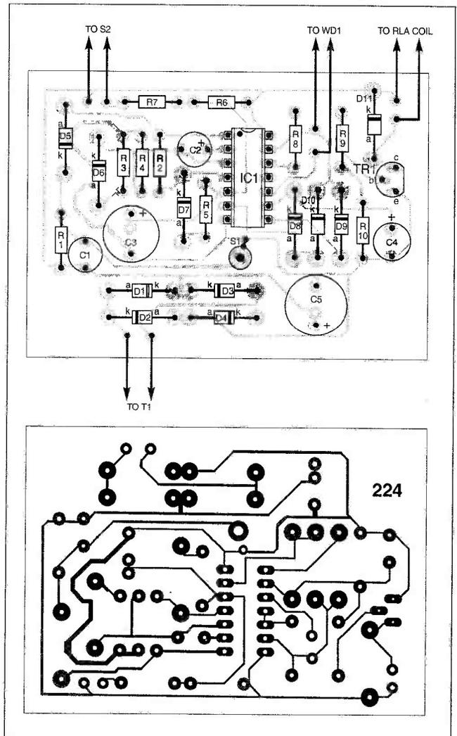
Fig.5. Full size p.c.b. layout for the Ironing Board Saver.
