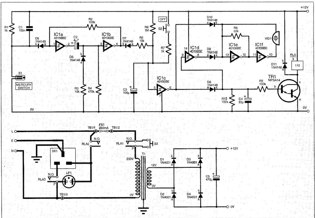
Fig. 1. Complete circuit diagram of the Ironing Board Saver.
