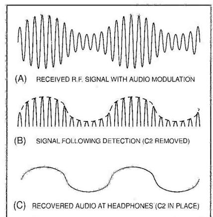
Fig. 9. Example waveforms produced with Fig. 8.
