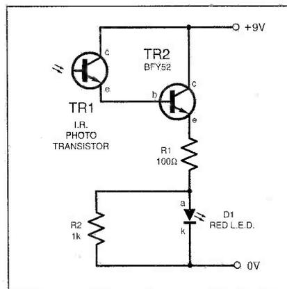
Fig.2. I.R. Remote Control Checker circuit.
