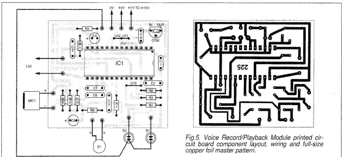
Fig.5. Voice Record/Playback Module printed circuit board component layout, wiring and full-size copper foil master pattern.
