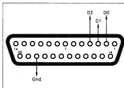
Fig.2. Connection details for the PC printer port.
