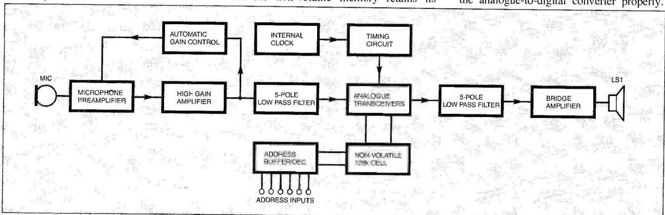
Fig.1. Simplified block schematic diagram for the ISD1416 voice chip.
