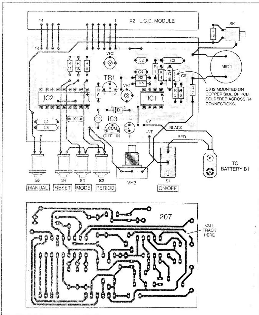
Fig.2. Printed circuit board component layout, interwiring and full size copper foil master for the Versatile Event Counter.
