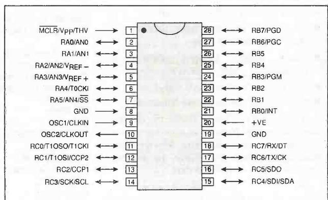
Fig.1. Pinout details for the PIC16F873/876 microcontrollers.
