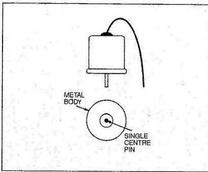
Fig.3. Wiring of S1, the vibration sensor.
