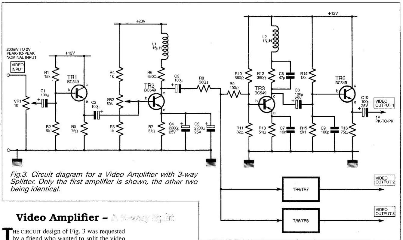
Fig.3. Circuit diagram for a Video Amplifier with 3-way Splitter. Only the first amplifier is shown, the other two being identical.
