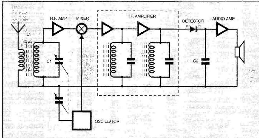
Fig. 11. Simplified superhet receiver.
