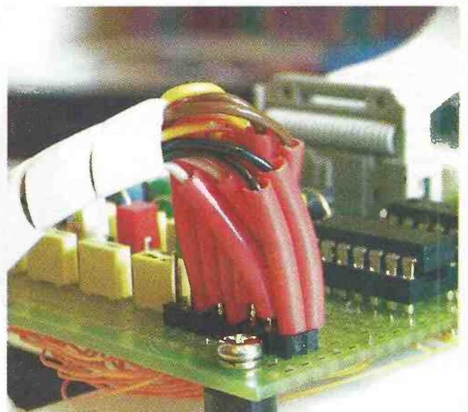
Microswitch leads connected to the interface board.
