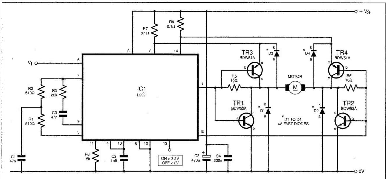
Fig.3. A high power motor controller suitable for 8A d.c. motors, with external power transistor bridge – courtesy SGS-Thomson.
