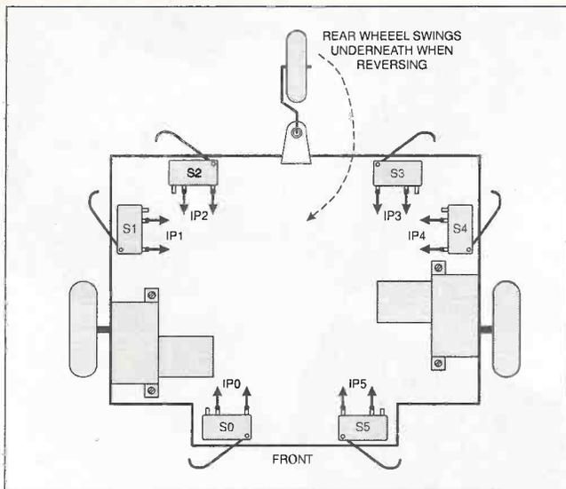
Fig.2. Layout and orientation of the six microswitches on the underside of the PhizzyB platform.
