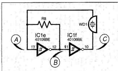
Fig. 2. Simplified piezo buzzer oscillator circuit.
