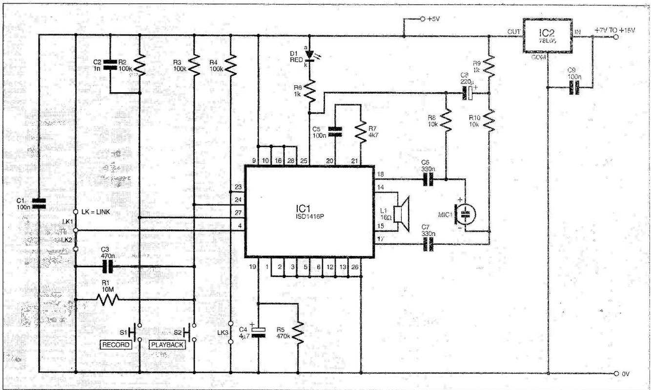
Fig. 3. Complete circuit diagram for the Voice Record/Playback Module.
