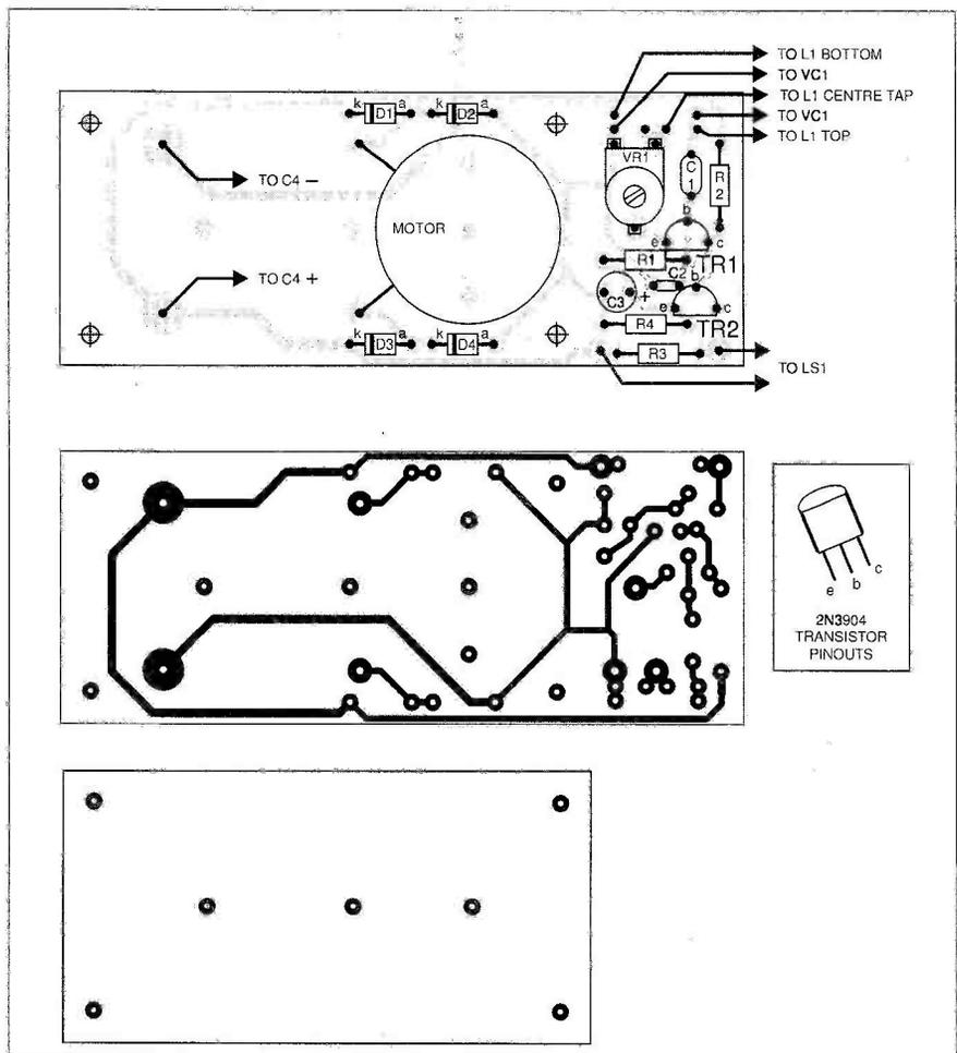
Fig.4. Component and full size track layouts for the printed circuit boards.
