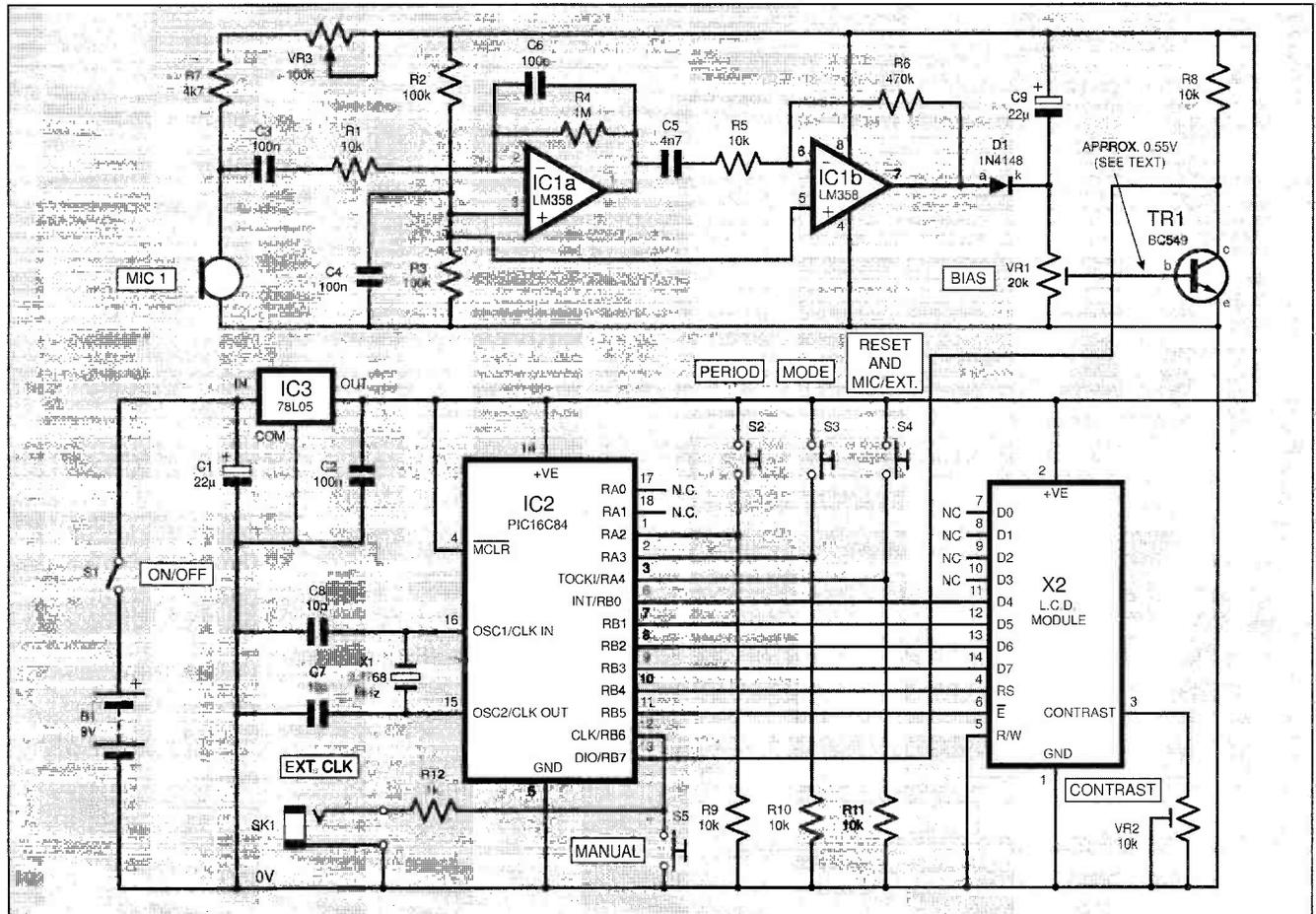
Fig.1. Complete circuit diagram for the Versatile Event Counter.
