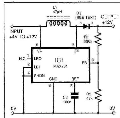
Fig.3. Non-bootstrapped operation, 12V output from 9V input.
