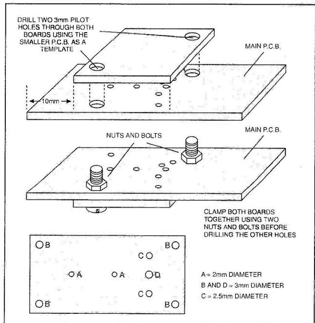
Fig.5. P.C.B. drilling details for the mechanical mountings.
