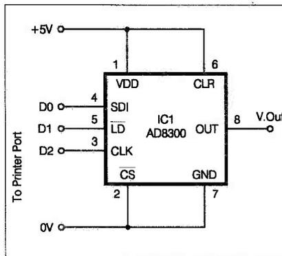
Fig.1. The circuit diagram for the serial DAC. The output potential is 0.5mV per bit.
