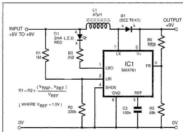
Fig.4. Circuit diagram for a 9V battery life extender, with low battery warning.
