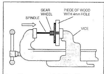
Fig.6. Mounting gear wheel onto spindle.
