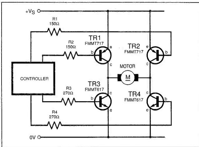
Fig.2. 'H' bridge motor driver capable of controlling the direction of the d.c. motor (2.5A maximum) – courtesy Zetex.
