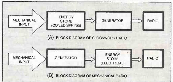
Fig.1. Comparison of the two energy generation methods.
