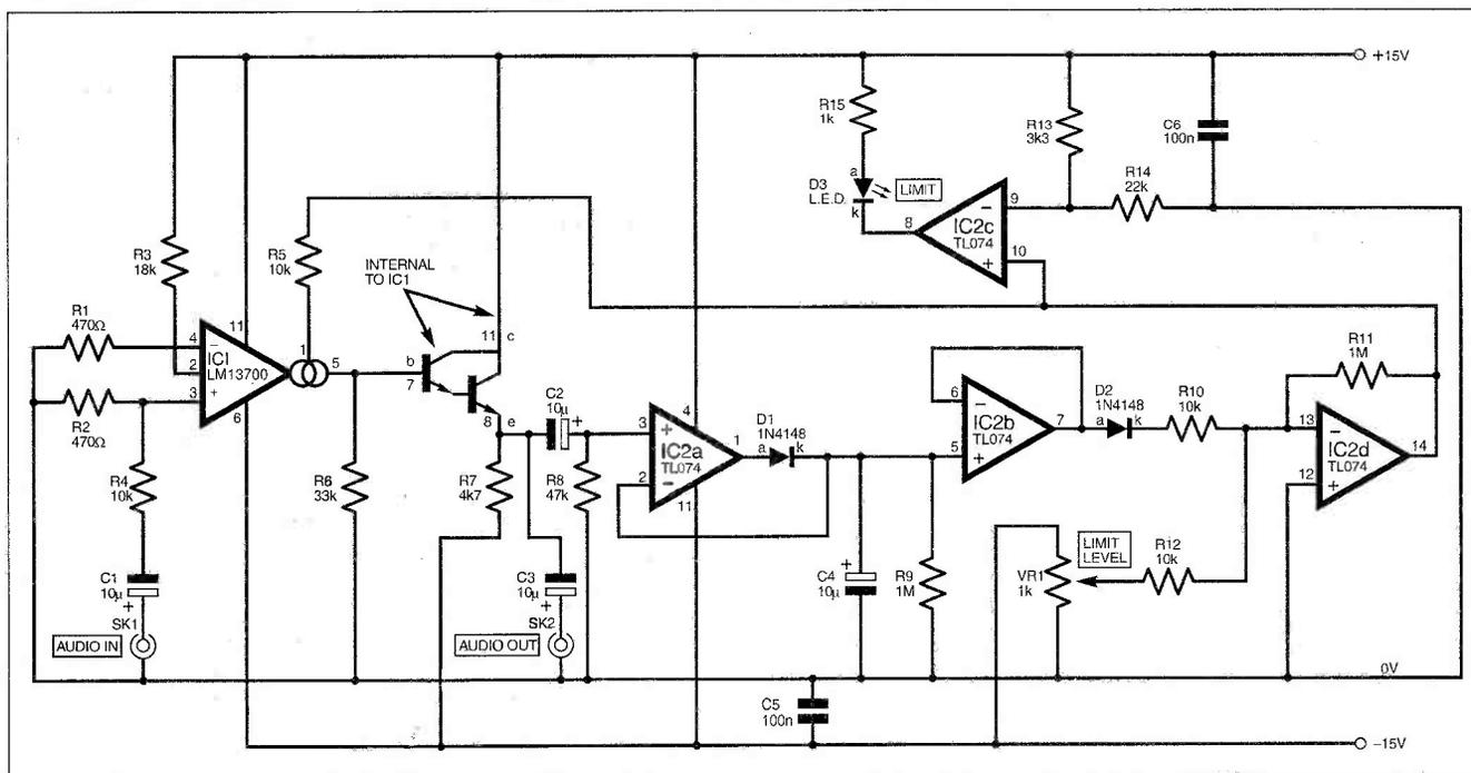
Fig.1. Circuit diagram for the Audio Limiter. Note the "split" power supply.
