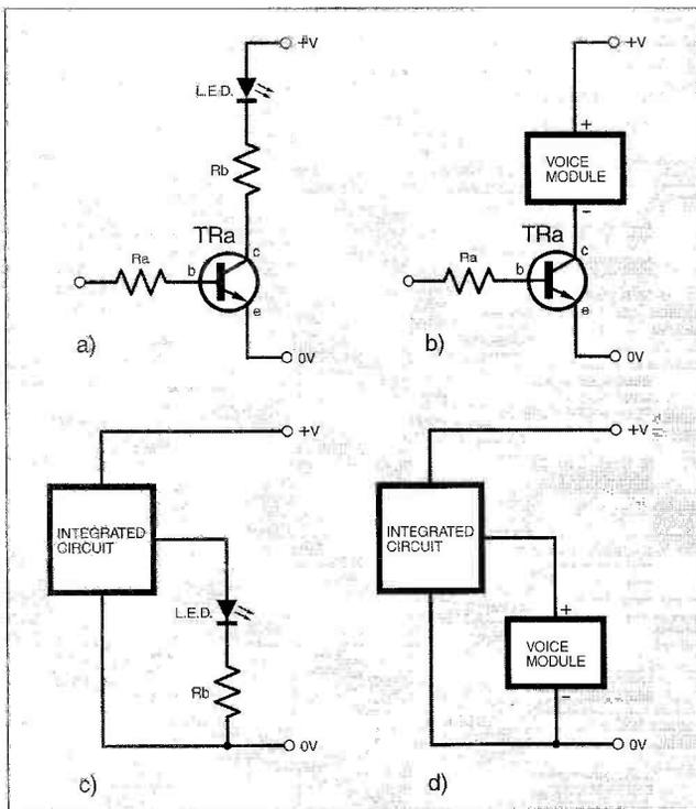
Fig. 6. Two examples of using the module in place of an l.e.d.
