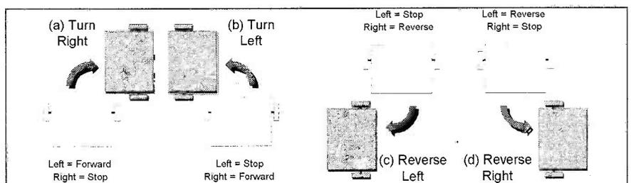
Fig.3: Cases where only one motor is active
