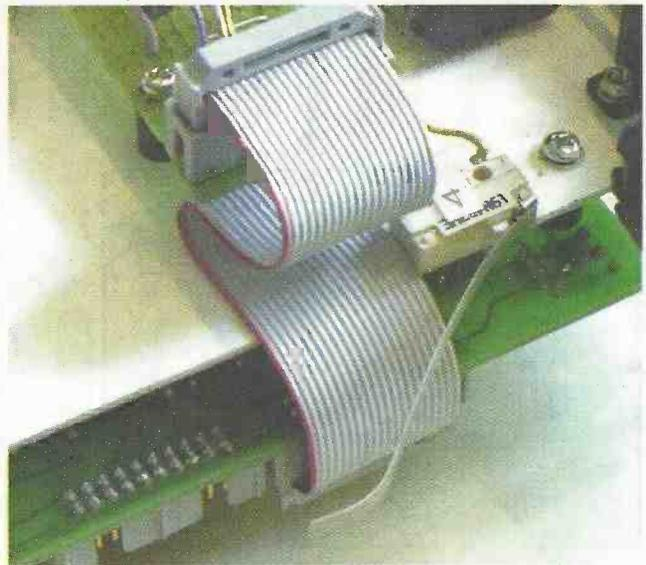
The ribbon cable for the motor controller needs folding to prevent it interfering with the microswitch.
