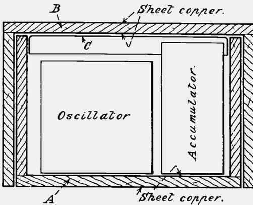
Fig. 2.—Simple screened oscillator.
