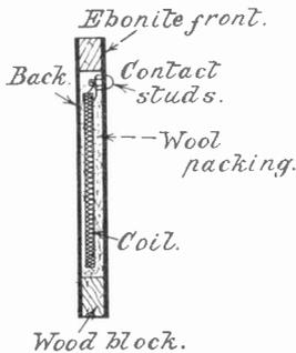
Fig. 4—Showing how the coil should be packed.
