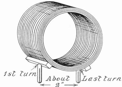
Fig. 5—Position of plugs on short wave coil.
