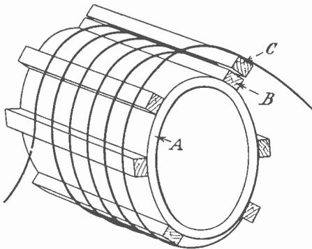
Fig. 4—A suitable method of coil construction for short waves.
