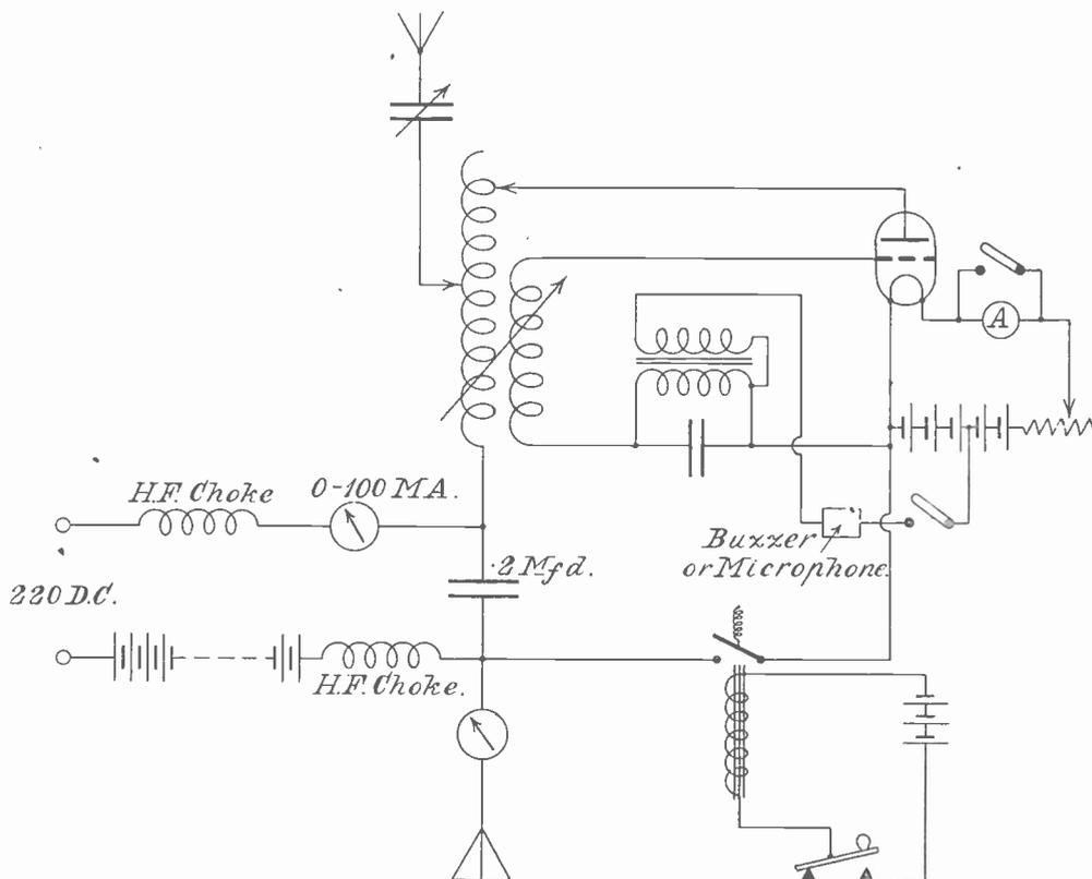
Fig. 2.—The transmission circuit showing method of keying.
