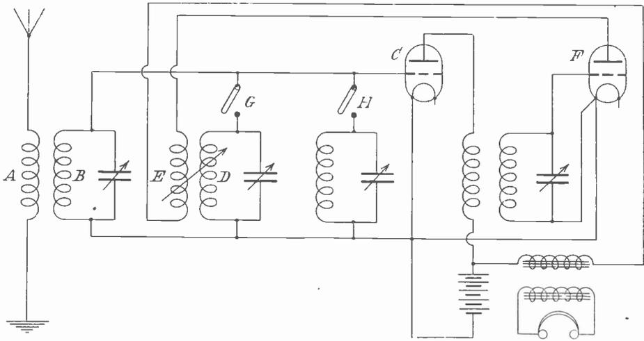
Fig. 3.—The fundamental principle of the Hinton rejektor system.
