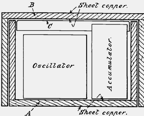
Fig. 2.—Simple screened oscillator.
