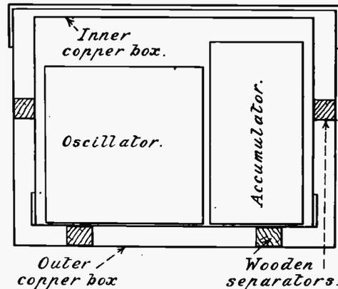
Fig. 1.—Triode oscillator screened with two complete copper boxes.
