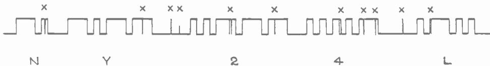
Fig. 5.—Sample of tape obtained from New Brunswick, U.S.A., (WII) with magnetic drum recorder. The rapidity of action of the instrument and the adjustment of the receiving circuit is such that the tape is not rendered illegible by atmospherics, automatic transmission taking place at 25 words per minute.
