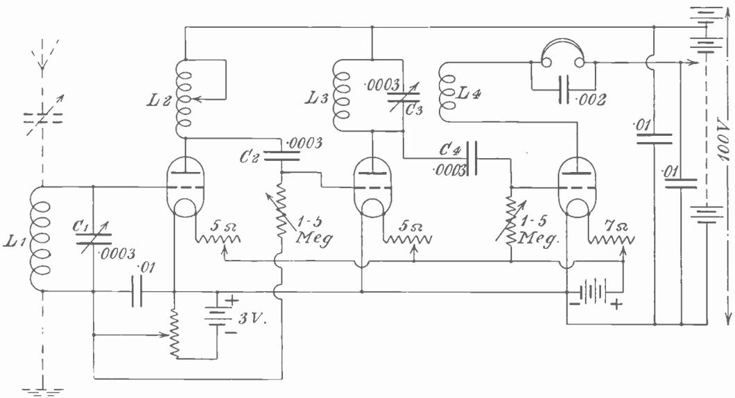
Fig. 6 - The circuit employed showing suitable valves for the components.
