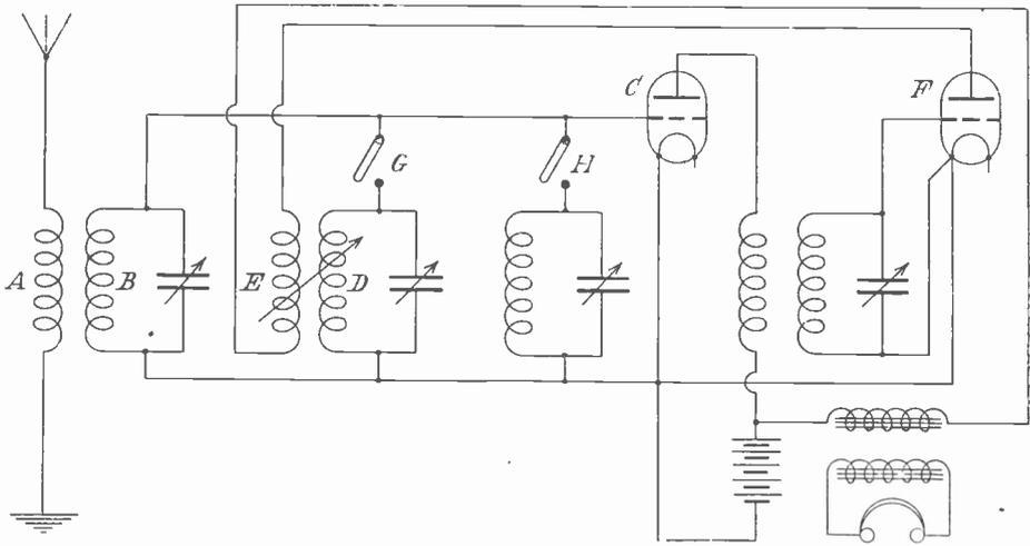
Fig. 3.—The fundamental principle of the Hinton rejctor system.
