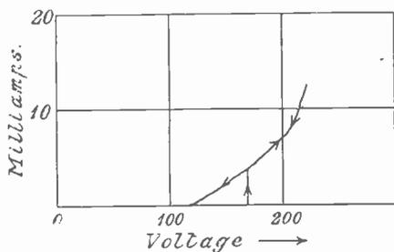
Fig. 1.—Typical characteristic of an "Osglim."
