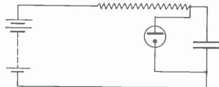
Fig. 2.—Circuit used for the generation of impulses.
