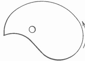
Fig. 2—Form of spade to give straight line tuning.
