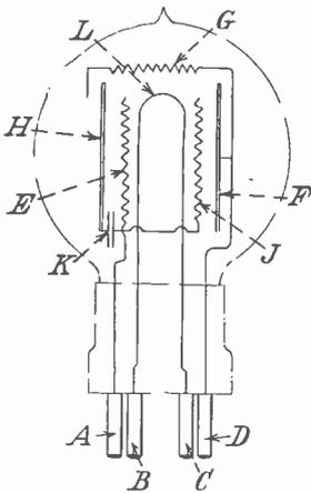
Fig. 4.—A "resistance capacity coupled" valve.
