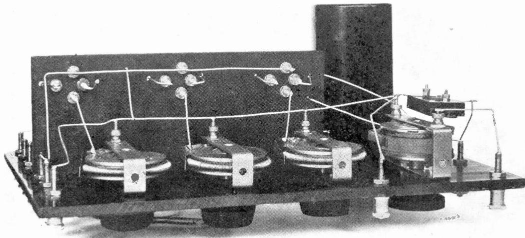
Fig. 8—Arrangement of wiring of the filament circuits beneath the valve panel.
