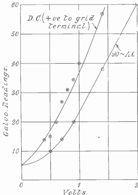
Fig. 1.—Calibration of Moullin voltmeter.
