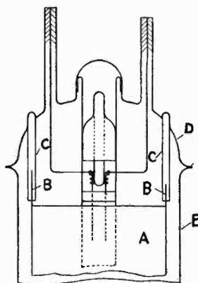
Patent No. 216,585 of C. Seymour, H. G. Hughes and T. E. Goldup deals with the construction of power valves of certain types in a manner to facilitate assembly. The anode supporting wires B are made of unequal length in order to facilitate their fitting into the supporting tubes C when the cap D of the envelope is being fitted to the main body E.
