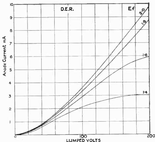
The valve was tested at 1.4, 1.6, 1.8 and 2.0V, on the filament, and its constants will be gathered from the accompanying table. The first exceptional point is the very large output, this being 10mA at the lower rated voltage, and no less than 19
