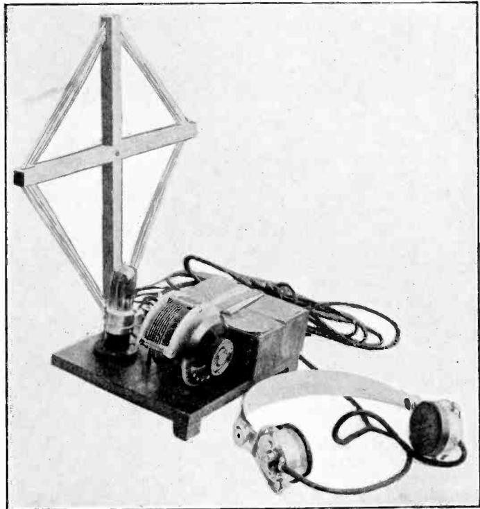
A "High-tensionless" Receiver: range 20 yards on 5XX1. It is used at Chelmsford as a test set.
