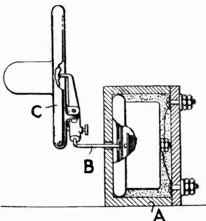
a gramophone "sound-box C. Thus telephonic vibrations produced in A are reproduced in the gramophone system. (Patent No. 213,936, R. E. B. Wakefield.)
