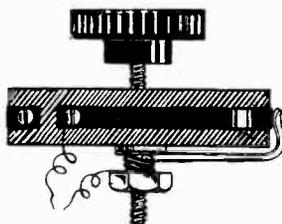
A piece of *passer-pout* makes an excellent grid-leak, and gives constant results. This material can be obtained from any good class stationers or photographic dealers at a very small cost.
