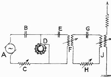
and D a frequency multiplier such as is common in long-wave high-power stations. Condenser E and transformer G form a system resonant to the desired frequency which serves to transfer the output of D at this frequency to the intermediate circuit and aerial system. We do not quite see where the novelty lies, however, in the mere use of an intermediate circuit.
