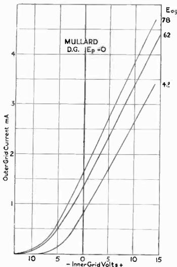
With the anode held at 0V, input to IG and output from OG, the valve behaved exceedingly well, as will be seen from Fig. 6. The
