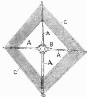
Clinker. The arms A of the frame are pivoted at their junctions to the central boss B so that they can be folded together when the frame is out of use. The mounting of the arms is so arranged that they open out a little beyond the position where they are in the same plane when the tension of the wires
