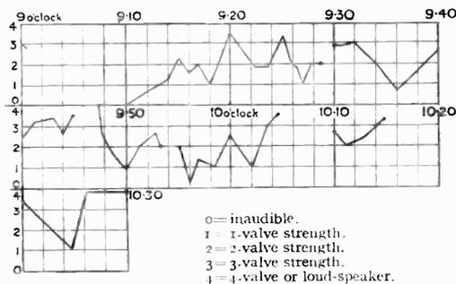
Long-distance reception over the earth's surface has problems of its own. Take, for example, fading, one of the bugbears apparently little is known about. Some nights fading is very pronounced from loud-speaker strength to inaudibility in, say, two minutes.
