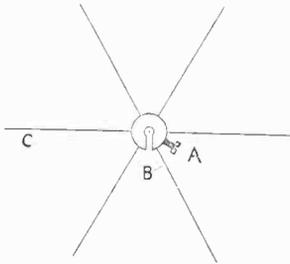
A boss B, adapted to be fixed on to an aerial wire by means of a set-screw A, carries a spike or number of spikes C, which act as discharging points to dissipate any electrostatic charge which may accumulate on the aerial.
