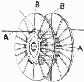
are separated by string in order to provide an air space between them. A former for use in constructing the coil is shown in the drawing.
