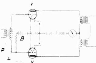
The explanation of the device as given by the inventor is as follows: When an alternating voltage is applied to the primary, the voltage on the secondary will, for half a wave, tend to make one grid
