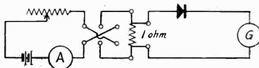
Fig. 2. Circuit for obtaining curves such as those in Figs. 1 and 3.
