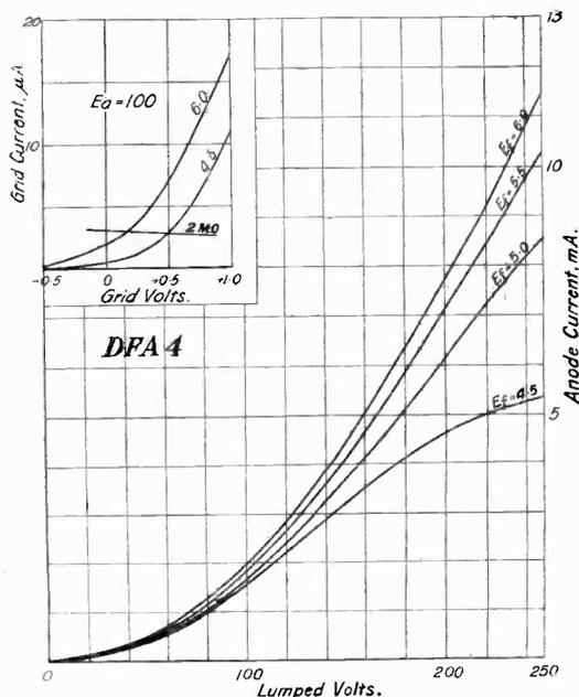
also rather below the average for valves with these filaments, being 30mA maximum instead of the usual 40. We are inclined to think that the filament of this sample had a resistance slightly above the average, and so was running cooler. The anode
