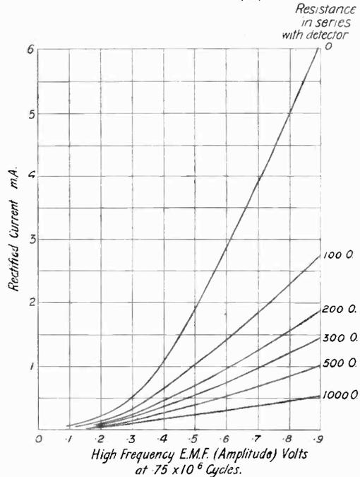
Fig. 9. Rectification characteristics for Galena with various loads.
