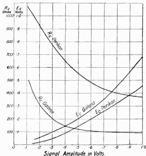
Fig. 13. Variation of  $E_c$  and  $R_c$  (apparent E.M.F. and internal resistance) for varying input voltage (large input).
