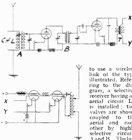
to use a wireless link of the type illustrated. Referring to the diagram, a selective receiver having an aerial circuit LC is installed; two valves are shown coupled to the aerial and each other by highly selective circuits A and B. The last
