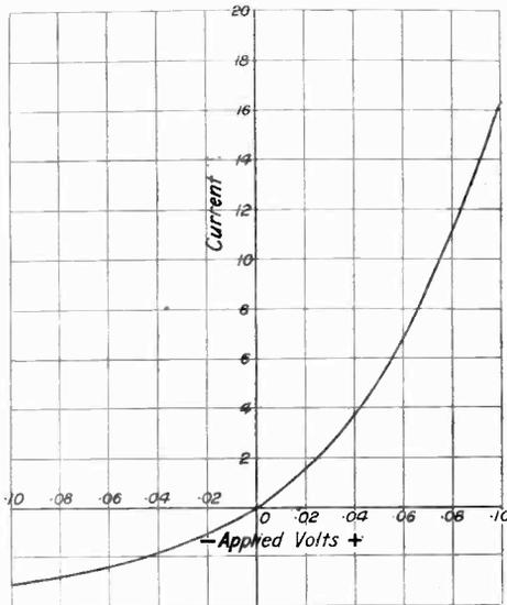
Fig. 3. A characteristic for very small input, the current is in microamps.
