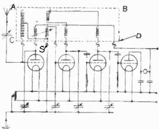
The invention also provides for a fixed magnetic reaction coil which is rendered operative electrostatically. The first claim of the patent is exceedingly broad and covers the use of a separate removable compartment containing all the high frequency coils. We were under the impression that we had seen a device of this nature several years ago, but, of course, we are open to correction.
