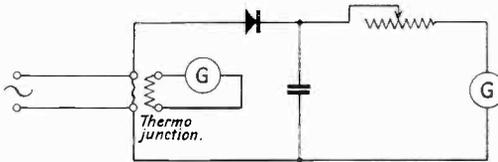
Fig. 8. The circuit used for measuring the "Rectification Characteristic" (D.C. output compared with H.F. input).
