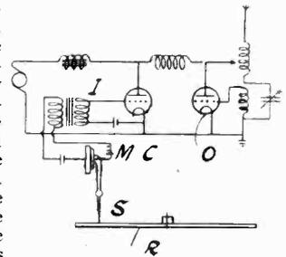
to control rather than to the transmission of intelligence and the record is arranged to transmit, when run at the correct speed, a predetermined series of acoustic signals. Interposed between the correct signals there are a number of interfering signals of various acoustic frequencies which renders the transmission unintelligible to any but authorised receiving stations.
