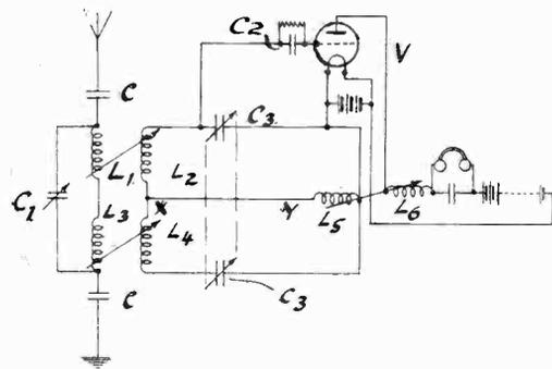
a reaction effect is obtained between  $L_2$  and  $L_5$  resulting in increased signals. Should oscillations be generated, it is stated that the currents being equal and of opposite phase in  $L_2$  and  $L_4$ , their combined induced effect in  $L_1, L_3$  in the aerial circuit will be substantially zero, or in other words there will be no radiation from the aerial.
