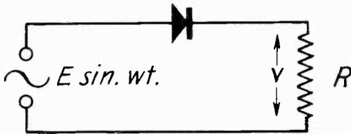
Fig. 5. The simplest output load.
