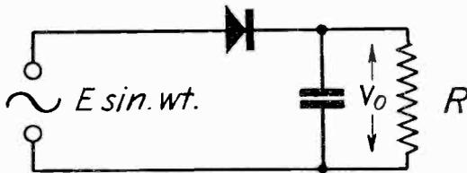
Fig. 6. As a rule the output load has a condenser to by-pass the high-frequency components.
