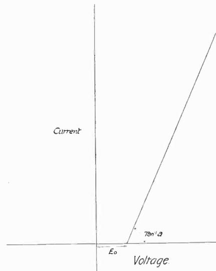
Fig. 4. At large amplitudes, the crystal characteristic approximates to a straight line.
