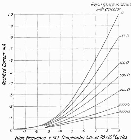
Fig. 10. Rectification characteristics for Perikon with various loads.
