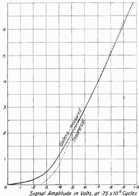
Fig. 12. The measured curve for large amplitudes approximates to that calculated on the basis of a simple straight-line law for  $i$  and  $e$ .
