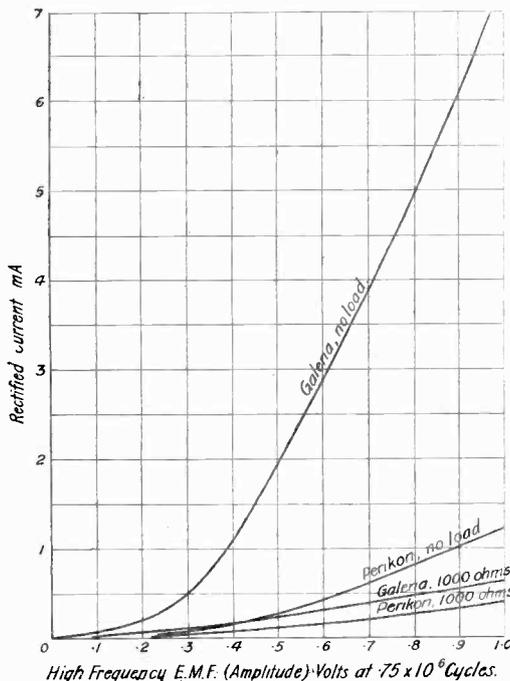
Fig. 11. Curves from Figs. 9 and 10 to the same scale, for comparison.
