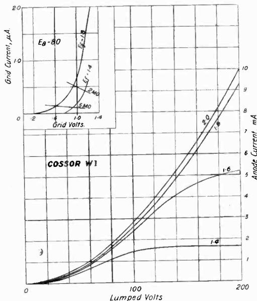
Our table shows the values of its constants at various filament heats; but we could not find all the saturation currents. On attempting to arrive at them, we simply caused a steady increase of current (at all filament heats above 1.6 volts) and found
