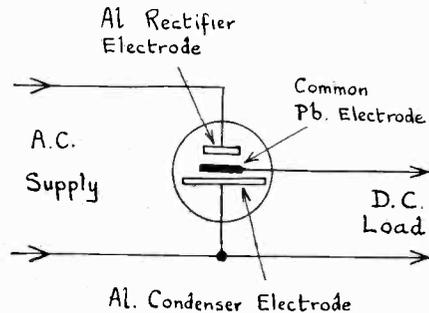
Fig. 6. Messrs. Siemens' Connection.
