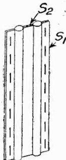
semi-circular channels, so that when the plates are placed together as shown, they form a double anode. The specification is very detailed, and describes several modifications, one modification being in the form of a cross, in which four channels are provided.
