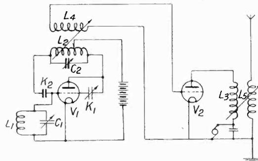
aerial coil  $L_5$ . Between the anode and the grid of the valve  $V_1$  is connected a variable condenser  $K_1$  of similar capacity to the coupled condenser  $K_2$ . It is stated that the regenerative coupling effect of the condenser  $K_1$  is equal and opposite
