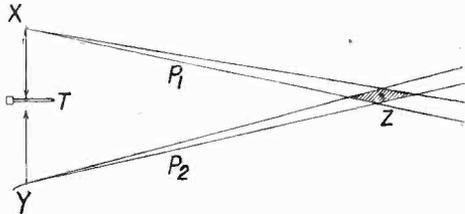
focusing the two beams on to the desired receiving point Z.
