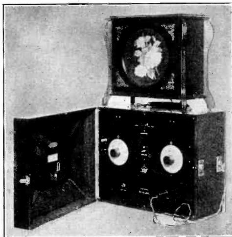
*A luxury portable set. That of the M.P.A. (Wireless), Ltd. The loud-speaker standing on it is manufactured under the Celestion patents.*
