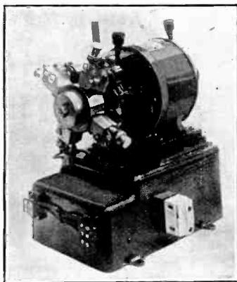
*One of the "M.W." rotary rectifiers for accumulator charging. Many types are made.*
