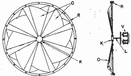
that although the diaphragm is formed of a number of sectors which vibrate more or less as a whole, owing to the fact that the sectors are combined rigidly near their point of actuation the maximum flexibility occurs at their extremities.
