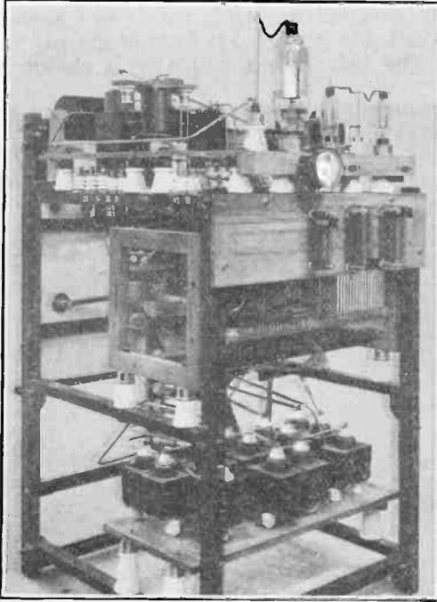
Fig. 6. Independent oscillator and modulating valves.
