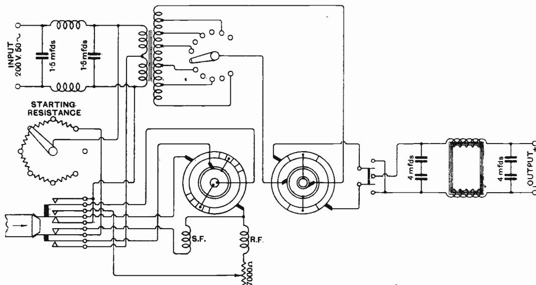
Fig. 10. *Simplified diagram of connections.*
