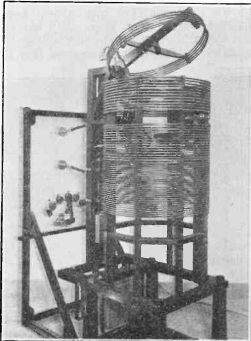
Fig. 8. Main anode coil and aerial coupling.
