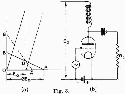
For the other type of circuit (Fig. 8b) altering  $R_e$  does not change the conditions in the valve so long as there is no alternating voltage on the grid. Hence in Fig. 8 when  $R_e$  only is altered the working line will swing about  $D$ , and the grid bias would have to be altered to make the working line pass through  $A$ .
