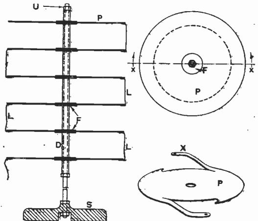
Durrant and K. I. Rayment. Essentially the aerial consists of a number of plates of appreciable area, supported co-axially one upon the other. Thus, in the accompanying illustration, a stand *S* is provided with an upright member *U* which
