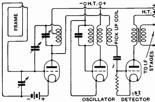
Fig. 5. Circuit showing method of neutralising.
