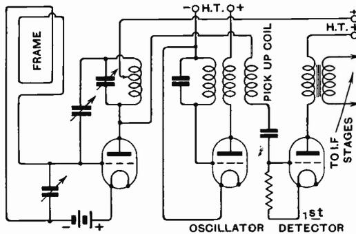
Fig. 5. Circuit showing method of neutralising.
