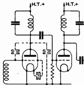
Fig. 1. Two circuits in cascade employing the neurodyne principle.
