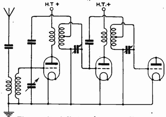
Fig. 2. Aperiodic transformer couplings.
