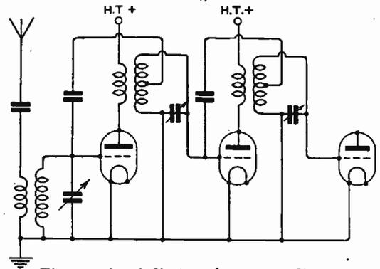
Fig. 2. Aperiodic transformer couplings.
