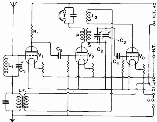
high frequency transformer to the rectifier, the output of which is fed back to the first amplifier. Thus, in the accompanying illustration it will be seen that the aerial circuit comprises an inductance *L*<sub>1</sub> and variable condenser *C*<sub>1</sub>, connected in the grid circuit of the first dual amplifier. The dual amplifier contains a resistance *R*<sub>1</sub> in the anode circuit, which is coupled by a .005 fixed condenser to the grid of the second valve *V*<sub>2</sub>. The anode
