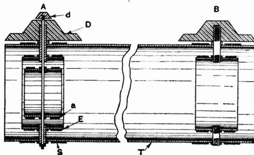
By this arrangement it is found easily possible to couple the two variometers together. The specification also provides for the use of one of the windings as a reaction coil.
