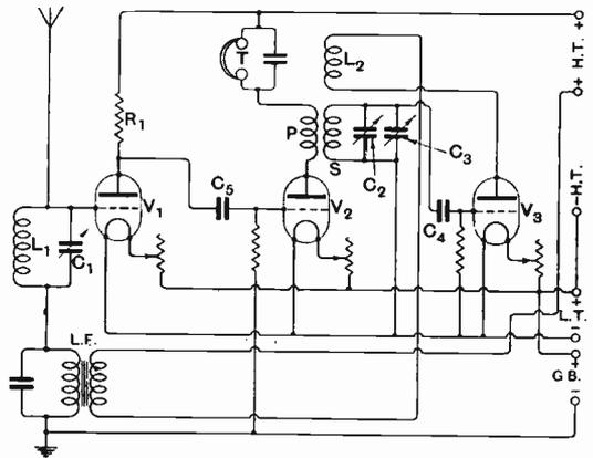
high frequency transformer to the rectifier, the output of which is fed back to the first amplifier. Thus, in the accompanying illustration it will be seen that the aerial circuit comprises an inductance  $L_1$  and variable condenser  $C_1$ , connected in the grid circuit of the first dual amplifier. The dual amplifier contains a resistance  $R_1$  in the anode circuit, which is coupled by a  $.005$  fixed condenser to the grid of the second valve  $V_2$ . The anode
