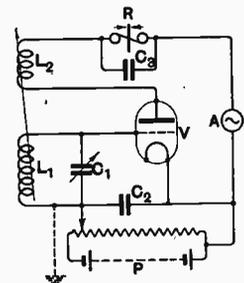
the grid and the filament with the result that the grid will become more positive on the positive half cycles. This increase of positive potentials is sufficient to cause the valve to oscillate when the valve is positive with respect to the filament. As soon as the valve commences to oscillate there
