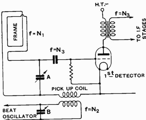
Fig. 3. Theoretical diagram of superheterodyne.
