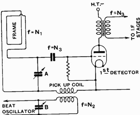
Fig. 3. Theoretical diagram of superheterodyne.
