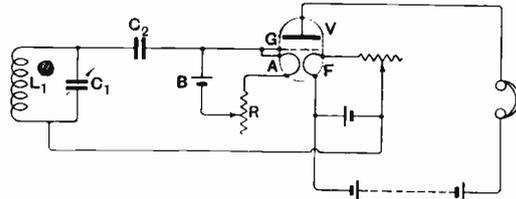
seen that if the filament *A* is heated it will emit electrons which will thus enable the charge which is collected on the grid to leak away to the main filament. In other words, the auxiliary filament *A* acts as the grid-leak of the arrangement, and the value of the grid-leak can be varied by controlling the rheostat associated with the auxiliary filament. In a modification of the invention, the second filament is used as the grid or control electrode.
