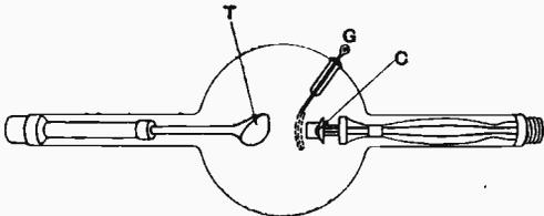
of the Coolidge type is shown, in which  $T$  is the target and  $C$  the cathode which is heated in the normal manner. A grid  $G$  is interposed between the cathode  $C$  and the target  $T$ , so that potential variations applied between the cathode and the grid will control the intensity of the rays which are emitted, thus causing a variation in the effect on the florescent screen, or other device which may be employed.
