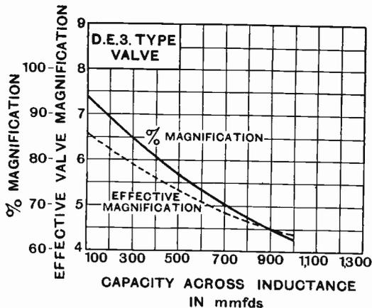
Fig. 9. Showing decrease in magnification with increase in capacity at a given wavelength, the inductance being gradually reduced as the condenser is increased (D.E.3 valve).
