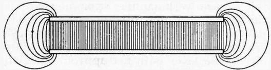
Fig. 1. Showing the distribution of the lines of force between the charged plates of a condenser.
