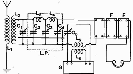
reception employing a low pass filter. The specification mentions that with ordinary heterodyne reception it is possible to obtain more than one adjustment of the local oscillator for any desired beat note, thereby resulting in confusion.
