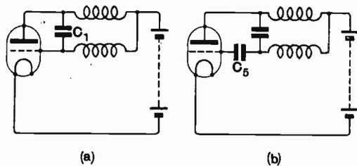
Fig. 4. Showing (a) Fig. 3 with  $C_4$  infinite and (b) a condenser  $C_5$  to prevent polarisation of the grid by the H.T. battery.
