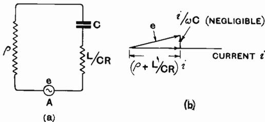
Fig. 7. Showing that at resonance the tuned anode combination is equivalent to a condenser  $C$  in series with an inductionless resistance  $L/CR$ , the whole being in series with E.M.F.,  $e$  and valve resistance  $\rho$ .
