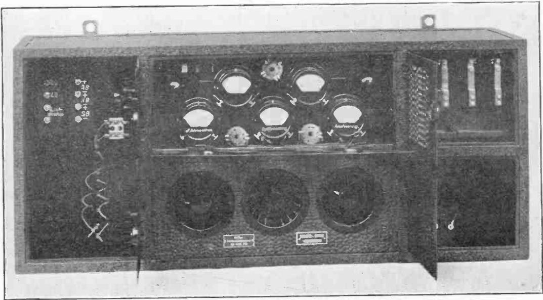
Fig. 19. *Transmission-modulation meter.*
