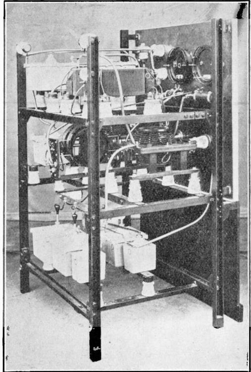
Fig. 12. Back view of panel for control of main anode and aerial currents.
