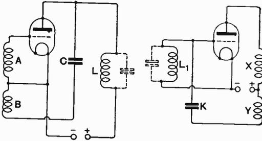
is connected directly between the anode and the H.T., and the other winding  $Y$  is connected to the grid through a capacity. Here, again, the capacity  $K$  forms the major portion of the capacity in shunt with an inductance  $L_1$ , connected, of course, this time in the grid circuit. This circuit should prove of interest to experimenters, and it is found to be very satisfactory in practice.
