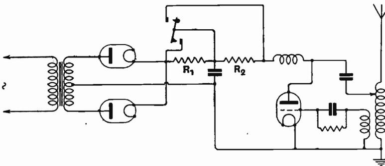
Fig. 3. A keying circuit in which the valve can oscillate weakly during the spacing intervals.
