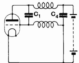
Fig. 3. A well-known short wave circuit for generating oscillations. The circuit is identical with Fig. 2 if  $C_4$  is large and if  $C_2$  and  $C_3$  are omitted from the latter figure.
