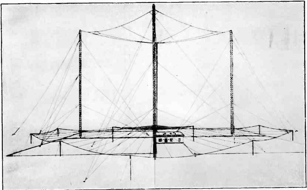
Fig. 4. Schematic view of aerial and counterpoise.
