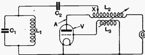
proportional to the number of turns of the inductance  $L_3$  between the anode and the connection  $X$ . In other words, the choke or inductance  $L_2$  functions in the manner of a step-down auto-transformer. In order that the system shall generate oscillations an inductance  $L_3$  is connected between the grid and filament of the valve, and is coupled to the inductance  $L_2$ . The specification is fairly detailed and contains several modifications of the scheme.
