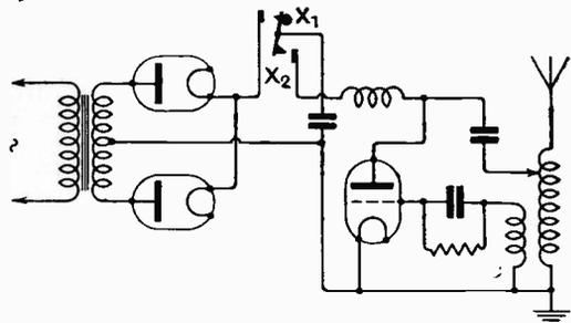
Fig. 1. *A plate keying circuit used on primitive transmitters.*
