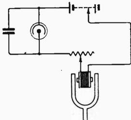
The method may be used for generating electrical oscillations of exceedingly constant frequency or for receiving wireless signals by the heterodyne method or for calibrating wavemeters.
