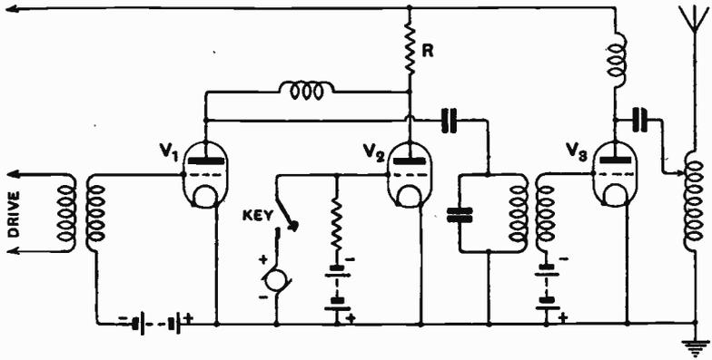
Fig. 9. Keying method applicable to high power transmitters.  $V_1$  is the intermediate magnifier,  $V_3$  the main magnifier, and  $V_2$  the absorbing valves.
