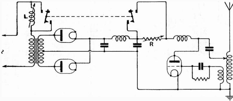
Fig. 4. Another keying circuit which produces a spacing wave.
