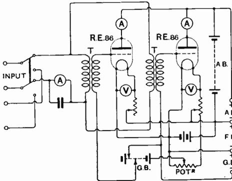
Fig. 21. Connections of the transmission-modulation meter.
