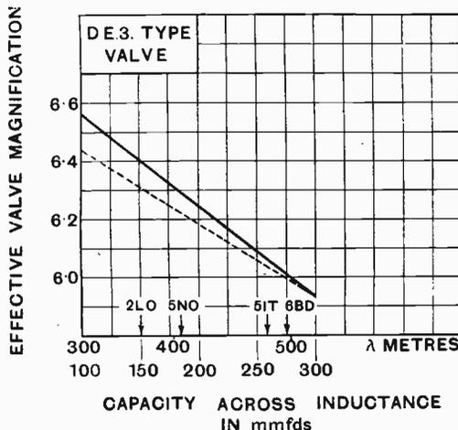
Fig. 8. Showing decrease in magnification with increase in wavelength (due to increase in capacity of anode tuning condenser). Calculated for D.E.3 valve for which  $m = 7$  and  $\rho = 22,000$  ohms.
