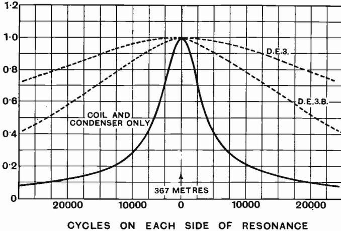
Fig. 10b. Showing relative selectivity curves of tuned anode with and without valve damping.
