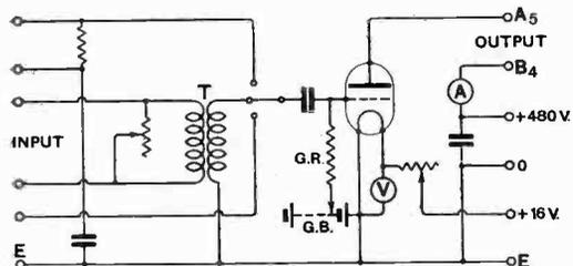
Fig. 16. Connections of the additional 4th stage amplifier.
