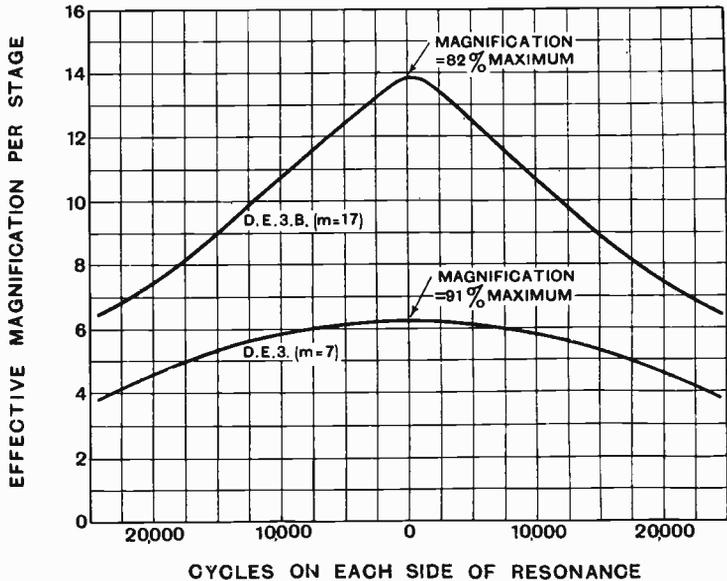
Fig. 10a. Showing magnification curves for tuned anode with D.E.3 and D.E.3B valves.
