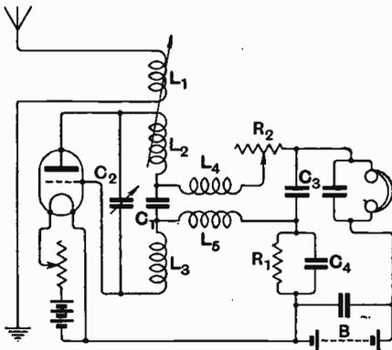
circuit contains an inductance  $L_1$ , tightly coupled to a split inductance  $L_2 L_3$ , tuned by a variable condenser  $C_2$ , the split inductance being connected by a fixed condenser  $C_1$ . Inductance  $L_4$  and  $L_5$  constituting the inductance of the quenching circuit, are associated with a condenser  $C_3$ . The lower
