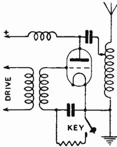
Fig. 6. Method suitable for small power transmitters using an independent drive.
