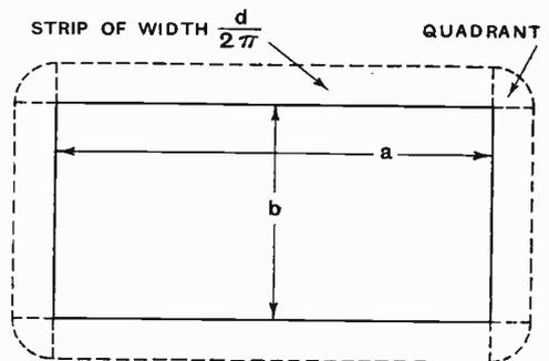
Fig. 3. Showing the effective size of a rectangular condenser plate.
