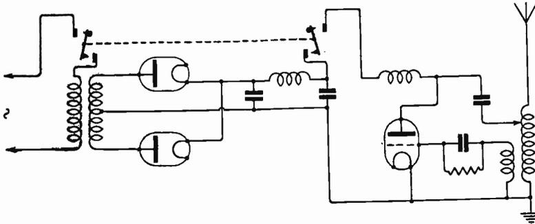
Fig. 2. Simultaneous keying of primary and plate currents.
