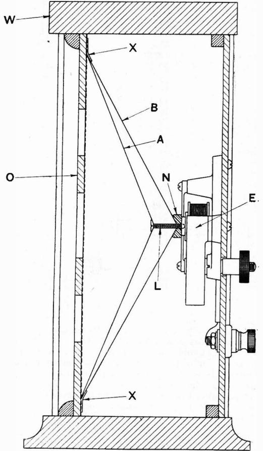
plug  $N$  to which they are joined by a screw  $L$ . This screw communicates with an ordinary electromagnetic system  $E$ , such as a telephone receiver, which is used to energise the cones. It is stated that the cones may be made of paper, parchment, thin wood, or metallic foil.
