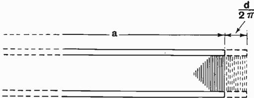
Fig. 2. Showing how the edge effect may be allowed for in calculations by assuming an increase  $d/2\pi$  in the length of the condenser plate.
