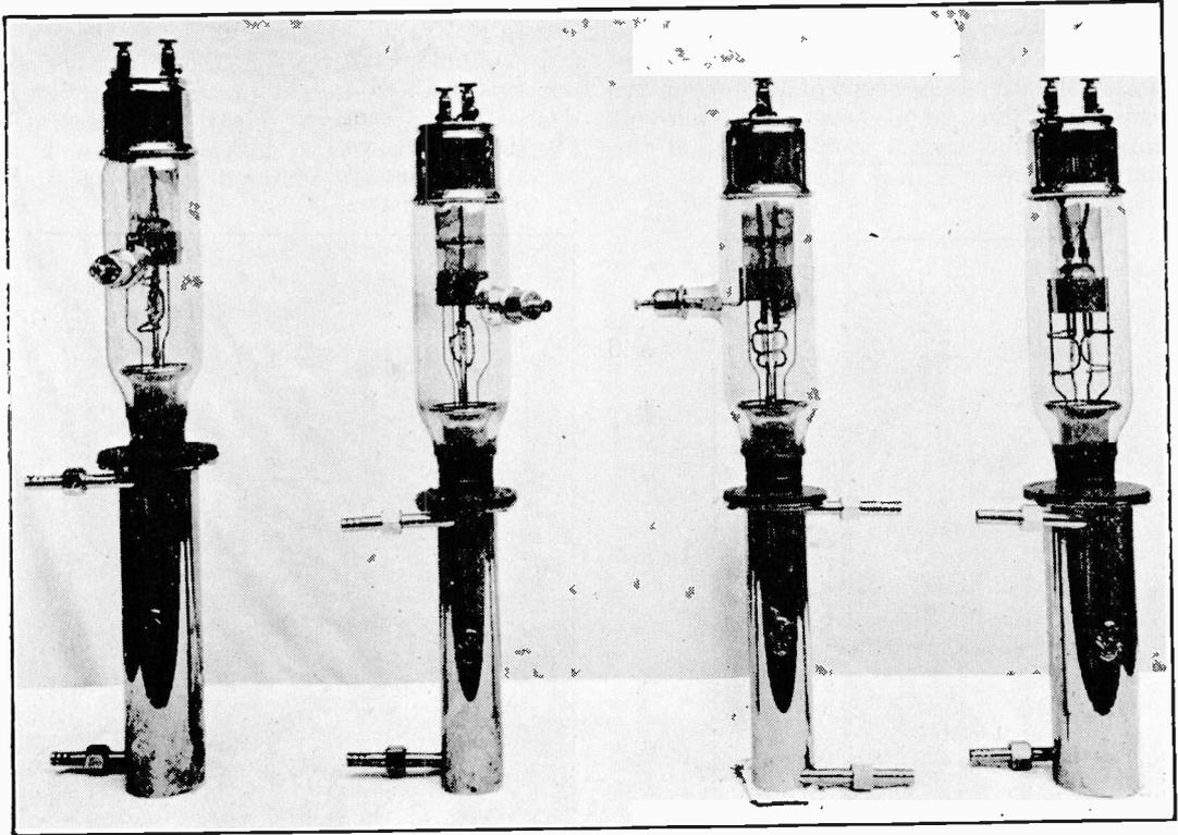
Fig. 9. Water-cooled power valve RS204.
