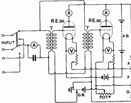
Fig. 21. Connections of the transmission-modulation meter.
