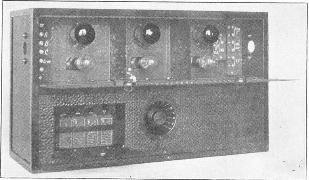
Fig. 13. Three-stage microphone amplifier.
