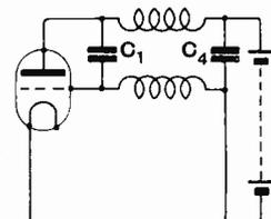
Fig. 3. A well-known short wave circuit for generating oscillations. The circuit is identical with Fig. 2 if  $C_4$  is large and if  $C_2$  and  $C_3$  are omitted from the latter figure.
