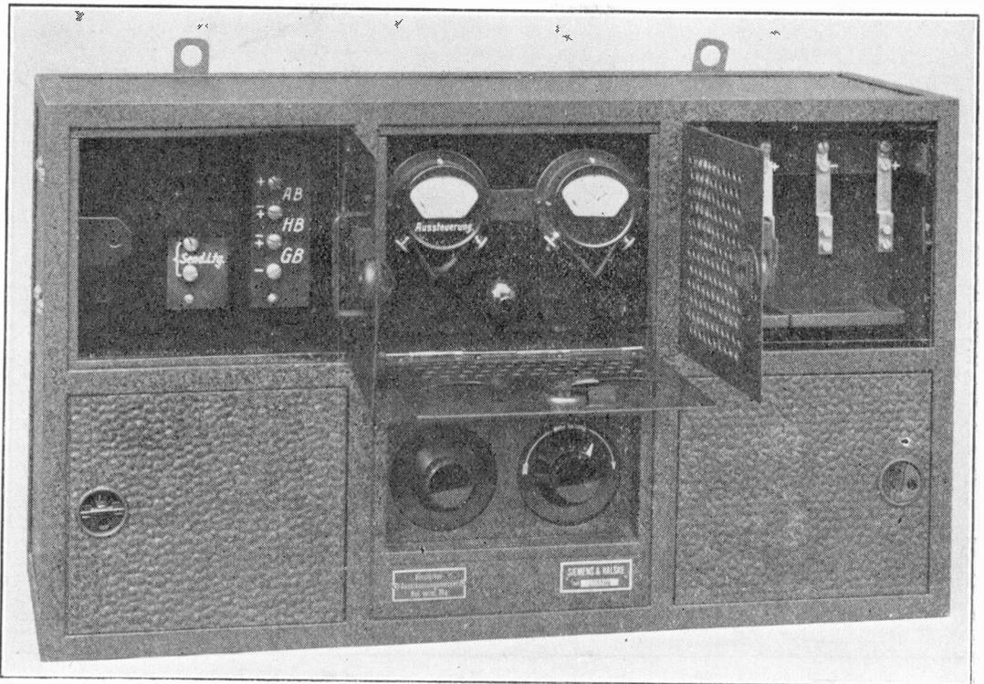
Fig. 17. *Amplifier modulation meter.*
