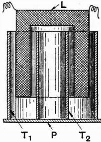
$T_1$  and  $T_2$  joined by a plate  $P$ , the tubes and the plate preferably being of copper. The inductance  $L$  is arranged so that its windings are between the two tubes, and means are provided for varying the tubes in relation to the inductance. It is stated that the two tubes act in the manner of a Faraday cage.
