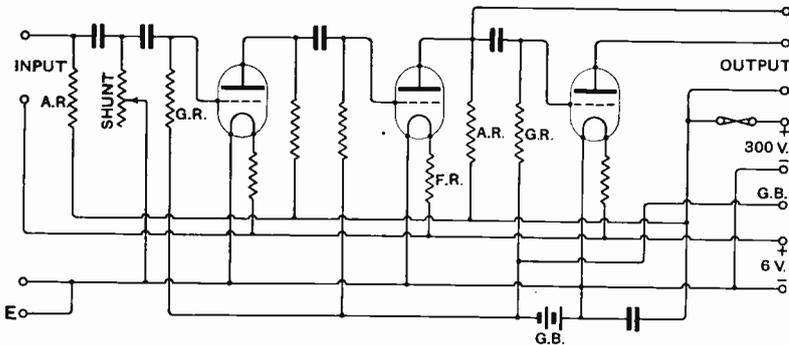
Fig. 14. Connections of the 3-stage microphone amplifier.
