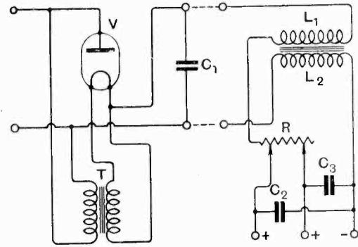
manner, and an integrating condenser *C*<sub>1</sub> is connected before the chokes. The remainder of the filter circuit is constituted by another condenser *C*<sub>2</sub> across two chokes *L*<sub>1</sub> and *L*<sub>2</sub> in each lead respec-
