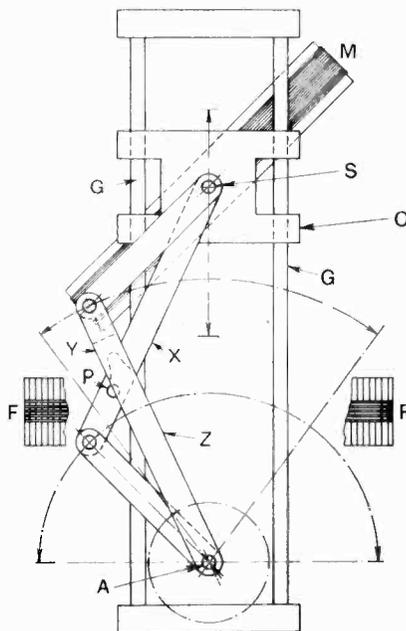
in the link arm X engages a guide plate Y on the link arm Z, and carries it over the top dead centre in a direction depending upon the rotation of the spindle A.
