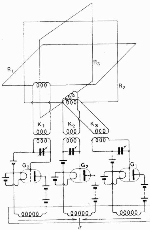
is independent of the angle of incidence of the arriving waves and their state of polarisation, since the continual changes in the direction of polarisation and angle of incidence of the incoming waves can cause marked variation of the signals being transmitted.
