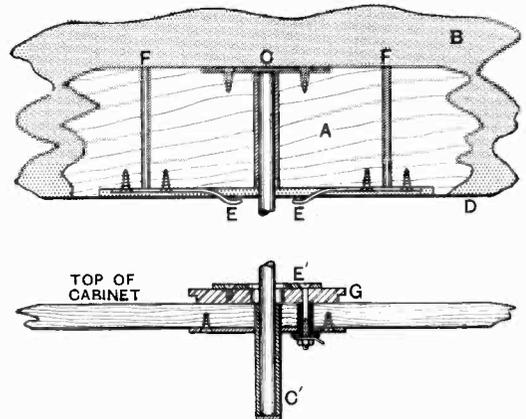
Fig. 40. Details of the combined spindle and contact arrangements for the frame. {The disc G is undercut to take the compass card.
