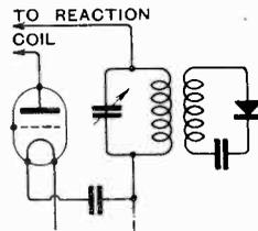
Fig. 25. An obvious reaction circuit, but not likely to be successful.
