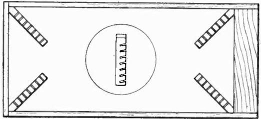
Fig. 39. The general design of the frame-lid: in the circle, a side view of one of the combs.
