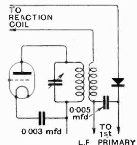
Fig. 26. This is a more satisfactory reaction arrangement than that of Fig. 25, but it is still by no means the best.
