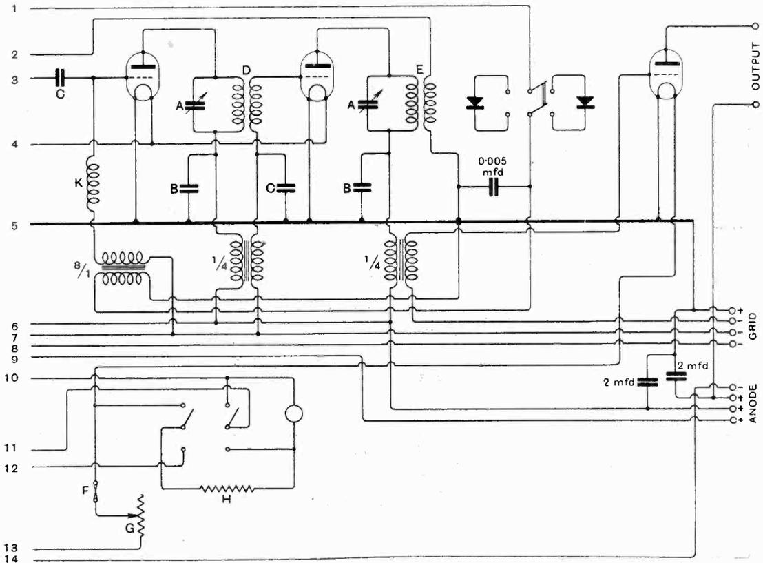
B, .003 $\mu\text{F}$ ; C, .0003 $\mu\text{F}$ ; D, McMichael air-core, No. 3; E, As "D." but secondary rewound to  $\frac{1}{2}$  turns; F, Burndy fixed resistor in holder; G, Filament rheostat; H, Series resistor for meter; K, 1,800 or 1,500 coil of low self-capacity; L, Variable leak. 1-5MO; M, McMichael "Autodyne" unit; N, McMichael reactor.
