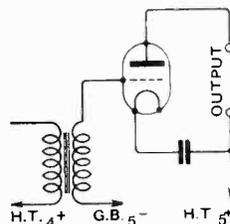
Fig. 28. As a matter of form, the power valve circuit is given, although it is of standard type.
