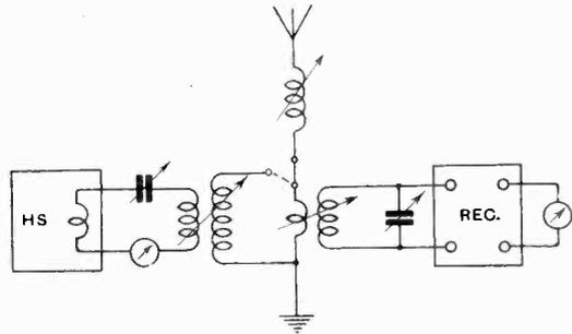
by the receiving signal, as indicated by the meter in the output of the receiver. Then knowing the ratio of transformation of the current transformer it is possible to determine antenna currents which do not allow of direct measurement.
