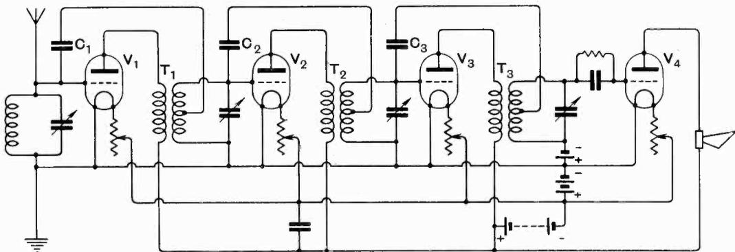
the primary of a transformer  $T$ . The tuning condenser  $C_2$  and balancing condenser  $C_3$  are mechanically linked so that any variation of the tuning condenser effects a desired change in the balancing condenser. A further feature of the
