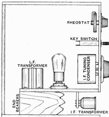
Fig. 30. The arrangement of the intermediate stages. All these components are centred on the same line.
