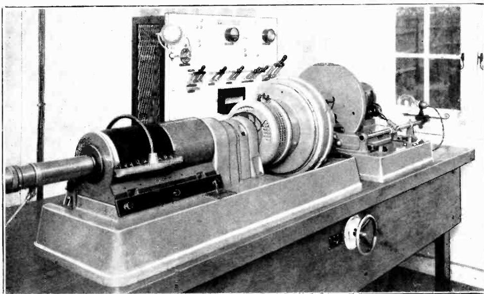
*Picture transmitting equipment. The tube on the left carries the dispersed light from the image to the photoelectric cell.*
