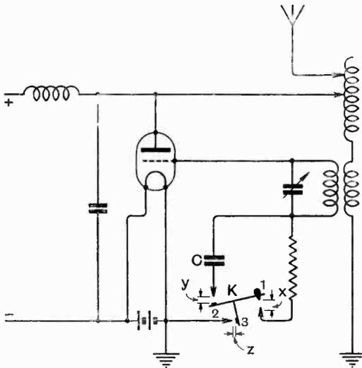
broken in a definite sequence. On breaking, the leak-resistance branch is opened first, and afterwards the branch containing a grid condenser; whilst in making, the condenser branch is closed
