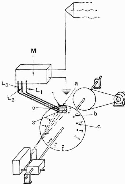
separate sets of spirally-staggered holes *a*, *b*, *c* are used to analyse simultaneously three distinct segments 1, 2, 3 of the object being televised. The relative setting of the spiral series of holes *a* is such
