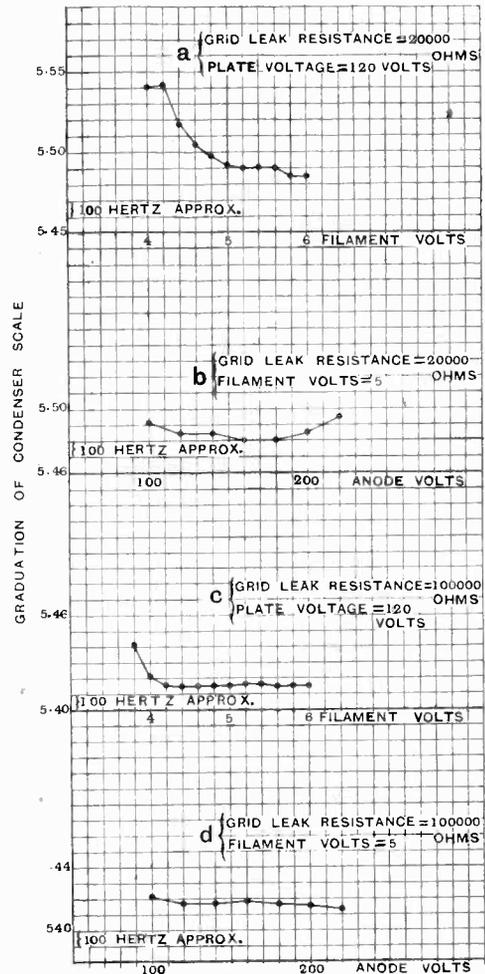
Fig. 4.—Curves showing the variation of calibration of the heterodyne wavemeter as a function of low-tension and high-tension voltages for a grid leak resistance of 20,000 ohms and 100,000 ohms.
