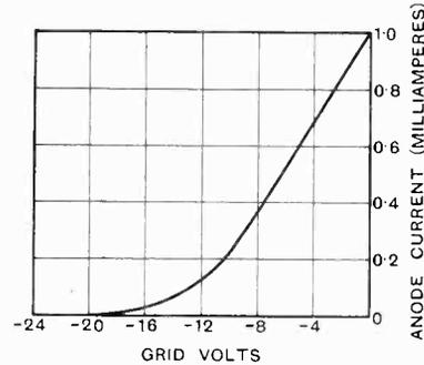
Fig. 12.—Characteristic for PM3 with anode resistance of 130,000 ohms.
