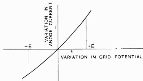
Fig. 2b.—Relation between changes in grid potential and changes in anode current.
