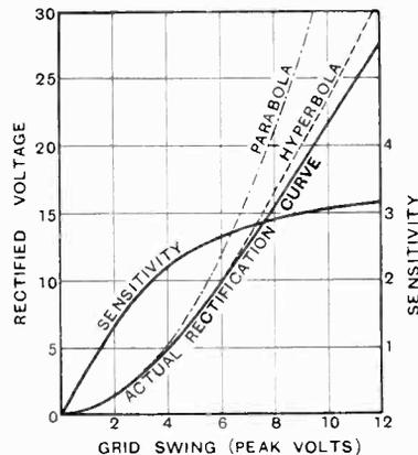
Fig. 9.—Rectification curve for PM3 valve,  $R = 130,000$  ohms, voltage about 190. The parabola most closely approximating to the curve for small values of the grid swing is also shown. The general features of the curve are more nearly those of an hyperbola, which is also shown. It is seen that for small grid swings the sensitivity is practically proportional to the swing. As the swing increases, however, the sensitivity approaches a limiting value.
