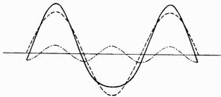
Fig. 5.—The full line curve represents the output of the rectifying valve for a heavily modulated carrier when the relation between the rectified voltage and the amplitude of the carrier wave is not rectilinear. The two dotted curves show the principal components of the wave, one the true tone, the other an alien tone of double frequency.
