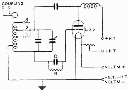
Fig. 2.—Diagram of connections of the heterodyne wavemeter.
