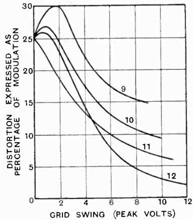
Fig. 16.—Showing variation of the distortion characteristic with the grid bias. The corresponding grid bias (in volts) is indicated on each curve.
