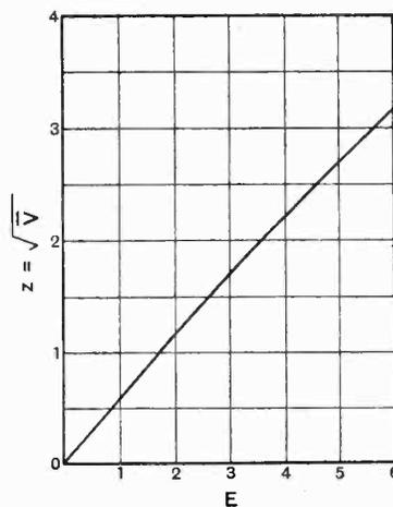
Fig. 17.—This curve represents another way of graphing the relation represented in Fig. 9 by the lower part of the hyperbola. From such a curve, approximating as it does to a straight line,  $\frac{dV}{dE}$  can be determined with much greater accuracy than it can from the original hyperbola.
