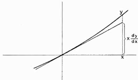
Fig. 6.—For small values of  $x$  the tangent is a sufficient approximation to the curve and  $y$  may be assumed equal to  $x \frac{dy}{dx}$ . As  $x$  increases it becomes necessary to allow for the fact that  $\frac{dy}{dx}$  is changing.
