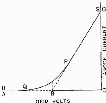
Fig. 8.—Characteristic of rectifying valve. It is seen that as grid swing increases the effective deviation from the ideal ABC diminishes.
