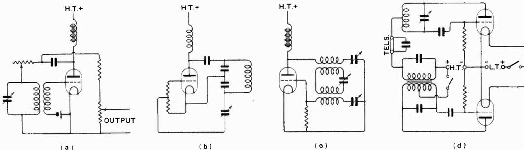
(a) Horton's Oscillator; (b) B.B.C. Master Oscillator; (c) Fromy's Oscillator; (d) Colebrook's Modulating Wavemeter.
