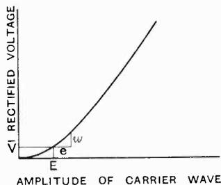
Fig. 3a.—Relation between rectified voltage and amplitude of carrier wave.
