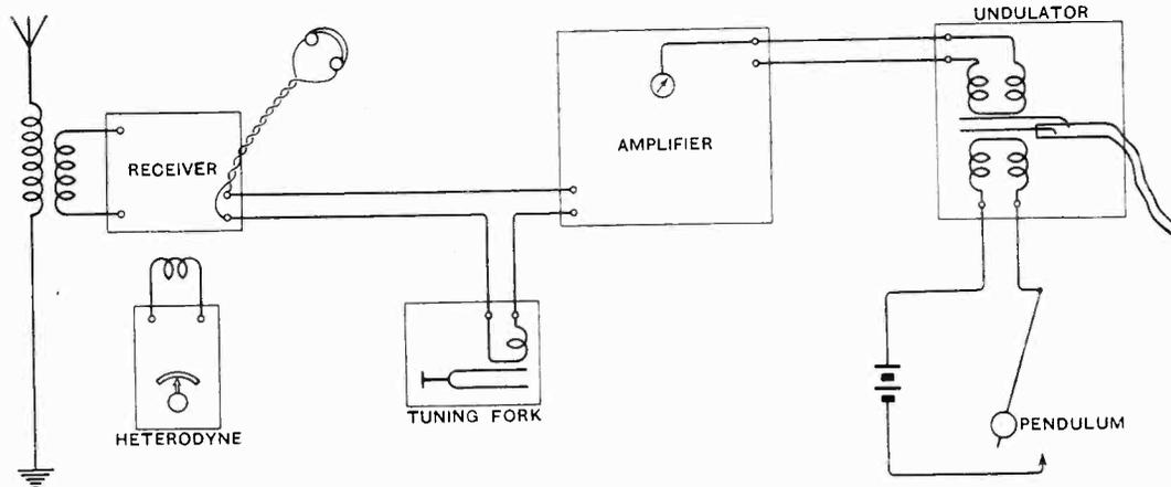
Fig. 8.—Diagram of connections of the apparatus for recording scintillation (frequency modulation).
