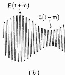
(b) Fig. 4b.—Modulated carrier wave.
