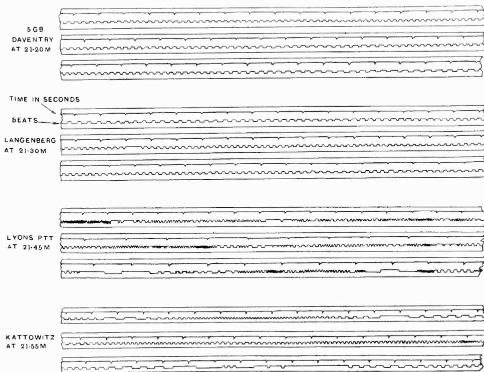
Fig. 9.—Examples of scintillation records for 4 different stations.
