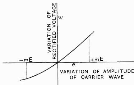
Fig. 3b.—Relation between changes in amplitude of carrier wave and variation of rectified voltage.
