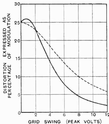
Fig. 14.—Showing reduction of distortion with increasing grid swing, grid bias 12 volts. The full curve shows the actual distortion; the dotted curve is the distortion calculated for a hyperbolic rectification curve (see Figs. 9 and 10).
