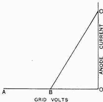
Fig. 7.—Ideal characteristic for rectification (after McLachlan).
