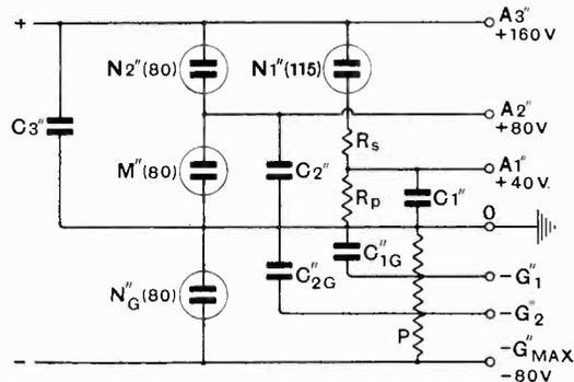
tions, oscillation and distortion, owing to the effect of change of load. Schröter has patented a method of avoiding such voltage fluctuations by the use of a glow-discharge tube in a parallel connection, but the writer points out objections to this plan (*e.g.*, the impossibility of making the grid voltages independent of the fluctuations) and advocates instead the substitution of similar tubes for the usual ohmic resistances.
