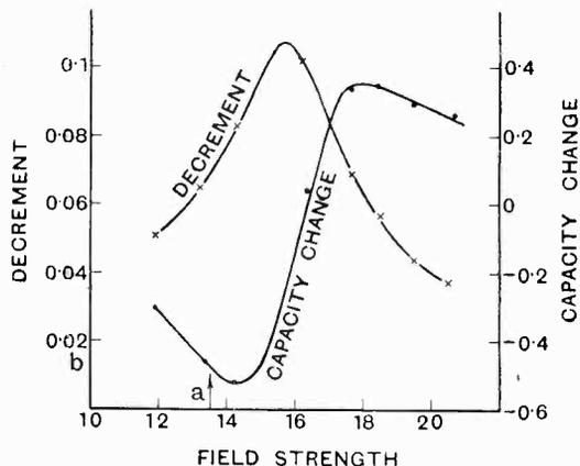
Fig. 2.—Experimental. a. Field strength at which the electron frequency = field frequency. b. Decrement for cold cathode.
