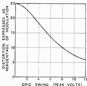
Fig. 10.—Showing reduction of distortion with increasing grid swing—hyperbolic rectification curve (see Fig. 9).
