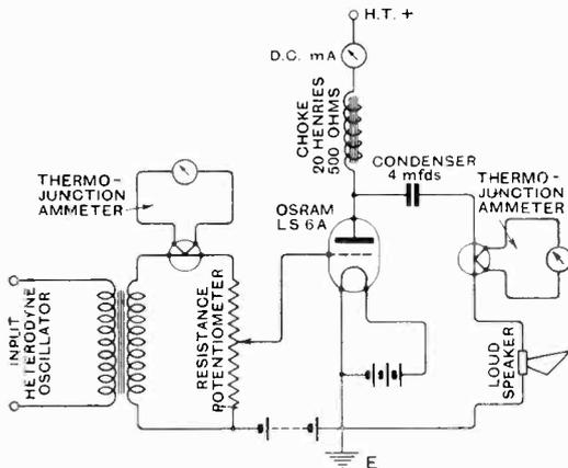
Fig. 9.—Power stage and loud speaker circuit diagram.
