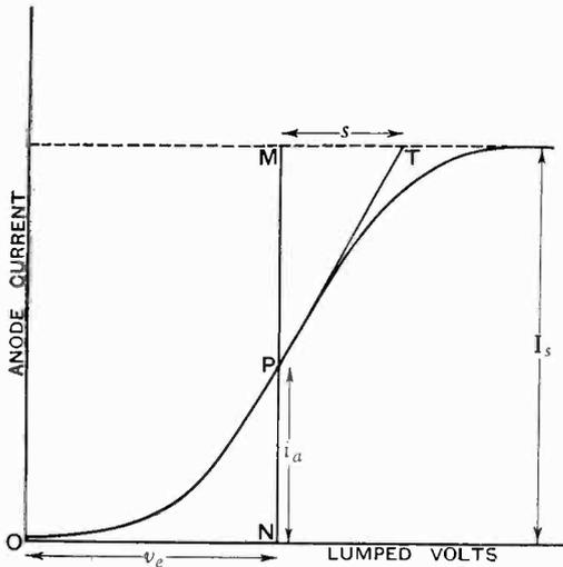
Fig. 1.—Derivation of  $s$  from lumped characteristic.
