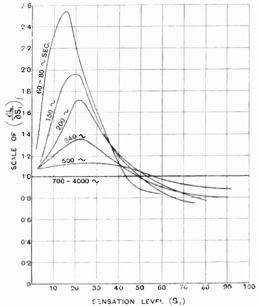
Fig. 6.—Variation of rate of change of loudness with sensation level at different frequencies.
