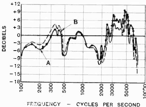
Fig. 7.—Response curves for moving coil loud speaker.
