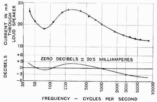
Fig. 8.—Variation of current with frequency through moving coil loud speaker.
