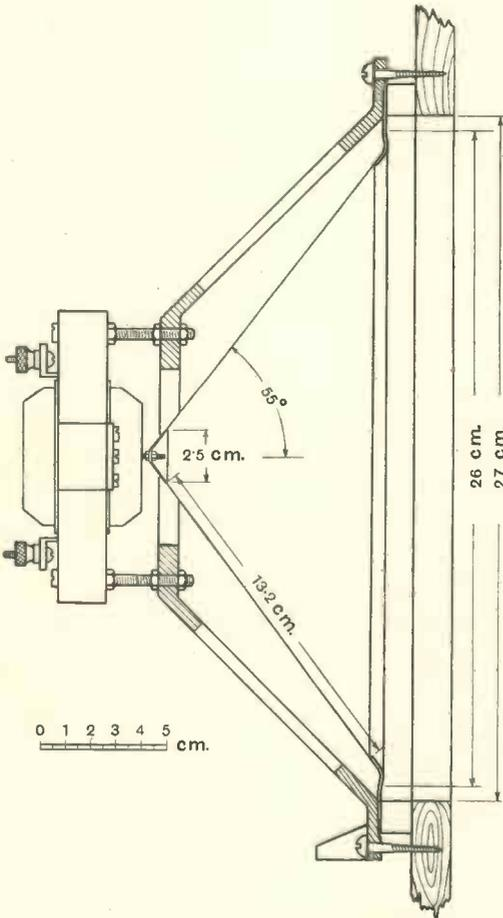
Fig. 1—Section of Inductor Loudspeaker showing principal dimensions.
