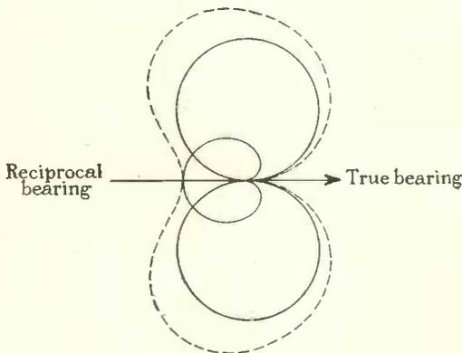
Fig. 1.—Addition of a cardioid to a figure-of-eight quadrature.
