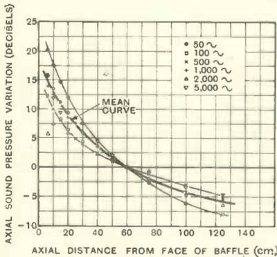
Fig. 6.—Axial sound pressure variation with distance for constant loudspeaker current.
