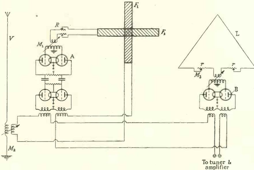
Fig. 4.—Circuit diagram of radio compass.
