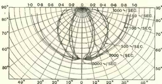
Fig. 3.—Measured polar curves of relative pressures for cone at several frequencies.
