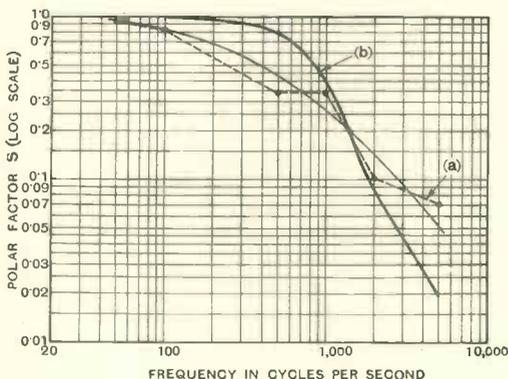
Fig. 9.—Polar factor variation with frequency, showing (a) Measured values for the cone, and (b) Calculated values for the rigid piston. ( $D = 26$  cm.).
