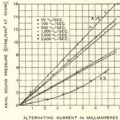
Fig. 7.—Axial sound pressure variation at 60 cm. with alternating current to loudspeaker.
