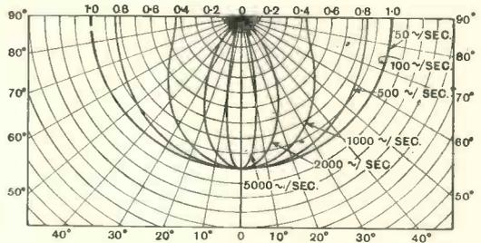
Fig. 8.—Calculated polar curves of relative pressures for rigid piston ( $D = 26$  cm.) at several frequencies.
