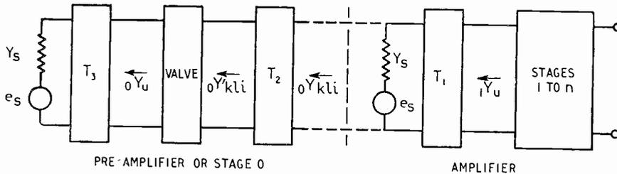
Fig. 7. The use of a pre-amplifier modifies the conditions for the following stage.
