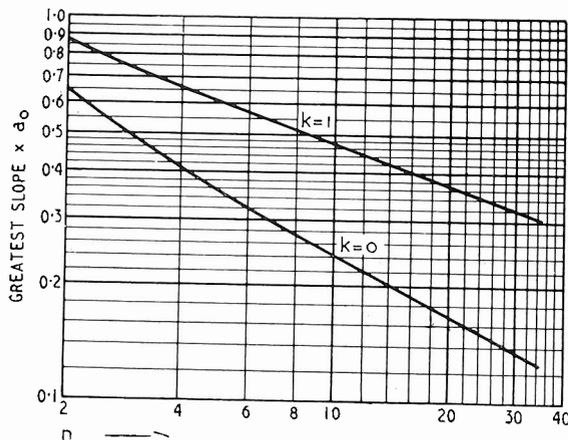
Fig. 5. The greatest slope of the modulation ratio (F.M.) for various numbers of circuits.
