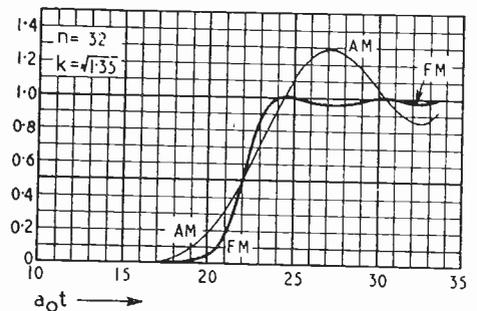
Fig. 3. The modulation ratio for amplitude and frequency modulation for a particular case of staggered circuits.
