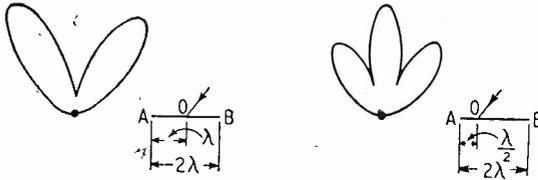
Figs. 9 and 10. *Experimental polar diagrams of transmitting aeriels. AB represents the aerial, and O the point of connection to transmitter.*
