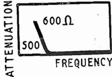
The thickened line in the pass-band shown in the derivation is unnecessary and merges into the boundary of the symbols.
