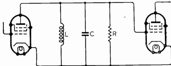
Fig. 1. A typical amplifier stage.
