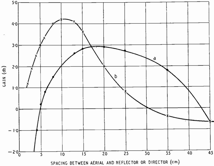
Fig. 12. Gain of  $\lambda/2$  dipole aerial with reflector (a) and director (b) over that of  $\lambda/2$  dipole without reflector.
