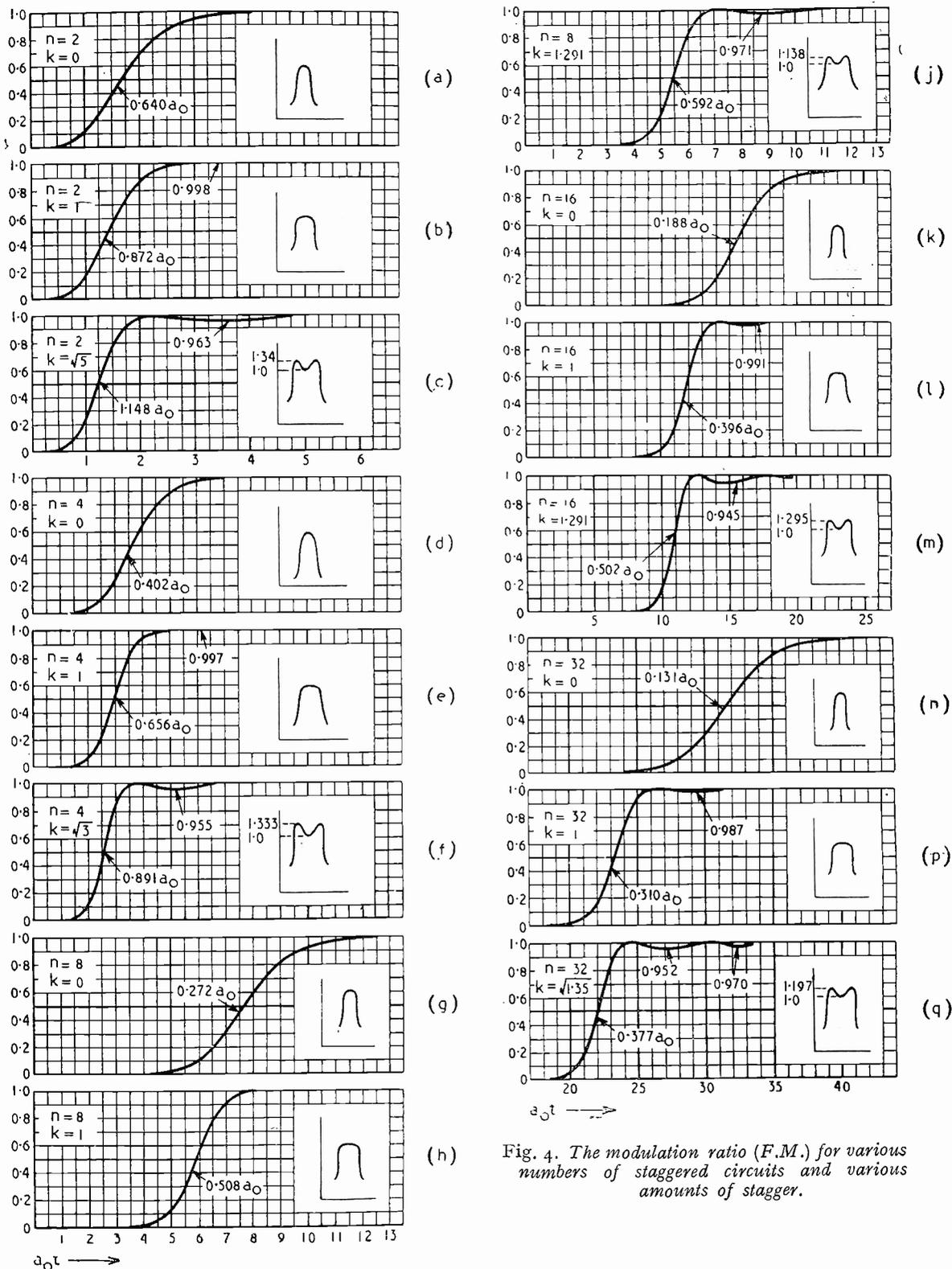
Fig. 4. The modulation ratio (F.M.) for various numbers of staggered circuits and various amounts of stagger.
