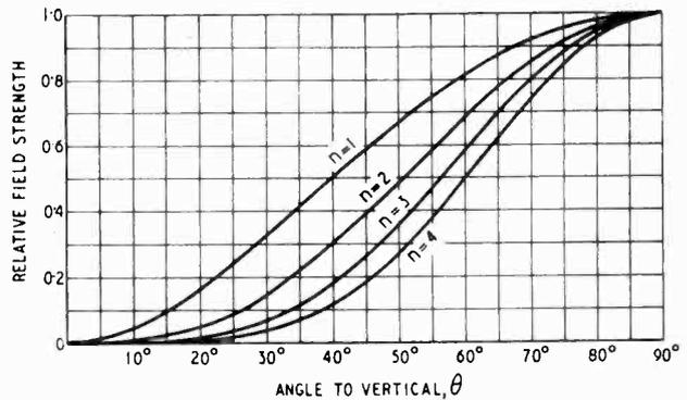
to  $A$  lags and due to  $B$  leads by an angle  $(q \sin \theta \sin \alpha - n\alpha)$ . If, therefore, the field strength due to a single vertical aerial, equal in height to the ring, and carrying a current equal to that of the ring, at an angle  $\theta$  to the vertical is  $f(\theta)$ , the field due to elements  $A$  and  $B$  is  $f(\theta) \frac{\delta\alpha}{2\pi} 2 \cos (q \sin \theta \sin \alpha - n\alpha)$ . The resultant field due to all the ring elements is therefore
