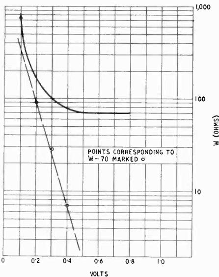
Fig. 14. *Crystal valve CV113 (silicon); forward a.c. resistance.*
