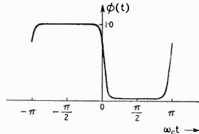
Fig. 25. Modulating function of a Cowan modulator.
