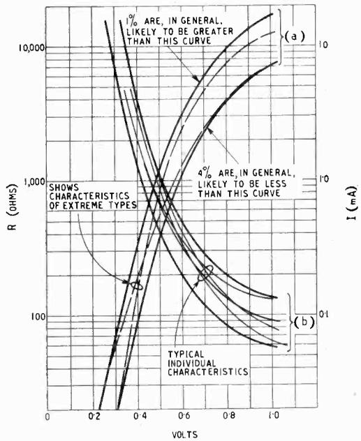
Fig. 8. Selenium rectifiers, type 7A. Curves (a) show the envelope of the V-I characteristics of 16 sample rectifiers and curves (b) give the envelope of the d.c. resistance characteristics.
