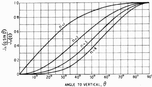
Fig. 2 (above). Curves showing modification of vertical polar diagram of a single vertical aerial for a ring radius of  $0.25\lambda$ . Total phase change round ring =  $2\pi n$  radians.
