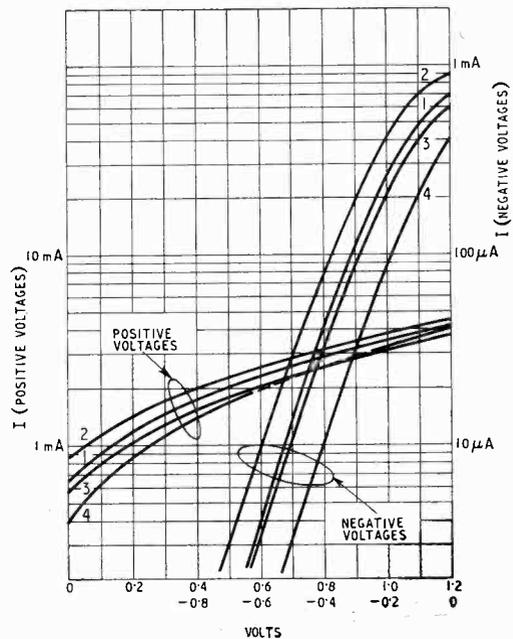
Fig. 18. Diodes type D1; V-I characteristics of four diodes (4 volts on heaters).
