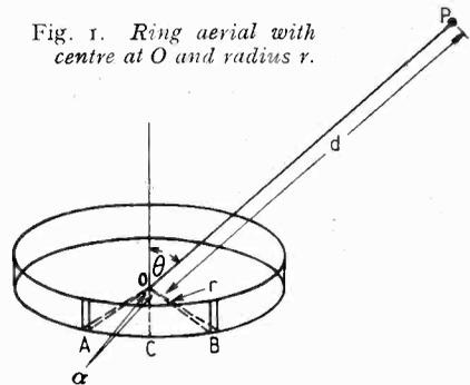
Fig. 1. Ring aerial with centre at O and radius  $r$ .
