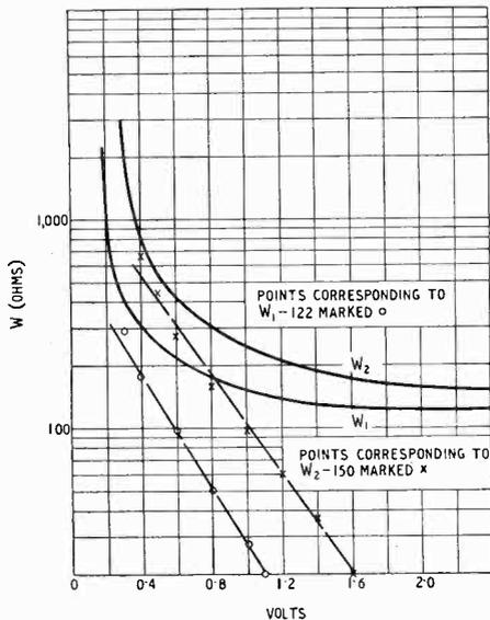
Fig. 17. Germanium crystal valves type VX4047; a.c. resistance characteristics of two sample crystals.
