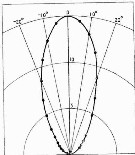
Fig. 11. Polar diagram of horn: wavelength = 9.2 cm.; H-vector plane.
