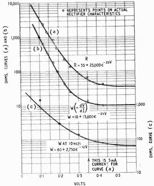
Fig. 2. Copper-oxide rectifiers. Curve (a) d.c. resistance (forward) of H1 disc; curve (b) a.c. resistance (forward) of H1 disc; curve (c) a.c. resistance of  $\frac{3}{16}$ -in diam. disc at 10 kc/s, according to Caruthers.
