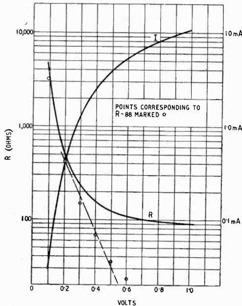
Fig. 13. *Crystal valve CV113 (silicon); forward d.c. characteristics.*
