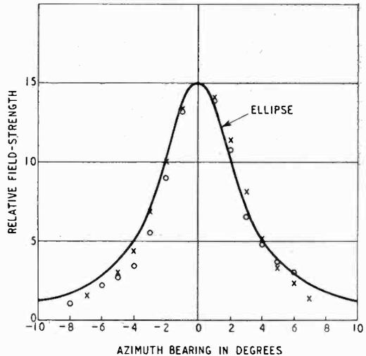
Fig. 8. Radiation pattern of paraboloid: wavelength = 6.2 cm.;  $\circ$  H - vector plane;  $\times$  E - vector plane.
