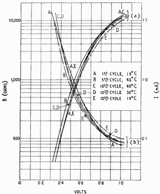
Fig. 11. Selenium rectifiers type 7A; forward  $V-I$  curves for various temperatures (a) and forward d.c. resistance (b).
