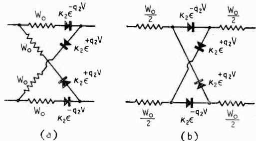
Fig. 26. Constant-impedance modulator.
