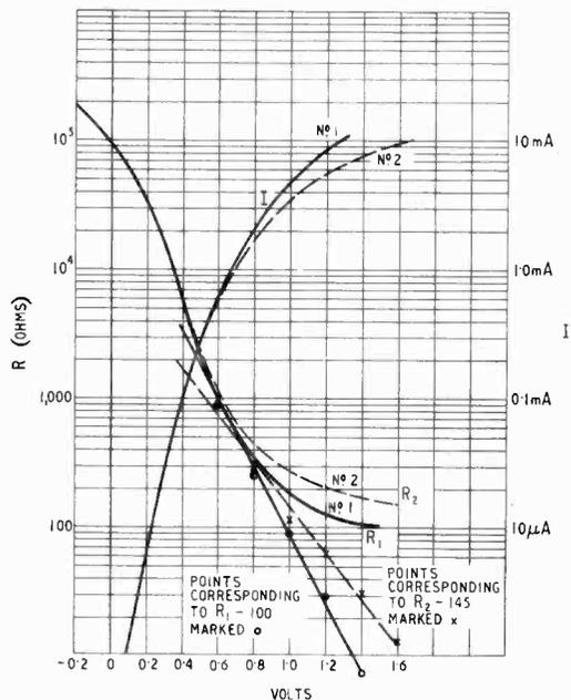
Fig. 4. D.C. characteristics (forward) after 5 temperature cycles of copper-oxide rectifiers, type G2.
