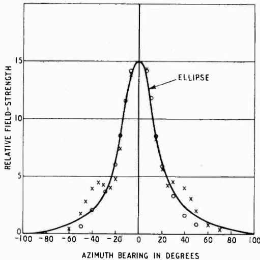
Fig. 9. Radiation pattern of horn: wavelength = 6.2 cm. ;  $\circ$  H - vector plane ;  $\times$  E - vector plane.
