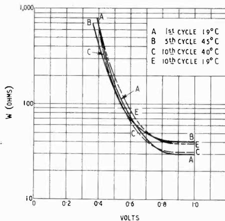
Fig. 12. Selenium rectifier type 7A; forward a.c. resistance at various temperatures.
