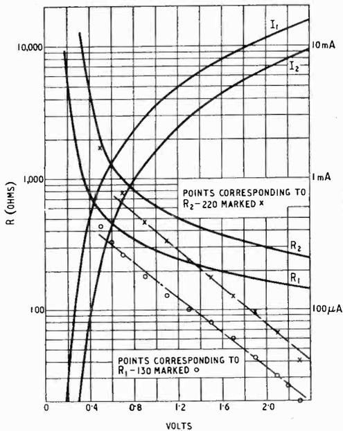
Fig. 16. Germanium crystal valves type VX4047; d.c. characteristics of two sample crystals.
