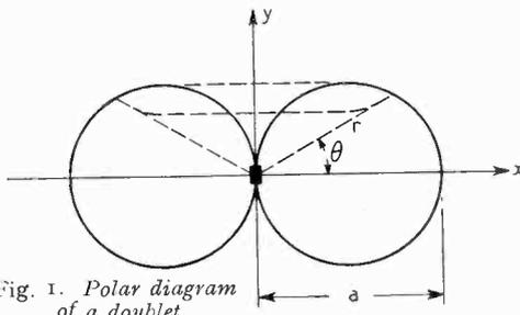
Fig. 1. Polar diagram of a doublet.
