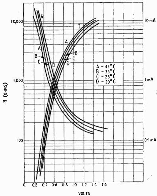
Fig. 6. D.C. characteristics at various temperatures on the 5th temperature cycle of copper-oxide rectifier type G2.
