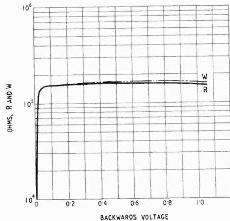
Fig. 3. Backwards characteristics of copper-oxide rectifier, type H1.
