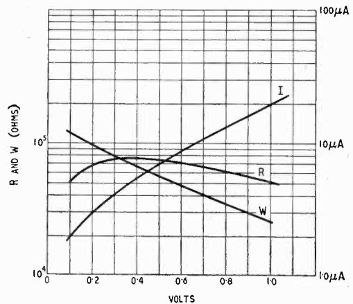
Fig. 15. *Crystal valve CV113 (silicon); backward characteristics.*
