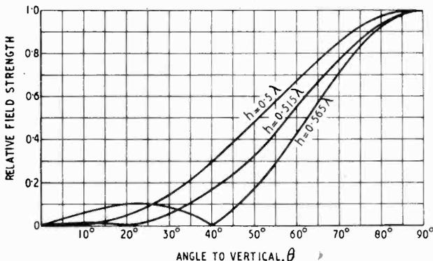
Fig. 4 (above). Vertical field-strength diagrams for a typical single anti-fading aerial, height  $h$ .
