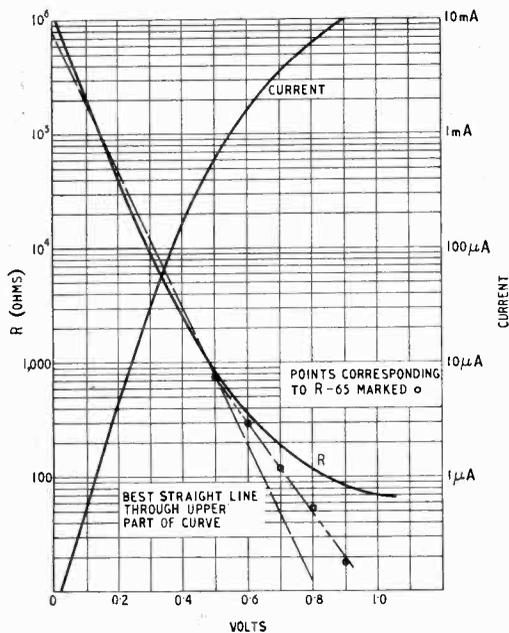
Fig. 7. D.C. characteristics (forward) of selenium rectifier type 7A.
