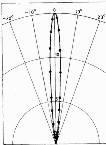
Fig. 12. Polar diagram of paraboloid: wavelength = 9.2 cm.; E-vector plane.
