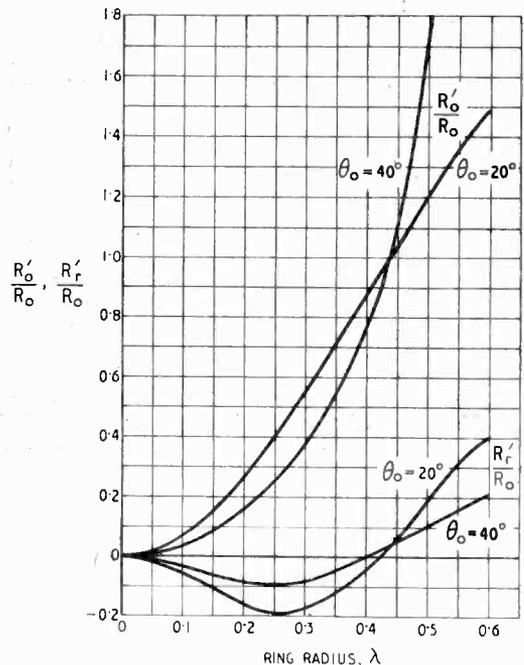
Fig. 7. Radiation resistance of central and ring aeri-als in the concentric-ring system.  $R'_0$  = effective radiation resistance of central aerial;  $R'_r$  = effective radiation resistance of ring aerial;  $R_0$  = radiation resistance of vertical aerial of same height as ring;  $\theta_0$  = angle of zero radiation.
