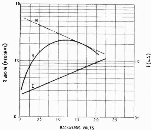
Fig. 10. Selenium rectifier type 7A; backward characteristic (N.B. Not the same rectifier as that of Fig. 7.)
