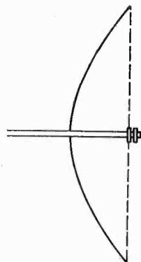
Fig. 6. Paraboloidal aerial.
