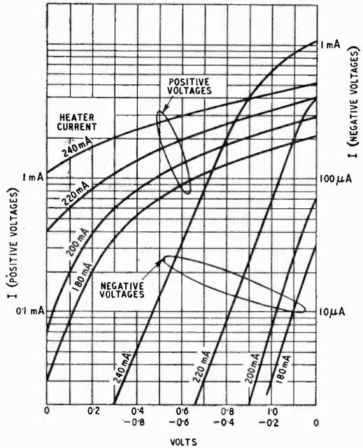
Fig. 19. Diode type D1;  $V$ - $I$  characteristics at various heater currents.
