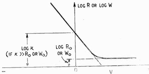
Fig. 1. The exponential resistance laws,  $R = R_0 + \kappa_1 e^{-g_1 V}$ ;  $W = W_0 + \kappa_2 e^{-g_2 V}$ .
