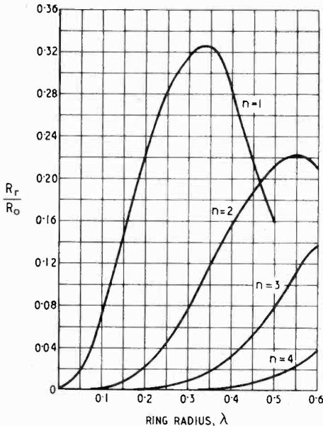
Fig. 6. Radiation resistance of phased-ring aerial system.  $R_r$  = radiation resistance of ring aerial;  $R_0$  = radiation resistance of vertical aerial of same height as ring.
