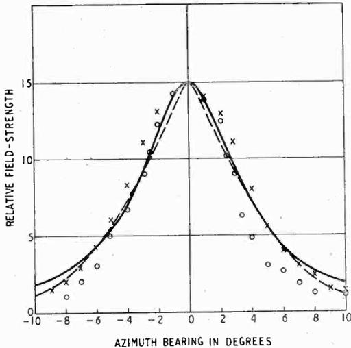
Fig. 7. Radiation pattern of paraboloid wavelength = 9.2 cm. Experimental observations:  $\circ$  H - vector plane;  $\times$  E - vector plane. Theoretical curves: — ellipse; - - - Gaussian function.
