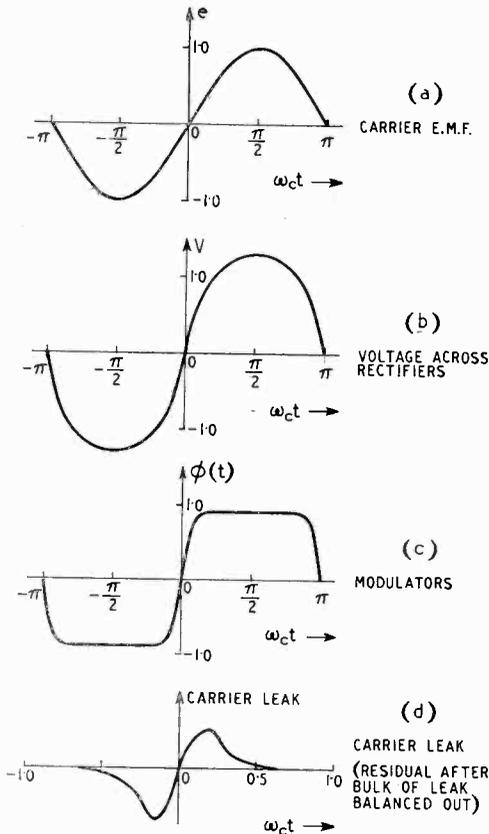
Fig. 23. The carrier e.m.f. is shown at (a); the voltage across the rectifiers at (b); the modulating function at (c); and the carrier leak voltage at (d). This last is the residual after the bulk of the leak has been balanced out.
