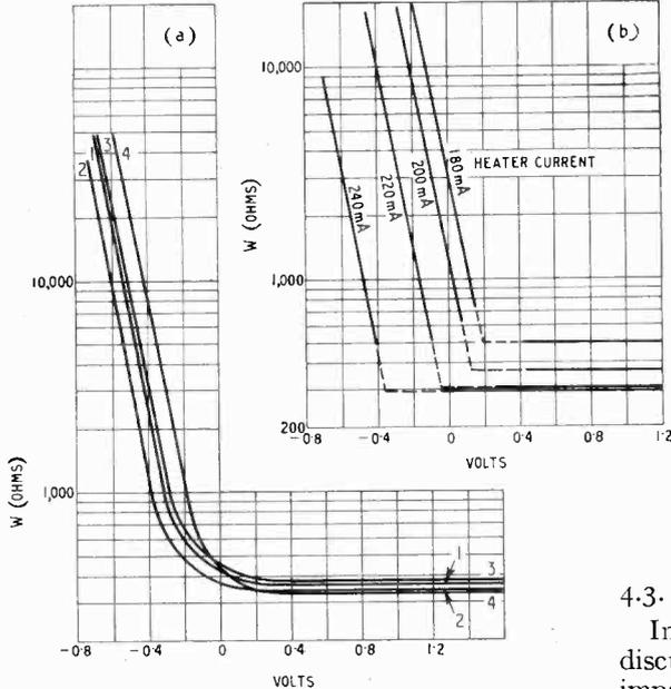
Fig. 20. Diodes type D1; (a) shows the a.c. resistance of four samples with 4 volts on the heaters and (b) shows the a.c. resistance of one diode for various heater currents.
