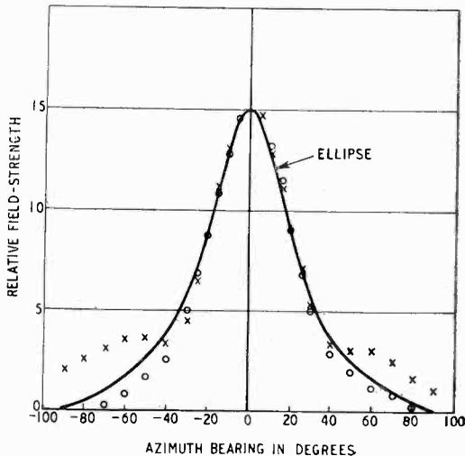
Fig. 10. Radiation pattern of horn: wavelength = 9.2 cm. ;  $\circ$  H - vector plane ;  $\times$  E - vector plane.
