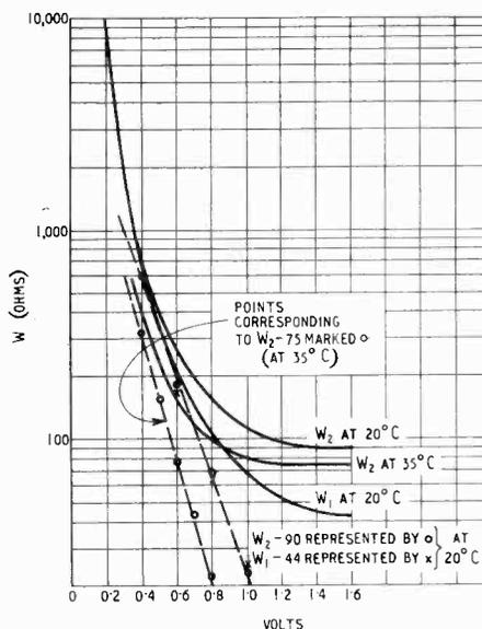
Fig. 5. A.C. resistance on 5th temperature cycle of copper-oxide rectifiers type G2.
