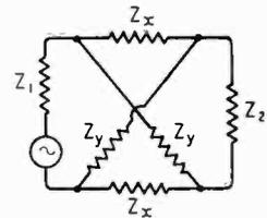
Fig. 22. Generalized transmission circuit of modulator.
