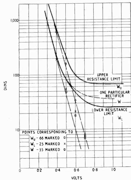
Fig. 9. Selenium rectifiers type 7A; envelope of a.c. resistance characteristics (forward) of sample of 16 rectifiers.
