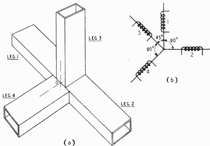
Fig. 1. The general form of a four-leg waveguide junction is shown at (a) and its transformer equivalent at (b).
