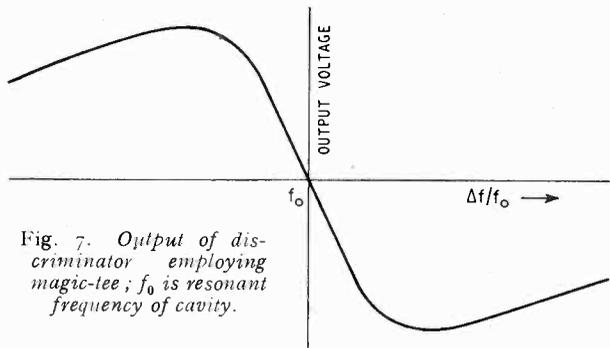
Fig. 7. Output of discriminator employing magic-tee;  $f_0$  is resonant frequency of cavity.
