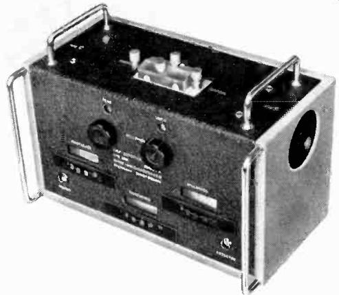
Direct-reading bridge, Type 801, for frequency range 1 to 100 Mc/s (Wayne Kerr).
