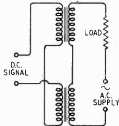
*Principle of d.c. magnetic amplifier.*
