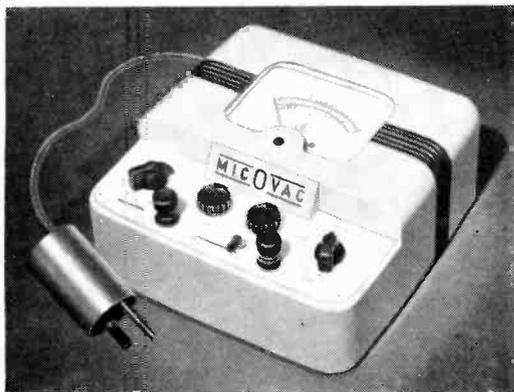
"Micovac" electronic test meter, with probe, for use up to 200 Mc/s (Electronic Instruments).
