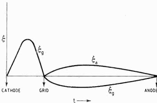
Variation of induced charge and induced current as a charge passes through the grid.
