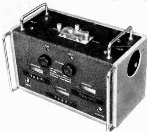
Direct-reading bridge, Type 801, for frequency range 1 to 100 Mc/s (Wayne Kerr).
