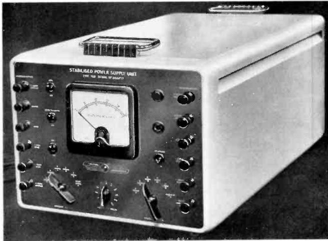
*Furzehill type 1931 stabilized power unit, with provision for metering the several positive and negative supplies.*
