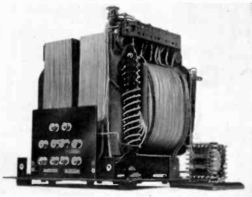
*Two examples of magnetic amplifiers by Electro Methods.*
