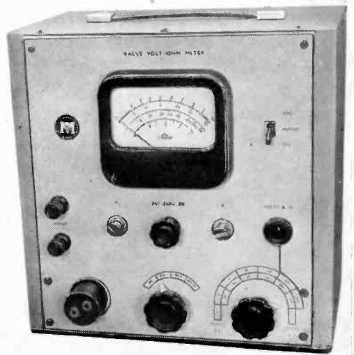
*Mullard valve volt-ohmmeter reading up to 10 kV.*
