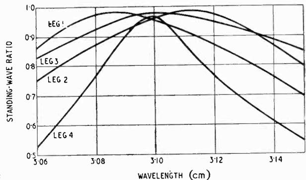
to some extent from that of a series T-junction. Considering the series-tee waveguide junction it seemed probable that transmission from the branch to the main guides could be improved by lowering the equivalent impedance of the latter to roughly half that of the side leg. The equivalent impedance<sup>3</sup> of a waveguide in the
