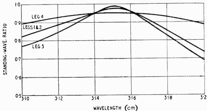
the shunt junction (that is, the reduction of the narrow dimension of legs 1, 2 and 4) and the employment of a matching rod for the series junction. The position for the metal rod is in the plane of symmetry with the free end projecting somewhat along the E-leg in the axial direction.
