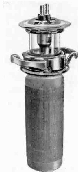
*E 1872 transmitting valve; anode dissipation up to 150 kW, frequency up to 30 Mc/s (Marconi-Osram).*
