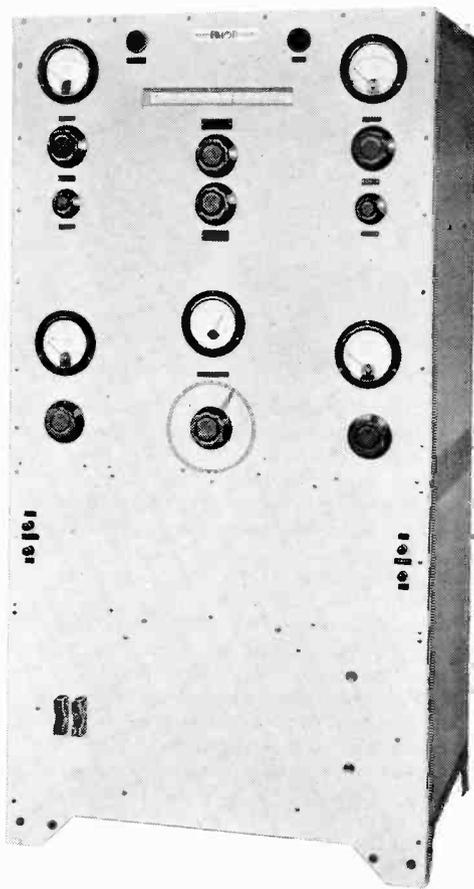
*Elliott high-stability 40-2,500 c/s current and voltage test generator.*
