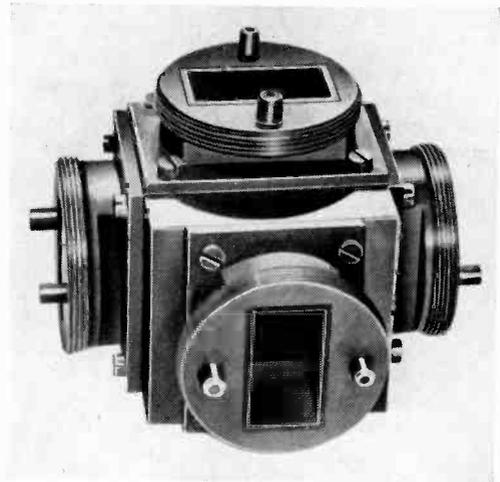
Fig. 5. Photograph of the magic-tee junction sketched in Fig. 4.
