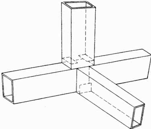
Fig. 2 (above). Inductive diaphragms are included in the waveguide legs for matching.
