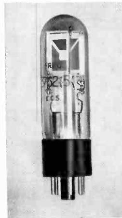
*Quartz-crystal oscillator for high-quality f.m. transmission.*
