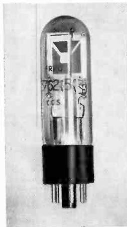
*Quartz-crystal oscillator for high-quality f.m. transmission.*
