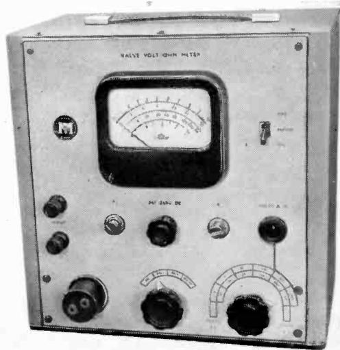
*Mullard valve volt-ohmmeter reading up to 10 kV.*
