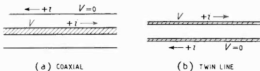
Fig. 1. Convention of sign for voltage and current. The convention shown is natural for waves travelling to the right.
