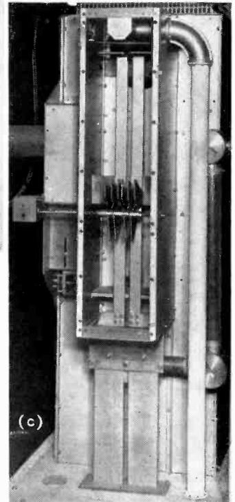
(c) Rear view of unit showing the grid-cathode line (back cover removed), with its tuning capacitor at the centre, and harmonic break-up capacitor at the upper end of the line. The pipe which runs from the air chamber at the base of the unit and enters at the top carries the cooling air for the transmitting valve filament seal. The drive input transmission line can be seen entering the grid-cathode line at a point near its short-circuiting capacitor.
