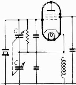
Fig. 4. Cathode-injection anti-resonant crystal-oscillator having good stability with considerable range of frequency adjustment.
