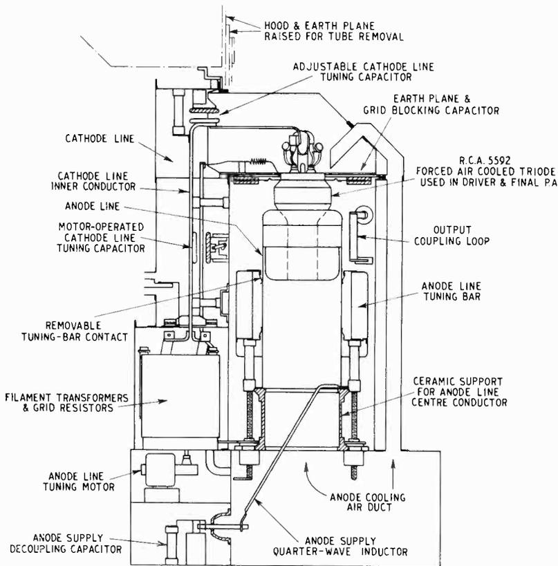
Fig. 11. General arrangement of the R.C.A. 25 kW 88/108 Mc/s frequency modulated earthed-grid coaxial-line amplifier unit. (Reproduction by permission of "Tele-Tech").
