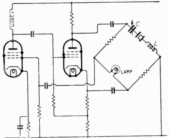
Fig. 6. Series-resonance bridge-type oscillator.
