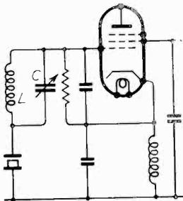
Fig. 5. Cathode-injection anti-resonant crystal oscillator with adjustable positive reactance in series with crystal, to provide the maximum range of frequency control.
