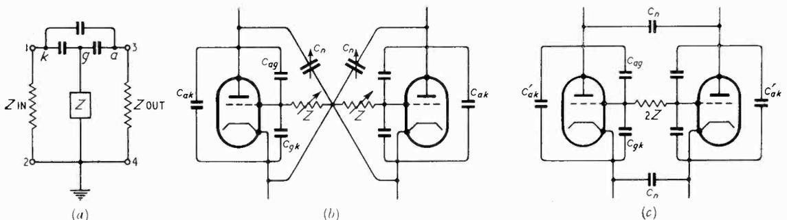
Fig. 8. (a) Equivalent network of earthed-grid amplifier in which the network is adjusted to give zero feed-through between input and output and reciprocally by the introduction of a reactance  $Z$  between grid and earth; (b) neutralization of earthed-grid amplifier for power gain control by combination of cross-connected capacitors and reactance between grids; (c) equivalent circuit of (b),  $c'_{ak} = c_{ak} - C_n$ .
