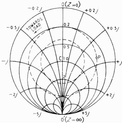
Fig. 6. The impedance mesh—resistive and reactive components.
