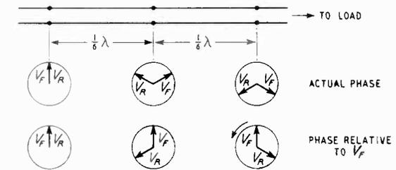
Fig. 2. Phase relations of the partial waves.
