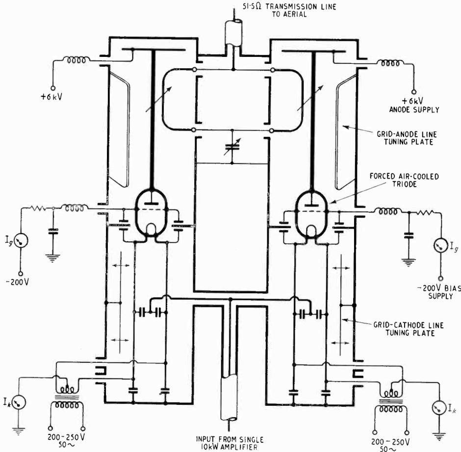
Fig. 13. 25-kW f.m. amplifier. Typical circuit arrangement of two 10-kW earthed-grid coaxial line f.m. amplifiers in parallel driven by a third 10-kW unit. In this case the tuning of the anode and cathode lines is accomplished by varying their effective  $Z_0$ .
