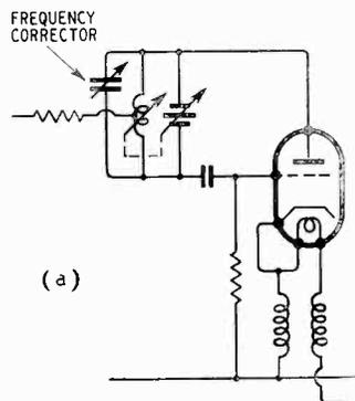
Fig. 3. Butterfly oscillator circuit (a) and mechanical forms of the semi-butterfly and true butterfly (b). The latter are shown in maximum frequency positions,  $x$  and  $y$  being the points of maximum potential difference.
