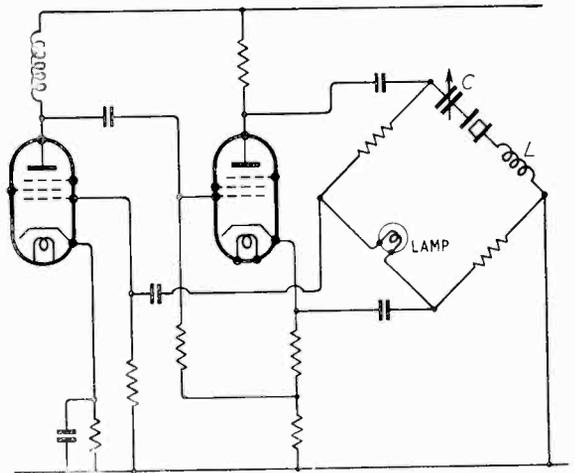
Fig. 6. Series-resonance bridge-type oscillator.
