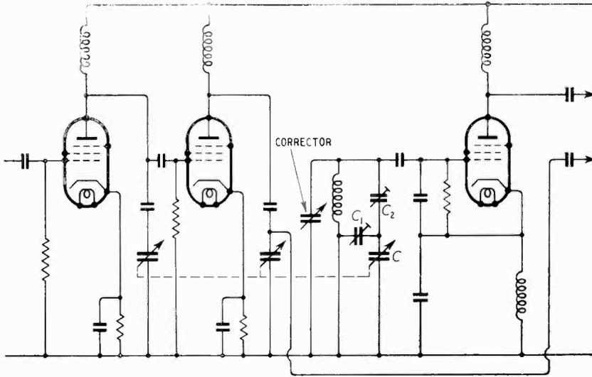
Fig. 8. 40 to 80-Mc/s amplifier oscillator unit.  $C_1$  and  $C_2$  are the tracking capacitors. The values are arranged to assist in producing linearity of the scale of main tuning capacitor  $C$ .
