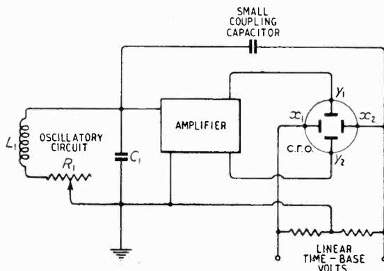
Fig. 1 Oscillatory circuit excited by linear time base.
