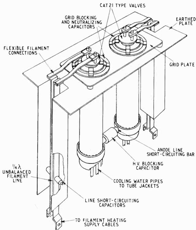
Fig. 9. Typical part arrangement of a 50-kW earthed-grid parallel-line amplifier showing the construction of the  $\lambda/4$  unbalanced lines for the filament-heating supply.
