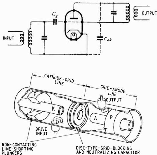
Fig. 10. Basic electrical and mechanical arrangement of earthed-grid coaxial amplifier.
