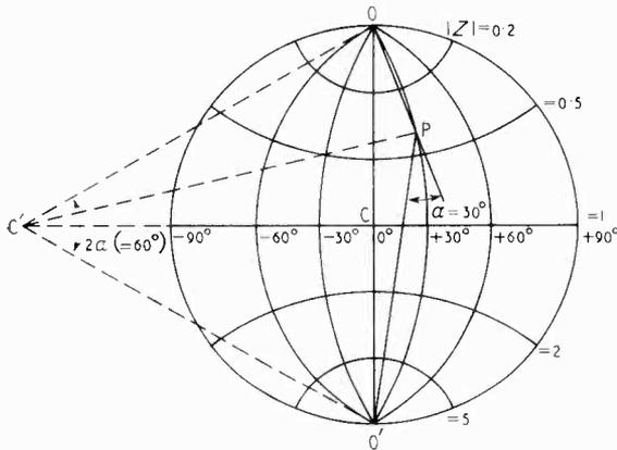
Fig. 5. The impedance mesh—magnitude and phase angle.
