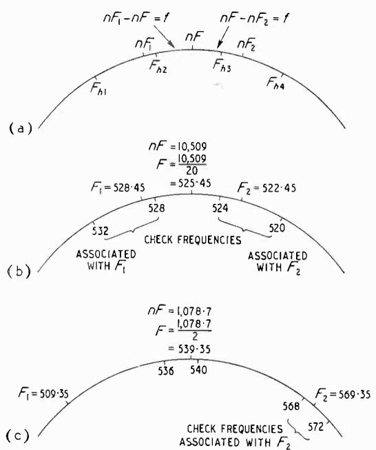
Fig. 10. Dial of reference oscillator;  $F_{h1}$  and  $F_{h2}$  are calibration check frequencies associated with channel  $F_1$ , while  $F_{h3}$  and  $F_{h4}$  are associated with channel  $F_2$ .
