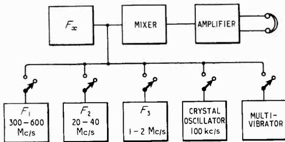
Fig. 1. Principle of usual heterodyne method of measuring high frequencies.
