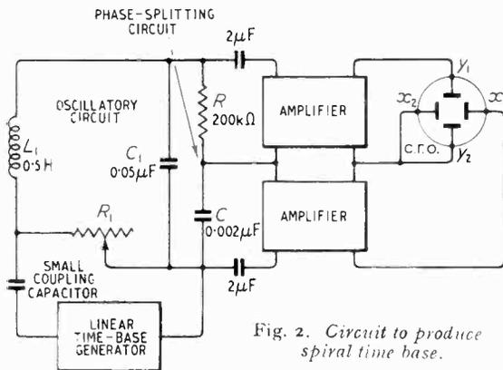
Fig. 2. Circuit to produce spiral time base.
