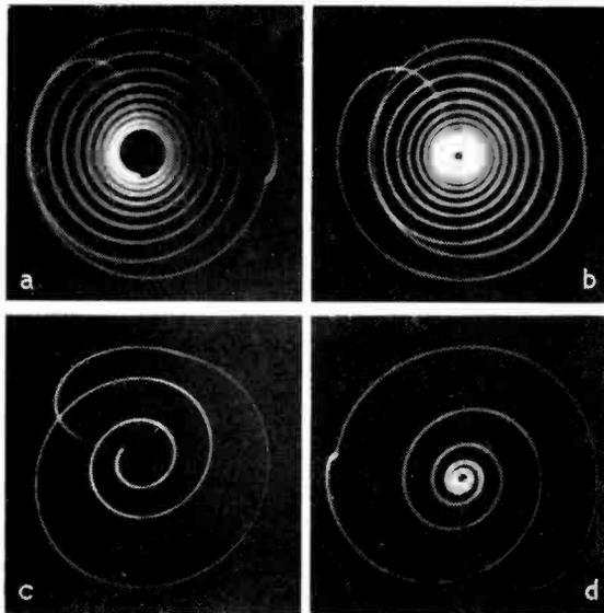
Fig. 3. Oscillograms of spirals of different frequencies: (a),  $Q = 17.1$ ,  $f = 2,280$  c/s; (b),  $Q = 16$ ,  $f = 1,950$  c/s; (c),  $Q = 13.4$ ,  $f = 1,040$  c/s; (d),  $Q = 8$ ,  $f = 780$  c/s.
