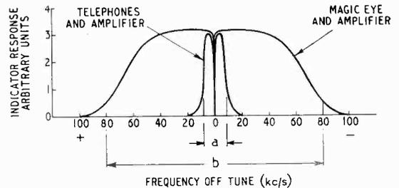
Fig. 9. This diagram illustrates the procedure for tuning to zero beat. The magic-eye indicator is used over band  $b$  of about 150 kc/s and the telephones over band  $a$  of some 15 kc/s.
