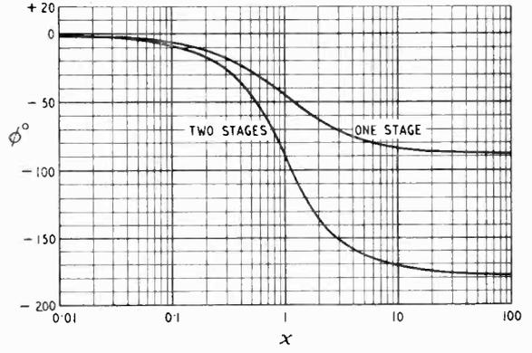
Fig. 4. Phase angle of frequency response for one and two stages.
