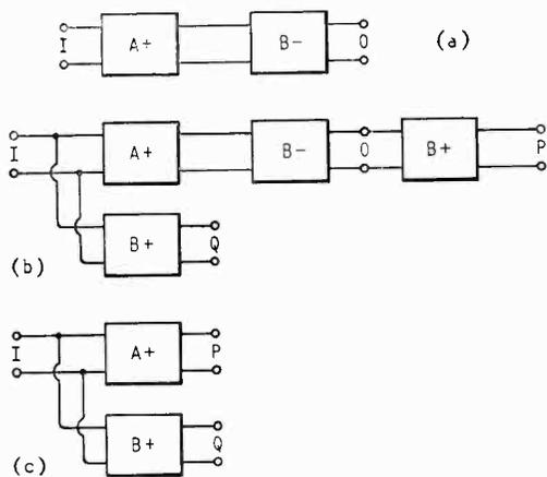
Fig. 5. Sections having positive and negative elements are grouped as at (a). The addition of two  $B+$  networks (b) leaves the phase difference between  $P$  and  $Q$  unaltered. The  $B+$  and  $B-$  networks cancel to give (c).
