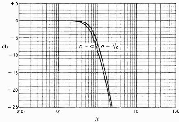
Fig. 5. Modulus of frequency response for three stages.
