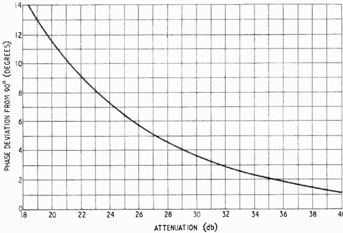
Fig. 2. Relation between phase-shift of one network and attenuation of the derived network.
