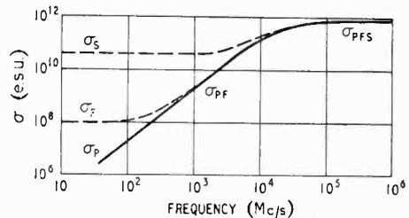
Fig. 3. Conductivities  $\sigma_p$ ,  $\sigma_p F$  and  $\sigma_s$  of pure, fresh and sea water; temperature 20°C.
