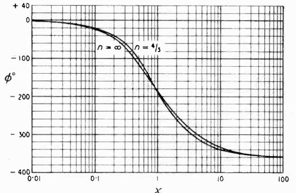
Fig. 8. Phase angle of frequency response for four stages.
