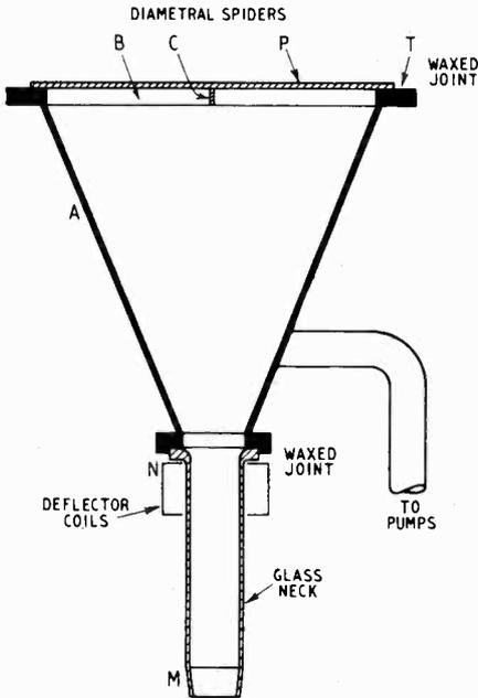
Fig. 4. Sketch showing possible construction of a metal-glass tube.
