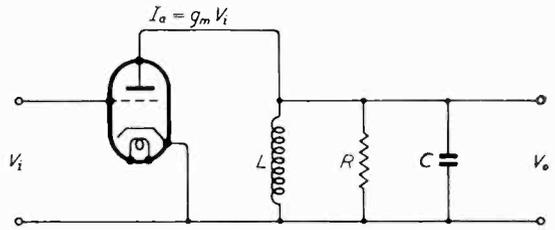
Fig. 1. Tuned amplifier stage.
