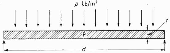
Fig. 5. Calculation of screen thickness.
