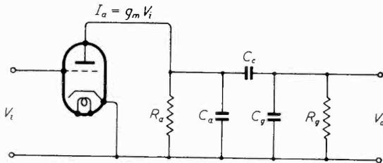
Fig. 2. RC-coupled amplifier stage.
