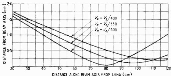
Fig. 3. Calculated space-charge-limited trajectories for  $E = 15$  kV,  $I = 150$   $\mu$ A and a beam diameter in the focusing lens of 4 mm.
