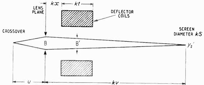
Fig. 2 (right). Beam dimensions of the derived tube.
