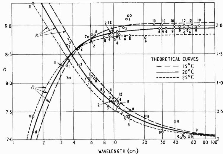
Fig. 1. Dielectric properties of water in the wavelength range 1 cm to 1 m; key to experimental observations:— 1. Abadie 15° C; 2. Esau & Bätz 19° C; 3. Conner & Smyth 25° C; 4. Cooper 22° C; 5. Szeberger 16° C; 6. V. Ardenne 18° C; 7. Eckert 15—20° C; 8. Knevr 22° C; 9. Weichmann 17° C; 10. Frankenburger 17° C; 11. Saxton 20°, 25° C; 12. V. Hippel 20° C.
