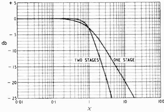
Fig. 3. Modulus of frequency response for one and two stages.
