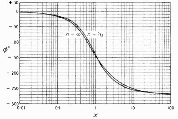
Fig. 6. Phase angle of frequency response for three stages.
