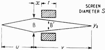
Fig. 1 (above). Essential beam dimensions of prototype tube.
