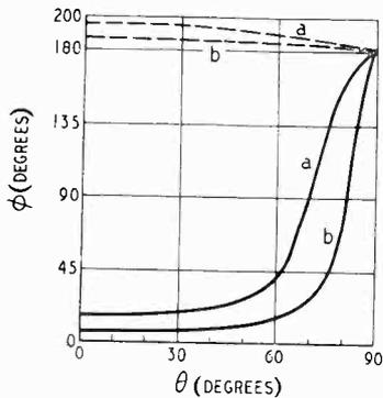
Fig. 6. Phase retardation on reflection at a fresh-water surface; temperature 20° C. Curves a and b are for wavelengths of 1 mm and 1 cm respectively. --- polarization perpendicular to plane of incidence ( $\phi_H$ ), — polarization parallel to plane of incidence ( $\phi_V$ ).
