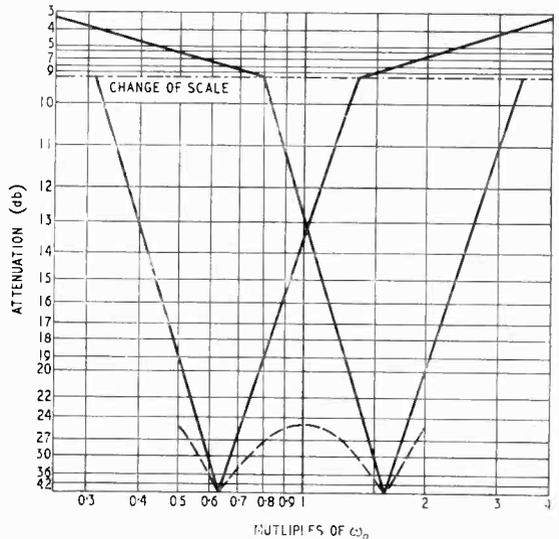
Fig. 4. Two sections in tandem with peaks at  $0.625 \omega_0$  and  $1.6 \omega_0$  (solid lines) give the response shown dotted.
