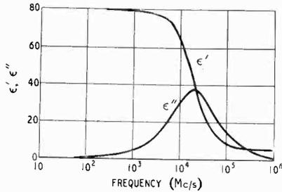
Fig. 2. Components  $\epsilon'$  and  $\epsilon''$  of the complex dielectric constant of pure water,  $\epsilon' - j\epsilon''$ , at a temperature of 20°C.
