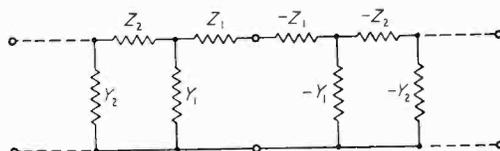
Fig. 6. This diagram illustrates how positive and negative networks in tandem cancel out.
