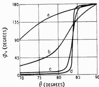
Fig. 5. Phase retardation,  $\phi_v$ , on reflection at a fresh-water surface of waves polarized in the plane of incidence as a function of angle of incidence  $\theta$ ; temperature  $20^\circ\text{C}$ . Curves a, b, c and d are for wavelengths of 1 mm, 1 cm, 10 cm and 6 m respectively.
