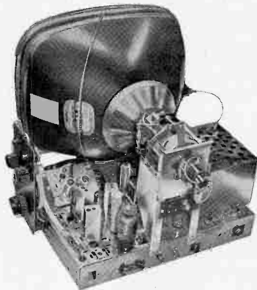
Chassis of McMichael receiver with 17-in. tube
