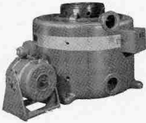
Goodmans VG109 vibration generator. Peak force generated is 9,900 lb at 20 c/s
