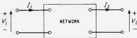
Fig. 1. The two-terminal-pair network has a matrix which is defined in terms of the input and output voltages and currents
