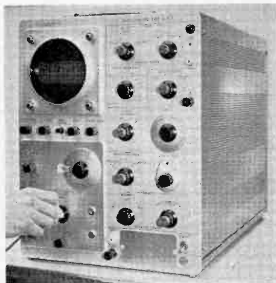
E.M.I. WM7 wide-band general-purpose oscilloscope. The Y frequency response is d.c. to 50 Mc/s ( -3 dB) using a plug-in Y amplifier giving 100\text{ mV}/\text{cm} deflection sensitivity
