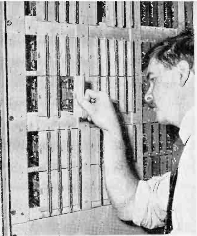
Plug-in units are used in the E.M.I. Editec 2400 computer. Printed circuits and transistors are employed
